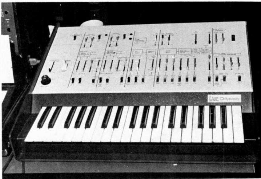
Fig. 12. ARP Odyssey synthesizer can route two keyboard voltages simultaneously to separate oscillators.
