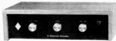
This unit is used by connecting its inputs to the speaker output terminals of the existing stereo amplifier. The output signals from the stereo amplifier are decoded, then amplified in a power output stage to drive two additional speakers for full Quadraphonic reproduction.
