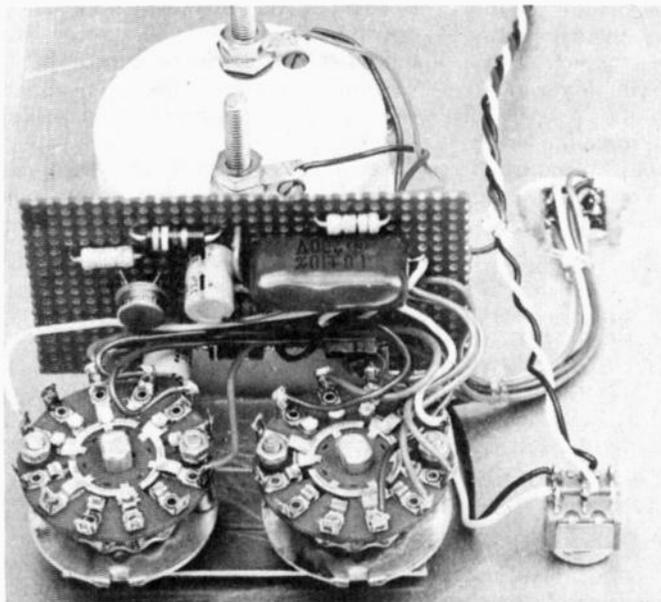
Showing the internal construction of the tester. Note that matrix board hold the majority of the components.
