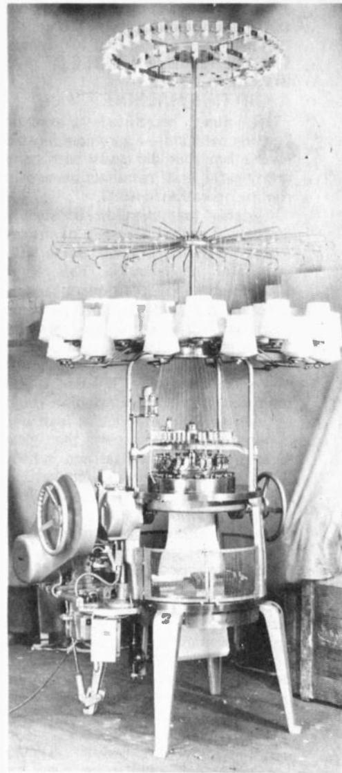
over tensioning and guidance heads then down into the centre of the circular knitting head. The knitted material is pulled off with the roller seen underneath the main frame. The mechanism is powered by an electric motor.
