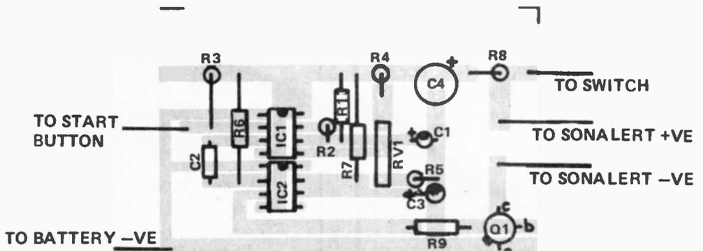
Fig. 4. Component overlay.
