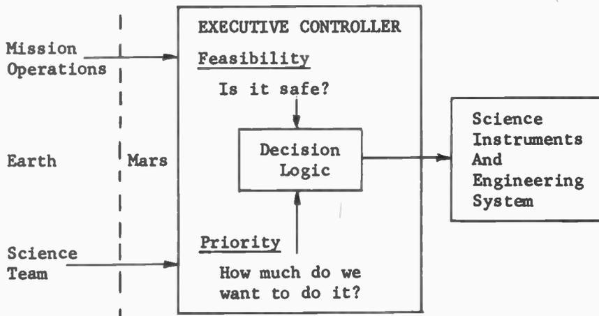
*Typical control system. On-board executive controller monitors data relating to robot's environment, ie, internal and external temperatures, power availability, wind speed, terrain, instrumentation condition etc, it then compares this against stored data relating to mission priority and desirability and then decides whether or not mission should proceed. The robot's decisions can at any time be overridden or modified by earth-based mission operating centre.*
