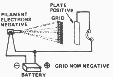
Fig. 9. The triode valve, invented by Lee De Forest, and a schematic of how it works.
