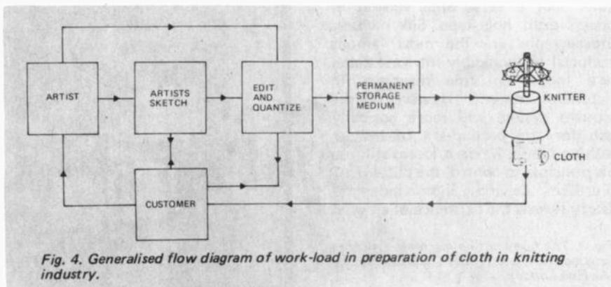
Fig. 4. Generalised flow diagram of work-load in preparation of cloth in knitting industry.
