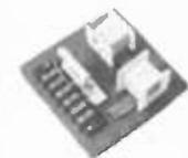
MODEL CN3 — is a three-way L-C crossover for woofer, mid-range and tweeter with crossover frequencies of 500 Hz and 4kHz at 8 ohms. Power handling 30W R.M.S. Chokes are pre-wound and full instructions are supplied. Kit Price **\$8.90 post \$1**
