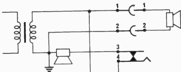
Fig. 1a. Example of using the type 05 connector inserted in position A. Both speakers are operational.
