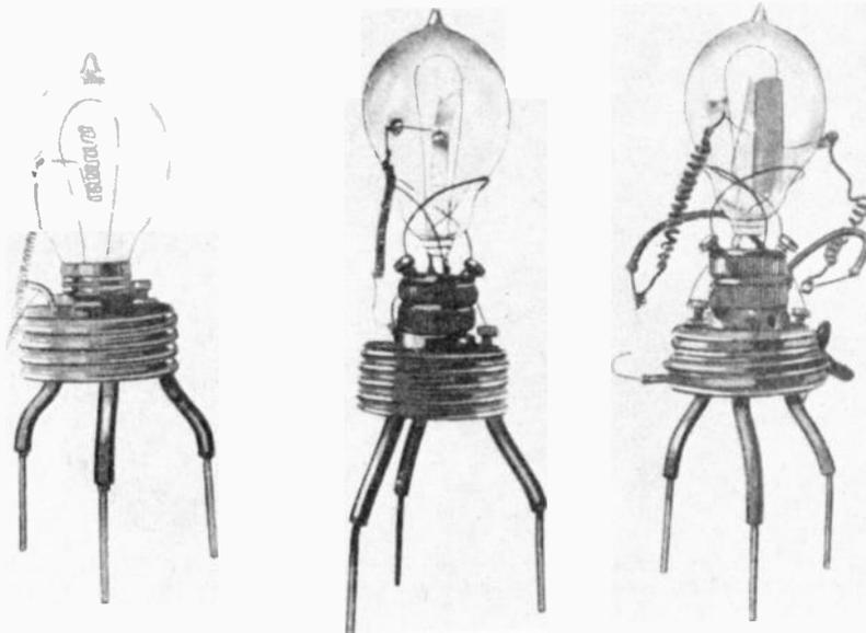
Fig. 8a. The Edison effect (b) Three of the actual diode valves used by Fleming in 1904.
