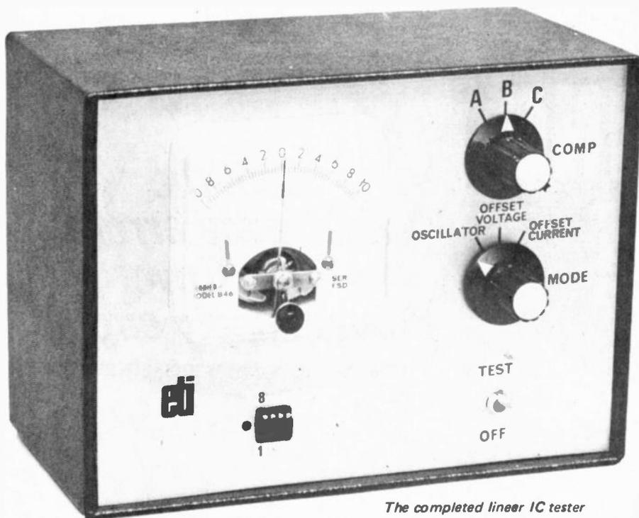
The completed linear IC tester
