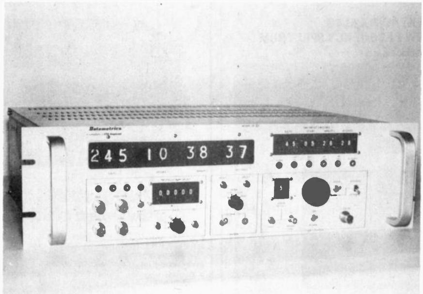
Datametrics is pleased to announce their Model SP-125 Universal Time Code Generator that is designed to serve as a Master Time Reference for distributing precision time code indices for indexing different recording mediums such as magnetic tape, camera film, and oscillographs.
