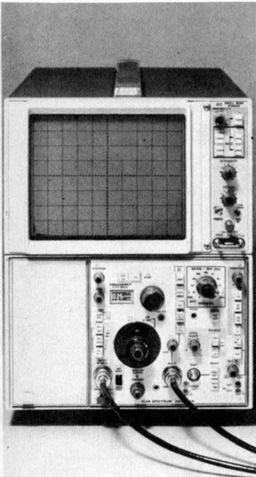
The new 5L4N is a 0-to-100 kHz spectrum analyzer that offers both high performance and economy. Tektronix state that the analyzer has unique features including push-button selection of 50 ohm, 600 ohm or 1 megohm input impedance with calibration appropriate to the selected impedance.
