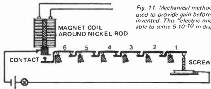
Fig. 11. Mechanical methods were often used to provide gain before valves were invented. This "electric micrometer" was able to sense  $5 \cdot 10^{-10}$  m displacements.
