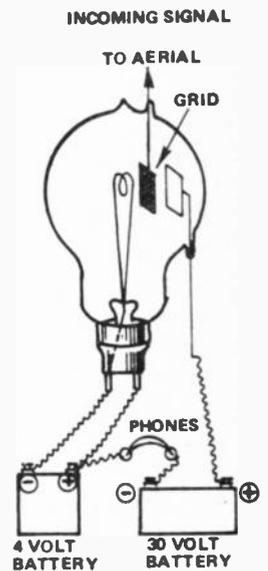
filament (cathode) and the plate (anode) if the grid is left unconnected. Signals connected to the grid either allow or prevent this action depending upon their polarity and magnitude — as shown in Fig. 9. A small varying signal voltage applied to the grid controls the flow of a large current in the anode circuit, thus obtaining gain (by producing a signal larger than that fed in).
