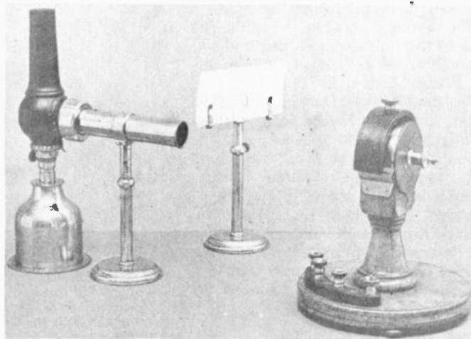
Fig.5. Kelvin's mirror galvanometer (1858). The oil lamp, at left, provided a light beam that was deflected by a mirror mounted on the coil of the galvanometer at right. The deflected beam moved across the calibrated scale at centre.
