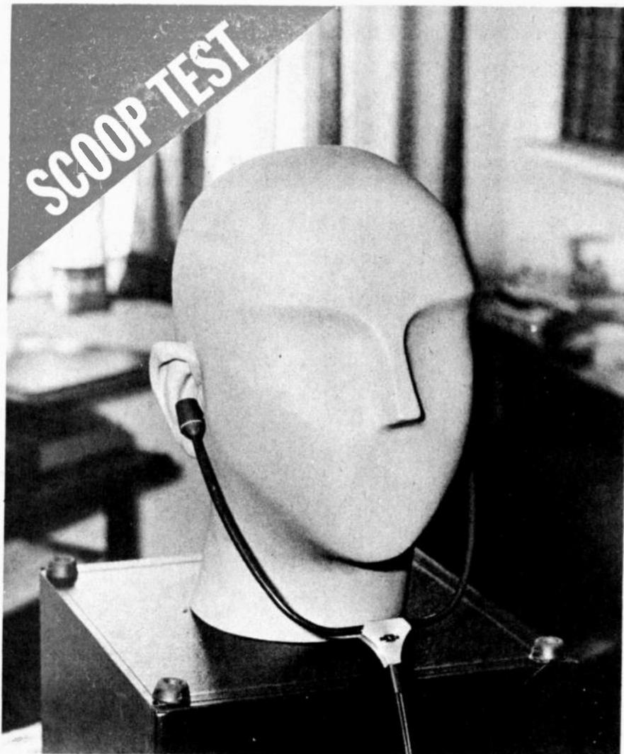
◀ *The Dummy Head with microphone assembly in position. Recordings may be made either by using the Head as shown here — or by wearing the microphones oneself.*
