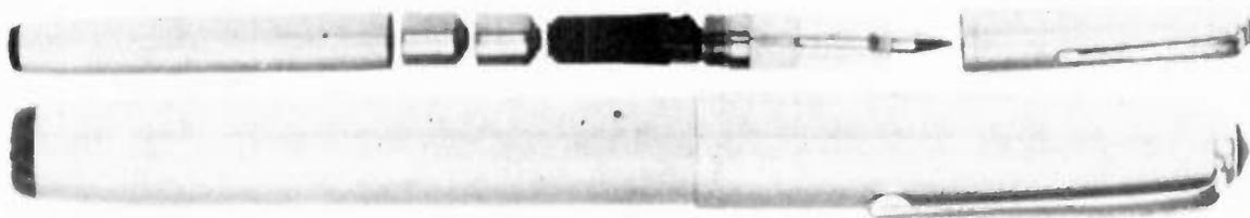
*This apparently harmless-looking pen is in fact an FM bug. The microphone is in the top half — transmitter, antenna and batteries in the lower half. Capable of operating continuously for three days on one set of batteries, this bug is claimed to have a range exceeding 100 metres.*
