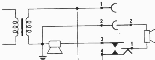
Fig. 1b. With the connector reversed, in position B, the internal speaker is disconnected.
