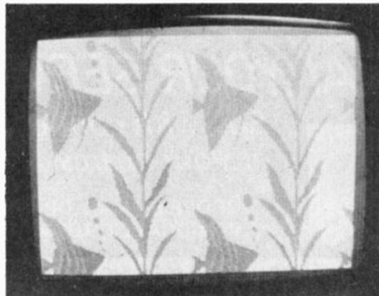
Fig. 7. The designer needs only to produce one cycle of the pattern — the computer-based colour display repeats it to provide a view of the complete pattern.
