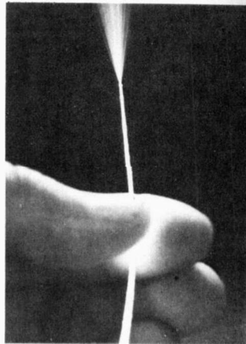
Like water from a hose, light pours out of the end of this nearly one kilometre length of light fibre.
