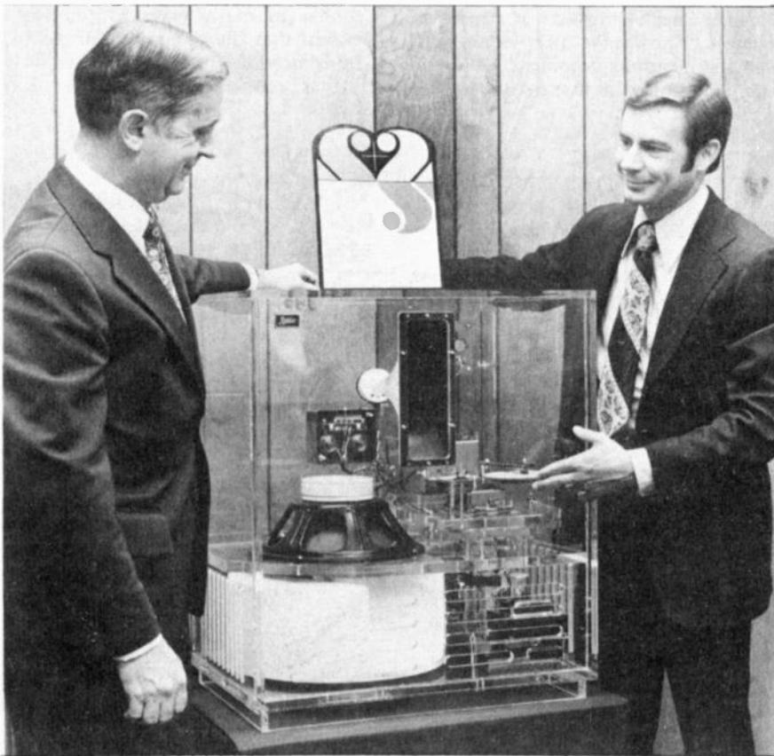
*The rotating baffle under the bass driver in Leslie's Plus 2 enclosure causes sound to 'sweep' the room, thus eliminating standing waves.*
