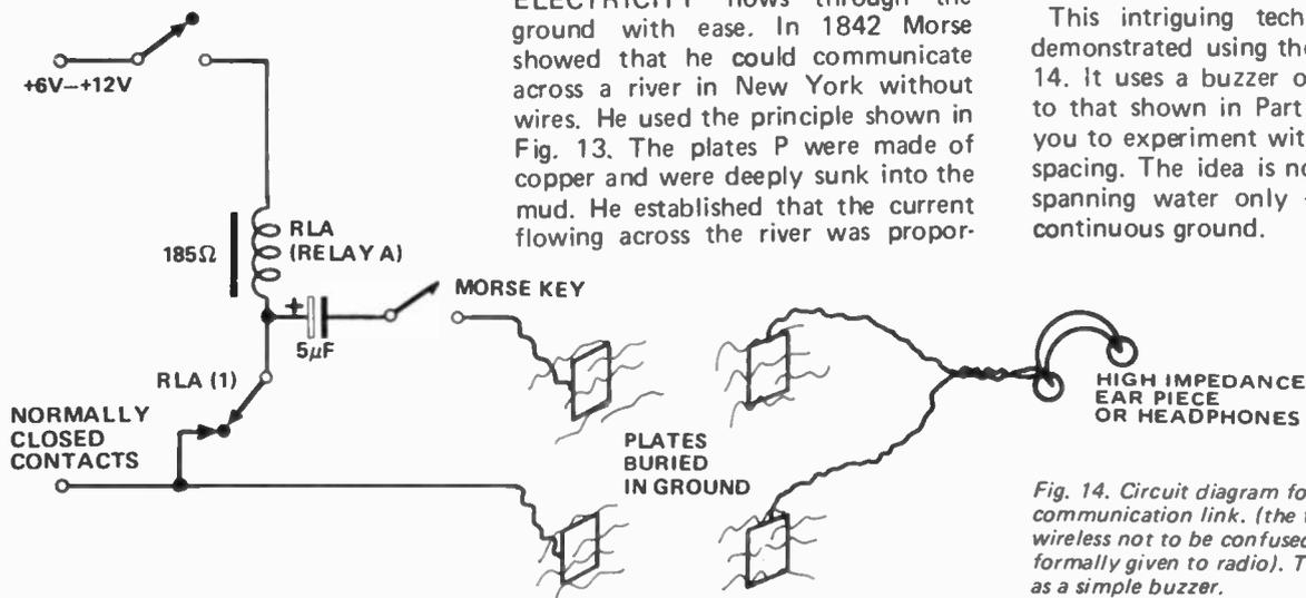
Fig. 14. Circuit diagram for a wireless communication link. (the term wireless not to be confused with the name formally given to radio). The relay acts as a simple buzzer.
