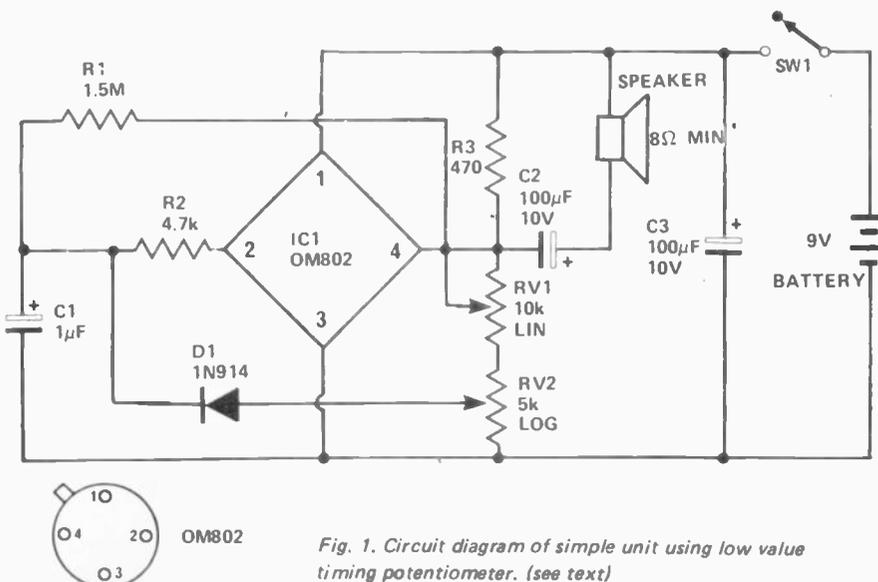
Fig. 1. Circuit diagram of simple unit using low value timing potentiometer. (see text)
