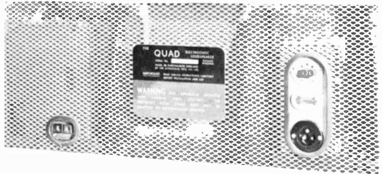
The warning is needed – there's 5000 volts behind the mesh panel.
