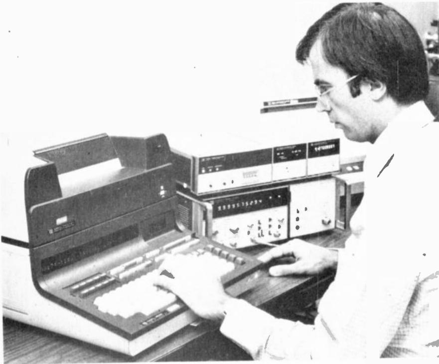
A quiet new thermal printer, Model 5150A from Hewlett-Packard, accepts data from BCD (binary coded decimal) or ASCII sources and prints up to 20 columns of alphanumeric information. Modular in construction, it is available in many different configurations including some in which it functions as an instrument-system controller.
