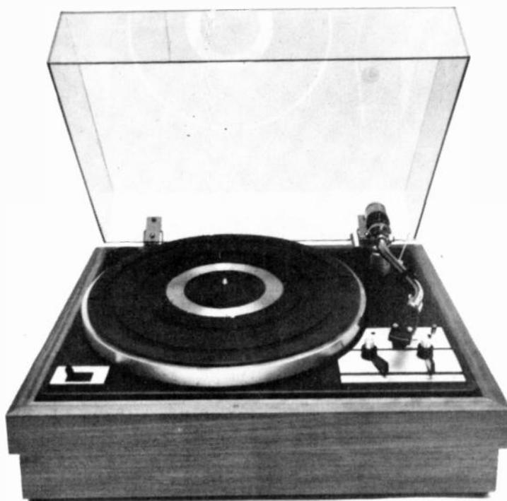
The Apan BFU-121 fully automatic CD4 ready turntable is a must for those who want the ease of automatic listening pleasure. It employs the following features – 4 pole synchronous motor – wow and flutter less than 0.16% W.R.M.S. – Signal to noise ratio better than 52 dB, – 12" diecast aluminium platter, weight 1.3kg – Static balance "S" type tone arm with anti skate device. Independent hydraulic lift. It comes complete with cartridge. Freq. 20-20,000 Hz.
