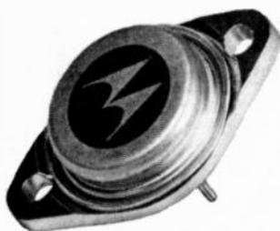
equipment had to use devices that were often only specified for resistive loads at room temperature operation. But real applications do not always conform to such simple constraints. Consequently, the designer was faced with the task of using minimally-specified power devices that had to operate at high temperature and had to control reactive loads. The characterisation of the Switchmode devices will alleviate the designer of such problems.
