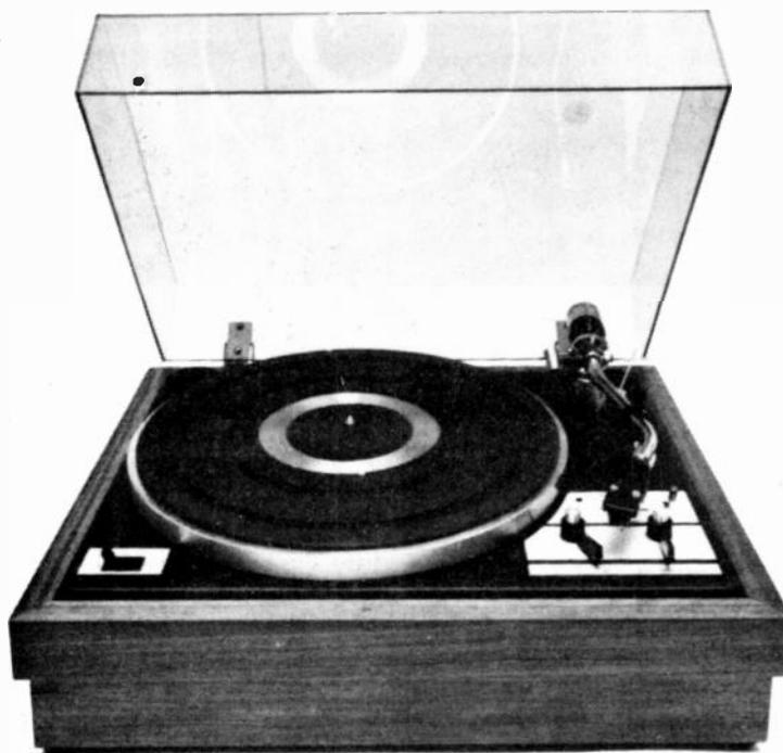
The Apan BFU-121 fully automatic CD4 ready turntable is a must for those who want the ease of automatic listening pleasure. It employs the following features — 4 pole synchronous motor — wow and flutter less than 0.16% W.R.M.S. — Signal to noise ratio better than 52 dB, — 12" diecast aluminium platter, weight 1.3kg — Static balance "S" type tone arm with anti skate device. Independent hydraulic lift. It comes complete with cartridge. Freq. 20-20,000 Hz.
