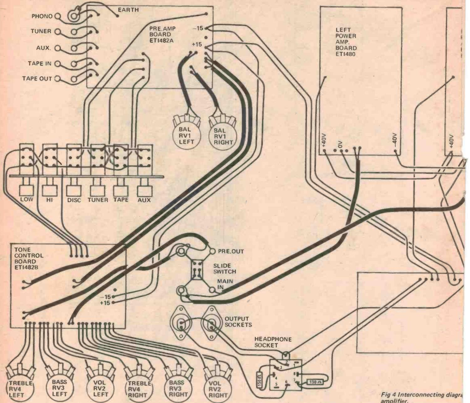
Fig 4 Interconnecting diagram for amplifier.
