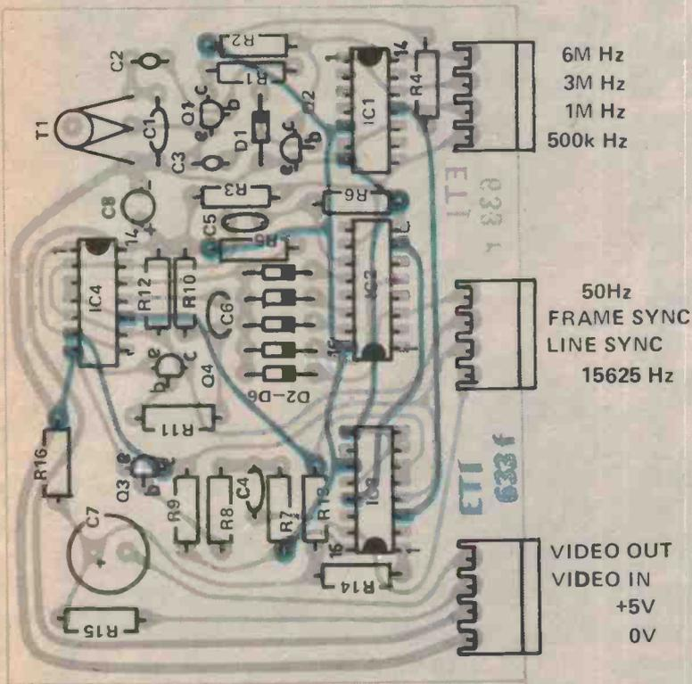
Fig. 2. Component overlay.
