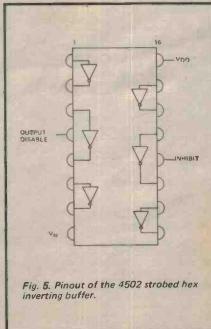
Fig. 5. Pinout of the 4502 strobed hex inverting buffer.
