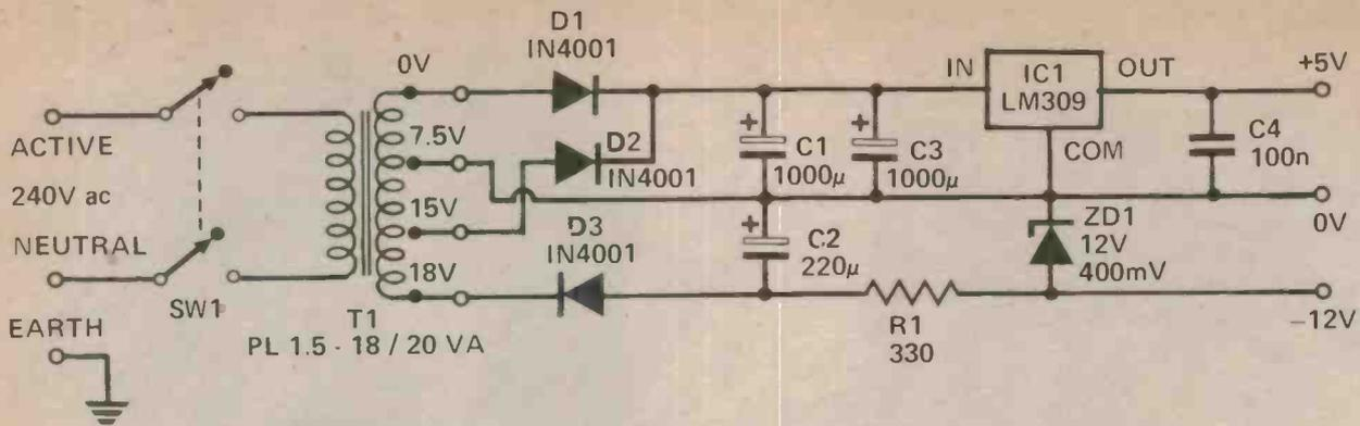
Fig. 3. Circuit diagram of the power supply.
