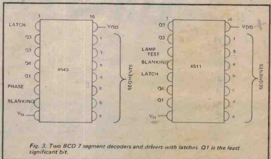
Fig. 3. Two BCD 7-segment decoders and drivers with latches. Q1 is the least significant bit.
