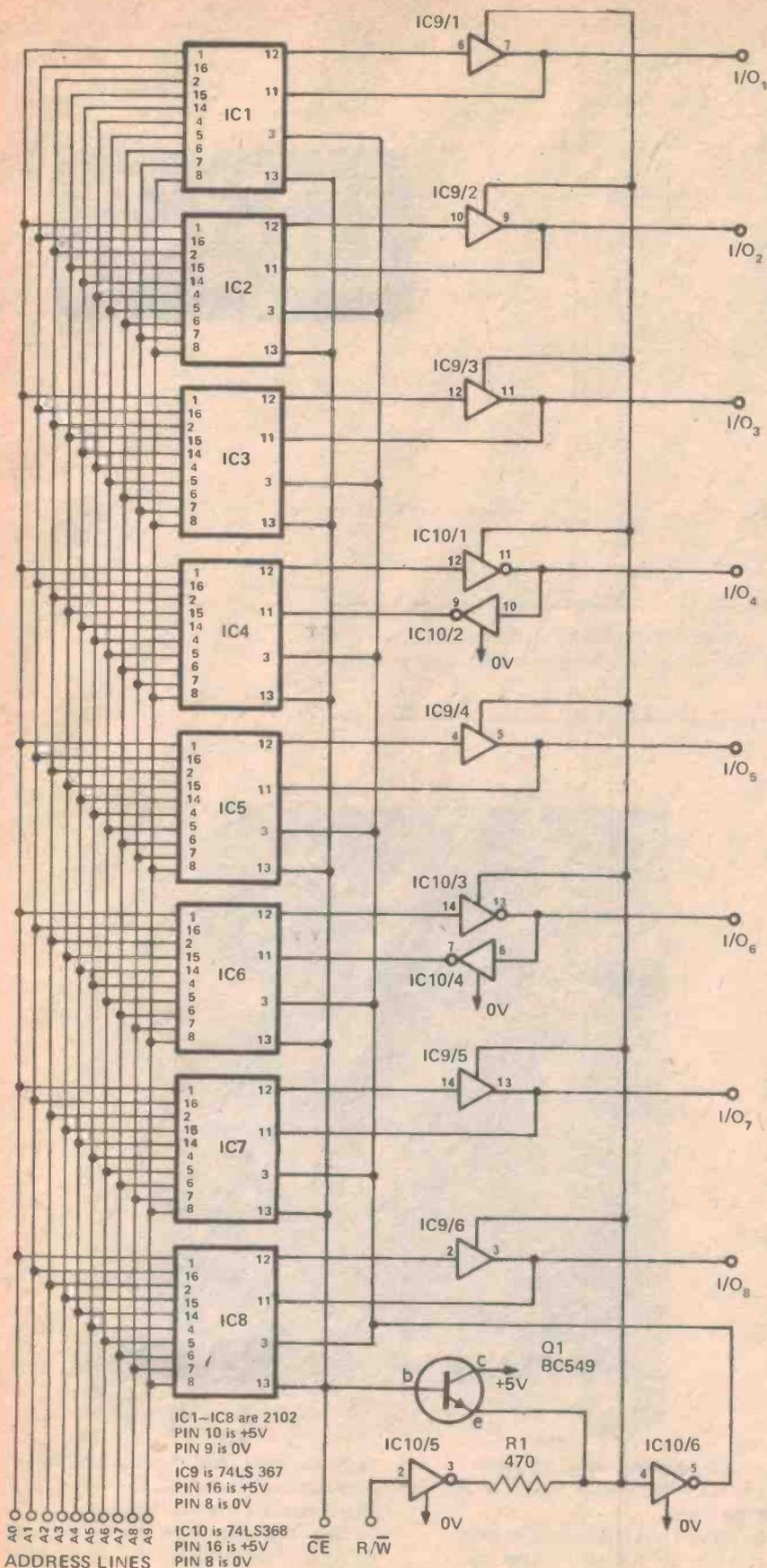
Fig. 1. Circuit diagram of the memory board.
