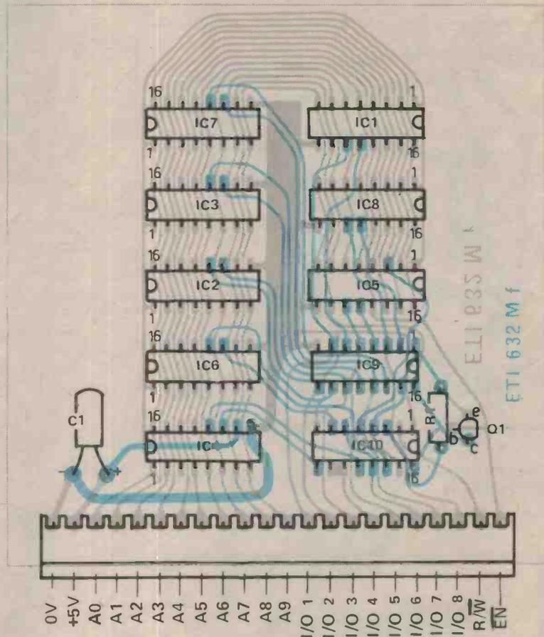
Fig. 4. Component overlay of the memory card.
