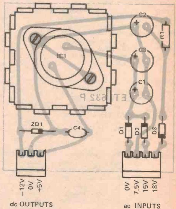
Fig. 6. Component overlay of the power supply board.
