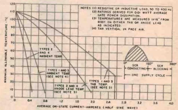
Graph 2. Maximum Allowable Temperatures for Half Sine Wave On-State Current.
