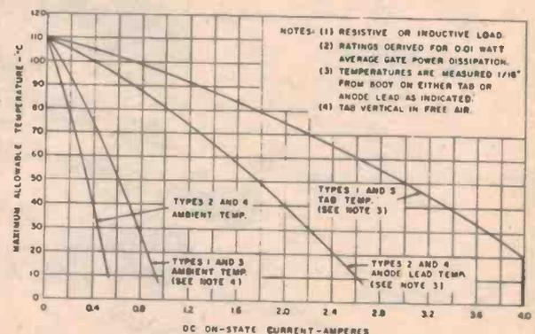
Graph 3. Maximum Allowable Temperatures for DC On-State Current.
