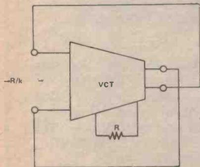
Fig. 5. VCT working as a negative resistance.
