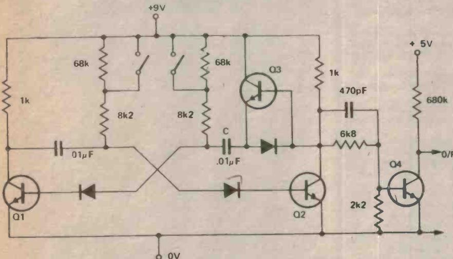
The circuit shown above generates a clean square-wave with very fast rise and fall edges; such a signal is essential for some applications such as the testing of amplifier transient responses, and the reliable driving of TTL.
