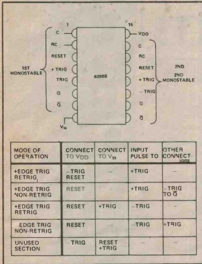
Fig. 4. The 4098B dual monostable multivibrator and method of achieving different modes of operation.
