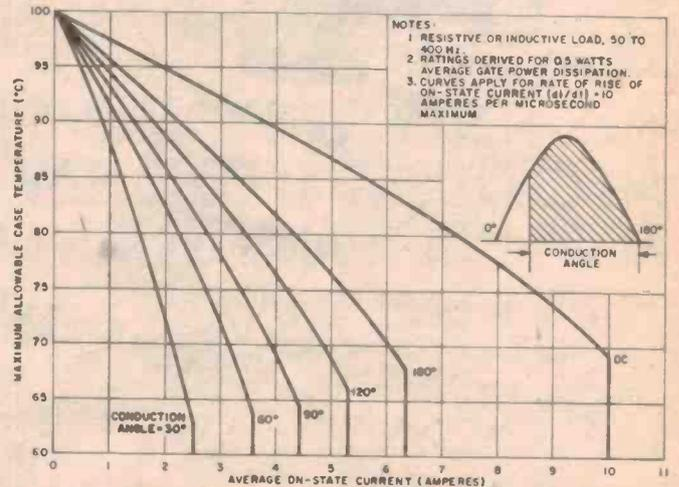
Graph 1. Max. Allowable Case Temperature For Half-Wave Rectified Sine Wave of Current.
