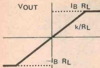
Fig. 11. Characteristics of the circuit in Figure 10.
