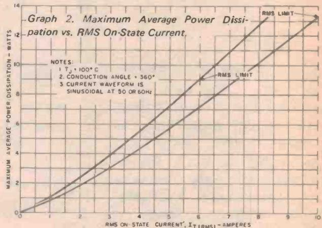
Graph 2. Maximum Average Power Dissipation vs. RMS On-State Current.
