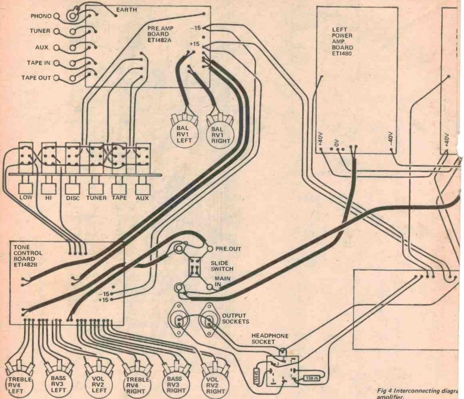
Fig 4 Interconnecting diagram of stereo amplifier.
