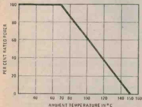
Fig. 1. Derating curve for most common metal glaze resistors — common to the majority of film resistors.
