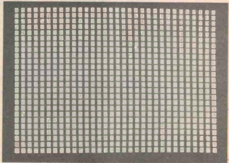
Test pattern with the ROM removed.
