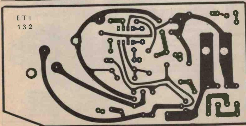
Fig 5. Printed circuit layout.
