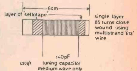
Fig. 2. Coil winding details
