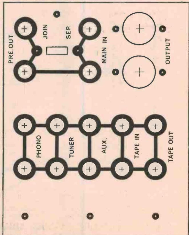
Fig 8. Printed circuit layout of the tone control board. Full size 110 x 80 mm.
