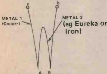
perature difference exists between the junction a and b. This voltage varies almost linearly with temperature for differences up to about 100°C, although this assumption should not be made in calibrating the thermometer for accurate measurement.
