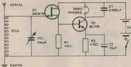
The circuit shown in the figure provides a simple radio receiver which is both sensitive and selective. A low-cost FET is used — the JUGFET 2N3819.
