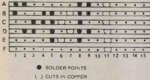
Fig. 2. This shows the places where you have to cut the tracks in the Veroboard. After mounting the components as shown in Fig. 3 the connections are soldered as indicated below.
