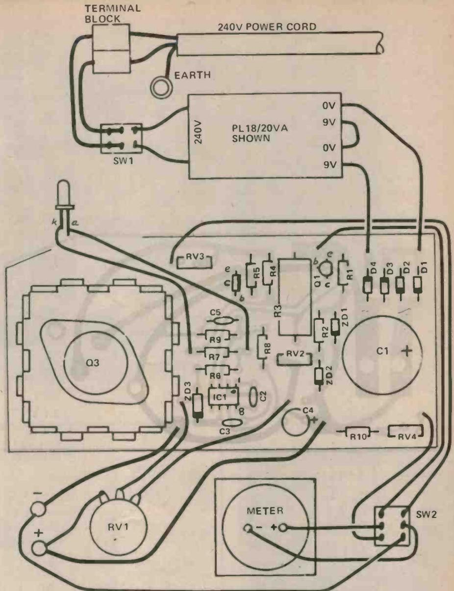
Fig 3. The component overlay and interconnection diagram.
