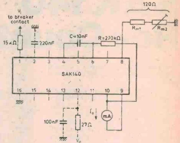
Fig. 2. In this circuit the temperature coefficient of  $I_o$  is 800 ppm/°C, determined by an internal diode between pins 7 and 8. If an external diode is used in the line from  $R_{m1}$  and  $R_{m2}$  it should connect to the IC on pin 7.
