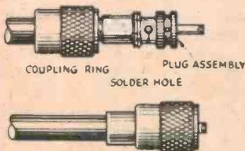
(d) Screw the plug assembly on the cable and adapter. Solder the centre conductor into the centre pin of the plug assembly. Solder the braid to the plug assembly through the solder holes. Use a hot iron with good heat capacity. Finally, screw the coupling ring onto the plug assembly.
