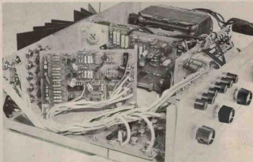
An internal view of the amplifier. Note that the preamp board is pivoted out and not in its final position which is parallel with the rear of the unit.
