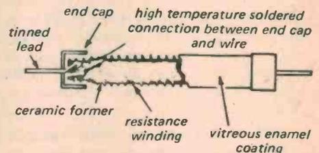
Fig. 4. Typical construction of small, cylindrical style wirewound resistor.
