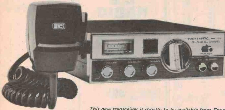
*This new transceiver is shortly to be available from Tandy stores. It gives LED readout of the channel number and features a PLL synthesiser (you don't have to buy extra crystals to get all channels).*
