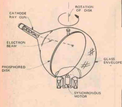
Fig. 4. 3-D display from a special CRT — a 1960's invention helping progress into 3-D television (Courtesy Electronics).
