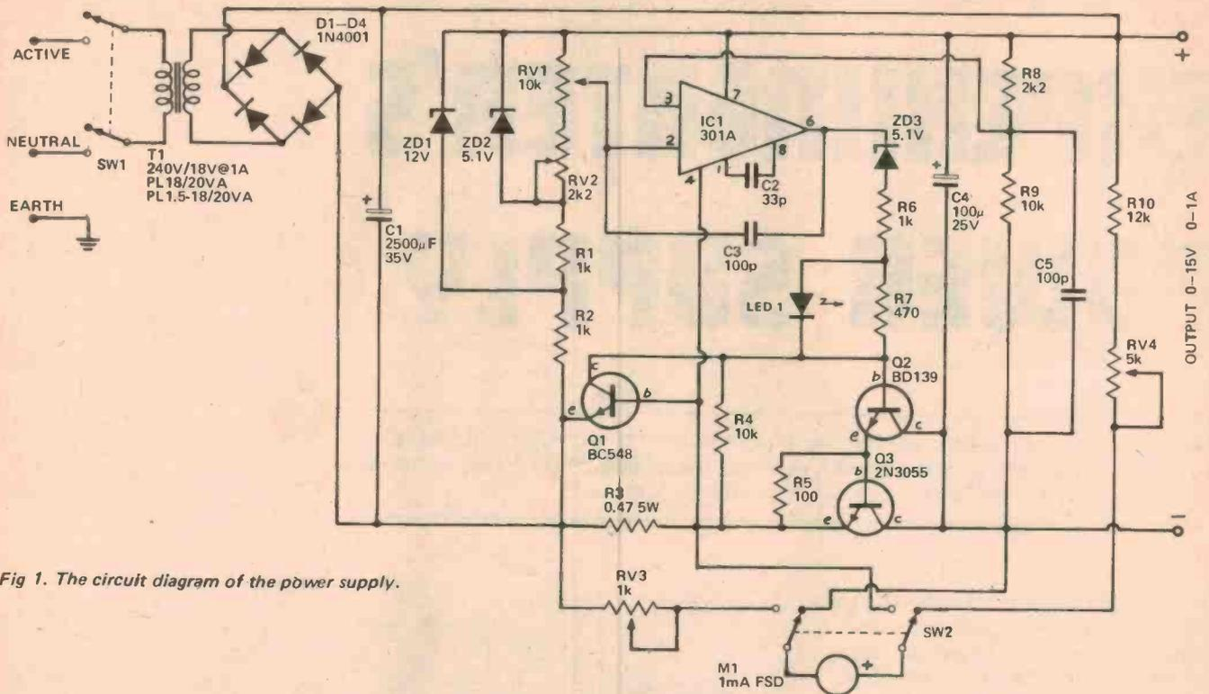
Fig 1. The circuit diagram of the power supply.
