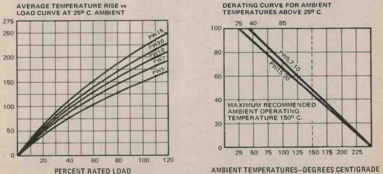
Fig. 7. Temperature rise and power derating curves for encapsulated (ceramic boat) style wirewound resistors.
