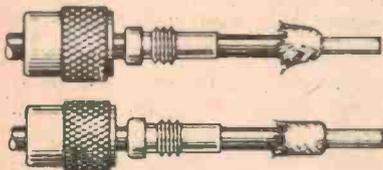
(b) Fan out the braid slightly and fold it back over the cable. Then compress the braid around the cable.
