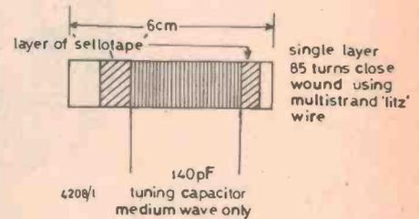
Fig. 2. Coil winding details
