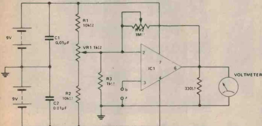
Connections to IC1 are for 8 pin DIL version of '741'
