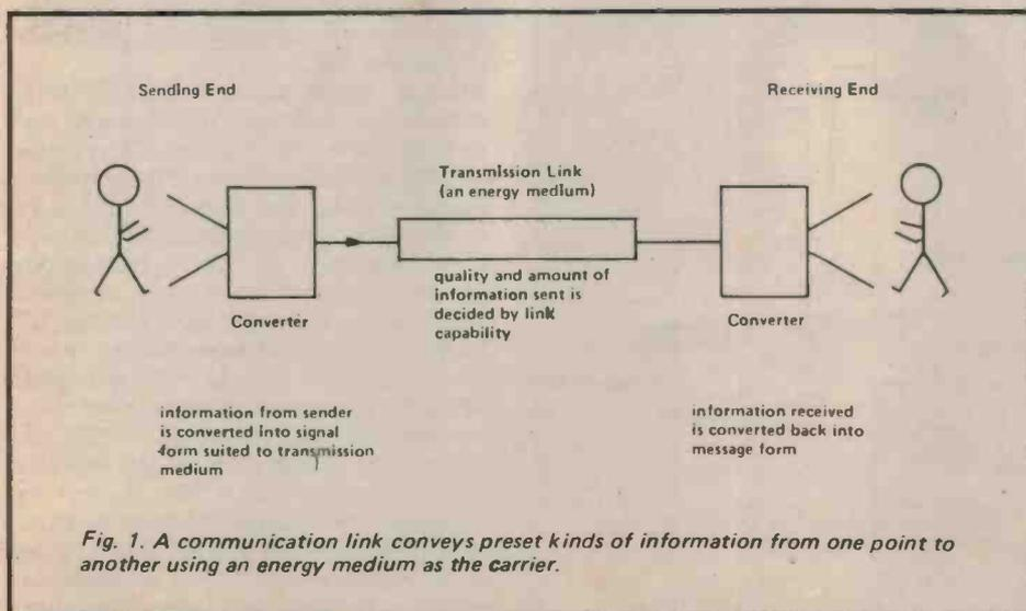
Fig. 1. A communication link conveys preset kinds of information from one point to another using an energy medium as the carrier.
