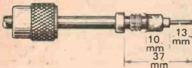
(c) position the adaptor shoulder about 37 mm back from the end of the cable. Press the braid down over the body of the adapter to the dimension shown and trim it. Next, bare the centre conductor at the end by removing 13 mm of the insulation... don't nick the centre conductor. Tin the exposed portion of the centre conductor.
