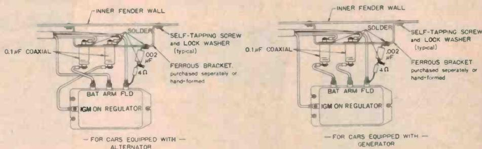
Fig. 5. Suppressing regulator noise - typical methods.
