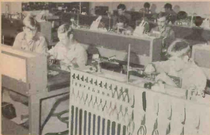
*This classroom is where the trainee learns how to solder. The instructor explains a particular soldering job on the blackboard and straight away the trainee tries it out using his temperature-controlled iron.*
