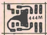
Fig. 3. The printed circuit layout of the small board which allows the LM379S to be used on the original board.
