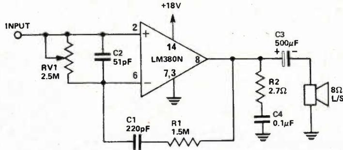
Fig. 9. The RIAA record player characteristic can be obtained with this circuit.
