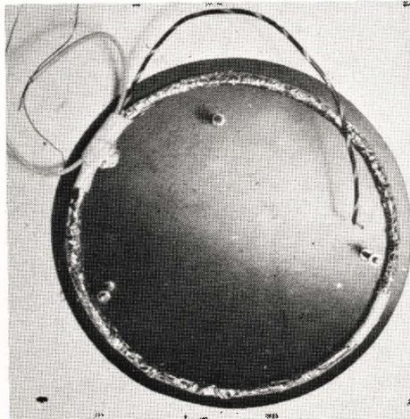
When screened the coil should be glued to the paxolin disc.
