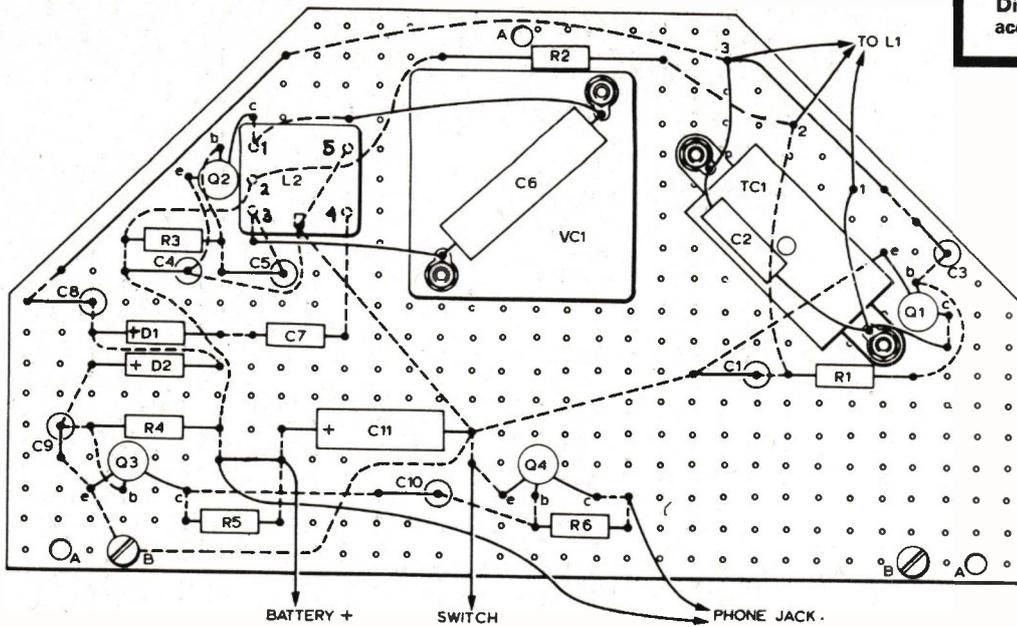
Fig. 3. Component layout — shown here mounted on matrix board (124.5 mm x 71 mm). Dotted lines show wiring on reverse side.
