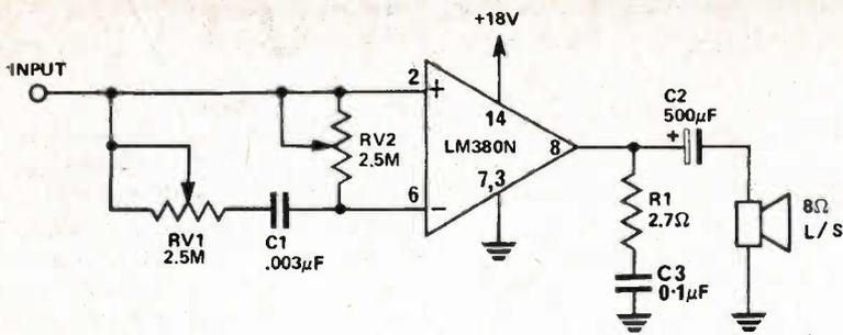
Fig. 7. High input impedance circuit with "common mode" volume and tone control.
