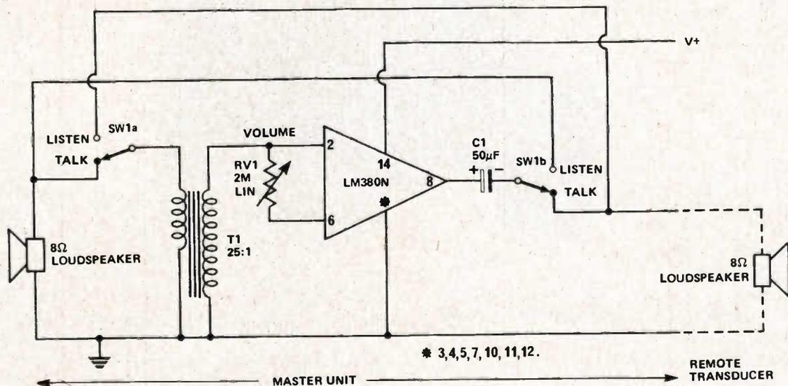
Fig. 14. Simple intercom circuit.
