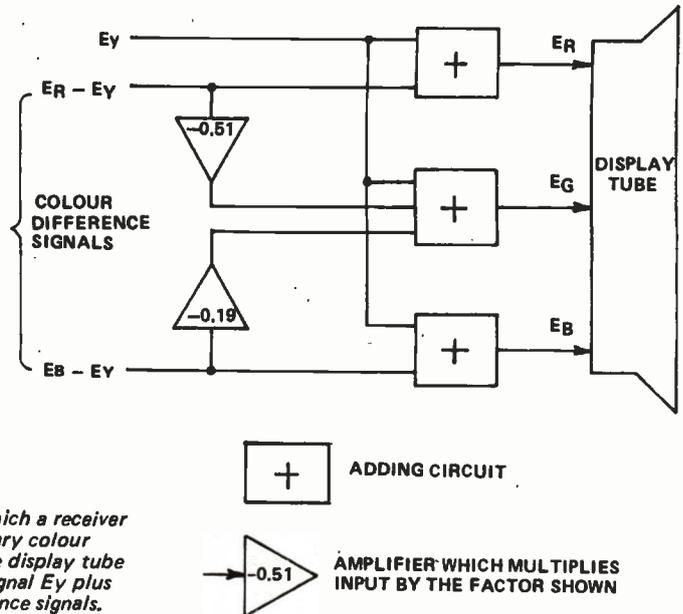
Fig. 10. Process by which a receiver reconstructs the primary colour signals required by the display tube from the luminance signal  $E_Y$  plus the two colour difference signals.
