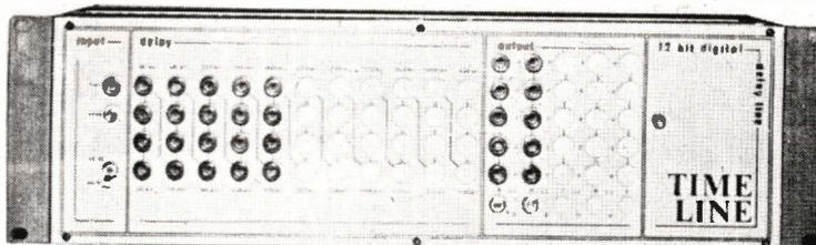
High resolution 12 bit digital encoding produces a full 72 dB dynamic range naturally, making the use of signal altering noise reduction unnecessary. Coupled with less than .1% distortion (measured at full output 400 Hz) the Time Line literally is a black box that generates time delays without any alteration to the signal.
