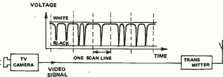
Fig. 11. Principle of tv scanning. The flyback at the end of a scan line to the start of the next is assumed to be instantaneous.
