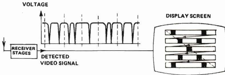
Fig. 12. Television display. The screen is scanned in synchronism with the camera by a spot of brightness controlled by the video signal. If the scan is sufficiently fast, an illusion of the televised scene is created.
