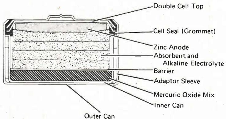
Fig. 4. Cross sections of a typical mercury cell.
