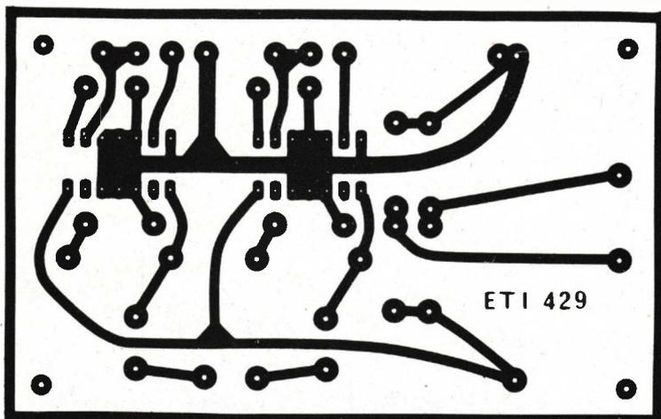
Fig. 5. Printed circuit board. Full size 97 x 61mm.
