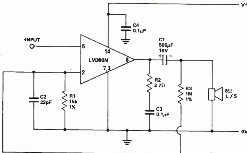
Fig. 5. Increased gain can be obtained by using this circuit.
