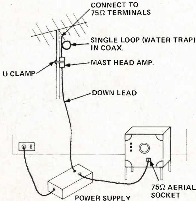
Fig. 4. How the amplifier is fitted to an existing system. Note that where the antenna was previously used with 300 ohm ribbon a balun must be used to match the antenna to the 75 ohm coaxial cable.
