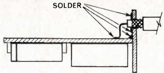
Fig. 3a. Side view of manner in which coax and end plate are fitted to main board. 3b. The completed assembly prior to assembly into the box.
