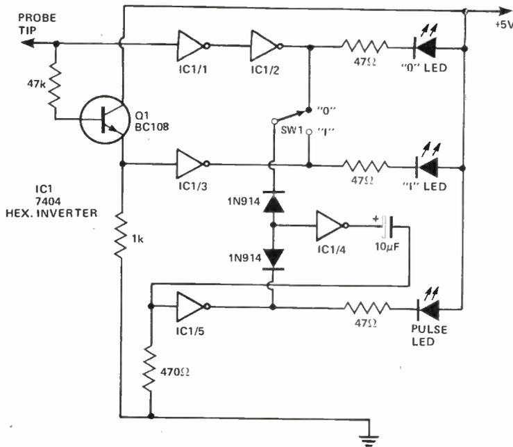
When working on digital equipment it is very often desirable to know the state of various points of the circuit. Usually an oscilloscope is used, however a very short duration pulse is usually hard to see unless the scope is a sophisticated wide-bandwidth type. This logic probe has its own readout which illuminates a LED indicating whether the point tested is a logical "0" or "1". It also indicates the presence of a
