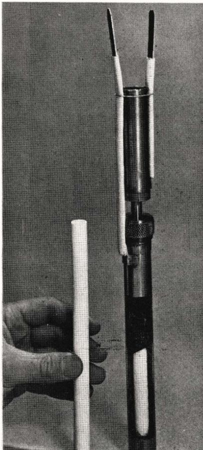
Fig. 12. Actual cell of ECRC Na-S cell showing the Beta-alumina tube used as a solid electrolyte.
