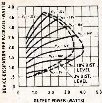
Fig. 12. Output power and dissipation of circuit shown in Fig. 11
