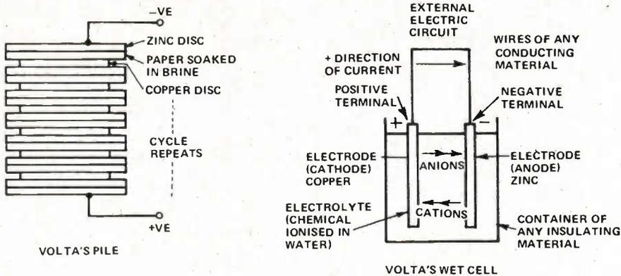
Fig. 2. Cross sectional diagrams of the first electrochemical cells — VOLTA'S pile and wet cell.
