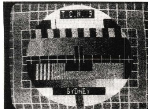
Fig. 5b. The same test pattern on a receiver with 16 dB less signal.
