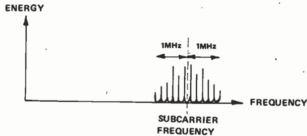
c) Modulating a high frequency (subcarrier) by a colour difference signal produces sidebands to  $\pm 1$  MHz.
