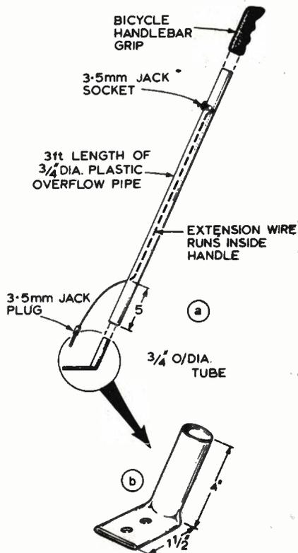
Fig. 2. Details of long handle and bracket
