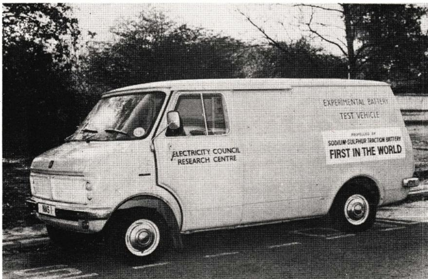
Fig. 10. This modified Bedford van was run around the streets of London to prove the first large battery of Na-S high temperature cells.
