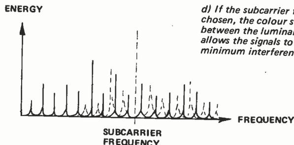
d) If the subcarrier frequency is carefully chosen, the colour signal sidebands lie between the luminance energy peaks. This allows the signals to be added together with minimum interference.
