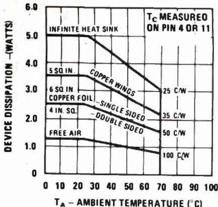
Fig. 4. Maximum device dissipation at various ambient temperatures, with and without heat sinking.
