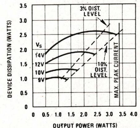
Fig.3. Device dissipation and output power at various supply voltages for (a) 16 ohm, (b) 8 ohm and (c) 4 ohm loads.
