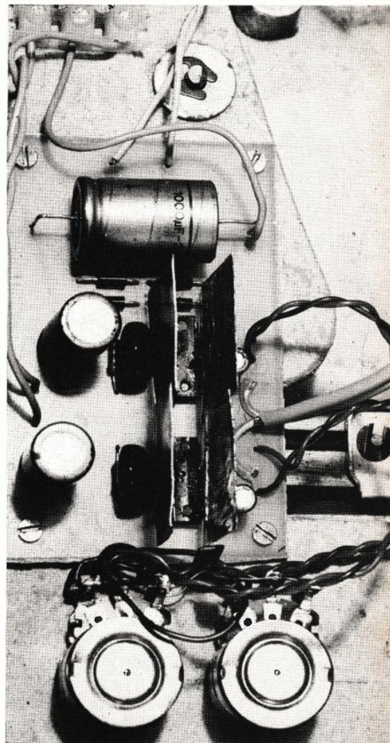
The completed amplifier fitted below a conventional record player. Transformer (not shown) is mounted well clear of signal leads.
