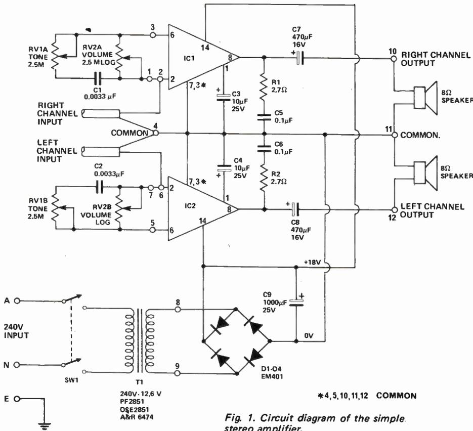
Fig. 1. Circuit diagram of the simple stereo amplifier.
