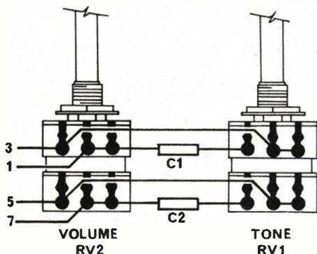
Fig. 4. Wiring to the volume and tone potentiometers.
