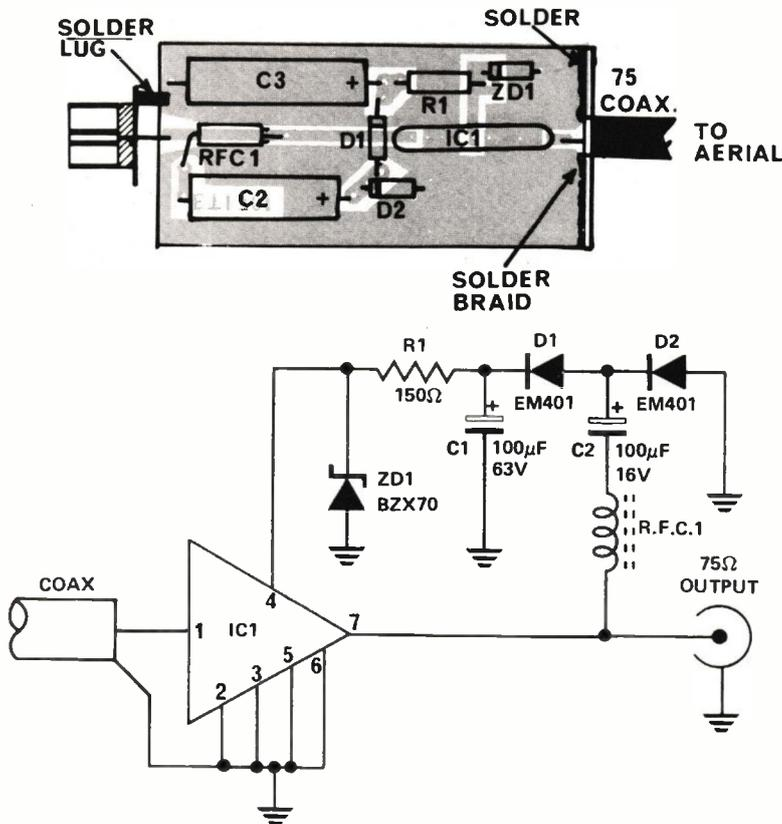
Fig. 1. Circuit diagram of masthead amplifier.
