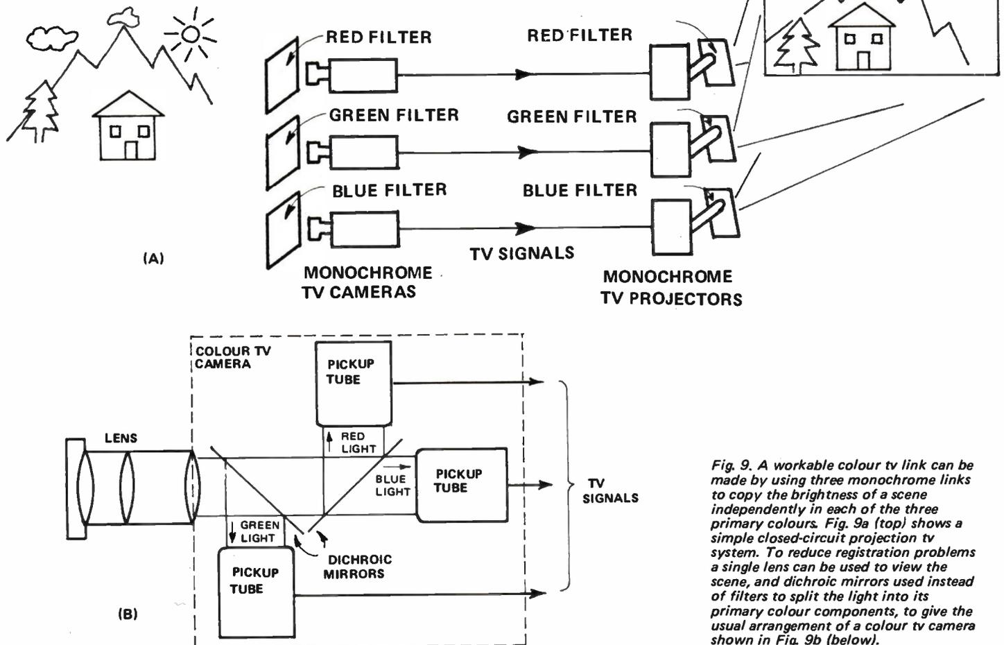
Fig. 9. A workable colour tv link can be made by using three monochrome links to copy the brightness of a scene independently in each of the three primary colours. Fig. 9a (top) shows a simple closed-circuit projection tv system. To reduce registration problems a single lens can be used to view the scene, and dichroic mirrors used instead of filters to split the light into its primary colour components, to give the usual arrangement of a colour tv camera shown in Fig. 9b (below).
