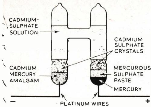
Fig. 5. The Weston standard cell delivers 1.0186 volts provided the load is minimal. It has found extensive use as a standard of the voltage unit.
