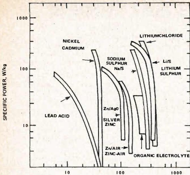
Fig. 5. Comparative chart of the main forms of high-temperature battery designs.
