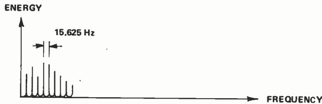
b) Energy in the colour difference signals tends to be concentrated at harmonics of line frequency.
