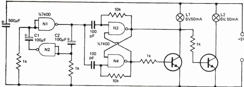
In this circuit a TTL quadruple NAND gate is wired as a multivibrator to actuate two lamp drivers.
