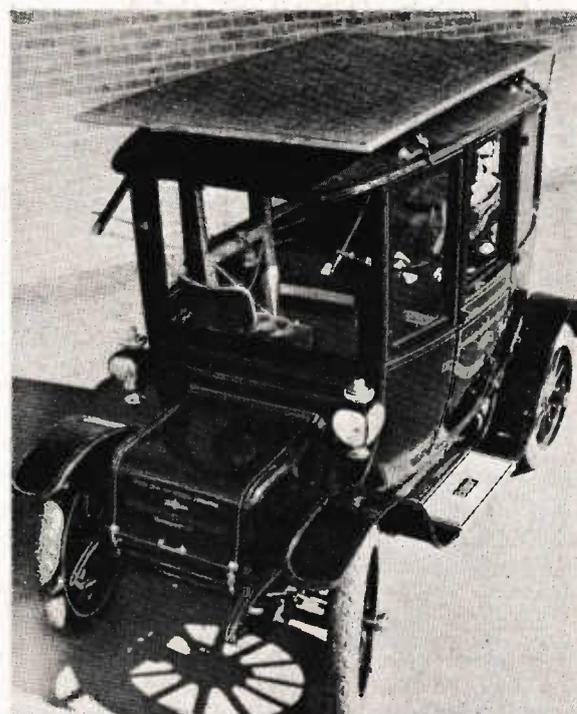
*This 1912 Baker Electric is now driven by solar energy! An array of 10 640 silicon solar cells mounted on the vehicle's roof charge intermediate storage batteries. Final drive is via the Baker's original dc electric motor*
