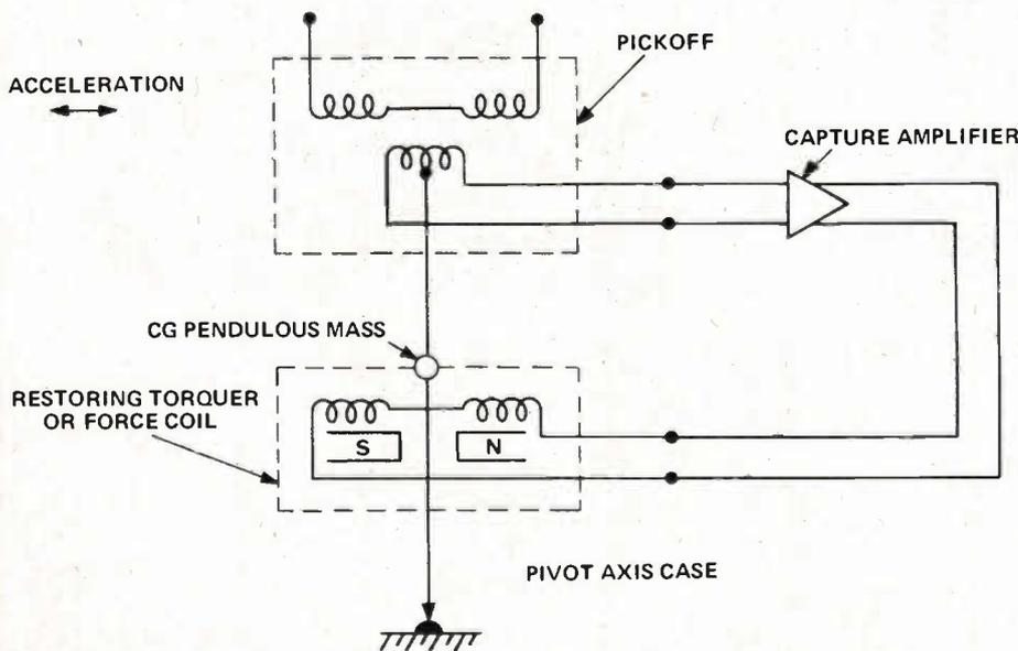
Fig. 4. This typical force balance pendulous accelerometer utilizes a differential transformer type pick-off, a high gain capture amplifier, and a dc permanent magnet force coil. These features typify many of the high precision force-balance accelerometers currently manufactured.
