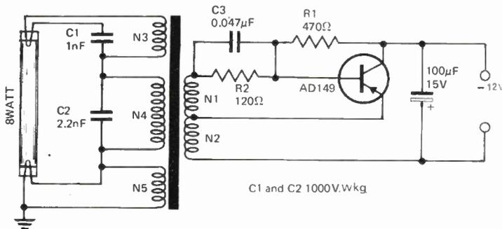
This inverter enables an 8 watt fluorescent tube to operate from a 12 V DC supply. Light output is equivalent to a 25 watt globe.
