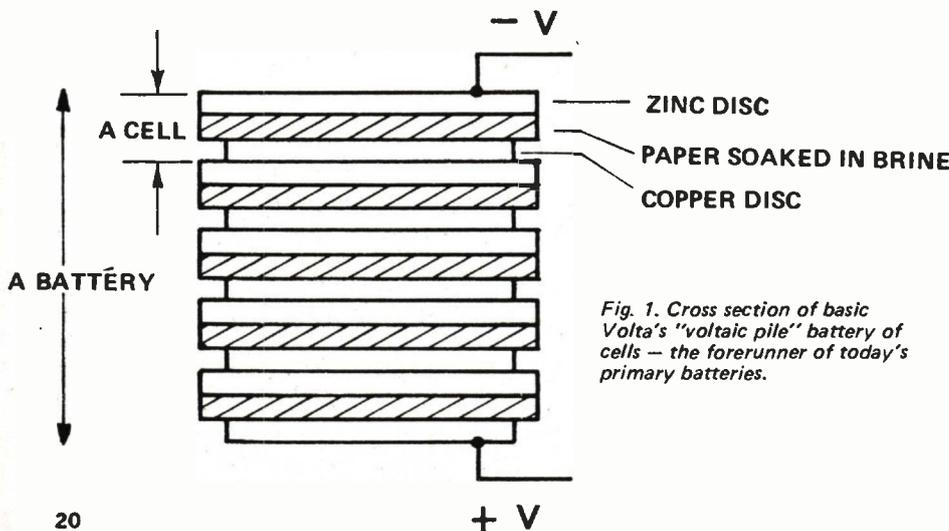
Fig. 1. Cross section of basic Volta's "voltaic pile" battery of cells — the forerunner of today's primary batteries.
