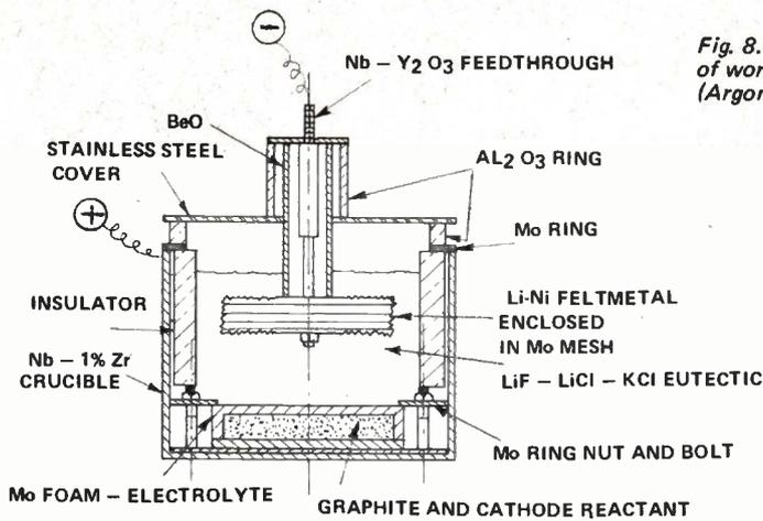
Fig. 8. An advanced form of workable Li-S cell (Argonne Laboratory).
