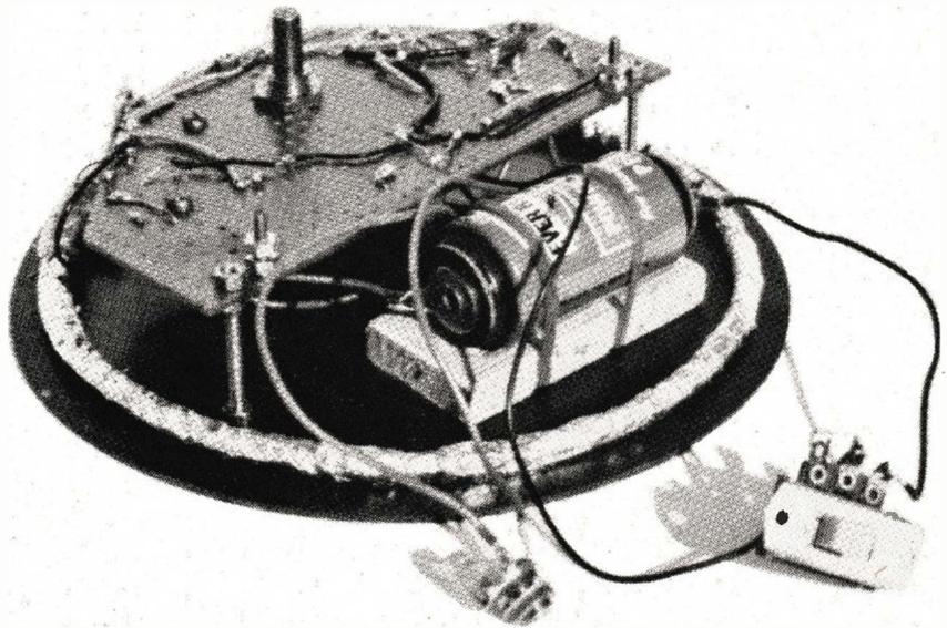
The main assembly without the case. The wires to the switch and earphone socket should be left reasonably long.
