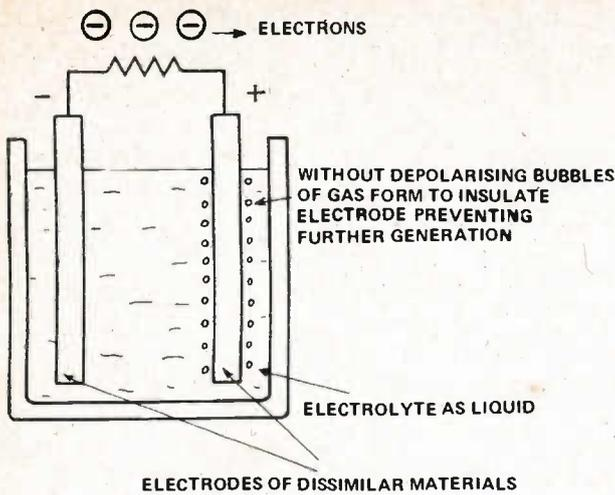
Fig. 2. Electrical cells can also be made with liquid electrolyte but means are needed to depolarise the electrode if it is to work for long.
