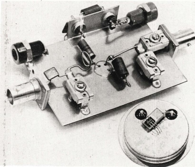
A unique beryllia-insulated die mounting technique is used to significantly improve the power dissipation and gain capabilities of a TO-39 style package. These improvements enable a designer to replace expensive stud mounted, medium-power
