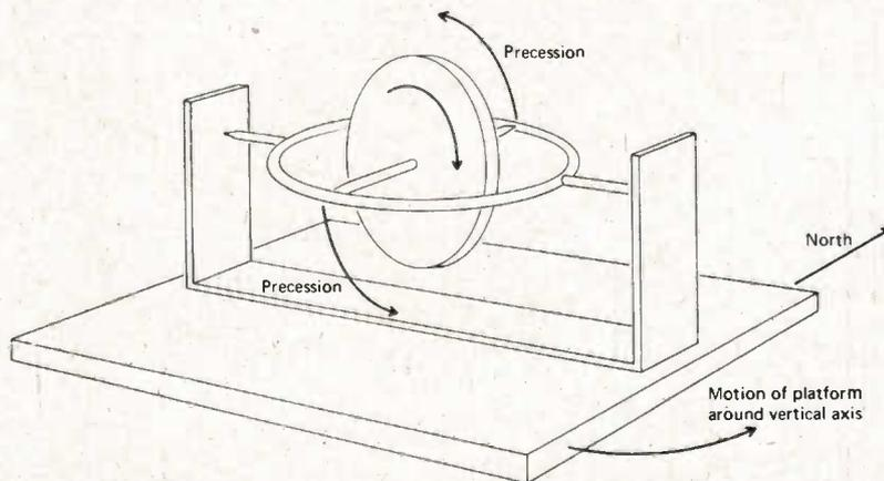
Fig. 2. How a gyrocompass works. If the assembly is caused to change direction in the horizontal plane, the rotating assembly 'precesses'. This so-called 'precession' is measured, thus providing data about the amount of directional change.
