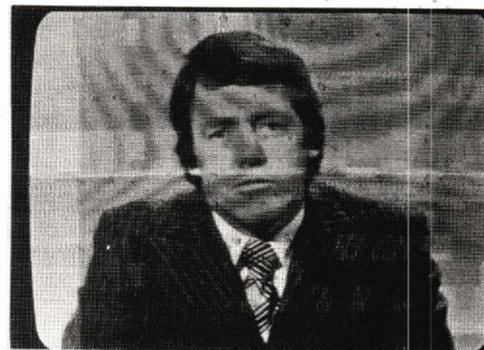
Fig. 5d. When using a wide band amplifier, too much signal on one channel may well interfere with other weaker ones. Here channel ABN2 is interfering with channel Ten. A simple attenuator ahead of the amplifier may be adequate. (If other channels are not too weak) alternately use a trap on the strong channel to selectively reduce its level.
