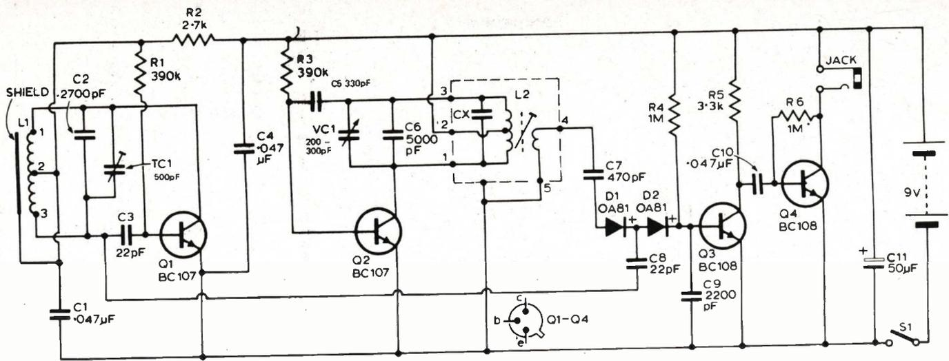
Fig. 1 The complete circuit of the ET1 Coin Collector. L1 is the screened search coil and L2 the modified i.f. transformer acting as the reference oscillator.
