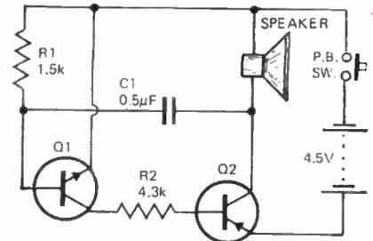
This circuit consists of an asymmetric multivibrator activated by a pushbutton. The loudspeaker is a transistor radio type with a voice coil impedance of about 25 to 40 ohms. Earpieces up to 500 ohms can be used for lower power output. R1 varies frequency over the audio range.
