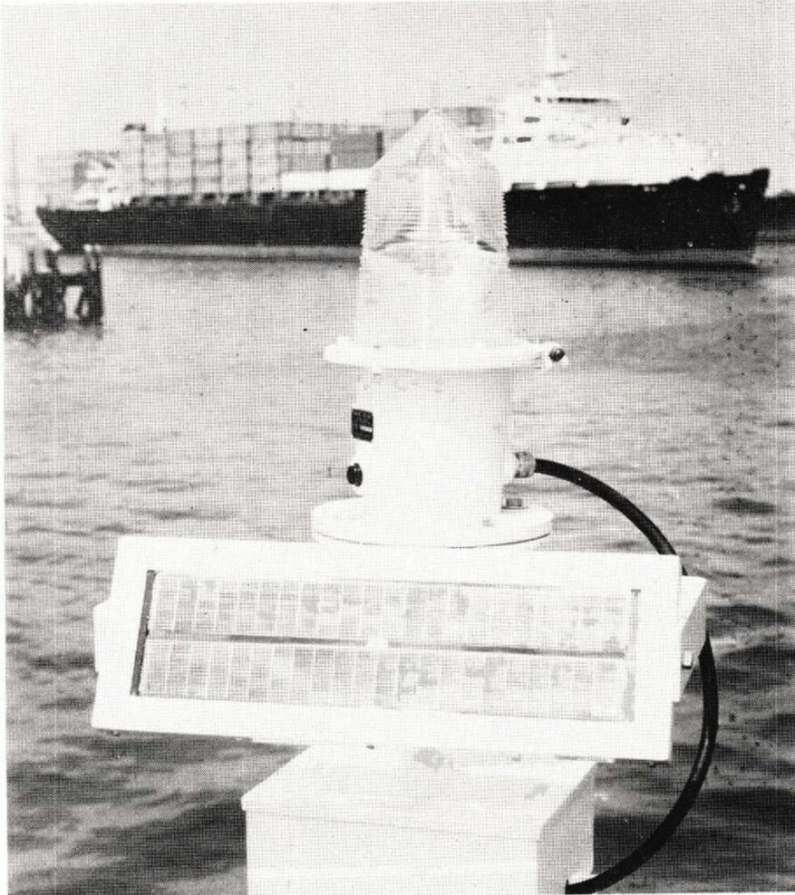
*Solar-cell powered buoy.*
