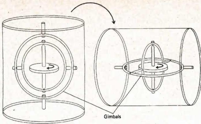
Fig. 1. This gyroscope is mounted in gimbals so that the rotating mass always points in the same direction — regardless of 'container' attitude.
