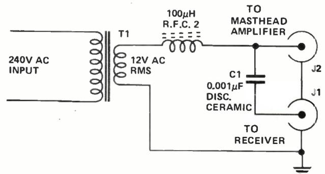
Fig. 1b. The power supply box circuit diagram. Note that outputs are taken to co-ax sockets on power supply box. Power is fed to mast-head amplifier via the signal co-ax.
