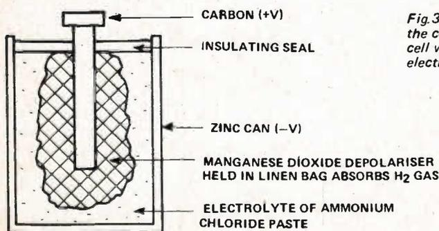
Fig. 3. Cross section of the common tubular dry-cell which uses a paste electrolyte.
