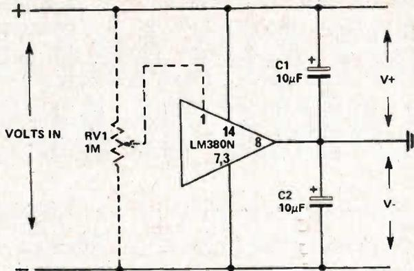
Fig. 13. Balanced output power supply
