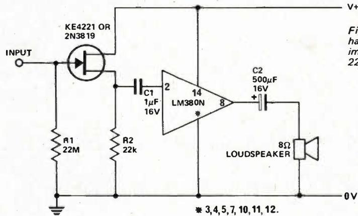
Fig. 10. This circuit has an input impedance of about 22 MΩ
