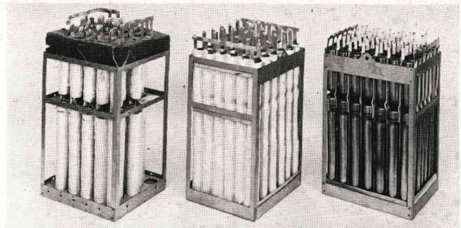
Fig. 13. Three stages of development increased packing density of the ECRC cells into the battery module. They must be electrically insulated from each other at an operating temperature of around 350°C.
