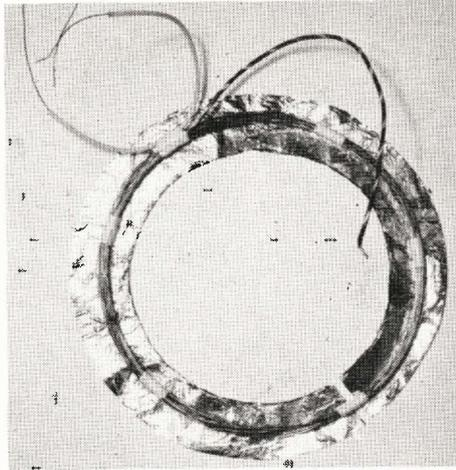
The coil should be laid on the aluminium foil as shown. Note the gap opposite the wire ends.
