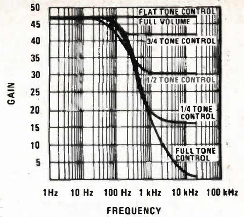
Fig. 8. The effect of the tone control circuit shown in Fig. 7.
