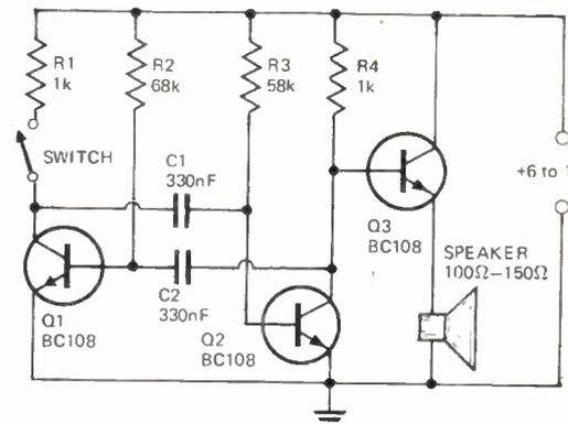
This circuit will give a sound like a ship's siren. It can be used with the low power output source for model ships if fed into a more powerful amplifier/speaker, as an alarm tone.
