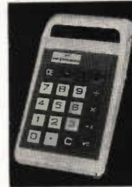
9 digit calculator with floating decimal point, Texas Instruments J.C.'s, 10 second fade on, .3" LED readout with instant recall, rechargeable nickel cadmium batteries
