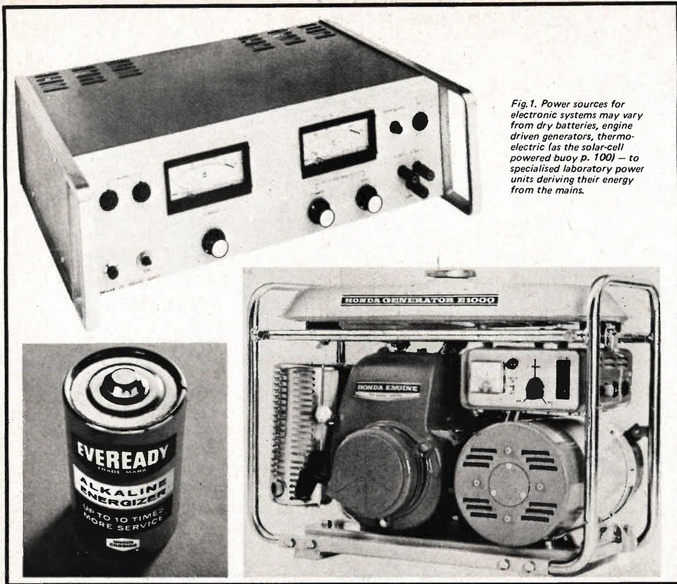
*Fig.1. Power sources for electronic systems may vary from dry batteries, engine driven generators, thermo-electric (as the solar-cell powered buoy p. 100) – to specialised laboratory power units deriving their energy from the mains.*
