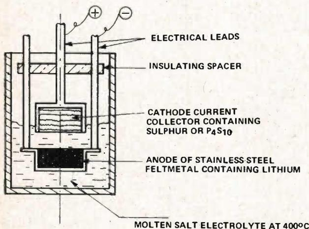
Fig. 6. Rudimentary lithium-sulphur cell design for use in laboratory test chambers — it is unsealed and lithium reacts with moisture explosively. (Argonne Lab.).
