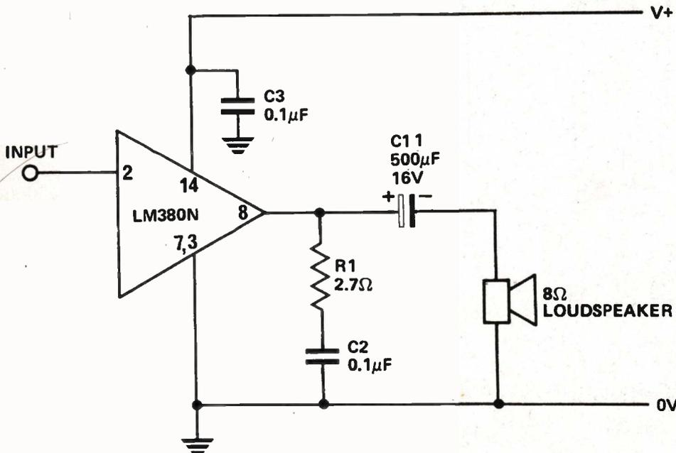
Fig.2. LM380N basic amplifier circuit.
