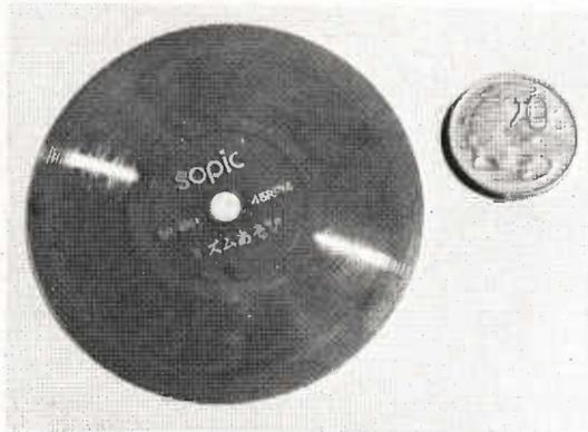
*The Sopic record is flexible transparent and may be pasted to the pages of lesson material as it does not have to rotate.*
