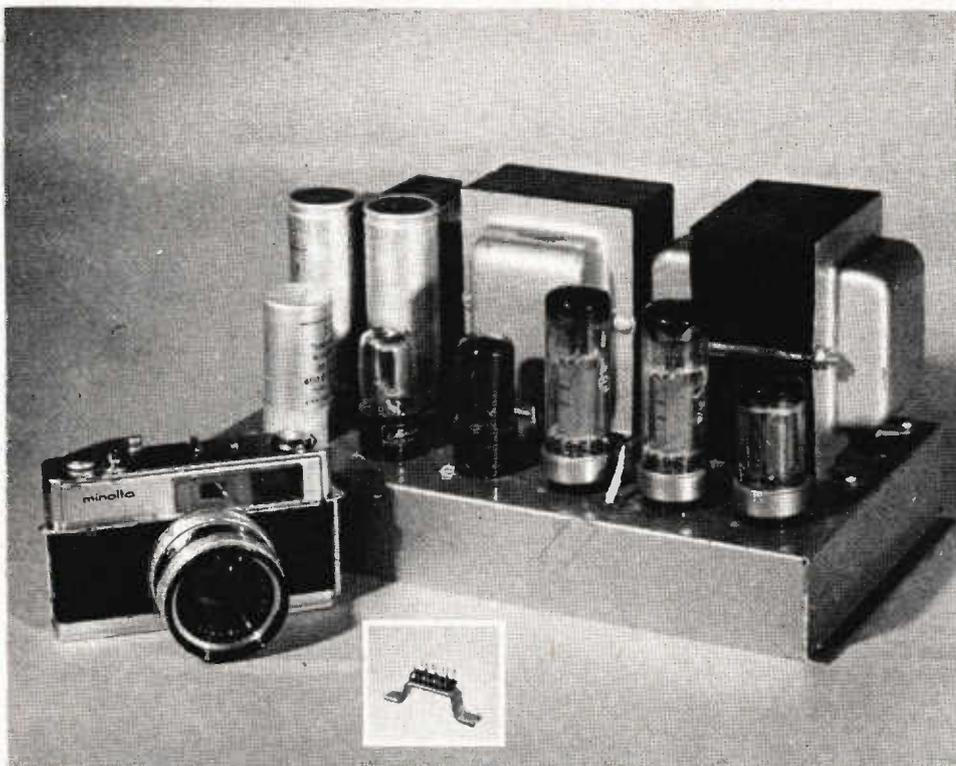
*Fig. 5. Dramatically illustrating the rapidly changing nature of electronic techniques, the tiny module (below) has virtually identical performance as the massive unit shown above it. Both are high power audio amplifiers.*
