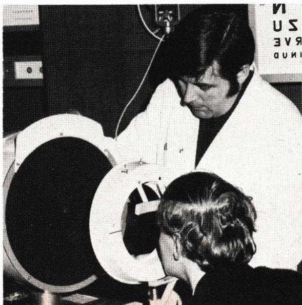
◀ Fig. 12. Friedman-Bedwell Visual Field Screener in use. Patient fixates central target through circular fluorescent tube which keeps lighting conditions consistent. Patterns, selected by a lever behind the white fascia, are flashed onto the black screen (in fact they are apertures illuminated by a xenon flash-tube).
