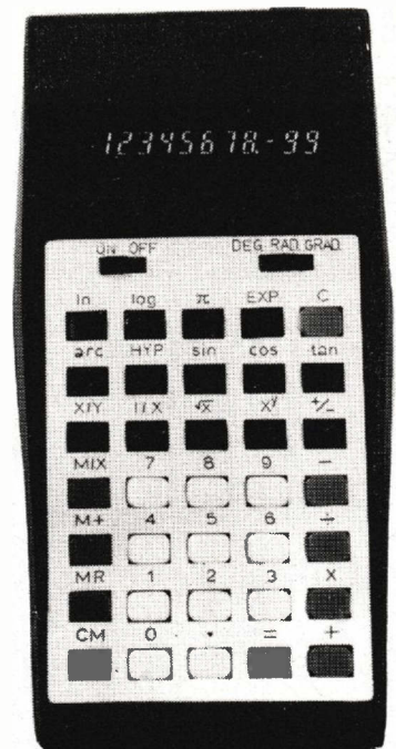
The Qualitron 1419 is unusual in incorporating hyperbolic functions.
