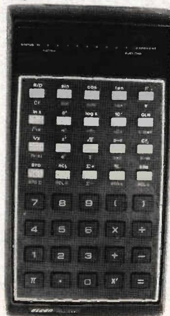
The SC60 from Elcon incorporates a selection of statistical functions and has the ability to overflow the normal 10-99 to 10+99 range by a further 100 decades at each end.
