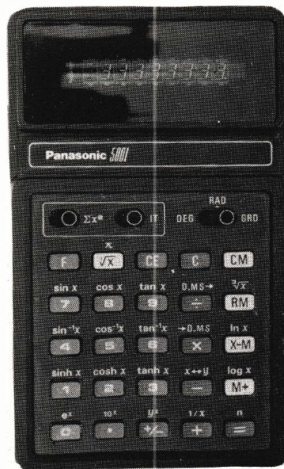
The Panasonic 5001 from National incorporates angular measure in grads, \sqrt[3]{X} and sum of the squares.
