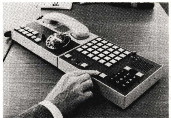
Thirty telephone numbers – of up to 20 digits each – can be dialled automatically by this new unit from Siemens. A dynamic read/write memory (RAM) stores the call numbers. Provision is made to store the numbers for at least two days in the event of a power outage.
