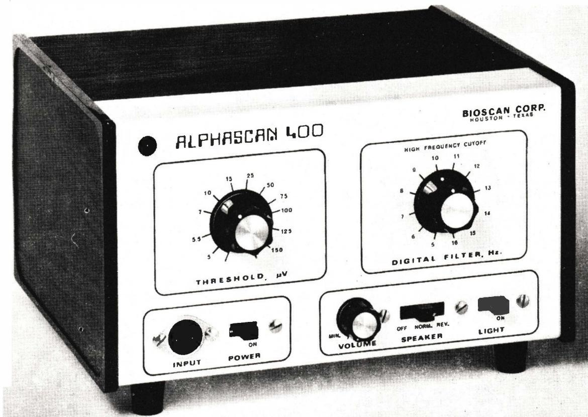
*Advanced alpha/theta instrument from Bioscan uses digital filtering and threshold adjustment to eliminate interference from spurious phenomena.*
