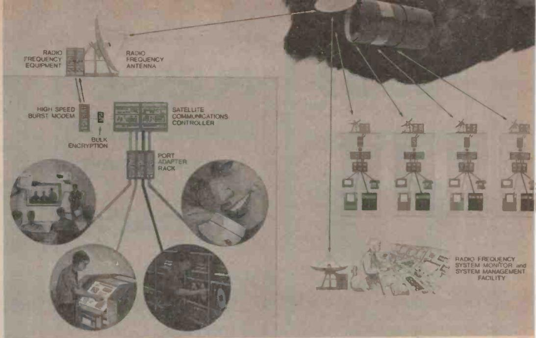
able to carry information equivalent to about 12,000 simultaneous telephone conversations. In addition, it is very easy to interconnect any number of points using a satellite, whilst the direct interconnection of only 12 cities in a terrestrial network can require 66 separate land-based links.
