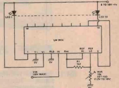
Figure 4. An alternative 1.2V to 10V fsd dot mode voltmeter.
