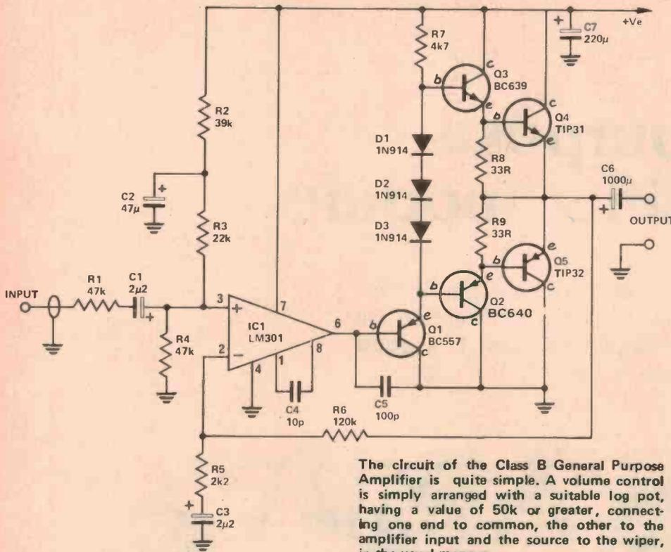
The circuit of the Class B General Purpose Amplifier is quite simple. A volume control is simply arranged with a suitable log pot, having a value of 50k or greater, connecting one end to common, the other to the amplifier input and the source to the wiper, in the usual manner.
