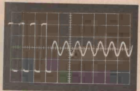
Performance of the Accuphase E203 on transient overload recovery test.
