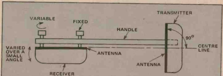
The pipe and cable locator employs an induction balance technique. The plane of the receiver antenna is set along the centre line of the transmitter antenna and at a right angle to it. To permit good 'nulling' of the received signal, the plane of the receiver antenna can be varied over a small angle by means of the spring-loaded adjustment bolt in the handle at the head of the receiver.
