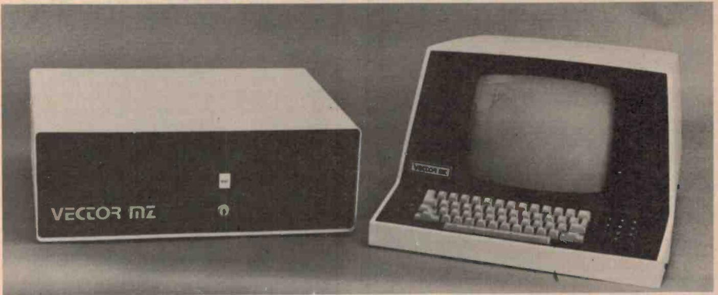
The basic Vector MZ System B consists of the computer (based on the S-100 bus) with twin minifloppies — at left — plus the MT 'mind-
