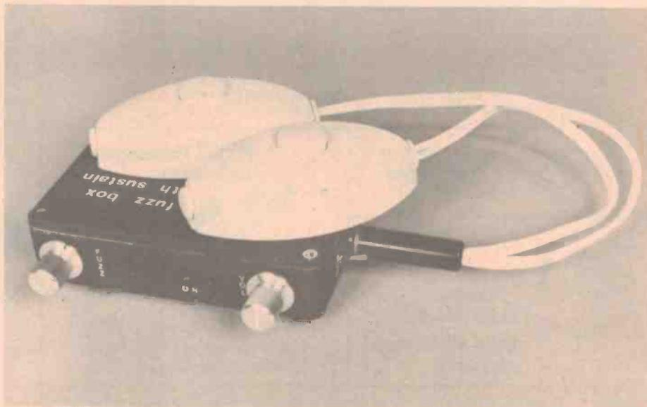
with a fixed compression ratio of 2:1. This compression effectively halves the dynamic range of the incoming signal by attenuating high level signals and
