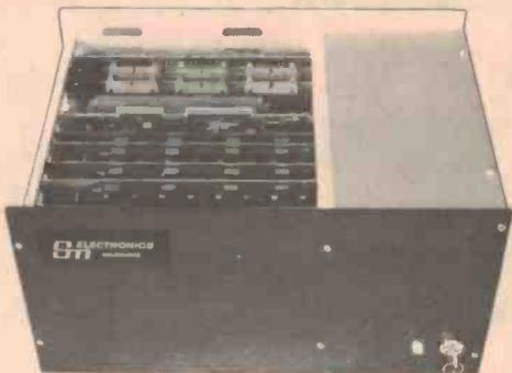
11 slot backplane, fully card guided. 15 amp power supply, fan, key switch, bench mount, rack mount, anodised aluminium. 5 edge connectors standard. S-100 Bench Kit \$345. S-100 Rack Kit \$306. 6800 Bench Kit \$370. 6800 Rack Kit \$330. Assembled prices add \$100.
