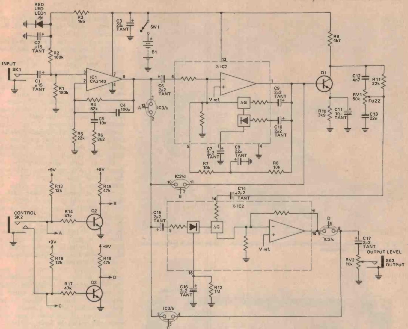
the op-amp input. If the input rises 6dB, the output can rise only 3dB.
