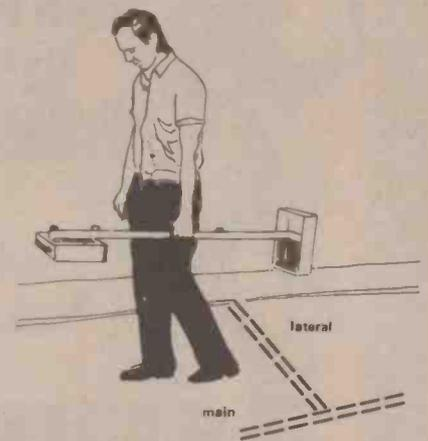
General use of the instrument. With the receiver correctly adjusted for a null, proceed along a line, or parallel lines, until an indication is received. For accurate location, cross the indication point from each side and mark with your heel where the indication is strongest. The location of the buried object is between the two marks.
