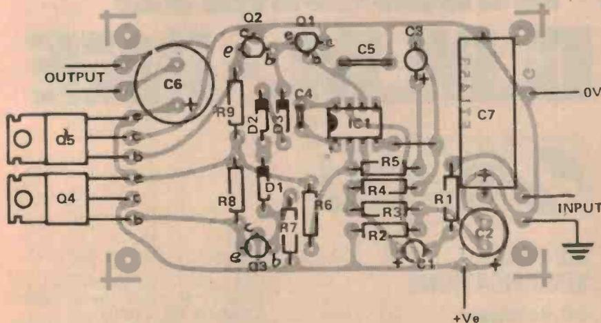
Overlay showing placement of components.
