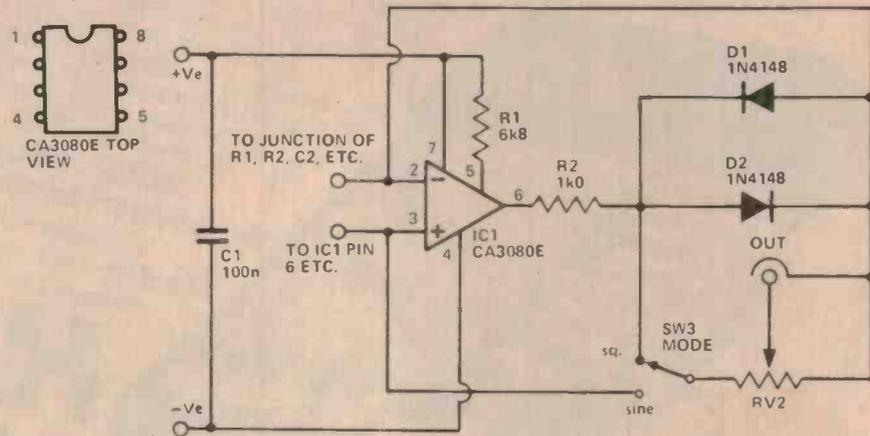
0.6 volts across D2. When the circuit is fed with negative going half cycles the non-inverting input is taken to a lower potential than the inverting one, causing a forward bias to be applied to D1, and producing a negative output potential of about 0.6 volts.
