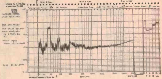
quartz lock function has inadequate signal sensitivity to allow it to operate. The background noise on FM is extremely low and the background noise on both FM, AM and on record play and tape recorder is almost as good as any amplifier we have tested. Where other manufacturers may have been prepared to sacrifice performance in order to provide the gargantuan power of 300 W per channel, Marantz appears to have sacrificed nothing by way of quality on this unit. Although we are
