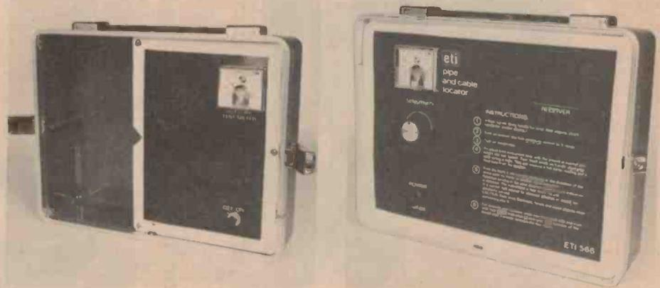
Overall views of the completed receiver and transmitter. The antenna loops are made to fit together so that the instrument may be made into a single case for transporting. The clips and carrying straps are 'dress up' options. The V-groove visible in the transmitter panel is where the handle sits.
