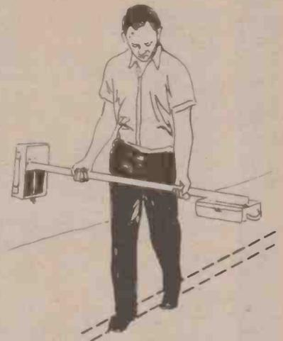
Locating the end of a pipe. Having determined the position of the pipe, hold the instrument as shown — the received signal will be quite strong until you pass the end of the pipe. The received signal will die away a metre or two from the end of the pipe, so any excavation should be back a little from this point.
