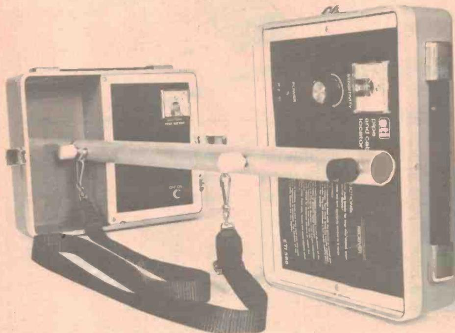
The completed instrument. The handle is secured by bolts, to which the knobs are attached, which pass through the handle into threaded receptacles in the case panels. The handle for general use is 1120 mm long overall. We also tried a shortened handle, 610 mm long, which improves sensitivity to small objects, but decreases ground penetration. The webbing strap is an optional refinement, used to lower the unit towards the ground to improve penetration.
