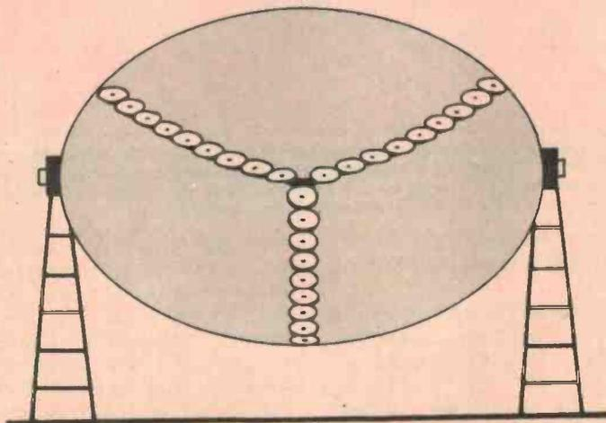
Many small antennas arranged in a 'Y' configuration can simulate the large, single dish telescope (as illustrated diagrammatically above) by utilizing the Earth's rotation. When the 'Y' system is rotated relative to the object being observed, in 8-12 hours "exposure time" the large telescope array will generate a high resolution 'picture' of the radio source it is set to track.
