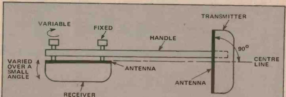
The pipe and cable locator employs an induction balance technique. The plane of the receiver antenna is set along the centre line of the transmitter antenna and at a right angle to it. To permit good 'nulling' of the received signal, the plane of the receiver antenna can be varied over a small angle by means of the spring-loaded adjustment bolt in the handle at the head of the receiver.
