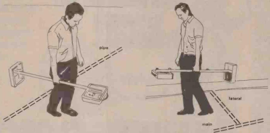
General use of the instrument. With the receiver correctly adjusted for a null, proceed along a line, or parallel lines, until an indication is received. For accurate location, cross the indication point from each side and mark with your heel where the indication is strongest. The location of the buried object is between the two marks.
