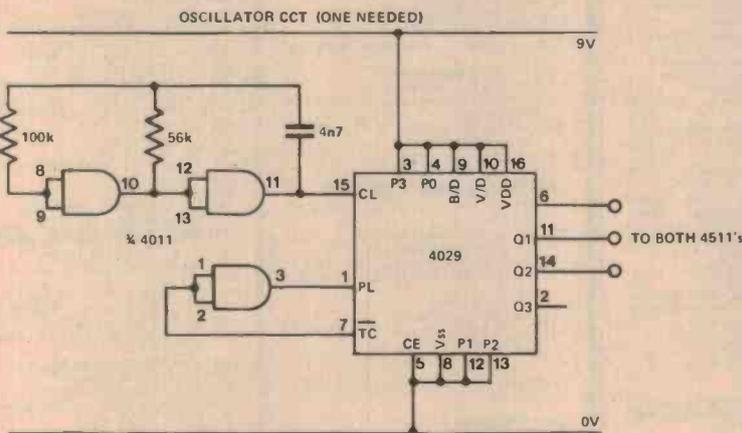
The high clock frequency ensures that the dice has a random result. Even if you attempt to touch both pads simultaneously, each die shows a different throw.
