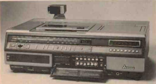
Facilities available on the HS 300 include fast picture search at seven times normal speed, slow motion search at half speed, freeze-frame, single frame advance and automatic rewind. In the freeze-frame and single frame advance modes the machine automatically searches for the most stable adjacent frame so as to avoid the picture deterioration often found in other VCRs operating in these modes.
