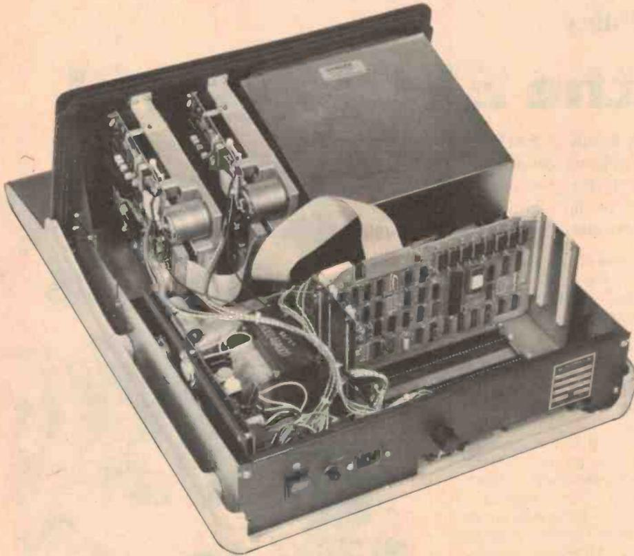
Inside the EXORset 30. Note the expansion card cage behind the enclosed VDU. Interface buss at lower right.
