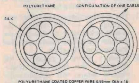
Figure 6. The Trio-Kenwood low capacitance tone arm wire.
