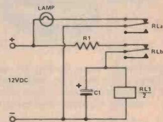
When the power is first applied, the capacitor charges through R1. When the voltage across the capacitor has risen sufficiently, the relay operates. Power is then disconnected from the relay coil, and C1, by the relay contacts in series with the supply and the capacitor starts to discharge through the relay coil. When the voltage across the coil falls below the 'hold in' voltage, the relay drops out. This is one flash cycle.
