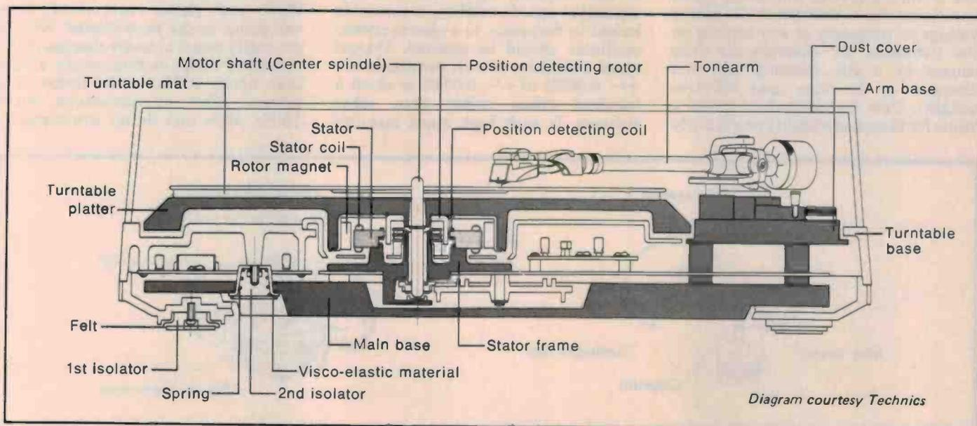
**THE BASIC REQUIREMENT** of any record player assembly is that the turntable shall rotate noiselessly, at the required speed without any short-term or long-term variations in this speed. This sounds a simple enough requirement, yet sophisticated, modern players contain quite complex circuitry with large numbers of integrated circuits and discrete components; indeed, the circuitry is too complex for us to reproduce in full for any of the latest players mentioned in this article!
