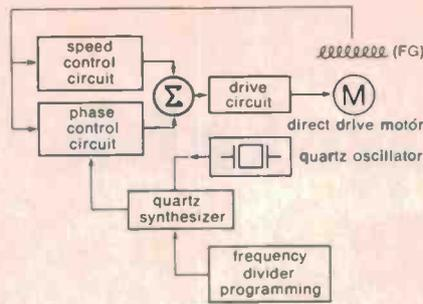
Block diagram of a quartz stabilised turntable drive circuit, as devised by Technics.
