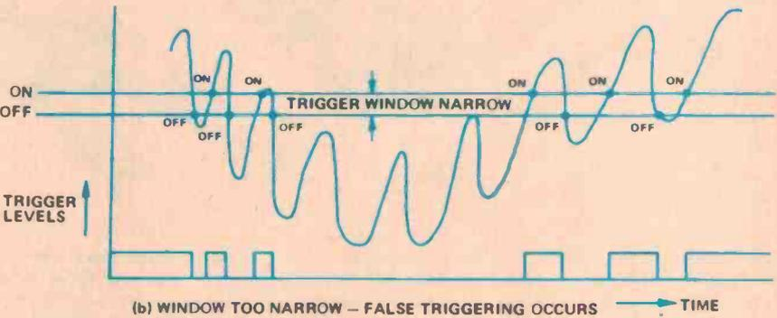
ABOVE: Trigger Window Diagram. The width of the trigger window will greatly affect the accuracy of measurement when attempting to take a reading on a signal having a high frequency component. Set the trigger window wide for best results.
