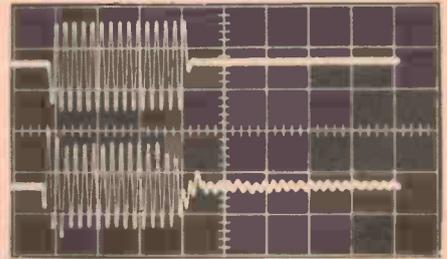
Tone burst response oscillographs of the Model A-2375 loudspeakers, measured with respect to 90 db steady-state spl at 2m on axis, LEFT: at 100 Hz, (20 ms/div, 80 dB spl). CENTRE: at 1 kHz (2 ms/div) and RIGHT: at 6.3 kHz (0.7 ms/div).
