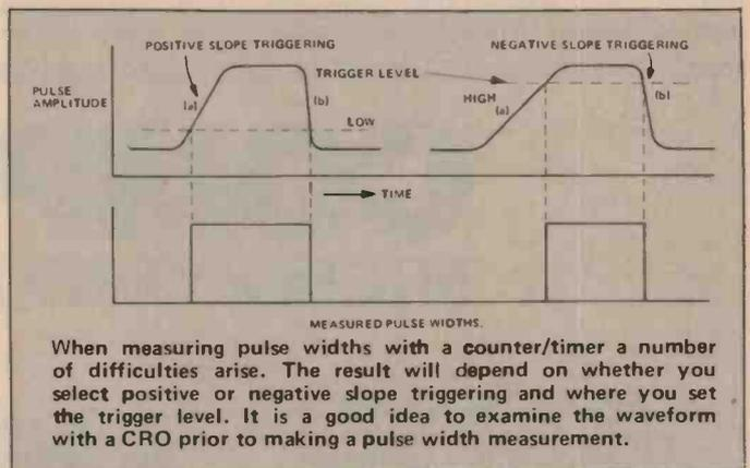
usually provided with a 'slope selection' control which determines whether the trigger operates on the positive or negative slope — (a), or (b) respectively in the diagram.
