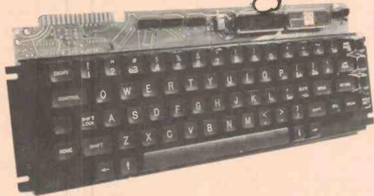
General Instrument's Keyboard Division has combined state-of-the-art microprocessor technology with the reliability and simplicity of capacitive keys to create a highly flexible, low cost keyboard for OEM's and hobby projects.
