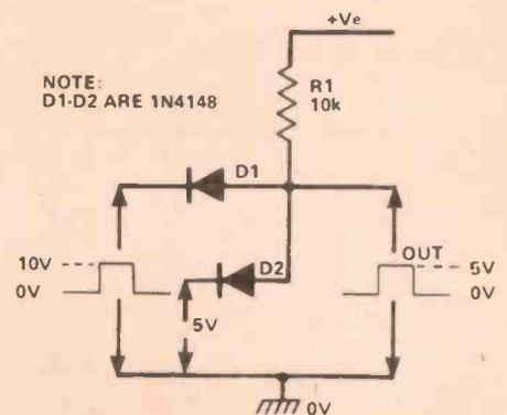
Figure 8. The effect of feeding a pulse to one input and a dc voltage to the other input of a two-input diode AND gate.
