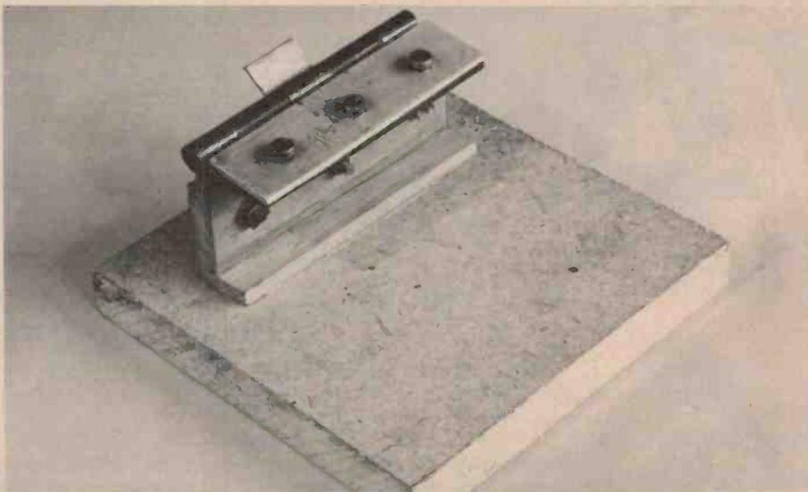
attached to the moving wing of the hinge by three clamping screws tapped into the wing.
