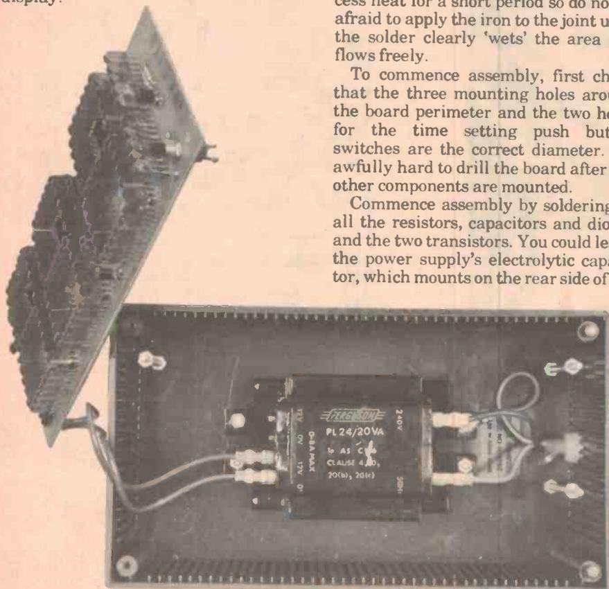
Inside the clock, showing how we mounted the transformer. Take care with the mains wiring.
