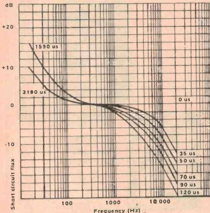
Figure 12. Recording characteristics to BS 1568: 1970.
