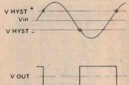
Figure 7. How the Schmitt trigger of Figure 6 works.
