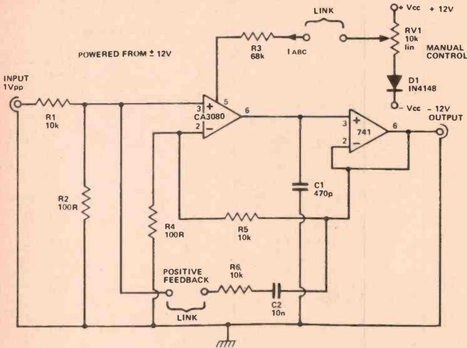
When this resistor is varied, the break frequency of the filter also varies.
