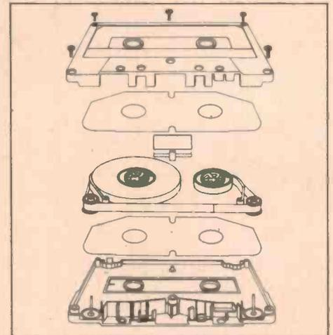
The patented BASF Security Mechanism (SM) prevents scrambling of tape and guides the tape smoothly within the cassette. A large strong window gives clear visibility to the best BASF ferro super I tape yet.
