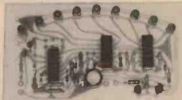
The 3002P.M. can be used to indicate power output of any amplifier from 5 watts to 300 watts. Several component changes converts the module from a power meter to a VU meter.
