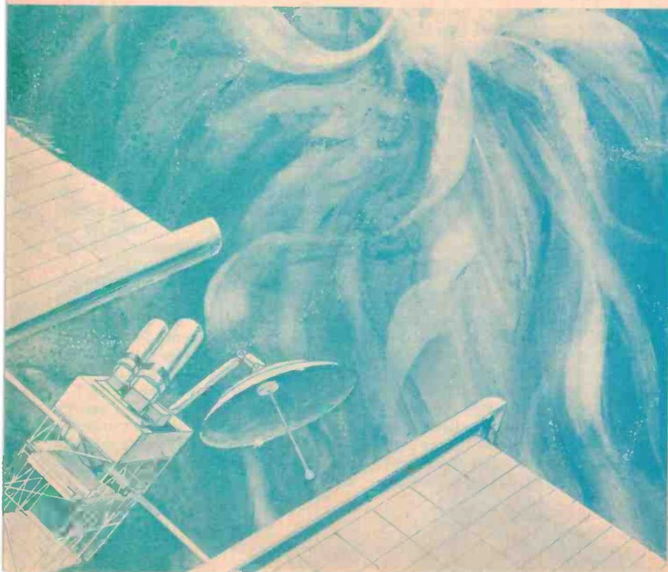
An artist's conception of an astronaut making a final check on an ion-driven spacecraft before separation from the Shuttle. The solar panels are retracting to the stowed position before the chemical rocket is fired to lift the vehicle above the Van Allen belts. The craft carries three communications satellites.
