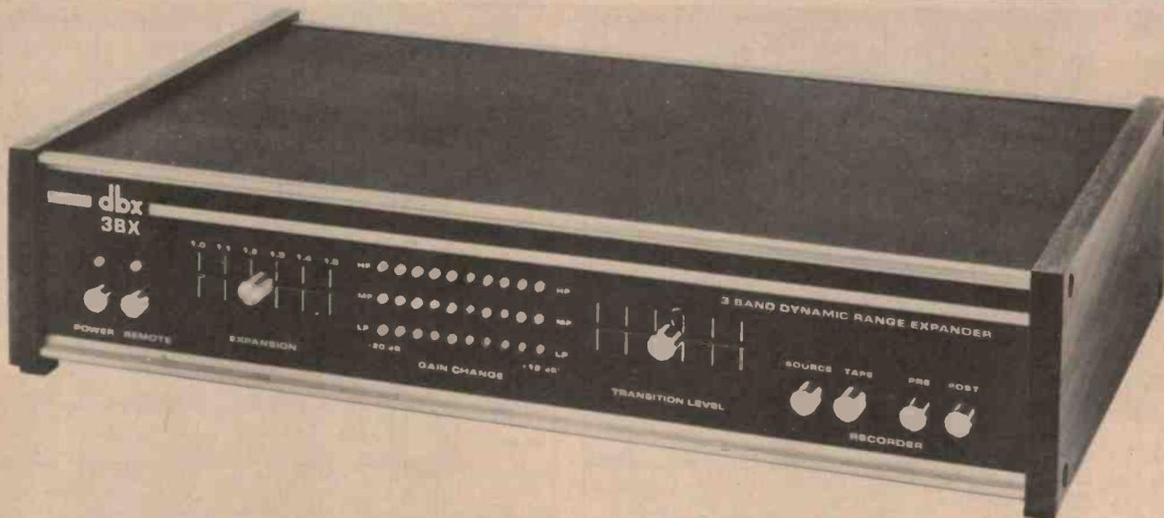
level changes back to normal there is a delay before the expander changes its output — this delay is known as the *release time*. In general, attack and release times are independent of each
