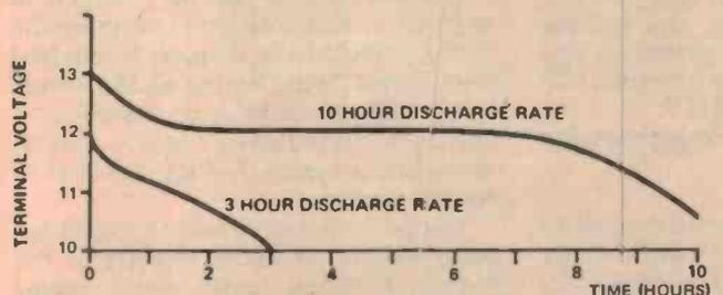
Figure 3. Typical discharge characteristics of a 12 V (nom.) nickel-cadmium battery (usually consisting of 10 cells in series).
