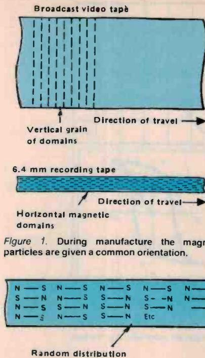
Figure 1. During manufacture the magnetic particles are given a common orientation.
