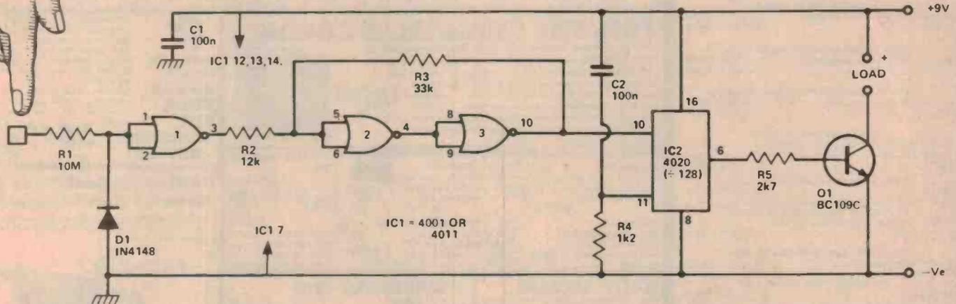
**THIS TOUCH SWITCH** is designed to provide on/off switching for 9 V battery operated equipment having a current consumption of up to 100 mA. It has a single touch contact which is briefly touched in order to change from on to off or vice versa. The circuit is operated by stray pick-up of mains hum which is coupled to the input of Gate 1 (which, like the other three gates employed in the unit, is connected to act as an inverter) via R1 when the input contact is touched.
