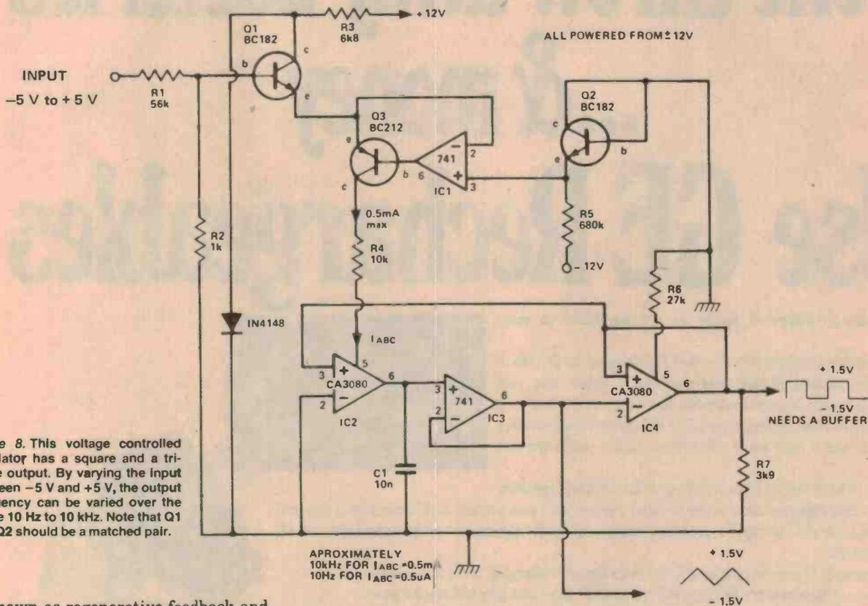
Figure 8. This voltage controlled oscillator has a square and a triangle output. By varying the input between  $-5\text{ V}$  and  $+5\text{ V}$ , the output frequency can be varied over the range  $10\text{ Hz}$  to  $10\text{ kHz}$ . Note that Q1 and Q2 should be a matched pair.
