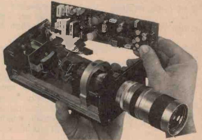
All the electronics for a new closed circuit TV camera are on a single printed circuit board.
