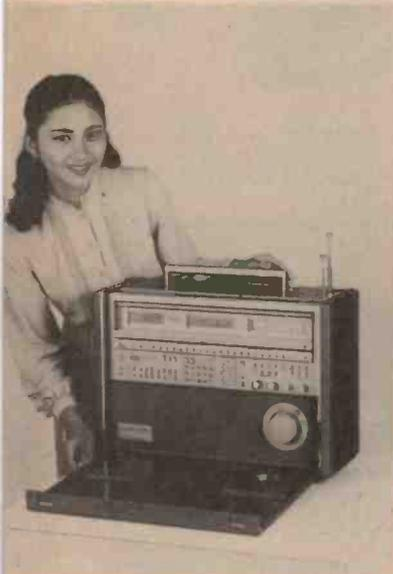
The RF-9000 has a phase-locked-loop synthesiser and double conversion super heterodyne circuitry which allows tuning in 100Hz steps on the long, medium and short wave bands and 10 kHz steps on
