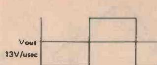
and finishing on axis crossings of the sinusoid. The CA3080 is configured here as a voltage comparator, used to detect these axis crossings and to produce a square wave output which then drives a binary divider (IC3). The divider produces a 'divide by sixteen' output which is high for eight sinewave cycles and then low for the next eight. This signal is then used to gate ON and OFF the sinewave.
