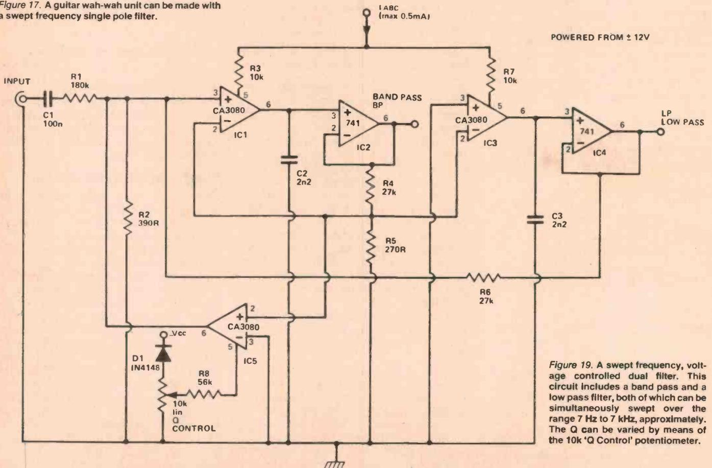
Figure 19. A swept frequency, voltage controlled dual filter. This circuit includes a band pass and a low pass filter, both of which can be simultaneously swept over the range 7 Hz to 7 kHz, approximately. The Q can be varied by means of the 10k 'Q Control' potentiometer.
