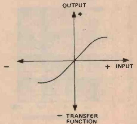
Figure 5. Transfer function of the Figure 3 circuit.
