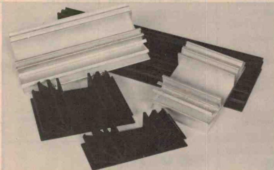
This heatsink, made locally by Rod Irving Electronics, is available in a variety of lengths, both anodised and unanodised. It measures 105 mm wide overall and the centre section is 35 mm wide by 5 mm thick. There are five fins on each side and a 220 mm length (anodised) has a thermal rating around 1°C/watt in free air. See Rod Irving Electronics, 425 High Street, Northcote Vic. 3070. (03)489-8131.
