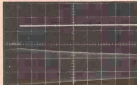
Dynamic characteristics. Expansion ratio — 1 : 1.5; Channel 1 input — 1 kHz tone burst; Channel 1 output is upper trace in each picture; Channel 2 input — 1 kHz steady state sine wave; Channel 2 output is lower trace in each picture. Left picture shows attack time ('scope on 50 ms/div.). Centre picture shows FAST release time ('scope on 200 ms/div.). Right picture shows SLOW release time ('scope on 200 ms/div.).
