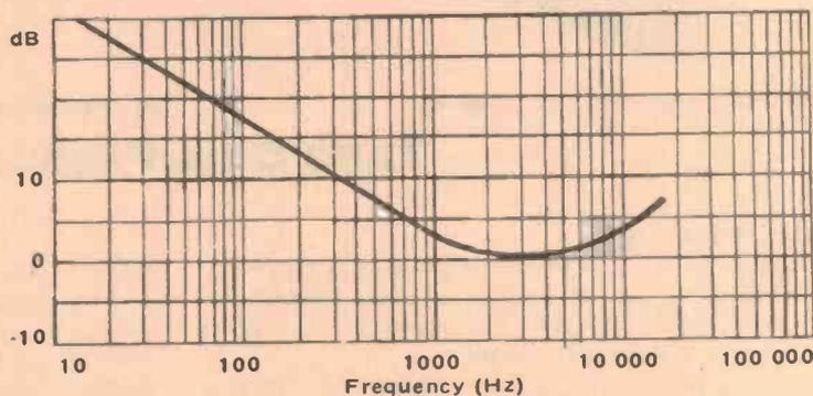
Figure 10. Theoretical response of the replay amplifier.
