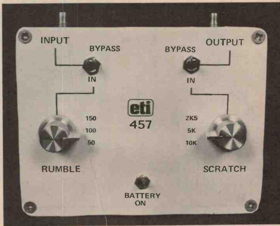
It is desirable to only modify enough of the amplifier's frequency response to reduce the problems, therefore we have included switchable cutoff frequencies for each filter. High frequency hiss can usually be removed with the 10 kHz filter while cracks will probably need a lower frequency cutoff.
