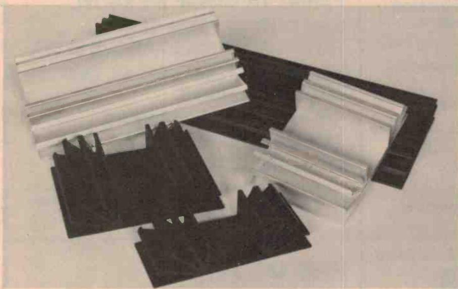
This heatsink, made locally by Rod Irving Electronics, is available in a variety of lengths, both anodised and unanodised. It measures 105 mm wide overall and the centre section is 35 mm wide by 5 mm thick. There are five fins on each side and a 220 mm length (anodised) has a thermal rating around 1°C/watt in free air. See Rod Irving Electronics, 425 High Street, Northcote Vic. 3070. (03)489-8131.
