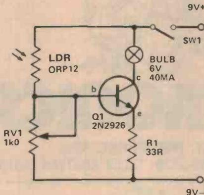
Since the circuit will have to operate in widely differing light levels, it is necessary to control the sensitivity of the circuit and this is accomplished by RV1. In high ambient light levels the value of RV1 should be low, this means that the transistor will remain switched off until the light level created by the match goes above this level. In low light levels the value of RV1 will be high.
