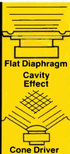
The most obvious difference... between the new Technics honeycomb disc speaker system and conventional speaker systems is that the speaker units are flat instead of conical. This flat sound radiating surface at last puts an end to all of the distortions inherent in the traditional cone-shaped design. Cone shaped drivers suffer from something called the 'cavity effect' which causes peaks and dips in the upper end of the driver's frequency range.
