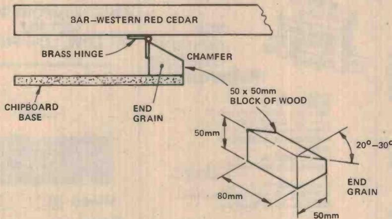
Figure 3. Hinging arrangement for the receiver antenna baseboard.
