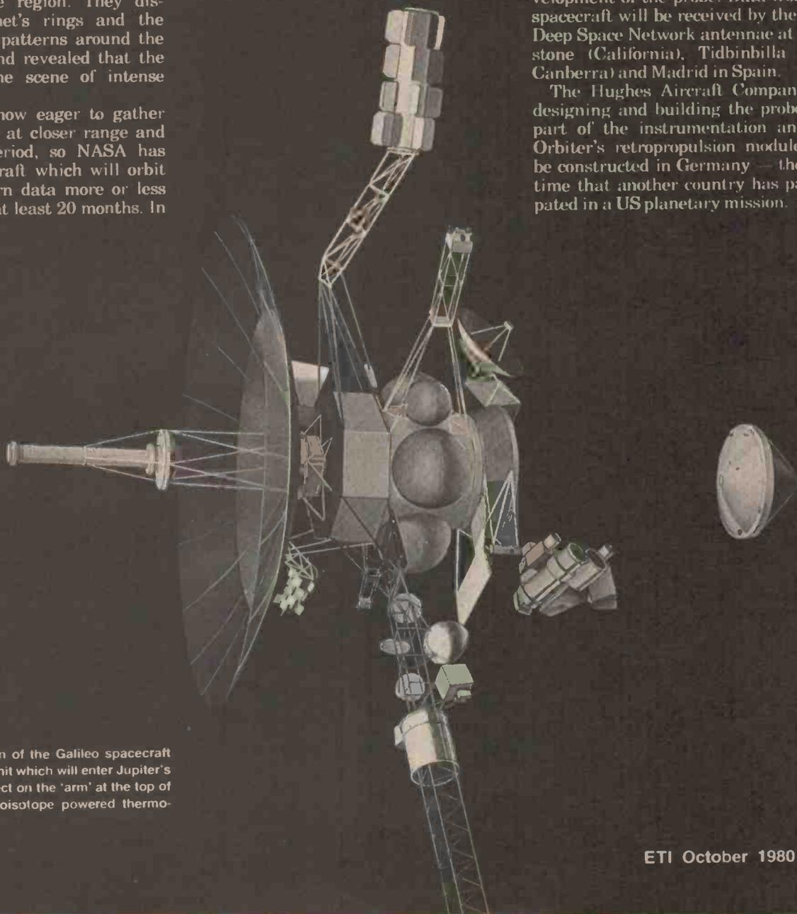
An artist's impression of the Galileo spacecraft releasing the Probe unit which will enter Jupiter's atmosphere. The object on the 'arm' at the top of the picture is a radioisotope powered thermoelectric generator.
