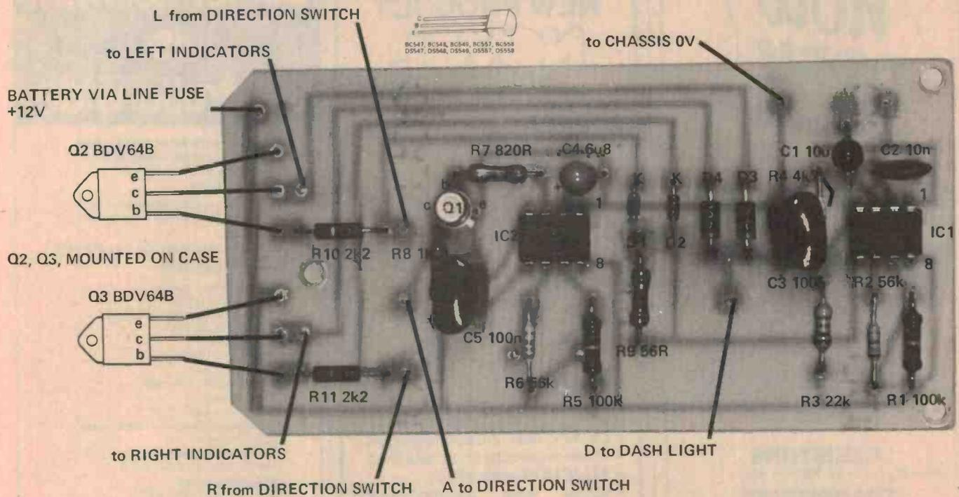
Component overlay and external component connections.
