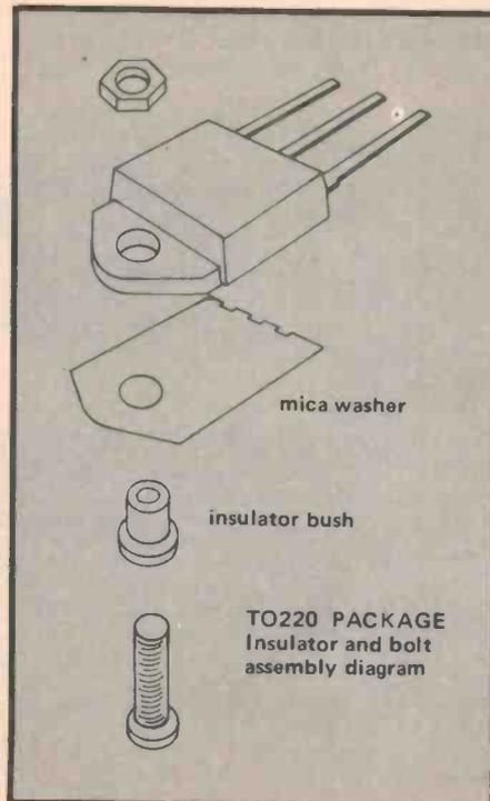
as shown in the photo of the prototype. The cases of these transistors are connected to the collectors and must therefore be insulated from the diecast lid. Mount the transistors using a mica or plastic insulator and plastic sleeves as shown in the diagram. Use an ohmmeter to check that there is an open circuit between the collectors and the diecast lid after the transistors are mounted.
