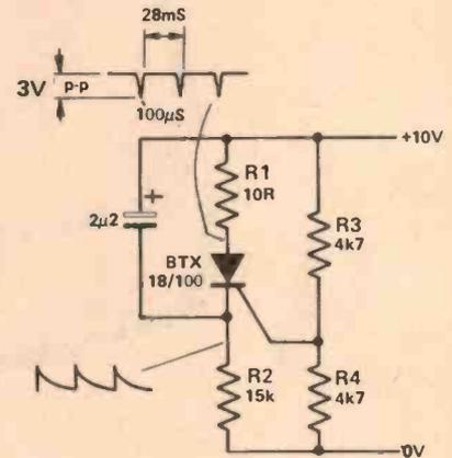
The circuit can be voltage controlled by altering the gate voltage, but this will also alter the output voltage. Another cunning circuit from Phillip Denniss of Chippendale, NSW.
