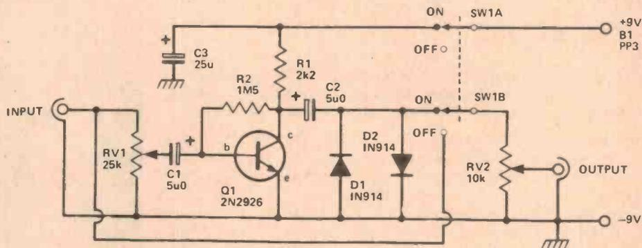
taken to the input and amplified by Q1 which is connected in the common emitter mode. This transistor will considerably increase the audio level and this is applied via a dc blocking capacitor, C2, to the two silicon diodes D1 and D2.
