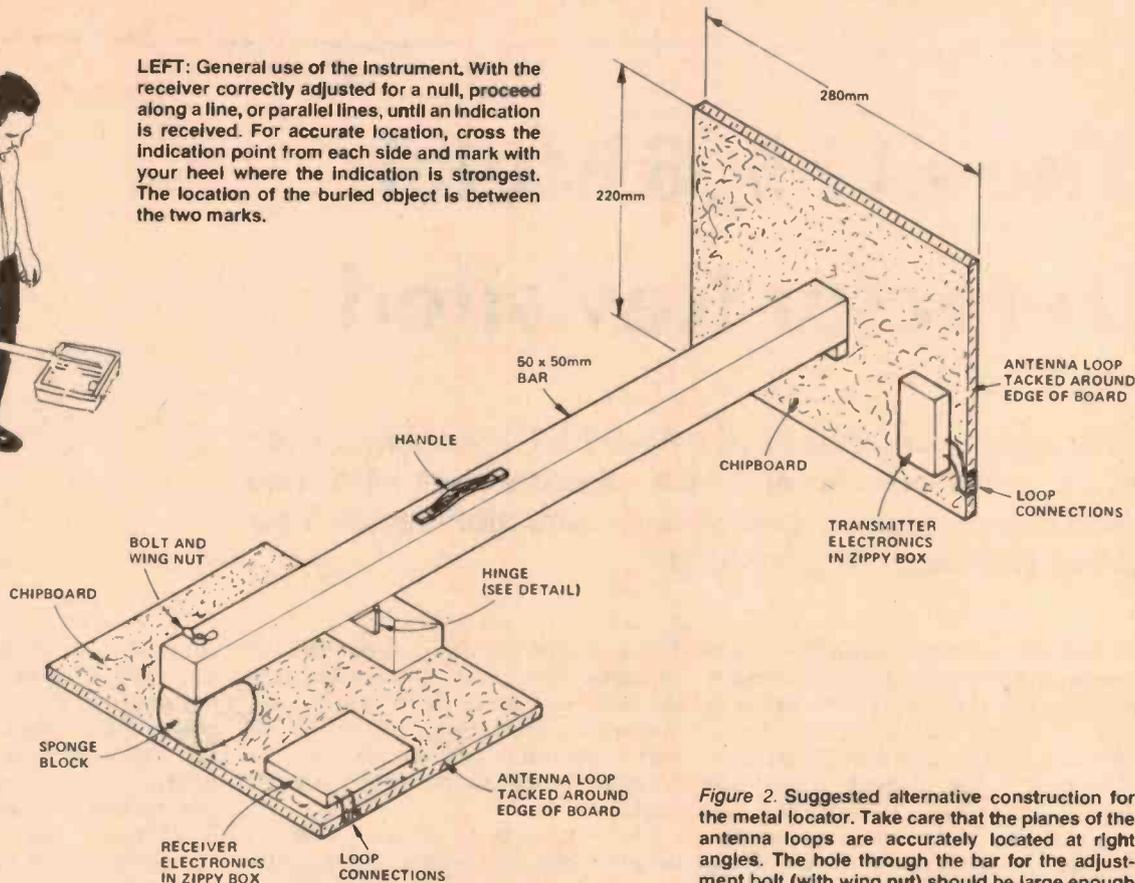
Figure 2. Suggested alternative construction for the metal locator. Take care that the planes of the antenna loops are accurately located at right angles. The hole through the bar for the adjustment bolt (with wing nut) should be large enough to clear the bolt when the receiver baseboard is fully angled towards the bar.
