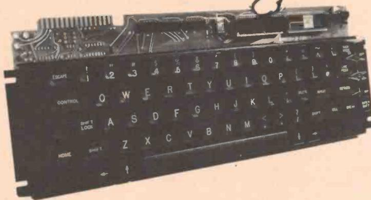
General Instrument's Keyboard Division has combined state-of-the-art microprocessor technology with the reliability and simplicity of capacitive keys to create a highly flexible, low cost keyboard for OEM's and hobby projects.
