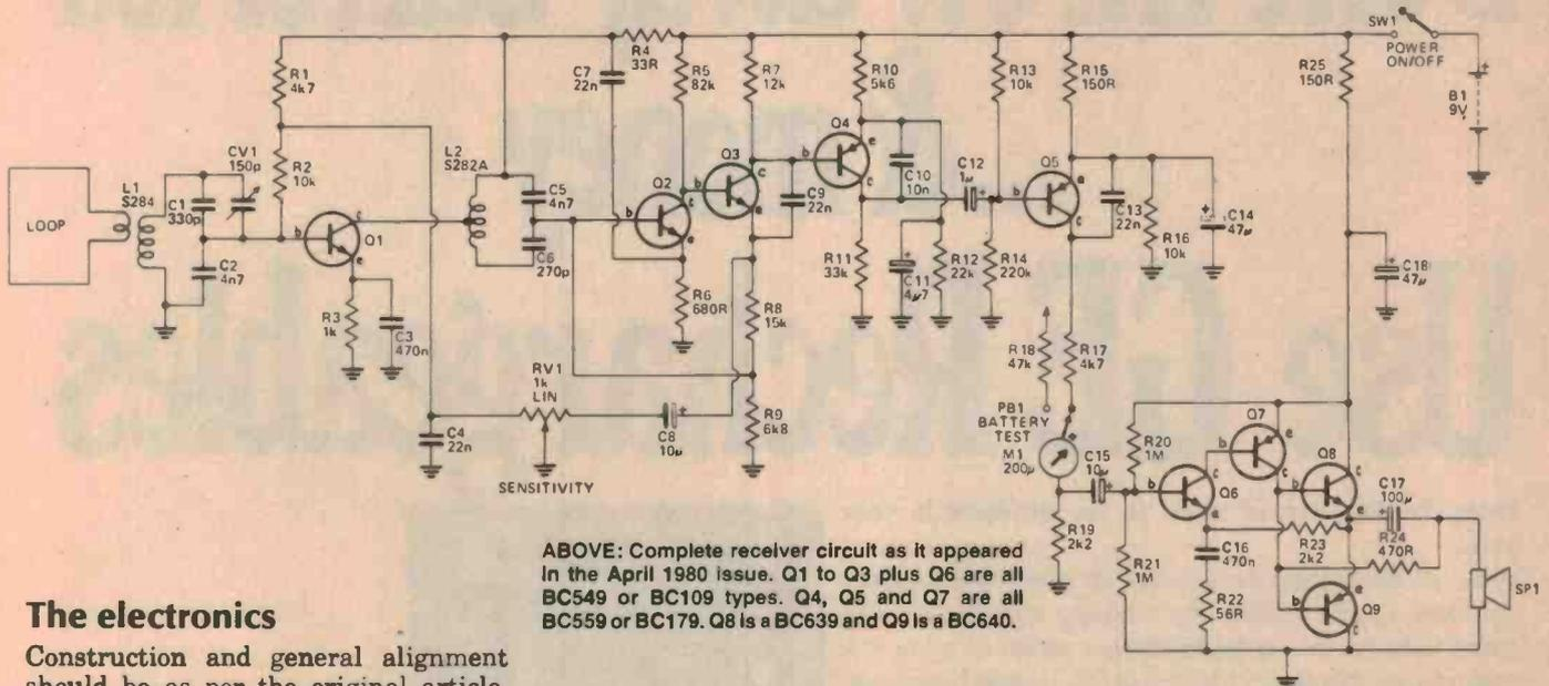
ABOVE: Complete receiver circuit as it appeared in the April 1980 issue. Q1 to Q3 plus Q6 are all BC549 or BC109 types. Q4, Q5 and Q7 are all BC559 or BC179. Q8 is a BC639 and Q9 is a BC640.
