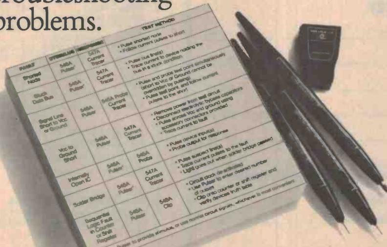
**Logic Pulser** stimulates IC's in-circuit for testing. Automatically drives the circuit to its opposite state. No unsoldering components or trace cutting. \$125-\$190.
