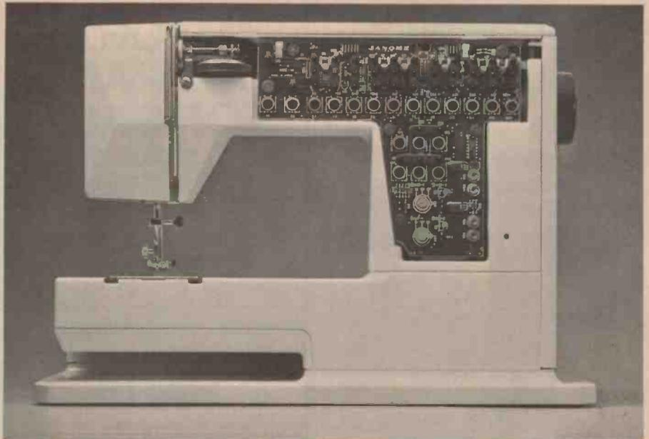
Behind the side panel is an array of LEDs to show which stitches have been selected.
