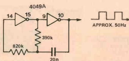
The oscillator circuit uses two inverters in a 4049 IC and oscillates at about 50 Hz. The frequency can be varied by changing the values of the capacitor and the two resistors.
