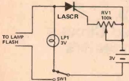
This is a simple but effective slave flash unit for use with the fusible type of flash bulb (magnesium filament). The firing is done using an LASCR which is an SCR which is triggered by light. When the master flash gun fires the LASCR is switched on, allowing current to flow to the flash bulb. The bulb blows and the LASCR turns off (as the supply is then not connected).
