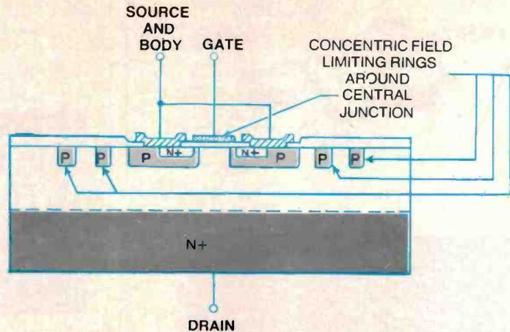
Figure 5. In the vertical DMOS device, current flows from the drain (N+) into the n-epitaxial layer (N-) then flows horizontally through a channel into the source. The concentric rings of p-type material around the main junction help improve the current capability and reduce the on-resistance. This form of construction achieves significantly higher voltage and current ratings compared to prior power MOSFETs.
