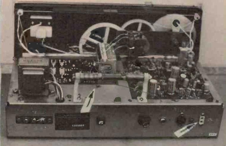
The upper arrow shows the four-section Band A loopstick coil. The arrow at lower right shows the STANDBY socket — now used for the loop input.
