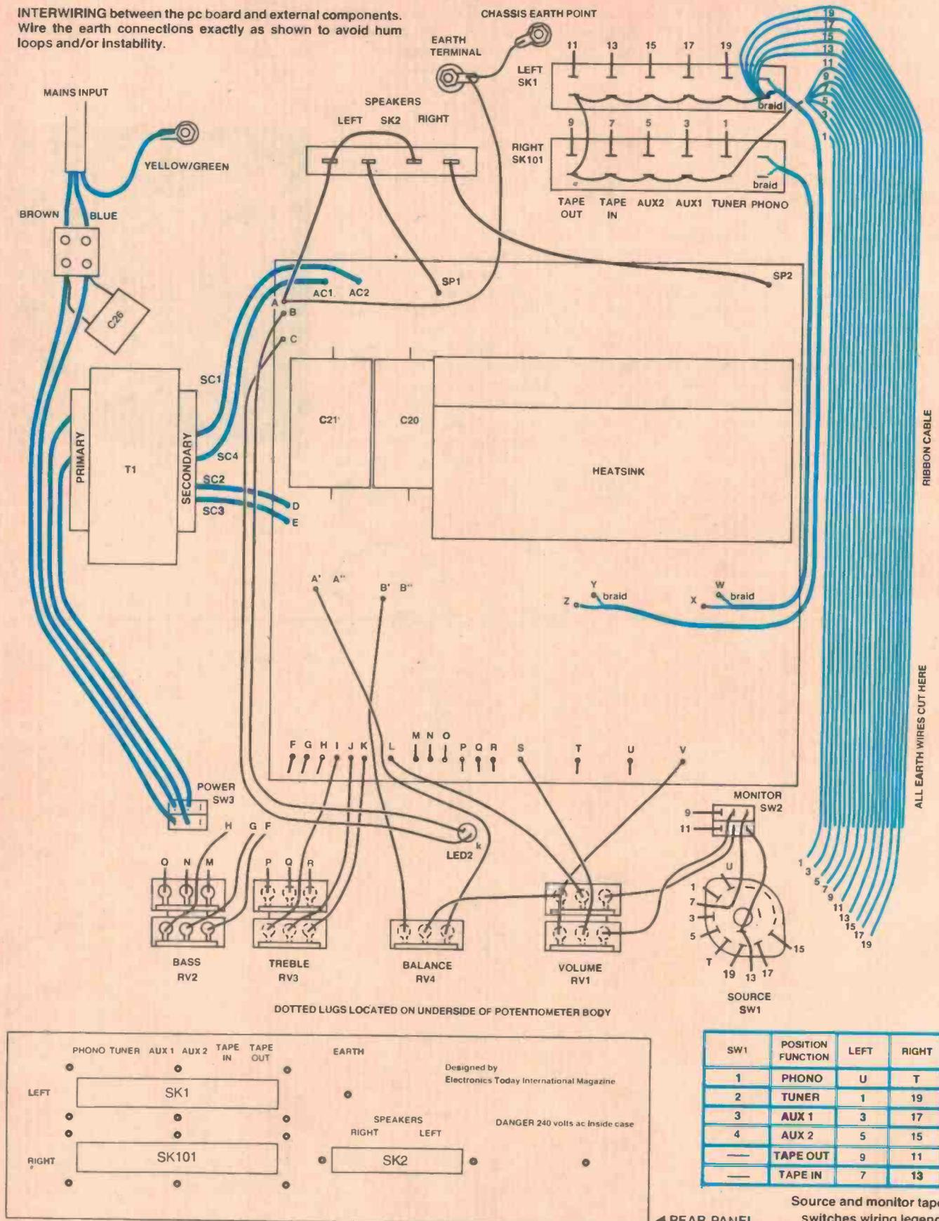
DOTTED LUGS LOCATED ON UNDERSIDE OF POTENTIOMETER BODY
