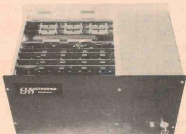
11 slot backplane, fully card guided, 15 amp power supply, fan, key switch, bench mount, rack mount, anodised aluminium, 5 edge connectors standard, S-100 Bench Kit \$345, S-100 Rack Kit \$306, 6800 Bench Kit \$370.00, 6800 Rack Kit \$330, Assembled prices add \$100.
