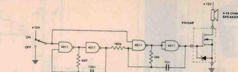
Figure 12. This two-tone alarm is a variation of the Figure 11 circuit.
