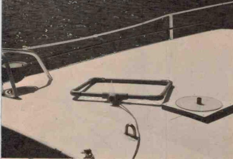
The completed loop assembly has a perspex pointer attached so that the direction may be read off a compass rose on the loop mount.
