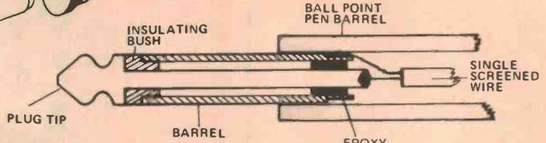
ABOVE: assembling the phono plug barrel and tip into the pen barrel.
