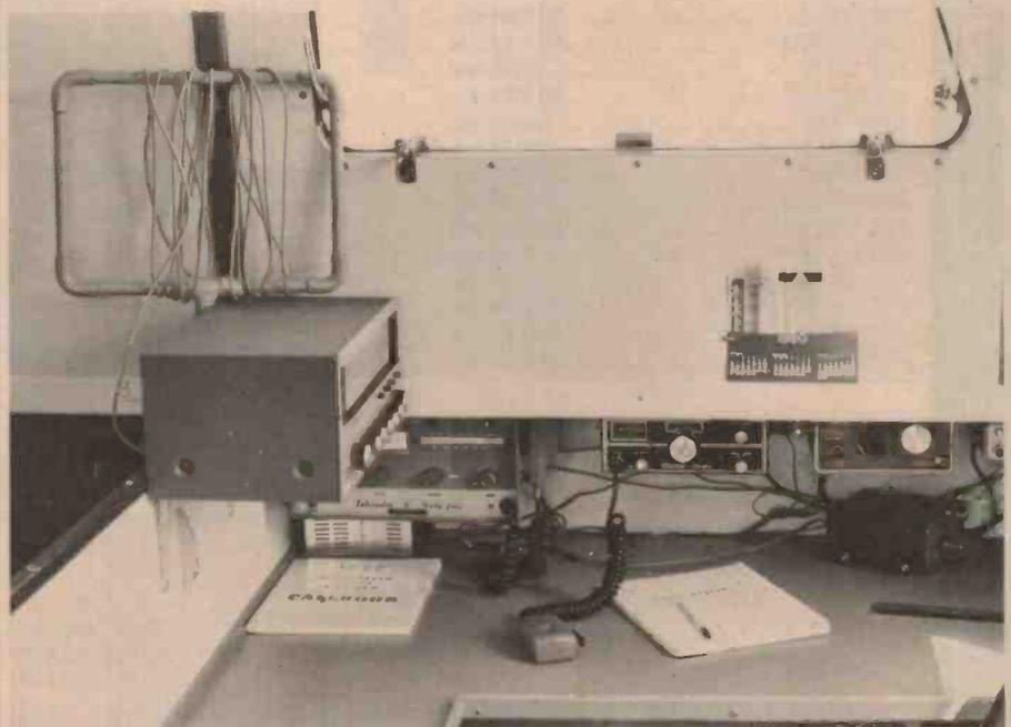
The 'electronics' aboard the Nikki includes a Teleradio 65 marine transceiver, a Swan 40m monoband rig, 146 MHz FM rig, a depth sounder and assorted other items.
