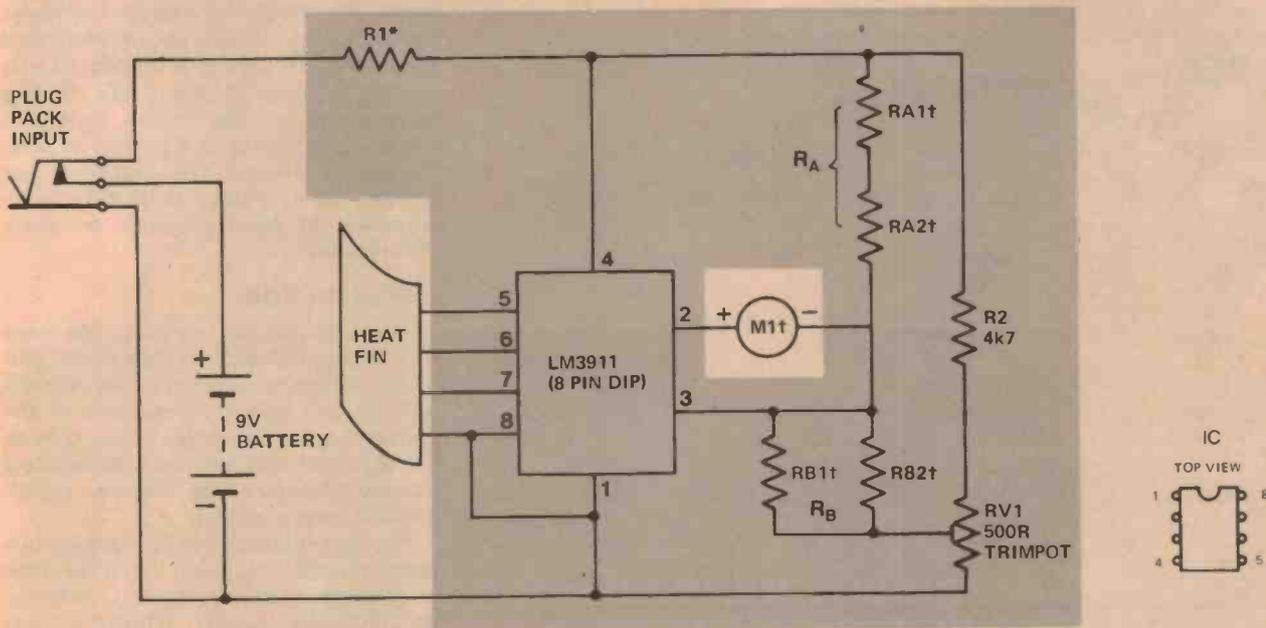
\*R1 = 470R (¼W or ½W) for 9 V operation; 1k8 for 12 V battery (11 - 15 V) operation.
