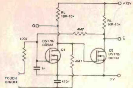
Figure 10. Capacitive touch switch will cycle on and off if finger is held on the sensor.
