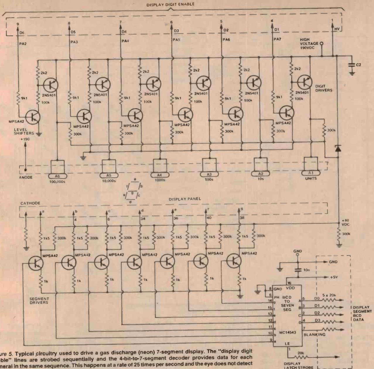
Figure 5. Typical circuitry used to drive a gas discharge (neon) 7-segment display. The "display digit enable" lines are strobed sequentially and the 4-bit-to-7-segment decoder provides data for each numeral in the same sequence. This happens at a rate of 25 times per second and the eye does not detect any flicker.
