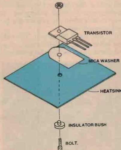
Assembling a flatpack transistor to a heatsink.
