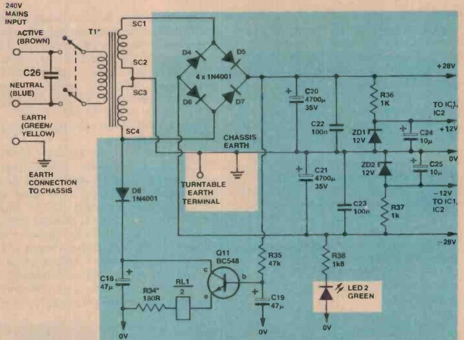
Power supply and speaker anti-thump circuit. A transformer with a secondary rated at 20 - 0 - 20 V at 1.5 A will provide 20 W per channel. For 5 W per channel operation, a 12 - 0 - 12 V at 0.8 A transformer is required. In the latter case, reduce the values of R36 and R37 to 390 ohms each and short out R34.
