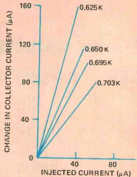
Figure 2. The transfer function of a superconducting transistor. Note the linearity of the function.
