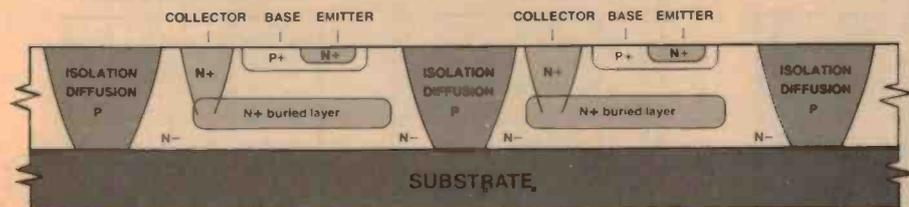
Figure 1. Cross-section of two transistors in a transistor array IC.
