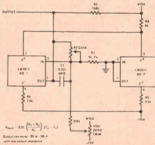
$$V_{\text{OUT}} = 0.01 \left( \frac{R_1 + R_2}{R_1} \right) (T_2 - T_1)$$
