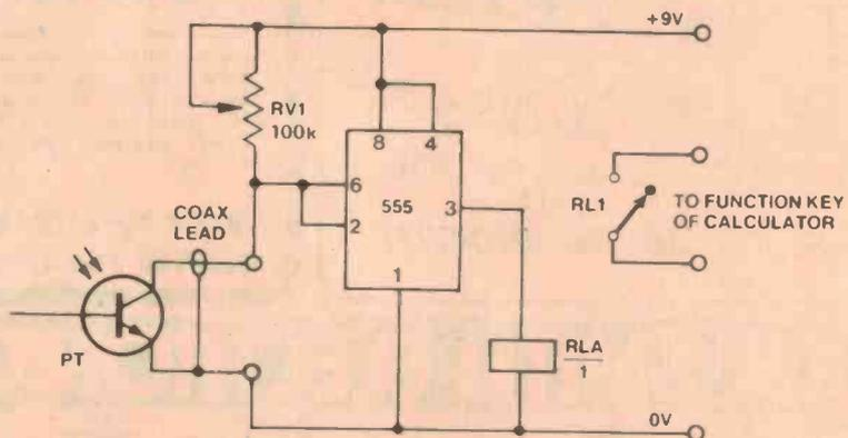
The circuitry is simplicity itself. The potentiometer (RV1) provides control of the triggering point of the 555. The function key you use on the calculator will depend on the make — the Tandy EC-201 (like most) will totalise using the = key, others employ the + key.
