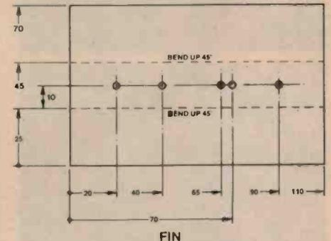
HEATSINK DIMENSIONS FOR 25 WATT UNIT.
