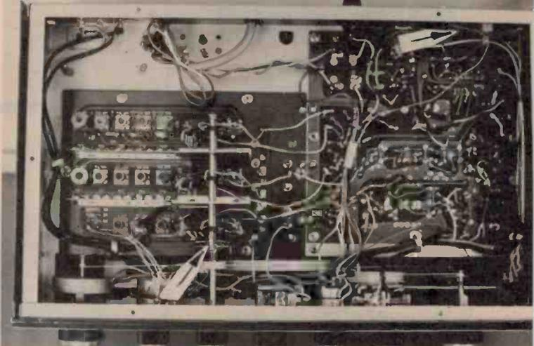
Underside view of the receiver. Arrow at lower left indicates which wafer section on the bandswitch is re-wired; at right, the STANDBY socket.
