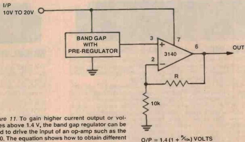
Figure 11. To gain higher current output or voltages above 1.4 V, the band gap regulator can be used to drive the input of an op-amp such as the 3140. The equation shows how to obtain different outputs.
