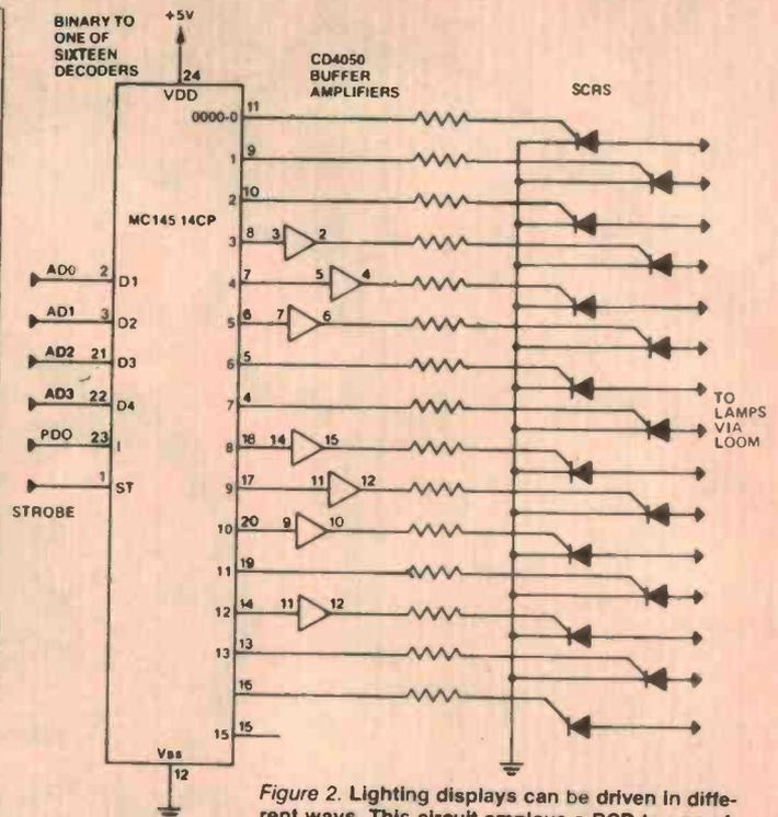
Figure 2. Lighting displays can be driven in different ways. This circuit employs a BCD-to-one-of-sixteen decoder driving an array of SCRs which control the lamps.
