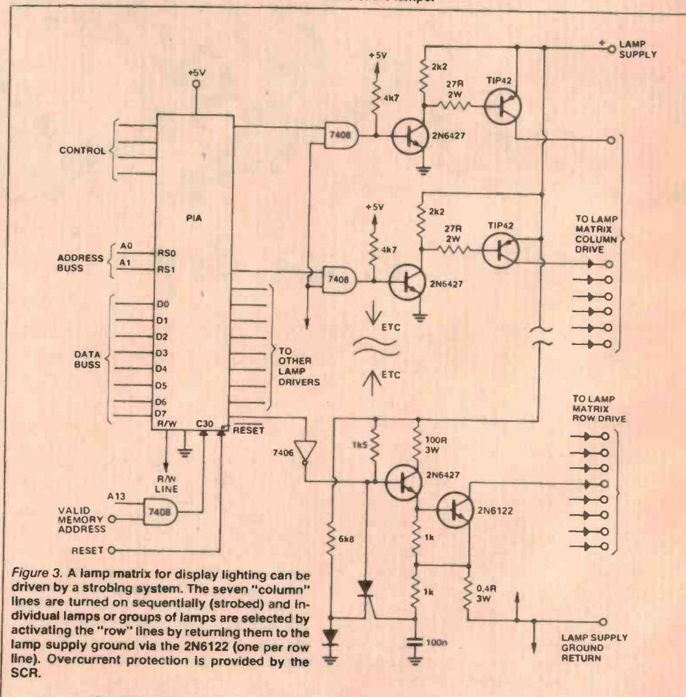
Figure 3. A lamp matrix for display lighting can be driven by a strobing system. The seven "column" lines are turned on sequentially (strobed) and individual lamps or groups of lamps are selected by activating the "row" lines by returning them to the lamp supply ground via the 2N6122 (one per row line). Overcurrent protection is provided by the SCR.
