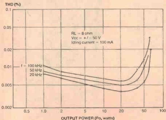
Figure 19. Distortion characteristics of the circuit in Figure 18.
