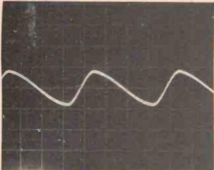
Waveform at the positive lead of C1, showing the 50 Hz ripple.
