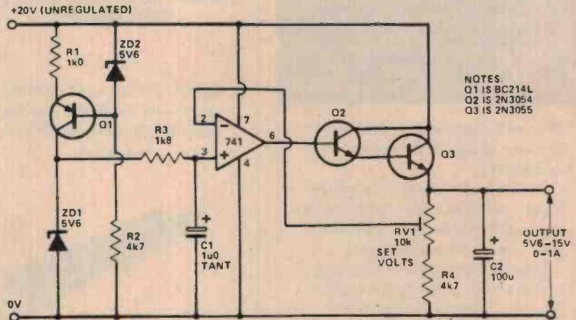
Figure 5. This circuit is a little more sophisticated and performs better than the Figure 4 circuit. This circuit will deliver up to 1 A output current, output voltage being variable between 5.6 V and 15 V. Thermal drift is near zero.
