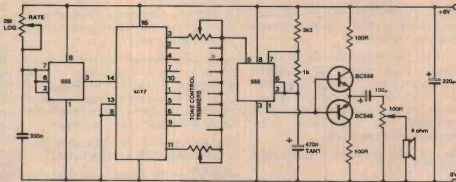
of the audio oscillator is fed to a complementary pair of transistors which drive a speaker for the audio output.
