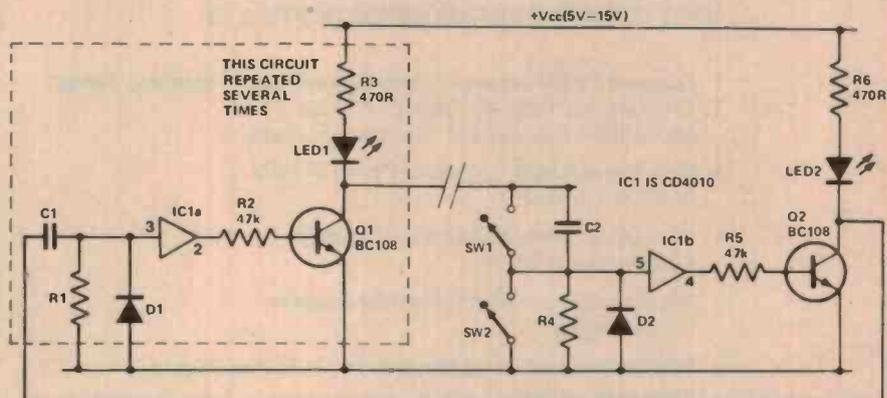
lower threshold. When it does, the output of IC1b will go low and Q2 will turn off. Then, C1 will charge via R6 and LED2, but the initial pulse will turn Q1 on via IC1a and LED1 will light. When C1 charges such that the input of IC1a goes below its lower threshold, Q1 will turn off, triggering the next inverter stage in the chain and so on, right
