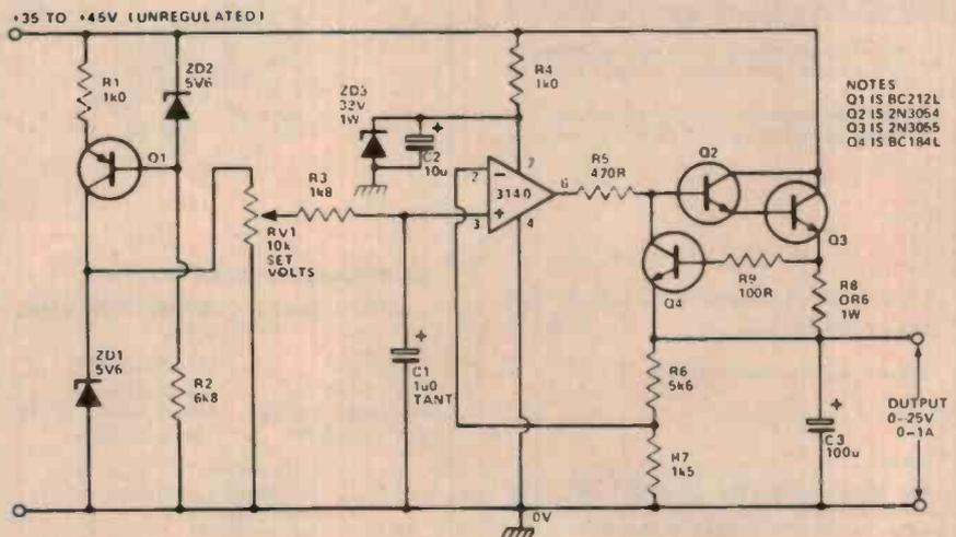
Figure 7. A further refinement is the addition of current limiting and overload protection. Q4 senses the voltage across R8 which is in series with the output. When the current exceeds 1 A, Q4
