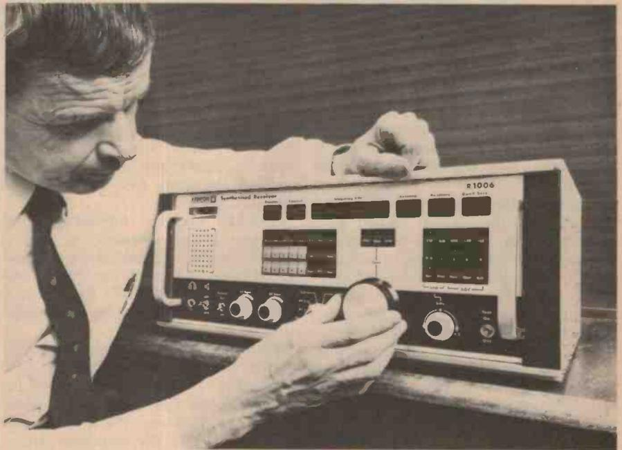
The Redfion R1006 receiver can control up to 99 remote receivers over any distance by ordinary telephone lines or radio links as appropriate.
