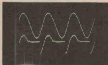
E) Same as pic (D) but with metal target near the search head. Note the increase in average dc level from the output of IC1b. The change in this signal is much larger for non-ferrous than for ferrous metals.
