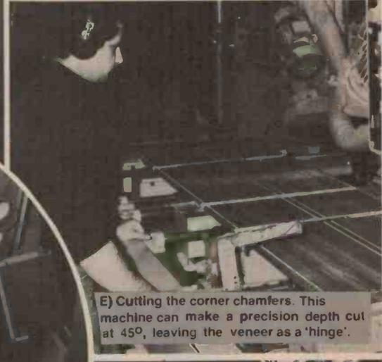
E) Cutting the corner chamfers. This machine can make a precision depth cut at 45°, leaving the veneer as a 'hinge'.
