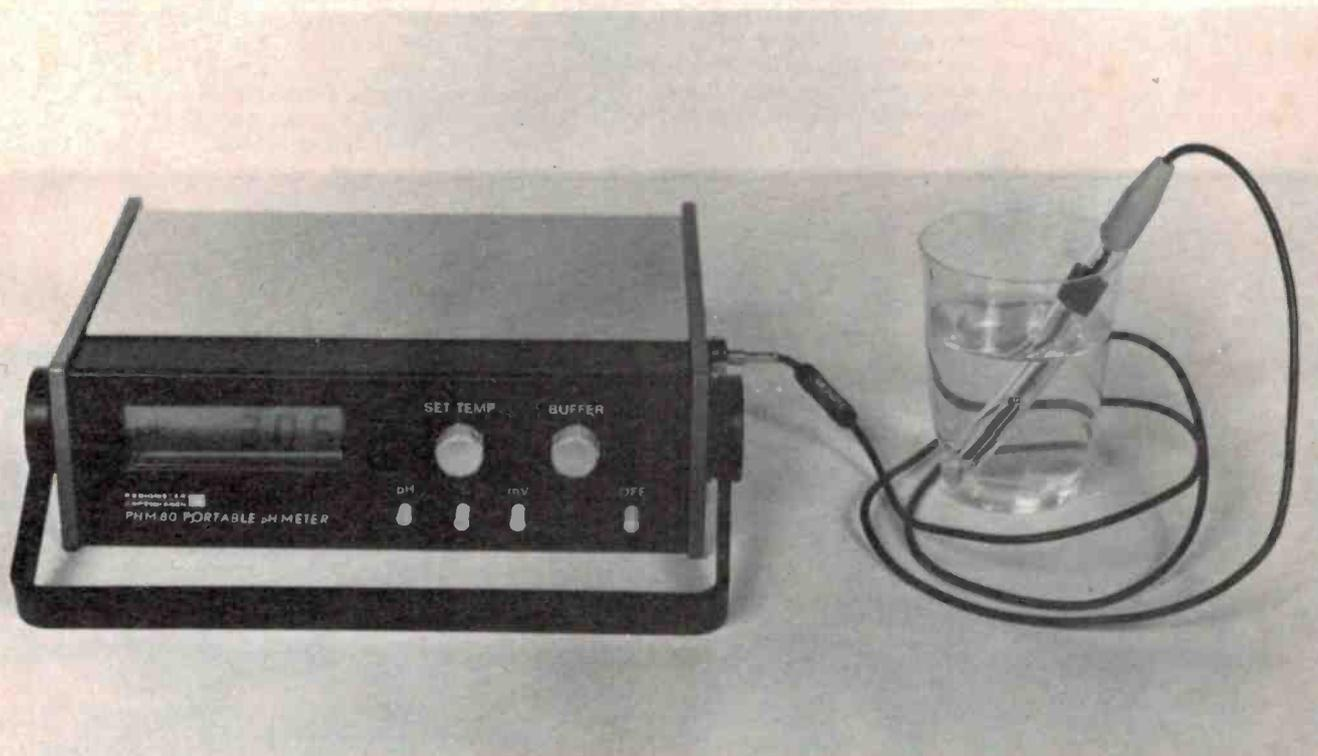
A high quality portable pH meter with a liquid crystal display that directly indicates the pH of the solution under test.
