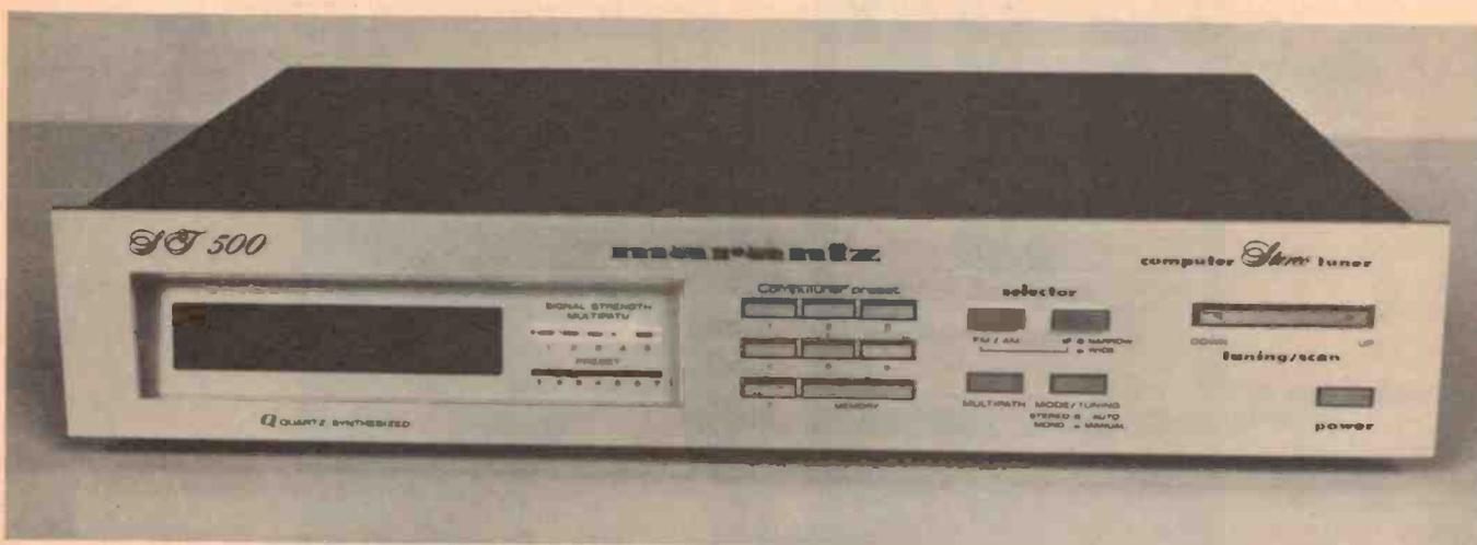
LARGE SCALE integration, generally in the form of the microprocessor, means that today's electronic equipment can be provided with features that not so long ago were only wild and impractical ideas in the minds of designers. The sophisticated tuning, preset and display features of the Marantz Computer Stereo Tuner are examples of the kind of elaboration that is now feasible.
