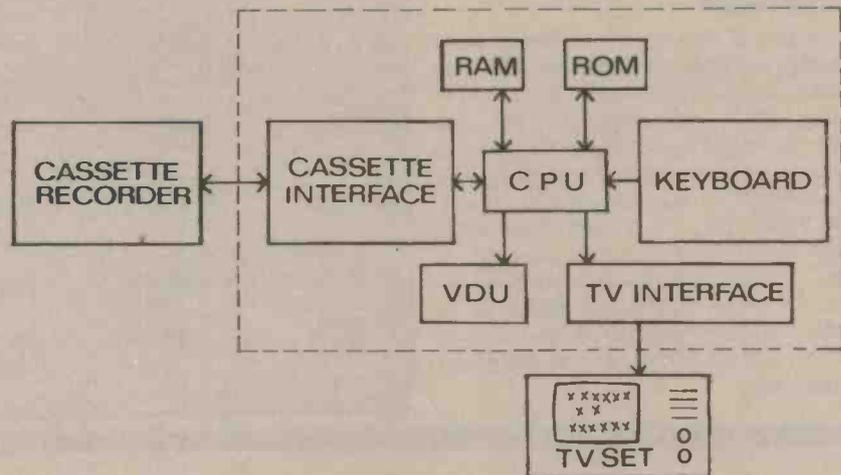
**CPU** stands for **Central Processing Unit**, home of the famous microprocessor. This part of the machine does all the thinking and corresponds to the 'clever bits' in a calculator.
