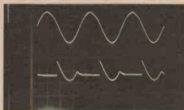
I) As per pic (G) but steel target held near search head. Note the decrease in average dc level of the signal at the output of IC1b, illustrating discrimination.
