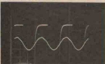
F) Received signal on emitter of Q2 (sine wave) superimposed on the output of IC4b. The phase difference between the two signals is adjustable through 180° by use of the course (TR1, TR2, TR3) and fine 'discriminate' controls. (Both traces 2 V/div, ac-coupled; time base 20 us/div).
