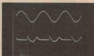
G) Top trace: received signal on emitter of Q2. Bottom trace: output of IC1b showing composite waveform of received signal 'mixed' with a dc level. Detector set to TR1 mode, discriminate control to 9. (Both traces 2 V/div, ac-coupled; time base 20 us/div).
