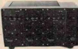
The new Ceitex Dimmer Rack — 12 channels, 2000 watts per channel in 3 x 4 way modules. This dimmer rack uses Flakey iron toroids for RF suppression — interference with audio systems is virtually non-existent. The Ceitex rack will drive either positive or negative control dimmer control desks — thus almost any dimmer control desk now available, will mate the Ceitex rack.
