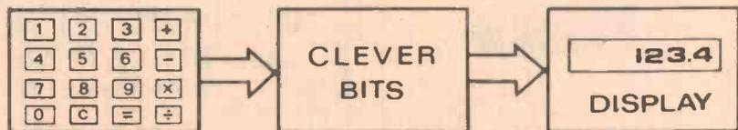
Figure 1. Block diagram of a simple four function calculator.
