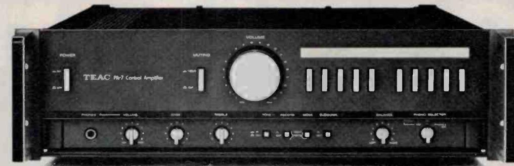
prevents the popping noise that would otherwise appear because of power surge when the unit is switched on and also prevents clicks when switching phono inputs.
