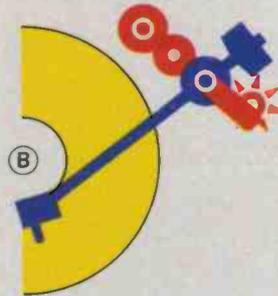
(B) Hitachi photo sensor tone arm return system with LED
