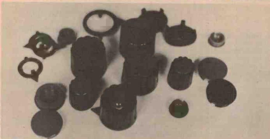
Collet knobs will fit where conventional grub-screw knobs will not. They are secured to a control shaft by a split sleeve and nut arrangement. These collet knobs, distributed here by Associated Con-
