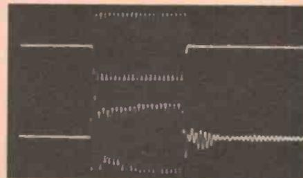
Tone burst response: left, at 100 Hz; centre, at 1 kHz; right, at 6.3 kHz.
