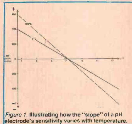
Figure 1. Illustrating how the "slope" of a pH electrode's sensitivity varies with temperature.
