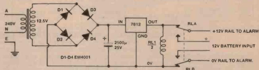
During mains failure, the 12 V supply rail from the regulator will discharge and the relay will drop out, connecting the supply rail for the alarm through to a 12 V battery.
