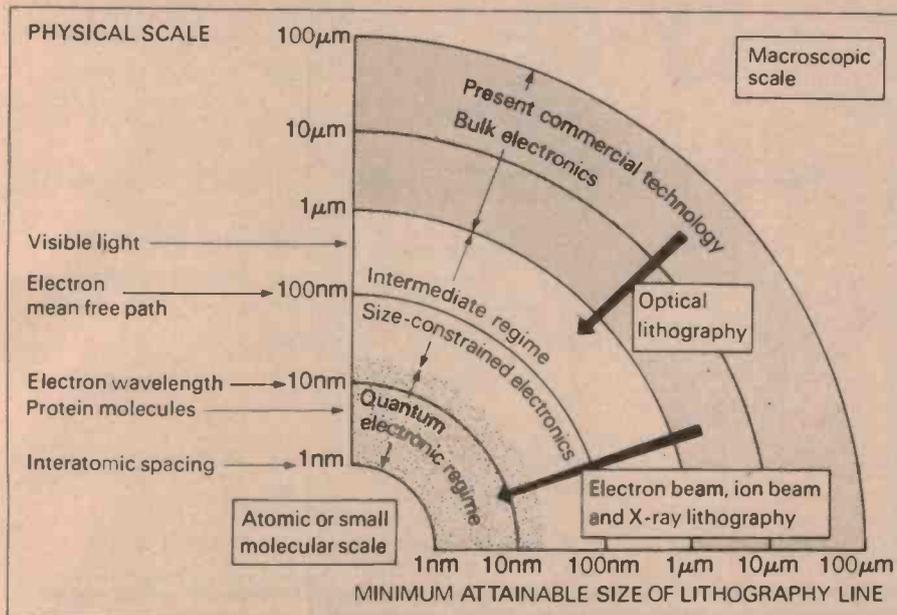
Figure 2. Orders of size for features in silicon-chip devices, showing sizes of lithography lines required.
