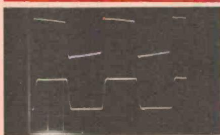
L) A more rigorous test shows the magnitude of the error signal with 10 kHz drive giving 20 V p-p output across a 2  $\mu$ F capacitive load. As before, lower trace is the module's output. The upper trace shows that, as expected, the error signal is much greater than with a resistive load, but still does not clip. This could safely be considered the worst realistic load from the point of view of TIM production. Scale for the error signal is again 200 mV/div.
