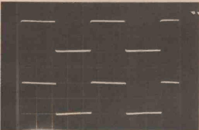
G) Square wave response of the ETI-477 module. Top trace is the 100 Hz input. Bottom trace is the resulting 20 V p-p output into an 8 ohm resistive load. The slight tilting of the output square wave occurs because of the high pass filter on the module's input and is therefore not a fault.
