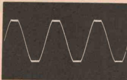
Figure 2. An amplitude-limited waveform — "clipping".
