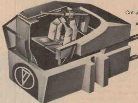
Cut-away section of a dual magnet Audio Technica cartridge.
