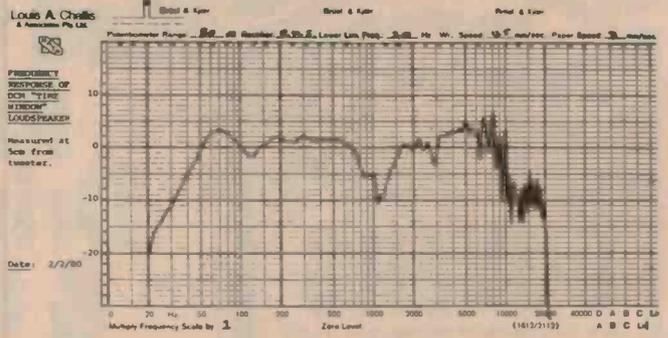
a series of some 15 well known loudspeakers when subjected to an impulse step response. DCM state that out of all of these systems tested the DCM Time Window provides the best response. Our own interpretation of the results they present is that the DCMs provide a performance that is as good as the best of the systems they evaluated and that the Quad electrostatic loudspeakers (which are generally regarded anyway as having a good transient response) appear to provide a comparable performance.
