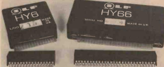
The U.K.-made ILP series of encapsulated audio modules should prove popular with audio enthusiasts. These plug-in modules make the assembly of a sound system quick and simple. Apart from preamps, a range of power amps are available ranging from 15 W to 240 W priced from around \$30 to \$150. Contact Electromark, 40 Barry Ave, Mortdale NSW 2223.
