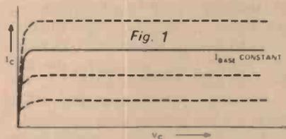
First, let's see how a constant current source works. Transistor Q1 and associated components provide the constant current source for the probe. Figure 1 shows the collector characteristics of a typical silicon transistor. They show that, if you hold the base current constant, the collector current will
