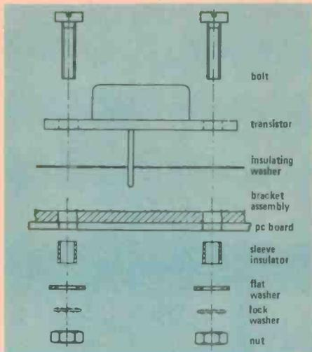
General diagram for mounting a TO3-cased device to a heatsink bracket and pc board assembly.
