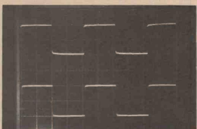
H) Square wave response of the ETI-477 with a 1 kHz input. In this case the load is 8 ohm resistive.
