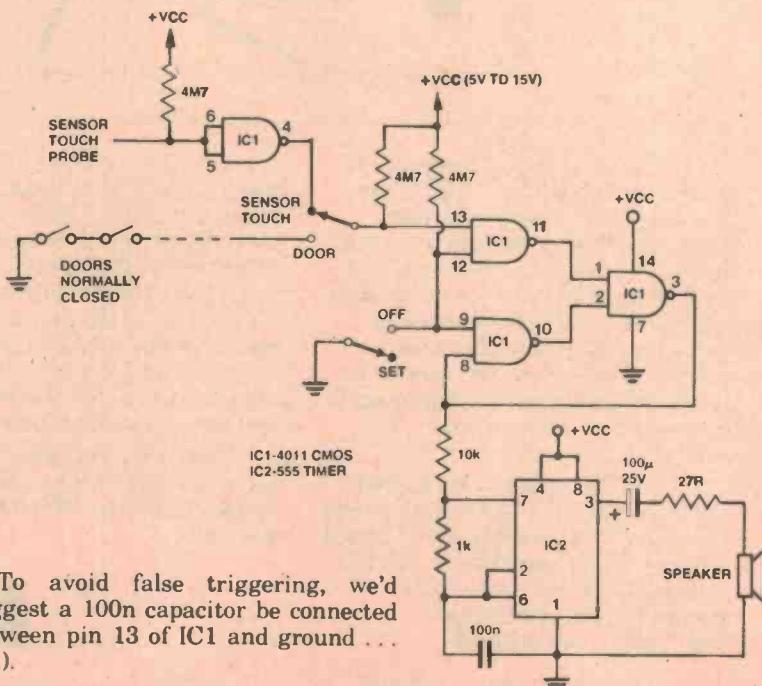
(To avoid false triggering, we'd suggest a 100n capacitor be connected between pin 13 of IC1 and ground . . . Ed.).
