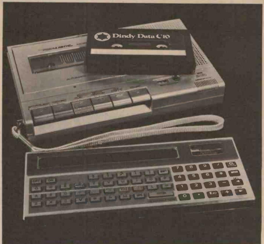
Tandy's TRS-80 pocket computer uses two four-bit microprocessors which communicate with each other via a common data buss. The first MPU accepts and interprets instructions, then passes them along to the second processor for execution.
