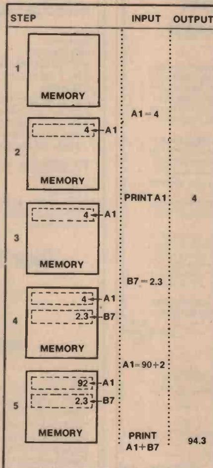
Figure 1. Memory at various steps during a calculation.
