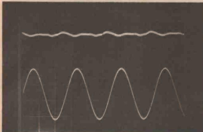
C) Total harmonic distortion, this time at 20 kHz, 10 W RMS output. The amplifier distortion is just becoming discernible above the resolution of the F242A. Note the difference between the distortion waveform shown here and that shown in B. THD here is around 0.004%.
