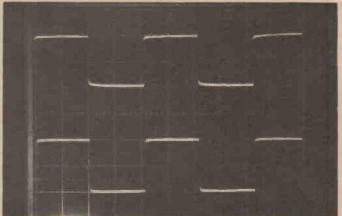
H) Square wave response of the ETI-477 with a 1 kHz input.
