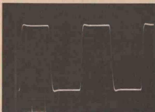
J) Oscilloscope photograph showing the module's performance into a reactive load. At left is the output waveform of the module, driven with a 10 kHz square wave. Output load is 2  $\mu$ F in parallel with 8 ohms. Note that there is no sign of oscillation or instability. This is a very strenuous test as normally the reactive load would exhibit a series resistance which limits the charge and discharge times for the capacitance.
