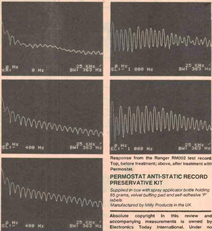
Response from the Ranger RM002 test record. Top, before treatment; above, after treatment with Permostat.
