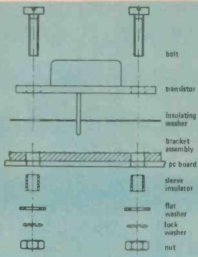
General diagram for mounting a TO3-cased device to a heatsink bracket and pc board assembly.
