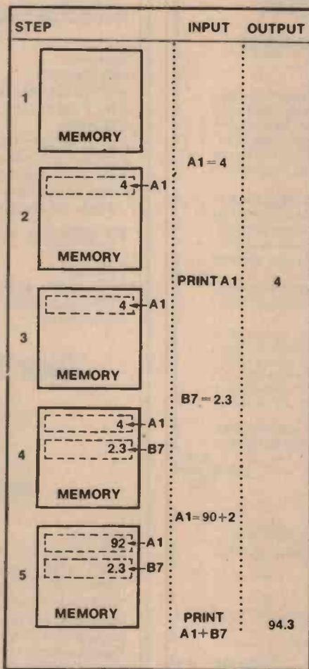
Figure 1. Memory at various steps during a calculation.
