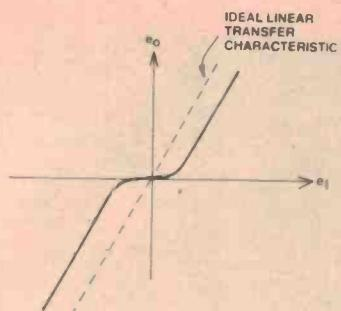
Figure 3. Illustrating the relationship between  $e_o$  and  $e_i$  for a bipolar output pair operated without bias, as shown in Figure 1. The result is 'crossover distortion'.
