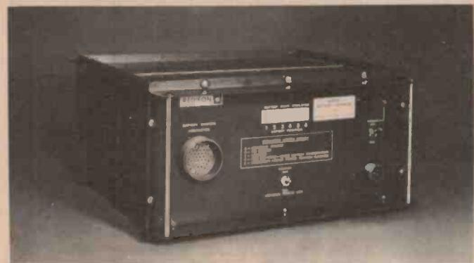
batteries impaired by the continual use of trickle chargers, which produces a gradual degradation in performance. They can be used as part of a planned maintenance programme to recondition such deteriorated NiCad batteries.
