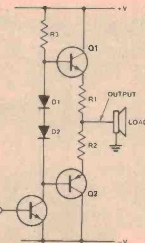
Figure 4. A common method of linearising the relationship between  $e_i$  and  $e_o$  in an output stage is to apply bias using two diodes (D1 and D2).
