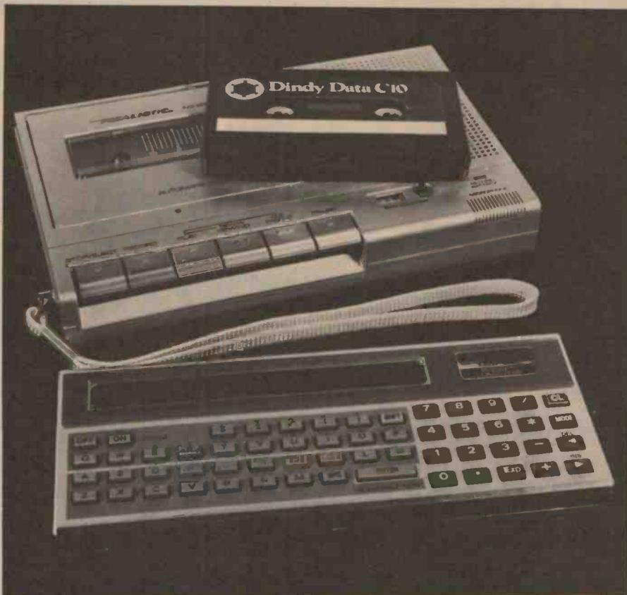
Tandy's TRS-80 pocket computer uses two four-bit microprocessors which communicate with each other via a common data bus. The first MPU accepts and interprets instructions, then passes them along to the second processor for execution.
