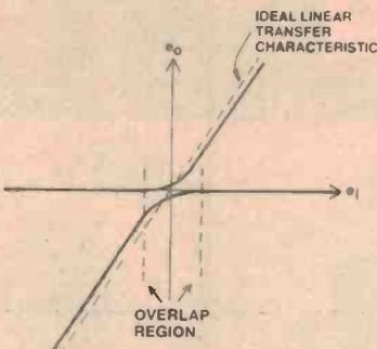
Figure 5. How the application of bias to the output devices affects the relationship between  $e_i$  and  $e_o$  — the 'transfer characteristic'.
