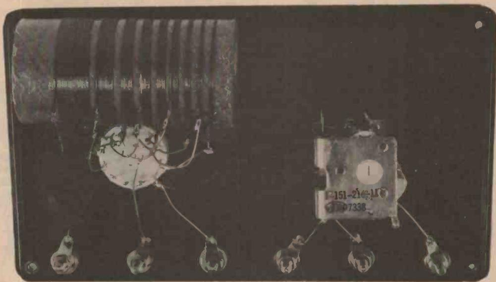
365 pF, which is quite adequate, but are about twice the size of the modern types and may have a 9 mm diameter shaft, necessitating a 'shaft reducer' extension piece. We'll have to leave that up to you.
