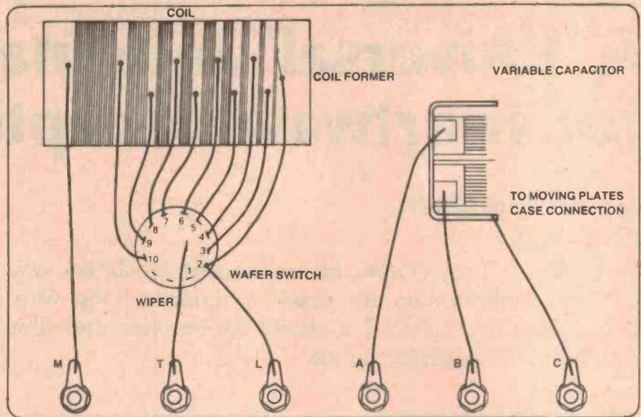
Wiring diagram. Compare this with the photograph on the right.
