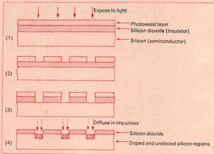
Figure 1. Photo-lithographic process for making integrated circuits: (1) An oxide layer is grown on the silicon wafer, followed by a photosensitive layer; (2) The photoresist is exposed and the pattern etched; (3) The exposed oxide layer is etched away; (4) The photoresist is stripped away and impurity atoms are diffused into the silicon layer. The final structure is equivalent to an array of planar transistors.
