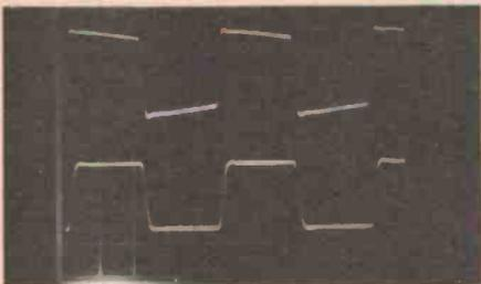
L) A more rigorous test shows the magnitude of the error signal with 10 kHz drive giving 20 V p-p output across a 2  $\mu$ F capacitive load. As before, lower trace is the module's output. The upper trace shows that, as expected, the error signal is much greater than with a resistive load, but still does not clip. This could safely be considered the worst realistic load from the point of view of TIM production. Scale for the error signal is again 200 mV/div.
