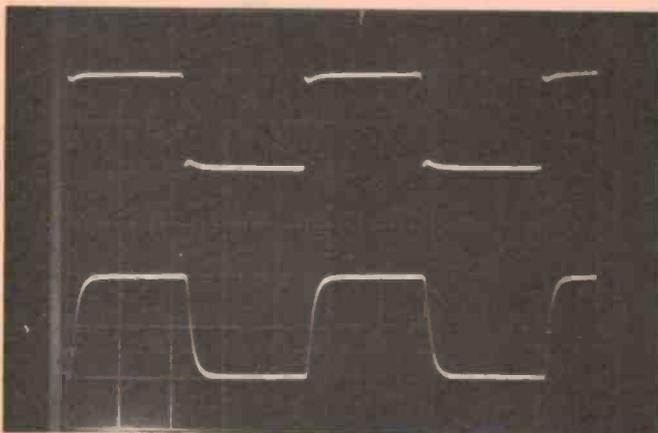
J) Square wave response at 10 kHz. Top trace is the input. The glitch after the rising and falling edges is due to a fault in the square wave generator. The harmonics produced, however, are well above the cutoff frequency of the input RC filter on the module. As a result, the output is a perfect band-limited square wave (lower trace).
