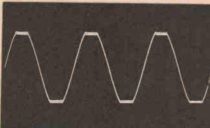
Figure 2. An amplitude-limited waveform — "clipping".
