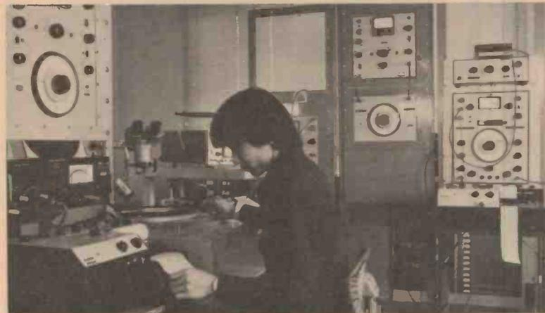
Measuring the response of a cartridge in the development laboratory.
