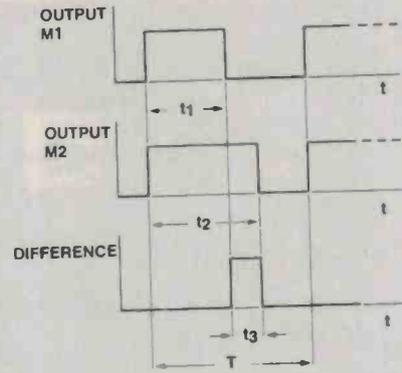
Figure 2. Illustrating how the output signal,  $t_3$ , is obtained. If  $t_2$  is fixed and  $t_1$  varies with variations in humidity,  $t_3$  will vary in direct relation to  $t_1$ .
