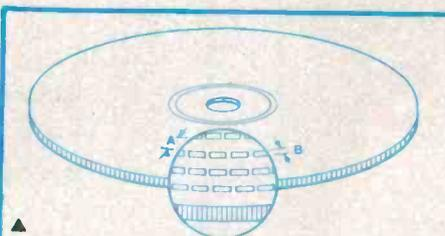
Information is encoded on Philips' Discovision disc as tiny pits only 0.6 μm wide (dimension B) by 0.1 μm deep, spaced 1.6 μm apart (dimension A).
