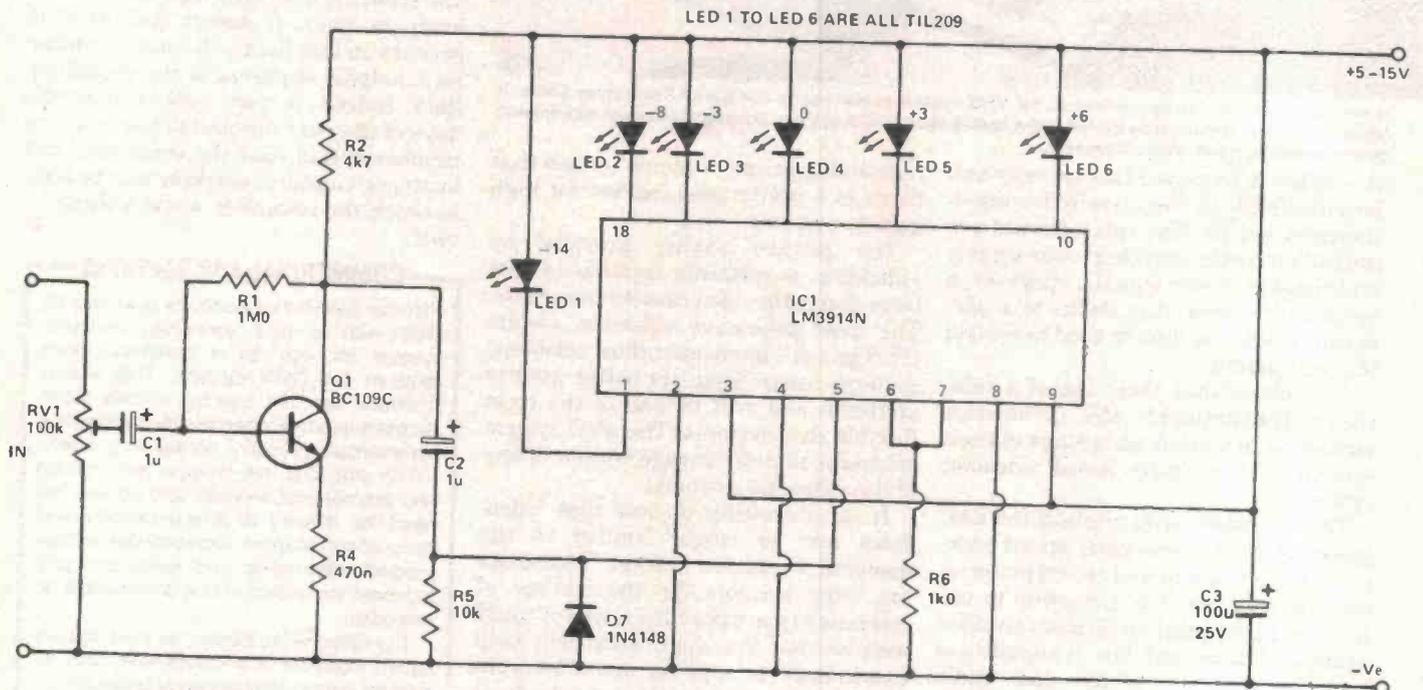
THIS VERY SIMPLE peak reading VU meter circuit uses six LEDs to indicate six signal levels. Indicators are provided at -14, -8, -3, 0, +3, and +6 dB or any other levels having the same spacing (e.g. -17, -11, -6, -3, 0, and +3 dB, if preferred). Only about 24 mV peak-to-peak is needed in order to activate the highest LED indicator, and so the circuit is sufficiently sensitive to be used with any normal item of audio equipment.
