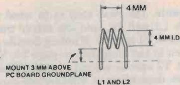
L1 AND L2 ARE WOUND WITH 22 SWG TINNED COPPER WIRE, THREE TURNS EACH, ON A 4 MM DIAMETER FORMER, AND SET TO A LENGTH OF 4 MM EACH. MOUNT THEM SUCH THAT THE LOWER PART OF EACH COIL IS ABOUT 3 MM ABOVE THE BOARD GROUNDPLANE.
