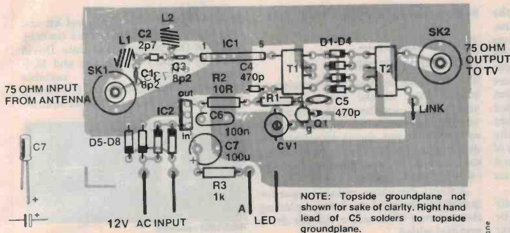
NOTE: Topside groundplane not shown for sake of clarity. Right hand lead of C5 solders to topside groundplane.
