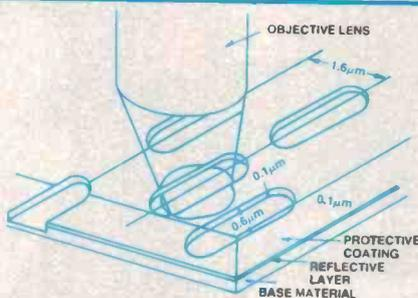
A laser reads the length of the microscopic pits, which contains the encoded information.
