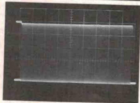
Transient overload recovery test (IHF-A-202)
