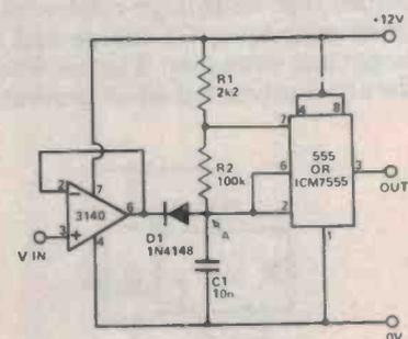
Figure 6. The voltage-controlled astable produces an output only when  $V_{in}$  exceeds two-thirds supply (8 V in this example).
