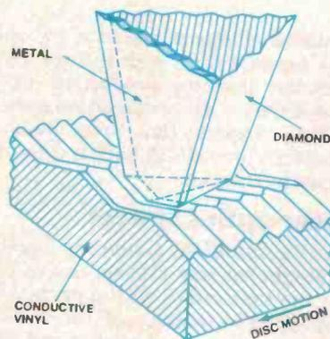
RCA's Selectavision system uses a metal-diamond composite stylus running in modulated grooves on the disc. The stylus tip is only 5 μm by 2 μm and the groove pitch is 2.6 μm. Wear is said to be its biggest problem.
