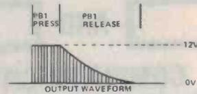
Figure 12. A method of amplitude-modulating the pin 3 output of the 555 astable in music and sound generator applications.
