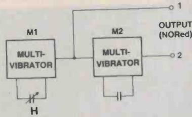
Figure 1. Block diagram of the circuit technique employed in the humidity meter. Two synchronised multivibrators provide an output signal which varies proportional to variations in relative humidity. 'H' is the humidity sensor.
