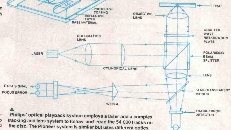
Philips' optical playback system employs a laser and a complex tracking and lens system to follow and read the 54 000 tracks on the disc. The Pioneer system is similar but uses different optics.
