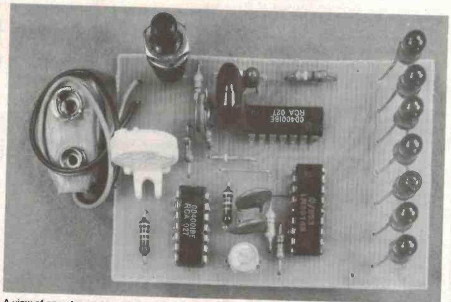
A view of one of our prototype humidity meters featuring the LED display. Note the sensor mounted on the board at the left, adjacent to the battery clip.
