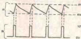
Figure 9. Alternative method of producing a non-symmetrical fixed ratio output from the 555 astable.
