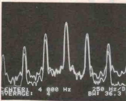
Measured performance of Dick Smith direct drive auto return turntable showing the trackability on the Shure TTR-103 test record.
