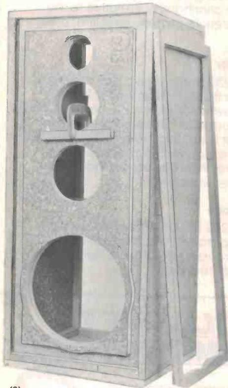
(3) The second (smaller) front baffle is attached next — screwed and glued in place.
