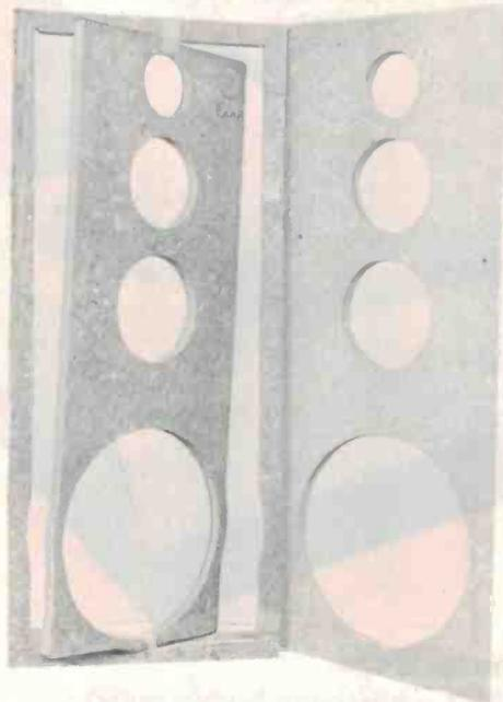
(1) Two identical front panels are cut and then a cut is made around one about 25 mm in from the edge, allowing for the woofer lip.
