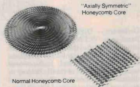
The 'axially symmetric' honeycomb core of the driver diaphragms compared to normal 'linear' honeycomb structure. The honeycomb core is sandwiched between thin aluminium sheets.
