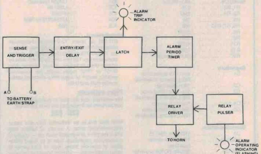
Figure 1. Block diagram of the ETI-330 car alarm showing the basic functional blocks of the circuit.
