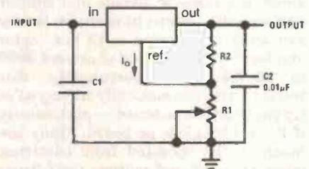
Showing how a three-terminal regulator can be arranged to have an adjustable output. The variable resistor, R1, here is replaced by a transistor in our regulator circuit below left.
