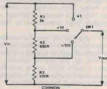
Figure 2. The method of designing this simple switched attenuator is explained in the text.
