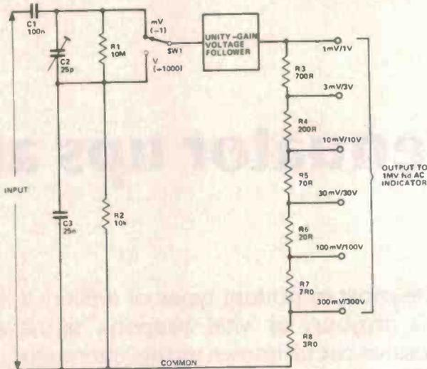
Figure 5. Typical attenuator sections of an ac millivoltmeter.
