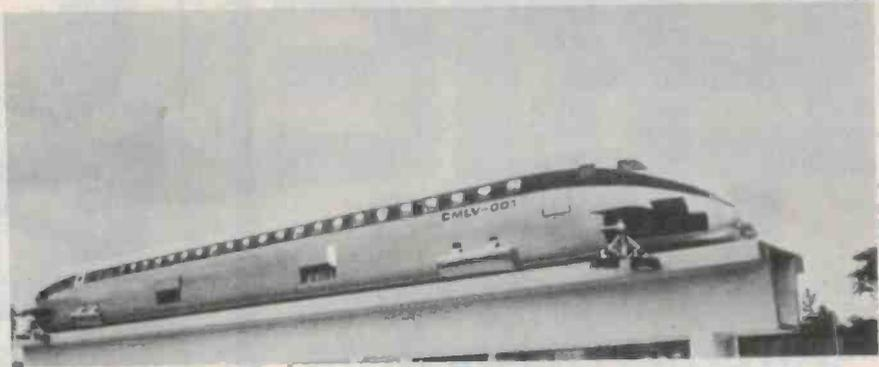
An outdoor view of the NRC-DME model, showing the deployed outrigger wheels and luggage compartments. (Photo: Pat Grieche, DME Canada.)
