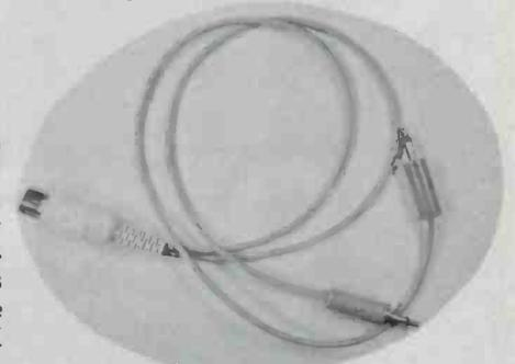
Make up a cassette interface cable. The DIN plug goes into the 660 and the two jacks to the recorder. To distinguish between the TAPE IN and TAPE OUT cables we made one longer and with a different coloured jack to the other.
