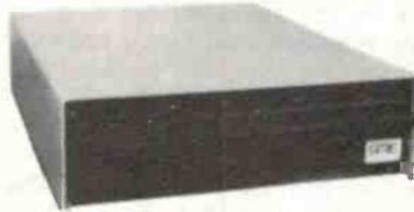
A new product from SME is a dual drive package available in a bench mount or rack mount style. It uses dual 8" double sided, double density compatible drives, in a low profile cabinet. Built in power supply, line filter & cooling fan. Drive interface is via a 50 way centronic type connector. This unit is supplied assembled & tested.
