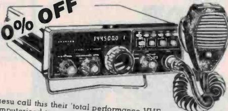
Yaesu call this their 'total performance VHF computerised transceiver.' And total performance it is! As the top-of-the-line Yaesu 2M family you'd expect a lot. You get FM, SSB CW over the full 2M band, with two VFO's, four memory channels, scanning, digital readout, hi/lo power switch & much, much, more. To sum it up in one word, supetb!
