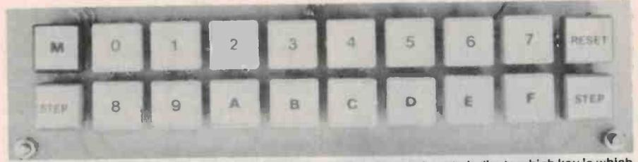
The FES-310 keyswitches we used have Scotchcal labels stuck on them to indicate which key is which.
