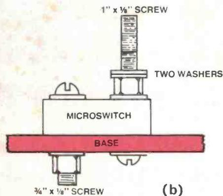
Figure 8. Locating and mounting the microswitches for the 'touch' or 'bump' sensor ring. (a) Orient the actuators clockwise around the base. (b) The 1" long screw is passed up from under the base through the outermost mounting hole. The  $\frac{3}{4}$ " screw passes downwards through the innermost hole. Use washers under each screw head and nut.
