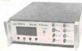
This unit has four different programmable outputs, clock controlled switch-ons/switch-off times selected days from the seven or eight day cycle can be "skipped". Ideal for operating air conditioning, fish tanks, hi-fi systems, tape recorders, slide and movie projectors and laboratory control etc.
