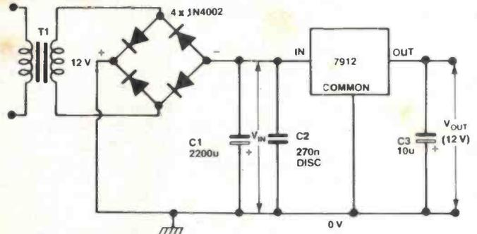
Figure 12. Circuit using a common three-terminal negative regulator.
