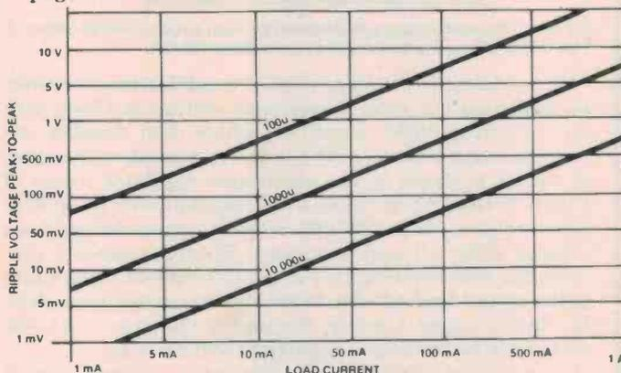
Figure 6. Filter capacitor selection chart (see text).
