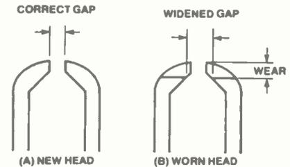
Figure 4. Effect of head wear on gap width (Teac).
