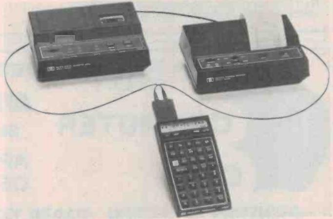
ment instruments. It connects the internal electronics of the machine to the HP-IL loop, allowing the machine to communicate with other devices on the loop and with the HP-41 controller.
