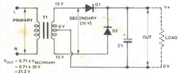
Figure 2. Basic single-ended supply using a centre-tapped transformer.
