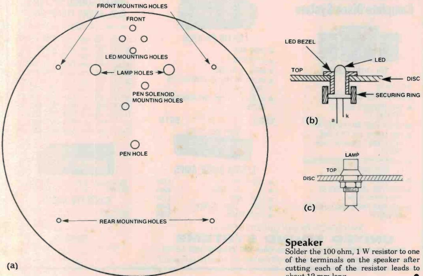
Figure 9. The inner plastic disc. (a) How to identify the various holes. (b) How to mount the LEDs and lamps.
