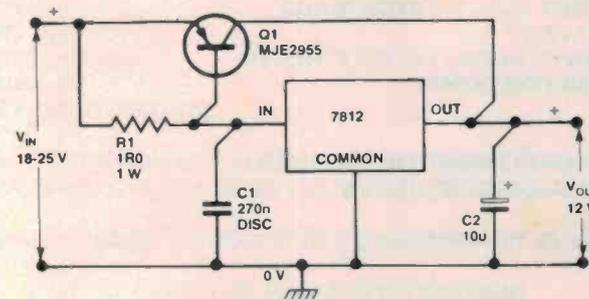
Figure 17. Increasing the output current capacity of a three-terminal regulator. This will deliver 5 A at 12 V.
