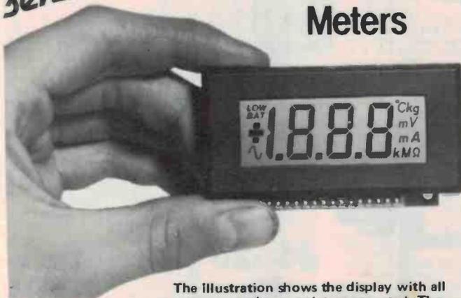
The illustration shows the display with all segments and annunciators actuated. The unit is housed in a neat plastic escutcheon. The DPM measures 72x36mm overall. Digital height - 15mm (can be read at distances up to 10 metres).
