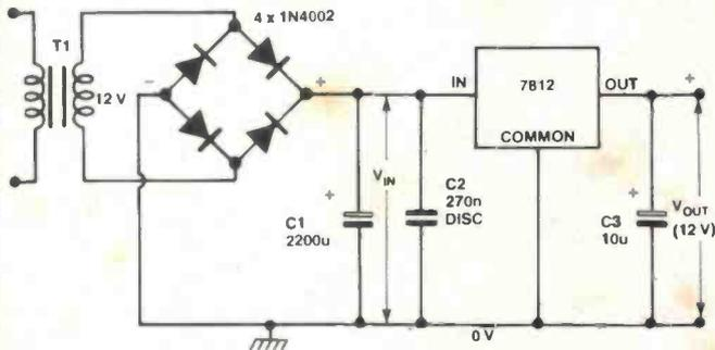
Figure 11. Circuit employing a common three-terminal positive regulator.
