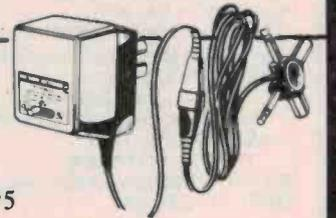
240V AC input and the choice of 3, 6 or 9V DC output. The current rating is 200mA which is more than enough for many applications. 4-way connector to suit most uses and reverse polarity.
