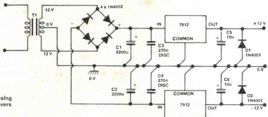
Three-terminal regulators are remarkably easy to use, as shown in the basic circuits of Figures 11 to 13, which show the connections for making positive, negative and dual regulator circuits respectively. The ICs shown in these examples are 12 volt units with current ratings of 1 A, but the basic circuits are valid for all other voltage ratings, provided that the unregulated input voltage is at least three volts greater than the desired output voltage.
