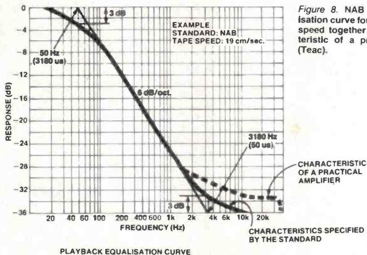
Figure 8. NAB playback equalisation curve for a 19.5 cm/s tape speed together with the characteristic of a practical amplifier (Teac).
