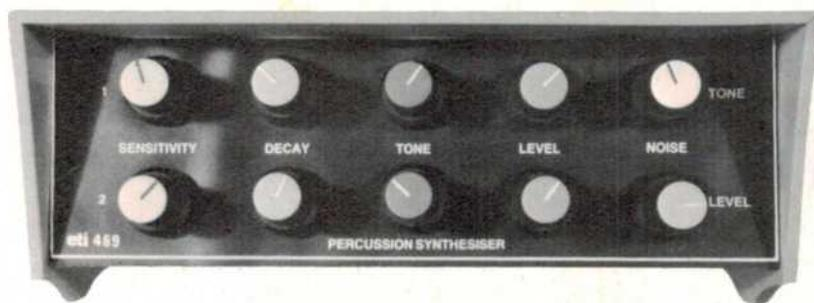
We housed our project in a light but sturdy ABS plastic case and attached a Scotchcal label to the front panel — artwork for this panel is reproduced on page 126. The two 'transducer' inputs, the output and supply input are located on the rear panel. Small speakers serve as input transducers and are mounted in separate small boxes.
