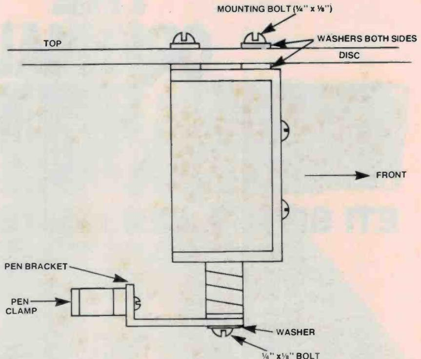
Figure 10. Mounting the pen solenoid.
