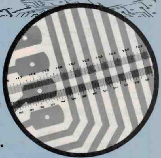
Introducing OPTO-SCALE from Bishop Graphics, the first glass linear measuring instrument to combine precision accuracy, functional design, hi-tech quality and unique performance features in one compact unit...all at an easily affordable price. With OPTO-SCALE there's no need for guesswork. The 610mm (24") precision scale pattern gives you overall accuracy to ±0.013mm (.0005"), with an incredible ±0.005mm (.0002") between adjacent lines.
