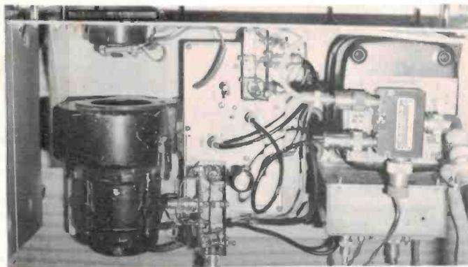
Inside the 1296 MHz transverter; transistomixer and amplifier in the centre, receiving converter at lower left.
