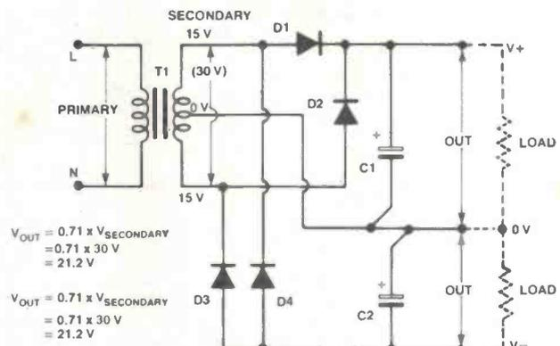
Figure 4. Basic dual supply using individual diodes.
