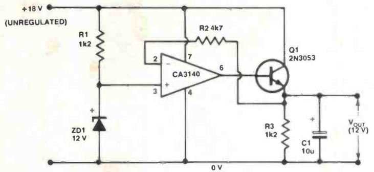
Figure 10. Op-amp based reg. provides 12 V at up to 100 mA with excellent regulation.
