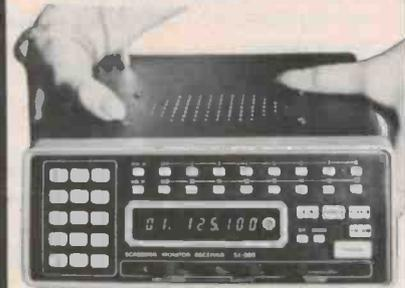
Monitors over 33,000 frequencies from 26 to 88 MHz, 108 to 180 MHz and 380 to 514 MHz. Bands included within this range are HF and UHF CB, 27 and 155 MHz MARINE, Australian LOW BAND, AIRCRAFT band, VHF SATELLITE band, 10 Mx, 6 Mx, 2 Mx and 70CMx AMATEUR BANDS, VHF High BAND as well as UHF two-way band.
