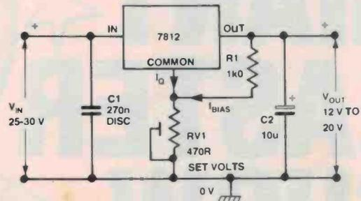
Figure 15. Improved method of varying output voltage.
