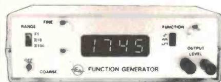
EA's new Function Generator covers the frequency range from 15Hz to 170kHz in three ranges with coarse and fine frequency controls. An economical 4-digit display has been incorporated to eliminate dial calibration. Sine wave distortion can be trimmed to around 0.5%. See EA April, 1982
