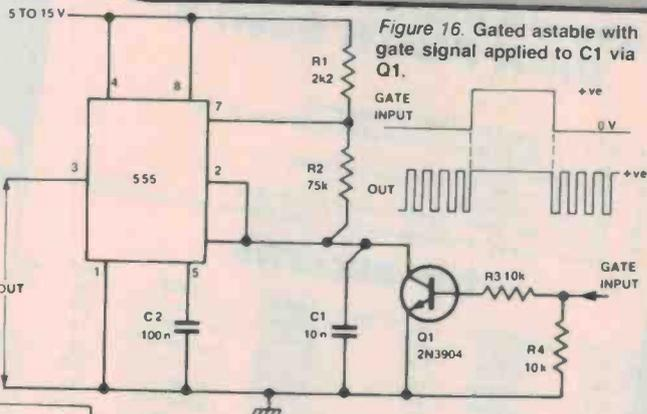
Figure 16. Gated astable with gate signal applied to C1 via Q1.
