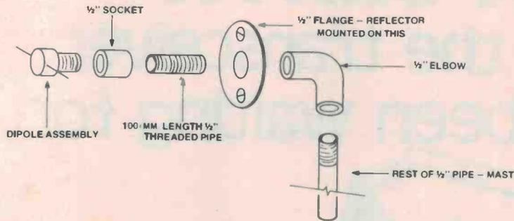
Figure 3. How the antenna support structure is made.
