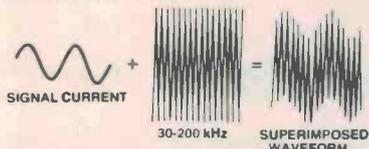
Figure 18. The addition of HF bias to the signal produces a composite wave (Teac).
