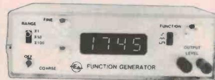
EA's new Function Generator covers the frequency range from 15Hz to 170kHz in three ranges with coarse and fine frequency controls. An economical 4-digit display has been incorporated to eliminate dial calibration. Sine wave distortion can be trimmed to around 0.5%.
