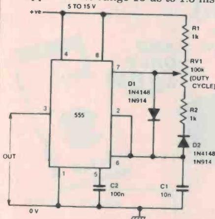
Figure 13. Astable with mark and space periods independently variable over about 15 us to 1.5 ms. Here, timing capacitor C1 alternately charges via R1-RV1-D1 and discharges via RV2-R2-D2.
