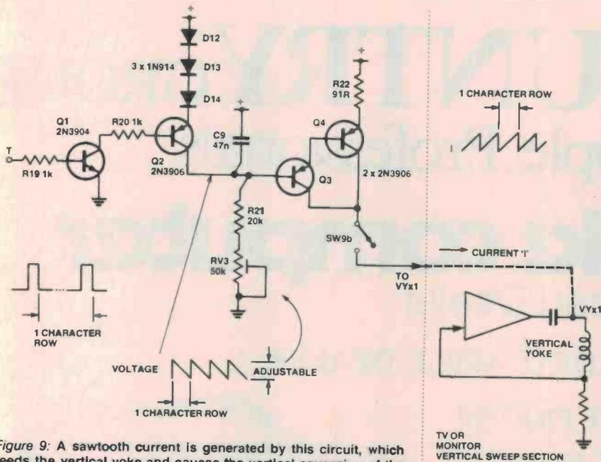
Figure 9: A sawtooth current is generated by this circuit, which feeds the vertical yoke and causes the vertical squeezing of the scan lines belonging to one character row.
