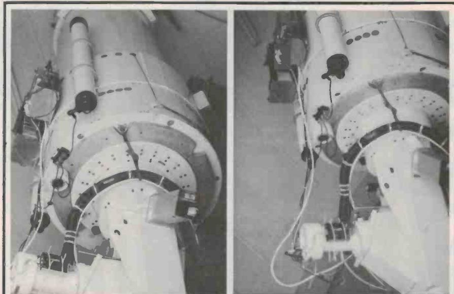
The Cassegrain Echelle Spectrograph and the 2D PCA on the 40-inch telescope at Siding Spring Observatory
