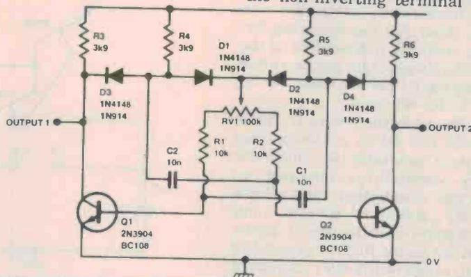
Figure 5b. Improved version of variable M/S ratio astable with waveform correction and sure-start facility.
