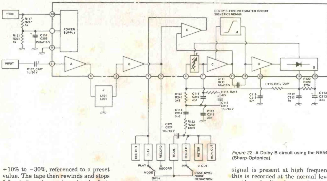
Figure 22. A Dolby B circuit using the NE546B IC (Sharp-Optonica).
