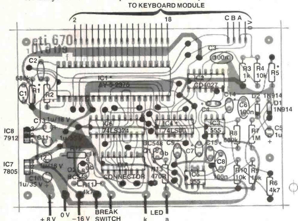
Printed circuit board component overlay. NOTE: ● — by itself means a feedthrough link; on a component lead it means solder the lead both sides of the board.
