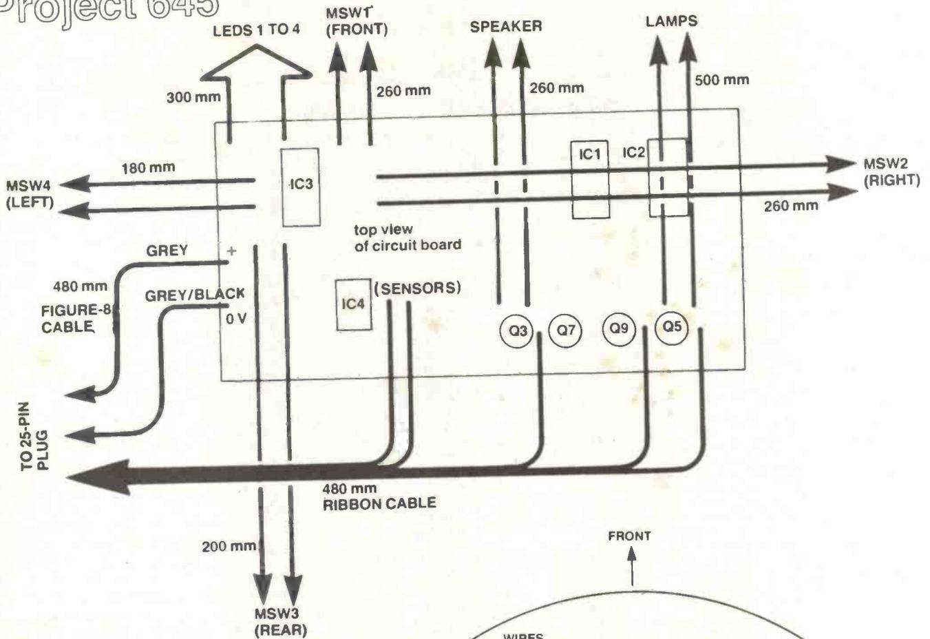
Figure 13. Lengths to cut the cables that run from the control board. Note that this drawing is only diagrammatic and does not indicate the actual termination points or dressage of each cable. The overlay, Figure 11, shows termination points, Figure 14 and 15 show dressage.
