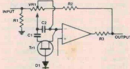
Figure 10. Part of the equalisation circuit of the Teac 35-2B recorder.
