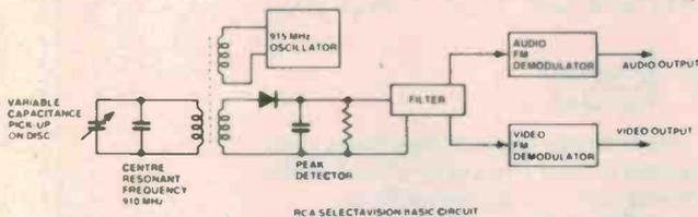
As the disc rotates, the information stored on it produces capacitance variations in a special capacitance pickup system, which is incorporated in the type of circuit shown. The pickup and its associated components resonate at a centre frequency of 910 MHz. Both the video and the audio information are picked up in this circuit.
