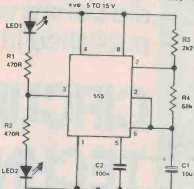
Figure 12. This two-LED flasher operates at just under 1 Hz. The LEDs flash alternately.
