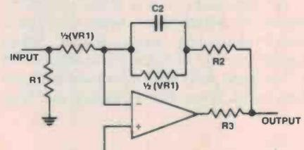
Figure 12. Equivalent circuit of Figure 10 when VR1 slider is on the right (Teac).
