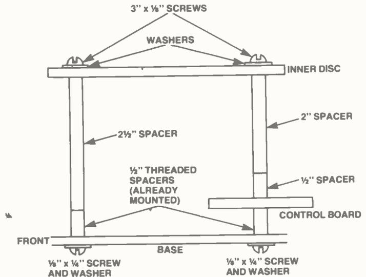
Figure 20. Assembling the inner disc and control board to the Turtle base.
