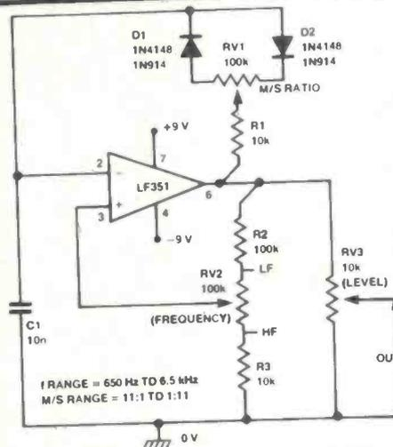
Figure 9. Variable frequency, variable M/S ratio generator.
