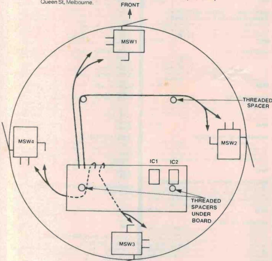
Figure 15. Routing the wires to the sensor microswitches.
