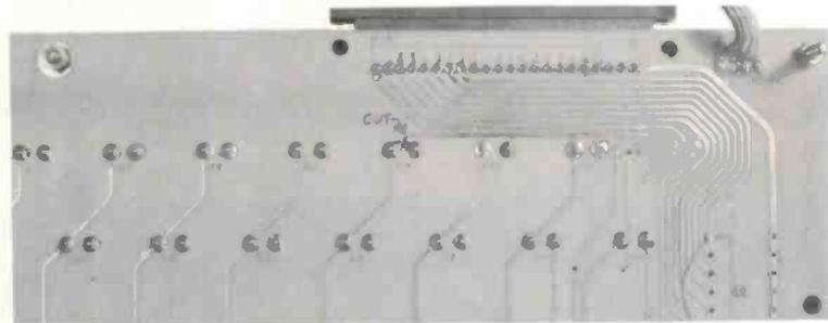
Figure 3. Modifications required to the rear of the keyboard pc board.
