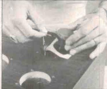
▲ Mount tweeter and mid range speakers. Connect the faders, seat them and screw into position. Note the use of a gasket (above) for prevention of air leaks.
