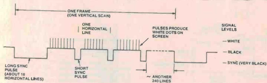
Figure 1: Simplified diagram of the composite video signal.
