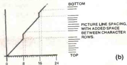
Figure 4b: Graph shows the effect of adding a step of current after each character row. Note the spaces in the scan lines.
