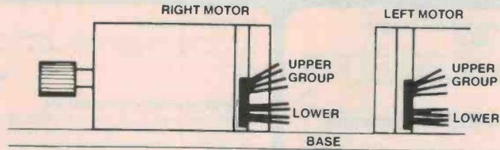
Figure 17. Identifying the groups of motor wires.
