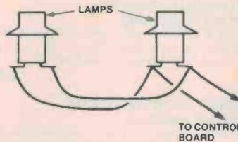
Figure 16. Wire the two lamps in parallel.
