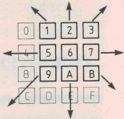
The 'standard' '660 keyboard showing the functions of each key. The heavy arrows indicate which way the cursor moves when you press that key. One press moves the cursor one pixel position.
