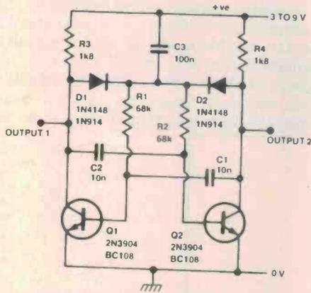
Figure 4. The 1 kHz astable with 'sure-start' facility.
