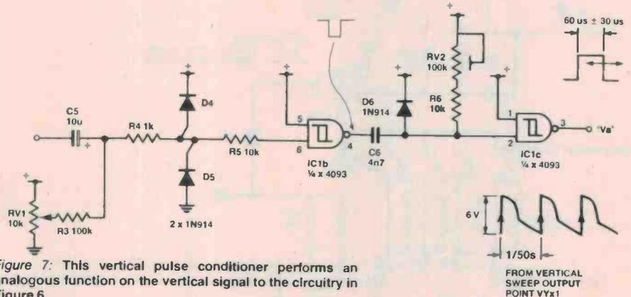
Figure 7: This vertical pulse conditioner performs an analogous function on the vertical signal to the circuitry in Figure 6.
