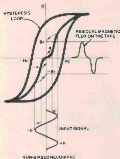
Figure 17. Recording without bias produces severe distortion (Teac).
