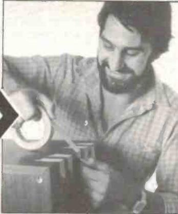
Assemble the cabinet and insert the crossovers as per instruction supplied. Bind the final join with masking tape to give strength while the join sets.
