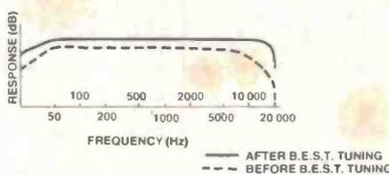
Figure 21. Improvement claimed by setting the parameters using JVC's B.E.S.T. system.
