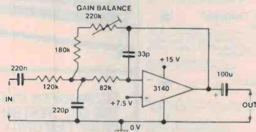
Figure 23. Adjustable-gain second-order low-pass output filter.
