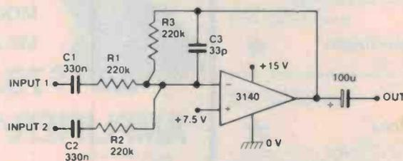
Figure 24. Combined two-input mixer/first-order low-pass filter.
