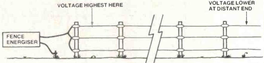
**Indications.** An electric fence doesn't deliver the same 'punch' over its entire length. This diagram shows you what to expect.
