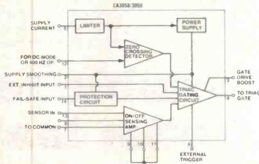
1. Limiter-Power Supply — permits operation directly from an ac line.
