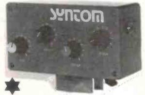
Original design from the UK magazine "Electronics and Music Maker" April 1981. Self-contained unit produces a variety of fixed and falling pitch effects. Trigger by tapping the unit itself or by striking a drum to which the unit is attached. The Jaycar "SYNTOM" comes complete with high quality pre-drilled moulded die ABS box 152 x 80 x 47mm with professional silk-screened front panel.
