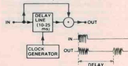
Figure 5. Double-tracking circuit.
