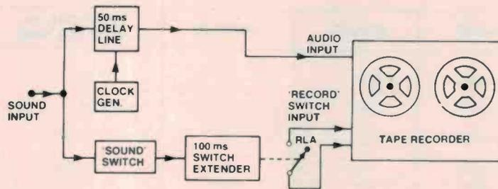
Figure 14. Automatic tape recorder with 'predictive' switching.
