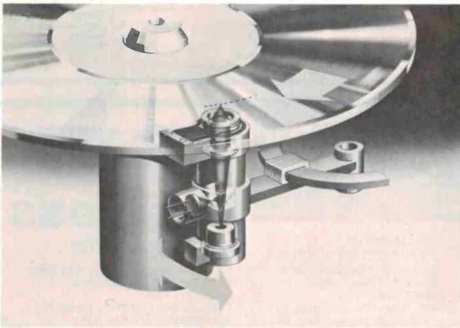
**Light reading.** Laser light is focussed into the disc's bright, reflective surface where it reads the microscopic pits as either a high reflected light level or a very low level since light is scattered in the pits. These signals are converted into electronic digits by the illustrated photodiode. Note the tracking arm, which moves from the inside to the outside with a progressive speed change from 500 to 200 revolutions/minute.
