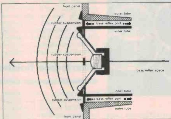
reflex port providing symmetrical loading of the bass diaphragm and lowering distortion, claim the Jamo manufacturers.
