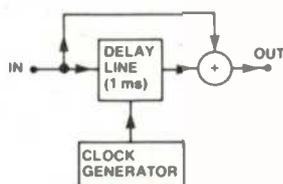
Figure 8. CCD comb filter. Notches are about 20-30 dB deep, 1 kHz apart.
