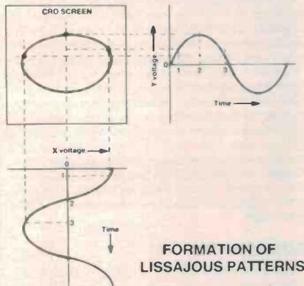
The two frequency sources must be stable or the pattern will roll around at a rate determined by the varying difference between the two sources.
