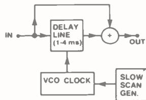
Figure 9. A phaser is a variable comb filter in which the notches are slowly swept up and down the audio band.
