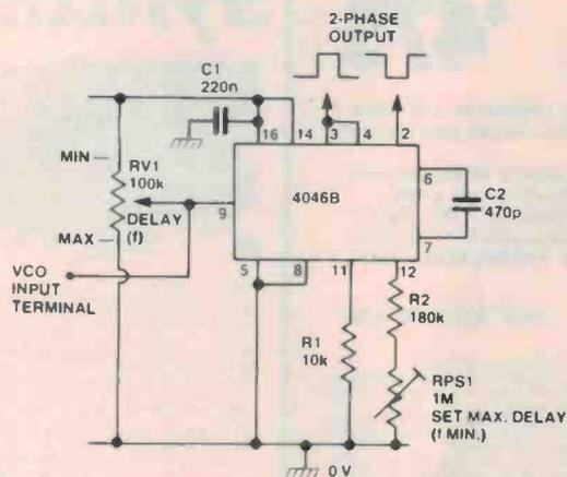
Figure 20. High-performance voltage-controlled two-phase CMOS clock generator.
