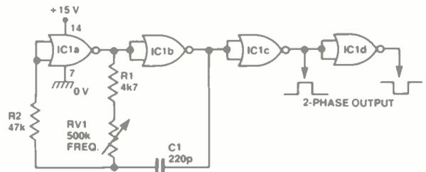
Figure 19. Variable-frequency general-purpose two-phase CMOS clock generator.
