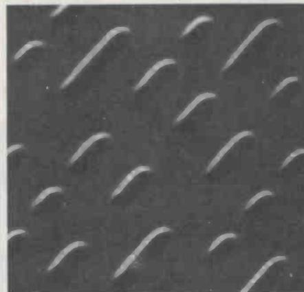
It's the pits! Compact disc pit structure, magnified 12 500 times. The pits are about 0.5  $\mu\text{m}$  wide and from 0.833  $\mu\text{m}$  to 3.56  $\mu\text{m}$  long. Tracks are 1.6  $\mu\text{m}$  apart.
