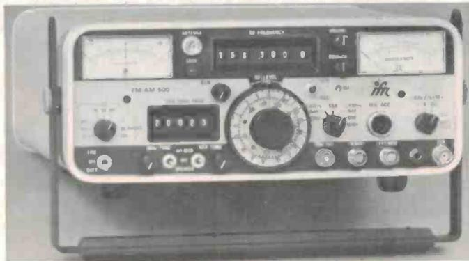
generator output is variable from 0 to 2.5 V RMS into a 150 ohm load.
