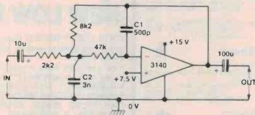
Figure 22. 25 kHz second-order maximally-flat low-pass filter.
