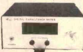
Here is an inexpensive Digital Capacitance Meter which measures from 1pF to 99.99uF in just three ranges. It's simple to use and features a big bright four-digit display with automatic updating and decimal points. EA March 80
