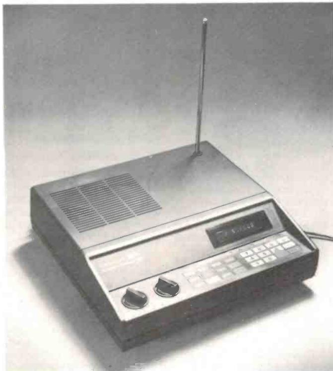
Available through Dick Smith stores, this latest Bearcat features a 16-channel memory (with battery back-up), auto or manual search over three bands (66-88 MHz, 138-174 MHz, 407-512 MHz), direct channel access, automatic channel lockout and priority functions plus patented selective scan delay so you don't miss the reply on two-way conversations.
