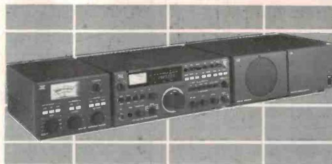
circuit of narrow BPF type; large multi-function display; remote control of frequencies and modes; overmodulation indication; unique ALC input; frequency data output.
