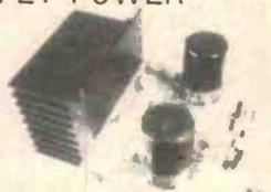
A general purpose 150W Mosfet Power Amp Module. Here's a high power, general purpose Power Amplifier Module for guitar and PA applications employing rugged, reliable Mosfets in the output. ETI 499 March 82
