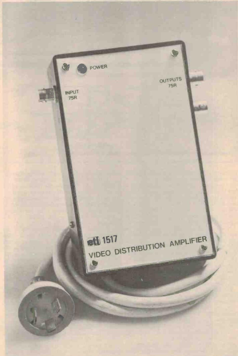
▶ Wrapped up, ready to go. The project and its power supply fit neatly in a large zippy box, leaving enough room to add a video enhancer later.
