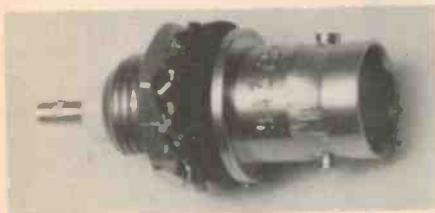
Start with the BNC socket. This has to be installed from the front panel. What I did was to take a 6 mm i.d. rubber grommet and force (roll) it onto the socket's thread after removing the nut, washer and earth lug. This then slips neatly in the 11 mm mounting hole marked FUNCTION. Secure it by putting the washer on first, then the earth lug, followed by the nut. Check that it isn't shorted to the chassis. Then mount the power
