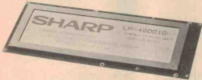
The LM-48001G features 237 x 70.5 mm wide viewing area and 480 x 128 full dots, making it possible to display 16 lines of 80 characters each. It can also display graphics, pattern,
