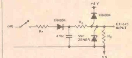
To drive an input direct from a logic gate output, no special interface is required.
