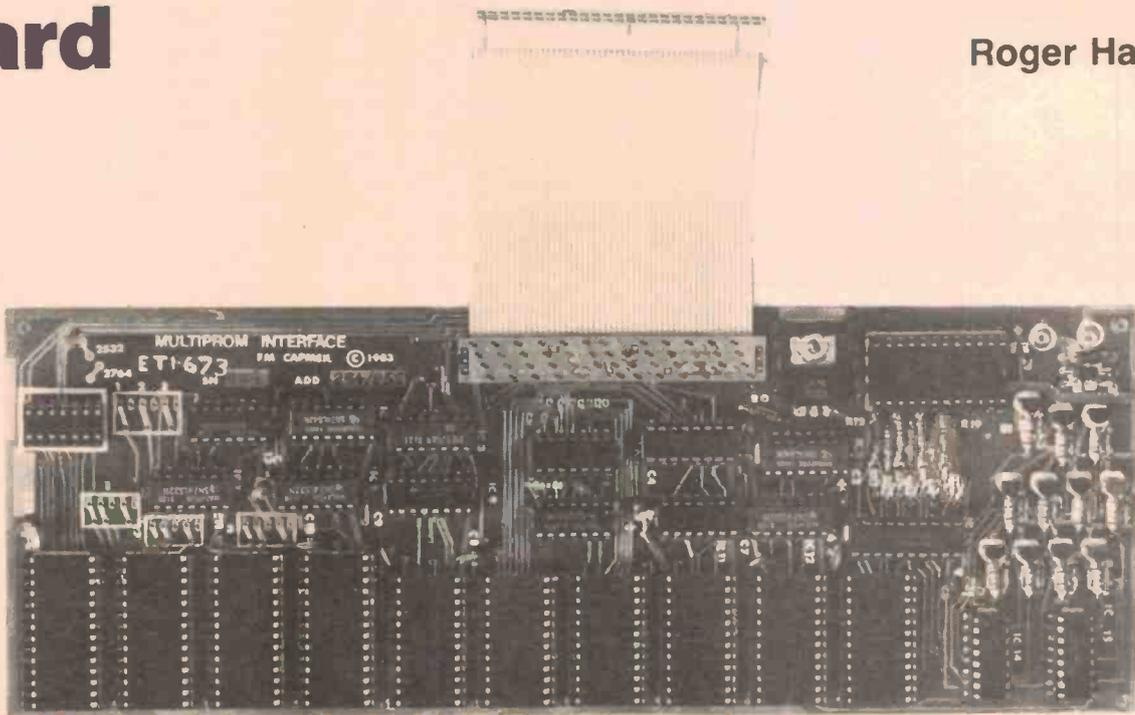
This project design by F. M. Capmeil, presented with the cooperation of Avtek Electronics, permits extending the ROM capacity of the Microbee to 44K, or to 308K total by daisy-chaining up to six slave boards to produce a sort-of high speed 'read-only virtual disk' (a ROD?). It takes 2532s or 2764s (can be mixed) and, in addition, provides 11 open-collector outputs and eight buffered inputs.
