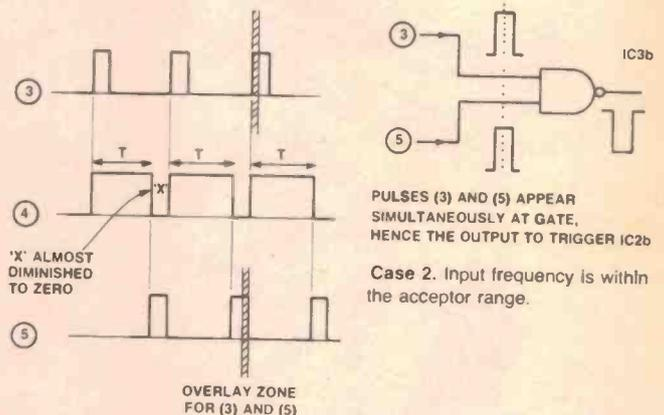
PULSES (3) AND (5) APPEAR SIMULTANEOUSLY AT GATE, HENCE THE OUTPUT TO TRIGGER IC2b
