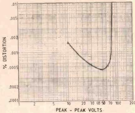
Perreaux SM2 preamplifier. IEC high frequency total difference frequency distortion.
