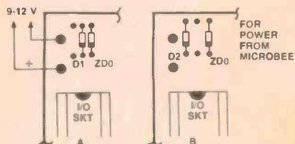
**Internal/external supply.** Connections for using an external power supply (A); (B) shows arrangement for obtaining power from the Microbee.
