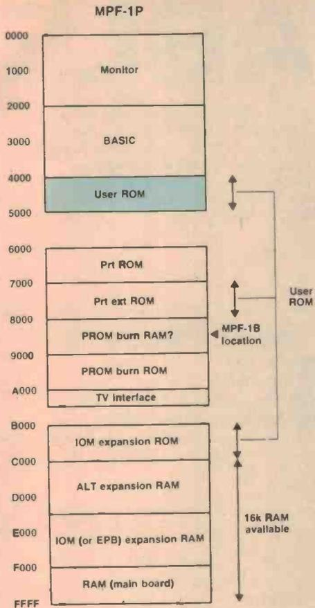
This area of ROM occupies U4 which alternatively can contain RAM at F000-F7FF. (This is usually the less desirable choice)
