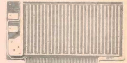
**S-100 WIRE WRAP CARD.** Gold-plated edge connectors, through hole plating, provisions for four regulators, distributed power rails, I/O connector provision on top of card.
