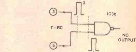
Case 1. Input frequency is below the acceptor frequency.
