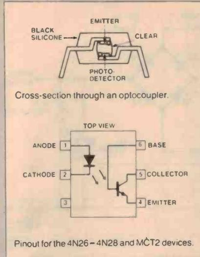
devices are spectrally well matched so that a small emitter device current can produce a reasonably large response in the detecting device.
