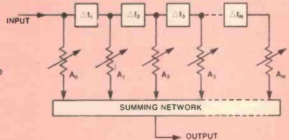
Figure 3. A transversal filter. In the SAW realisation the tap amplitudes  $A_0$ - $A_N$  are set by the length of the IDT fingers and the time delay between taps is controlled by the relative positions of the fingers.
