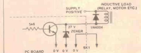
The maximum supply voltage the BC548s will stand is 30 V, so any supply should be kept below 90% of this value (i.e. below 27 V). A 27 V zener is used to protect each output transistor. note that any external supply used to power the device being switched should have its 0 V line returned to the MultiPROM's 0 V line.
