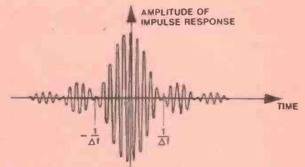
Figure 4. Responses of an ideal bandpass filter. The amplitude and phase responses are 'single-sided' (no negative frequencies) representations and the impulse response is derived by considering a pseudo-impulse (a very short pulse) modulated onto a carrier at the filter centre frequency. The impulse response is infinite in extent in time.
