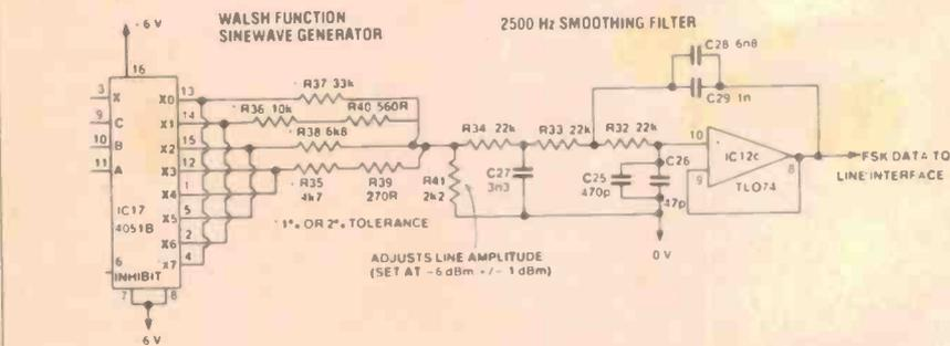
**Set line level.** The transmit line level has been found to be too high in practice at -6 dBm, swamping the reactive channel. Reduce it to -18 dBm or lower by lowering the value of R41. Richard White suggests 270R.
