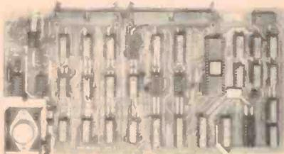
**FDC-II.** Enhanced floppy disk controller, IBM 3740 compatible, operates 5" & 8" and single/d density drives, handles up to 4 drives, runs multi-density CP/M2.2 & MP/M 2. Vectored interrupt operation optional. List Price \$465.
