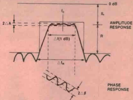
Figure 6. Major parameters of a bandpass filter.
