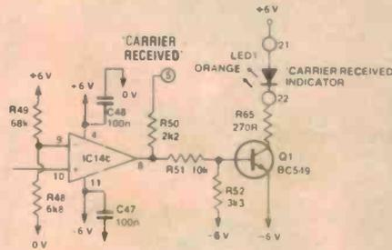
R48 to ground. Here is this portion of the circuit corrected.
