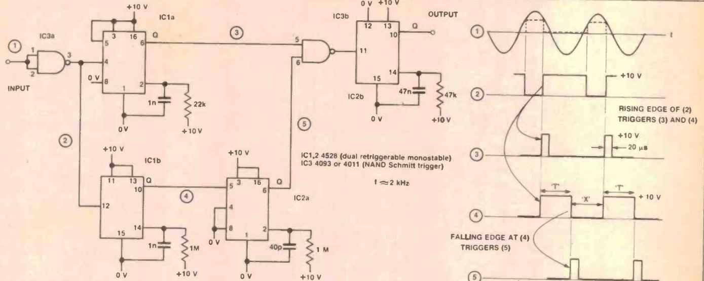
Audio frequency switch. Sine wave input (peak value equal to supply voltage) applied to input will cause output to go high within a certain narrow range of frequency. Response outside this range is zero.
