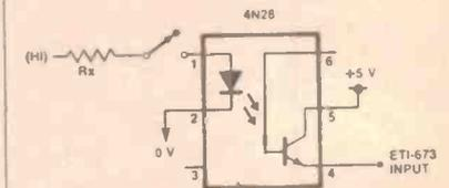
If the input is a pulse or varying dc level signal, then it is necessary to use a signal conditioner. This circuit should do the job:
