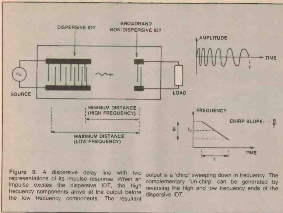
that since  $T/BT = 1/B$ , the compressed pulsewidth or time resolution is of the order of the reciprocal bandwidth.
