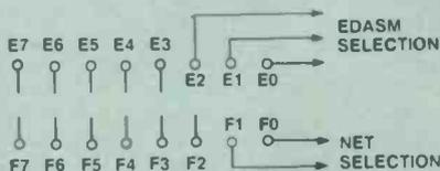
The remaining outputs are used to drive 11 transistors. They are F3 to F7 and E2 to E7. The collectors of the transistors are brought to the input/output socket, SK1.
