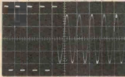
**PMF 1150B power amplifier transient overload recovery test (IHF-A-202).** 10 dB overload re rated power into eight ohms, both channels driven. Overload duration: 20 ms; repetition rate: 512 ms.
