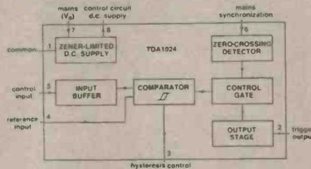
by selection of the resistor value connected between pins 3 and 1. Hysteresis is minimum with pin 3 open, so I have left it open.
