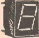
Litronix red single digit displays. Lite pipe construction. Type DL-750 common cathode type. Character height .630". 7 segment D.P. left light output (MCD). 20mA (typ). Forward voltage typ 3.4V Max 4.00
