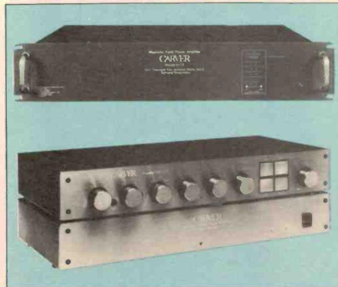
The Carver M-200t power amplifier produces 120 W minimum continuous power per channel into 8 ohms, 20 Hz to 20 kHz with less than 0.05 THD. It weighs 3.6 kg and measures 44 x 23 x 6.5 cm.
