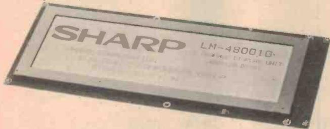
The LM-48001G features 237 x 70.5 mm wide viewing area and 480 x 128 full dots, making it possible to display 16 lines of 80 characters each. It can also display graphics, pattern,
