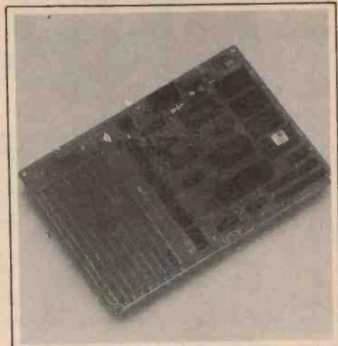
IOM-MPF-1P Input/Output and Memory board. This provides the Counter-Timer chip, the Communication Interface chip and the Parallel I/O chip kits to interface with the outside environment. It provides an extra 6K RAM and 4K ROM.
