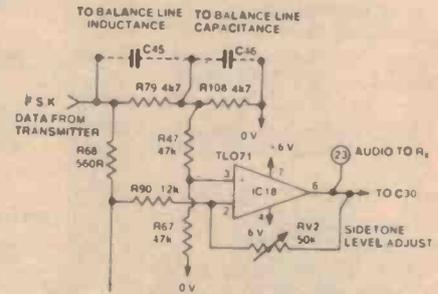
Line balance. Line balance requires fine adjustment. Make RV2 a 10-turn panel-mount pot. if you like. See (4) above.
