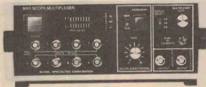
$\pm 5$  V (10 V peak-to-peak) with a frequency response which is flat to 12 MHz and 3dB down at 20 MHz; input impedance is 1M, G.S.C. claim.
