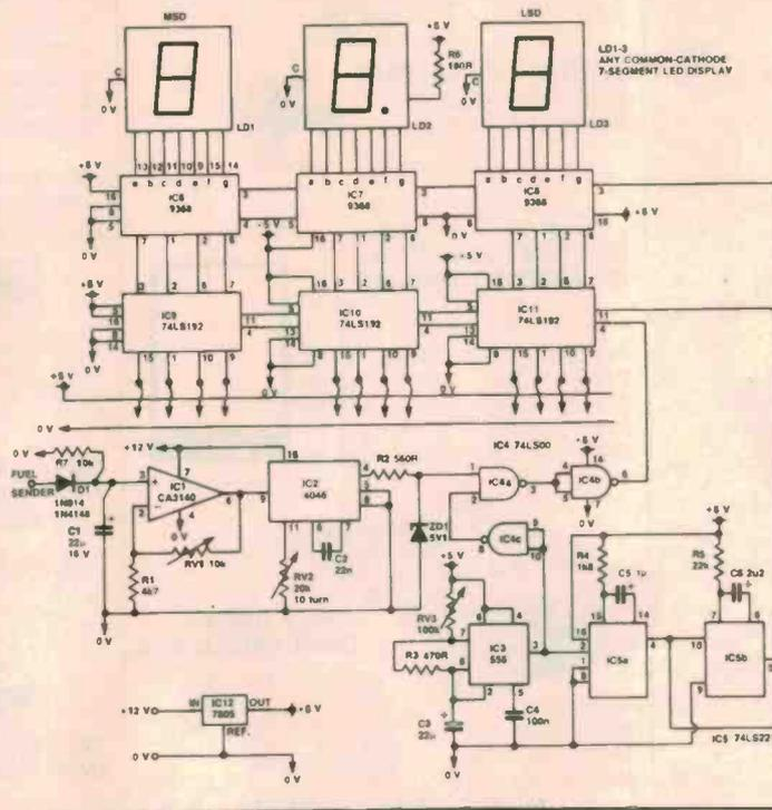
input of the following stage, etc. Note that the output of IC2 is clipped by the action of ZD1 to 5 V to suit the input of IC4.
