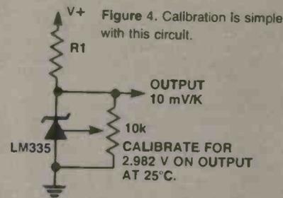
Figure 4. Calibration is simple with this circuit.
