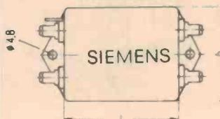
The PROMARK PULSE PRUNER is a high energy metal oxide varistor and a multi-element balanced LC line filter which work together to clip spikes and hold back RF interference. These are a must for computer power inputs — Also great for Hi-Fi's to keep out taxi's, CB's, etc., from your Wagner & Strauss.
