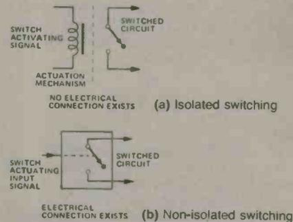
Unlike electromechanical switches, most solid-state electronic switches do not provide ideal isolation between the actuating signal source and the controlled source.
