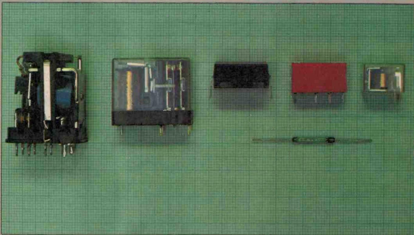
While solid-state switches have now replaced electromechanical relays in many applications and types of service, there are still innumerable areas where the old-fashioned (?) relay still reigns supreme — and is likely to do so for many years to come. This feature covers all the theoretical and practical aspects of relay technology and includes a survey of all forms and types, from the common to the bizarre.
