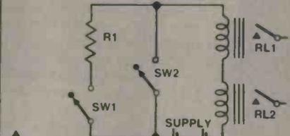
Figure J. Sequential switching. Closing SW1 will energise the sensitive relay RL1 but not the general purpose relay RL2. Switch SW2 shorts out the current limiter R1 and closes RL2.
