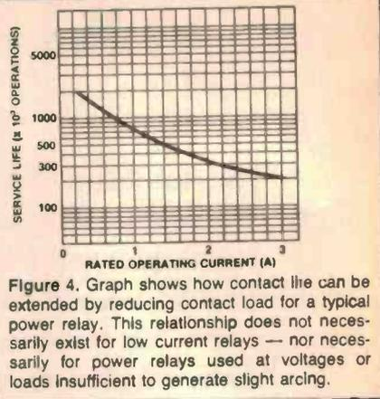
Figure 4. Graph shows how contact life can be extended by reducing contact load for a typical power relay. This relationship does not necessarily exist for low current relays — nor necessarily for power relays used at voltages or loads insufficient to generate slight arcing.
