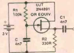
longer forward biased. Once this occurs, capacitor C will again begin to charge up via R1 and so complete one cycle of oscillation.
