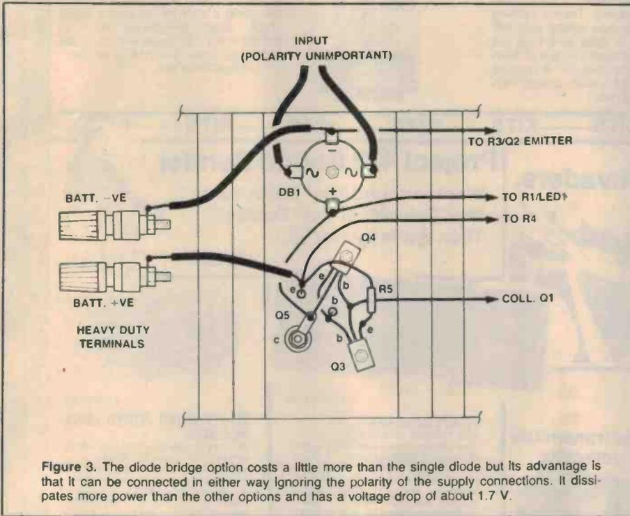
Figure 3. The diode bridge option costs a little more than the single diode but its advantage is that it can be connected in either way ignoring the polarity of the supply connections. It dissipates more power than the other options and has a voltage drop of about 1.7 V.
