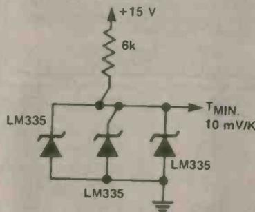
Figure 3. The basic LM332 circuit.
