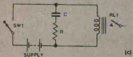
Figure L. Adding a few components slows down relay operating time. (a) slow to operate, (b) and (c) slow to release.
