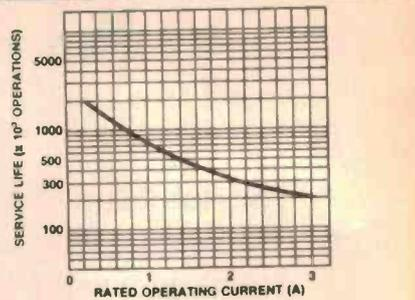
Figure 4. Graph shows how contact life can be extended by reducing contact load for a typical power relay. This relationship does not necessarily exist for low current relays — nor necessarily for power relays used at voltages or loads insufficient to generate slight arcing.
