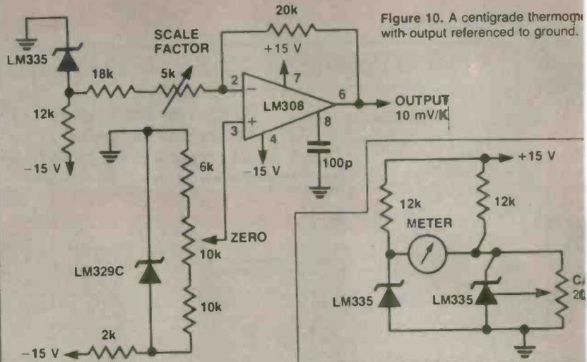
Figure 10. A centigrade thermometer with output referenced to ground.
