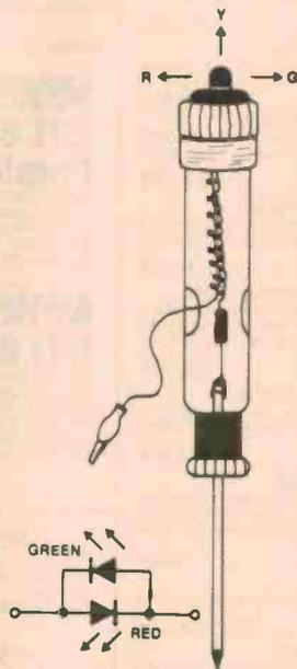
I wanted something rugged, comfortable, safe, attractive and useful. I decided to use an ordinary 240 V neon mains tester/screwdriver as the carrier/probe for the tester. Ellistronics has one which has an amber body and plastic sheaf along the screwdriver shaft, topped with a neat red plastic cap and contact.
