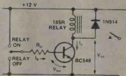
Figure M. Reducing triggering currents by adding transistor or IC amplifier. (a) single transistor. (b) higher amplification using two transistors. (c) simple operational amplifier.
