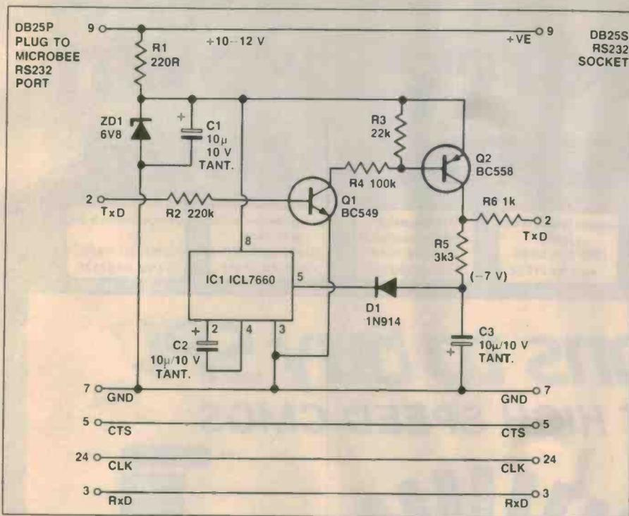
Mount the resistors, capacitors and semi-conductors first, taking care to correctly orientate the semiconductors and tantalum capacitors. Mount the DB25 plug and socket last — making sure you get each at the correct end of the board. The plug goes at the Microbee end, the socket at the output end. When mounting these, bolt them to the board before soldering the pins so that no stress is placed on the soldered joints.
