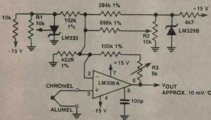
fed to the inverting input of the LM308, the output of this operational amplifier falls.
