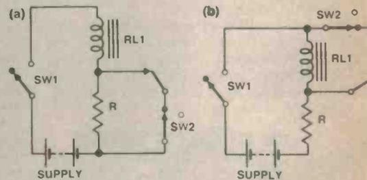
▲ Figure D. These two configurations are commonly used safeguarding electrically powered machinery. In neither instance can relay RL1 be energised, by closing SW1, unless SW2 is open.
