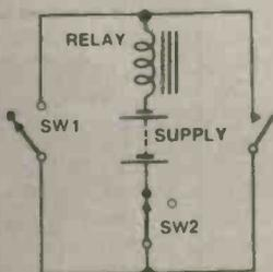
▲ Figure C. Electromagnetic latching circuit. When SW1 is closed a second set of relay contacts close, by-passing SW1. The relay will now remain latched on until power is removed (by opening SW2).
