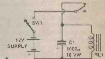
▲ Figure E. Ultra-reliable low frequency oscillator/flasher.
