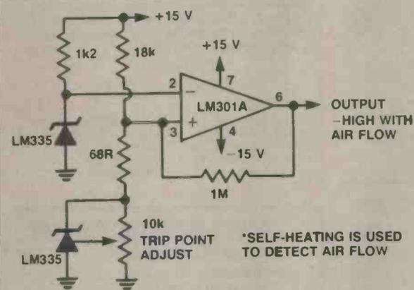
Figure 12. A differential temperature sensor with amplifier gain of ten.
