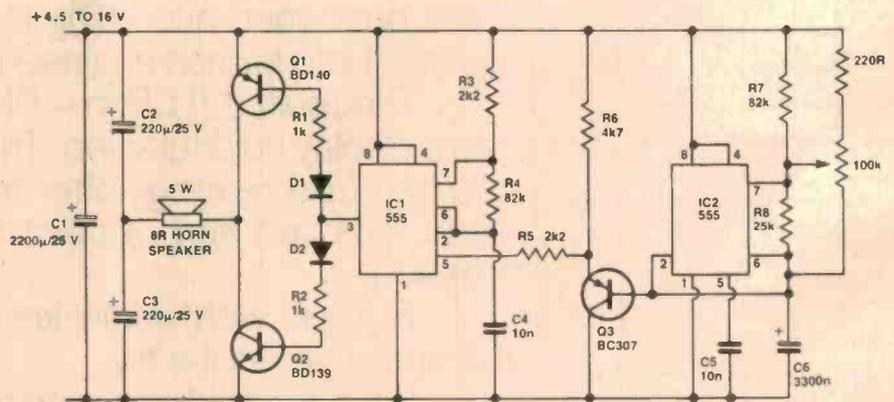
470  $\mu$ F capacitors for C2 and C3.
