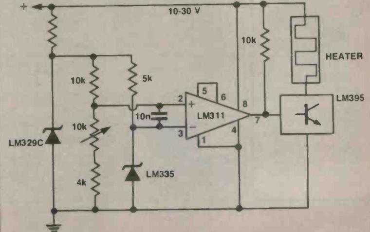
Figure 13. A thermostatic heater controller.
