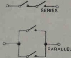
**Series.** You can connect contacts in series to reduce the effects of arcing and to improve voltage rating; however, contact/contact resistance increases and may affect current rating.
