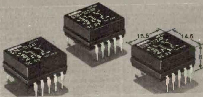
Many designers specify unnecessarily complex and sometimes inherently unreliable solid-state componentry to interface their logic or other circuitry to drive medium to high current loads. Yet printed circuit board mounting relays may be driven directly from TTL and CMOS logic gates, or buffers or drivers. The necessary bits and pieces have been available for at least a decade!
