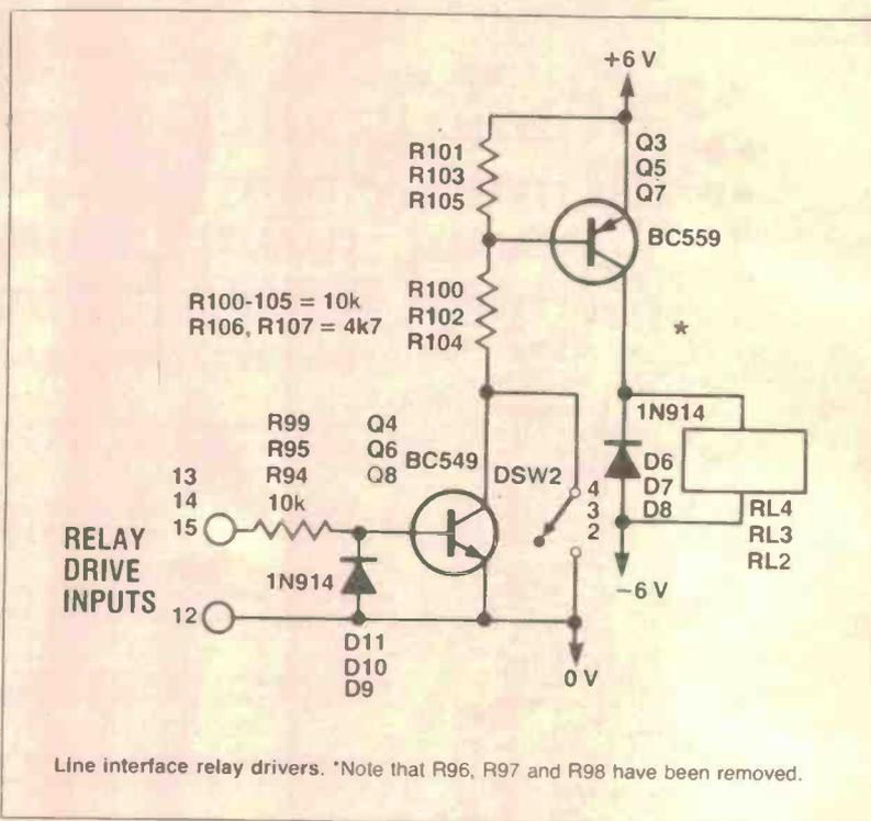
Line interface relay drivers. \*Note that R96, R97 and R98 have been removed.
