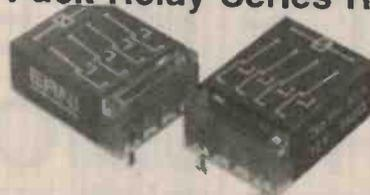
An electromagnetic relay with two or four bifurcated contacts, it provides excellent results, both in dry load switching (gold) or high load switching of up to 4 Amp (Ag Cdo).
