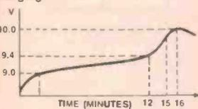
Figure 2. Voltage/time curve charging 6x1.0 Ah NiCd cells at 4 A.
