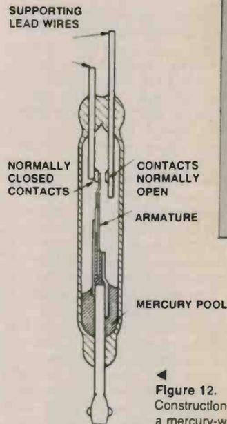
◀ Figure 12. Construction of a mercury-wetted relay.
