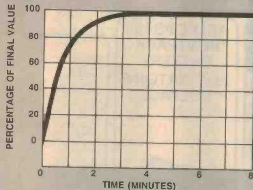
Figure 5. Response time of the LM335 to a temperature change in free air.
