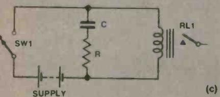
Figure L. Adding a few components slows down relay operating time. (a) slow to operate, (b) and (c) slow to release.
