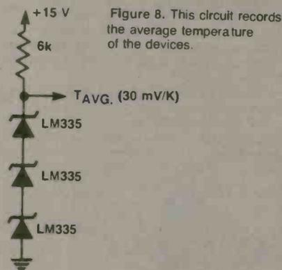
Figure 8. This circuit records the average temperature of the devices.
