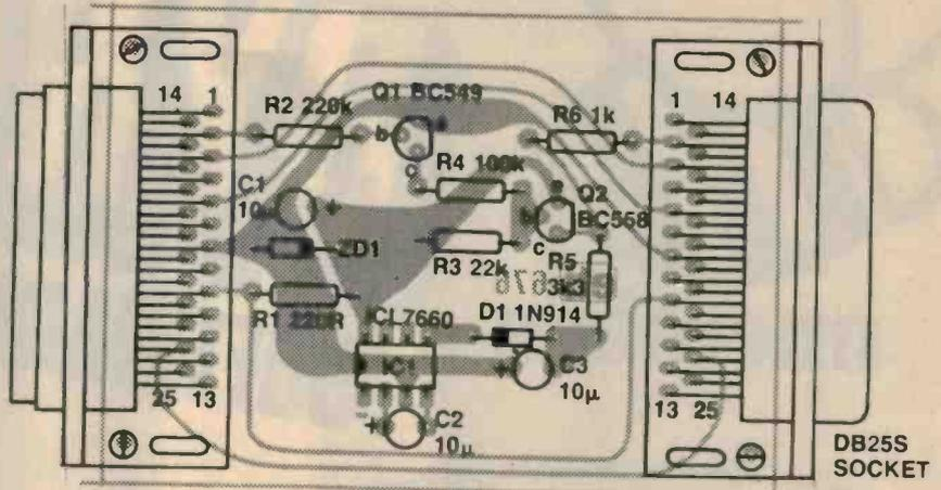
you're assembling the project this way. Note that two links are required, but these should be soldered in later. An IC socket may be used for IC1 but note that pins 1, 6 and 7 *do not* make connection to the copper strips of the Veroboard. If you're using a socket, snip off or remove pins 1, 6 and 7, otherwise cut off the pins from the IC.
