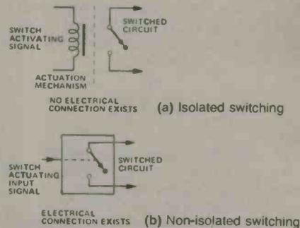
Unlike electromechanical switches, most solid-state electronic switches do not provide ideal isolation between the actuating signal source and the controlled source.
