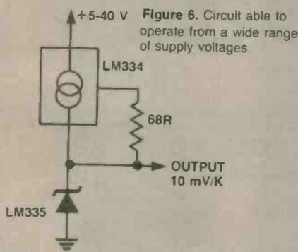
Figure 6. Circuit able to operate from a wide range of supply voltages.
