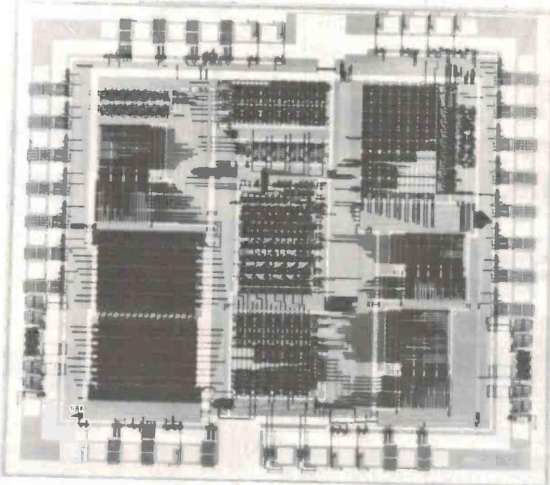
**Their first.** First VLSI chip to be designed by Silicon Compilers was this 8001 Ethernet data-link controller, designed for Seeq Technologies. Although design work began two years after Intel had started on their controller, Seeq was able to begin selling finished chips after only eight months — one year ahead of Intel
