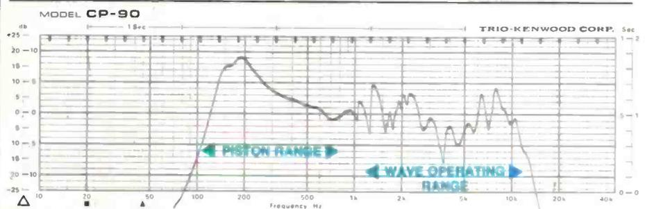
**Pistons and waves.** Typical response of a low frequency drive unit, showing the piston operating region and the wave operating region.
