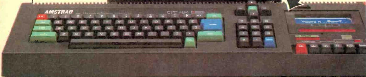
It's mouthwatering. 64K of RAM, 32K of ROM, a high resolution greenscreen VDU, integral cassette data recorder, typewriter style keyboard, numeric keypad and a very fast extended BASIC.
