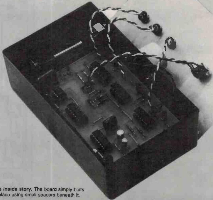
The inside story. The board simply bolts in place using small spacers beneath it.
