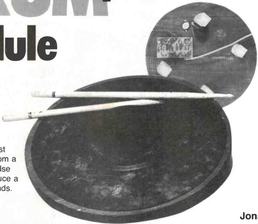
This simple, low-cost module operates from a sound pickup or pulse input and can produce a wide variety of sounds.
