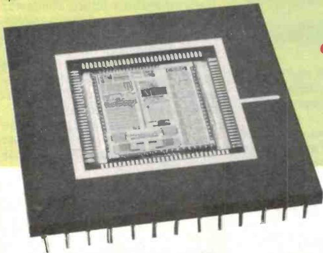
The 102 000-transistor chip, designed and constructed as a design exercise, is a voice recognition device.
