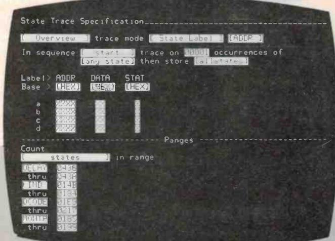
Figure 4. Trace specification for tracing state activity of monitor, decode and display modules.
