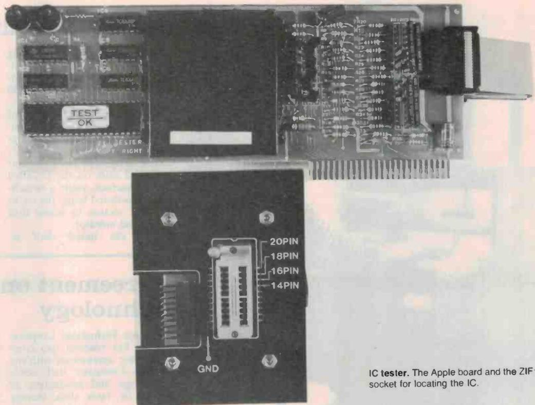
IC tester. The Apple board and the ZIF socket for locating the IC.
