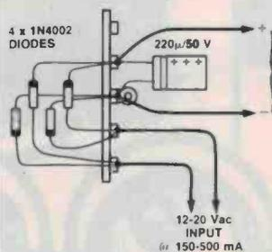
**Power supply.** Suggested construction details for a power supply. The ac input may be from a plugpack or ordinary transformer.
