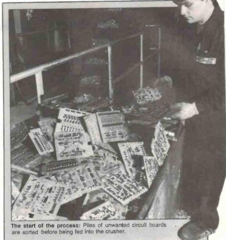
The start of the process: Piles of unwanted circuit boards are sorted before being fed into the crusher.
