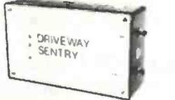
Activated by your car's headlights, the "Driveway Sentry" will turn on a driveway or garage light so that you can make a safe exit from your car on the darkest of nights. At the end of 5 minutes, it will automatically turn the light off again. (EA Dec. '82).
