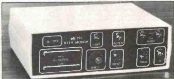
Hey, good lookin'! The ETI lab (thanks to Geoff Nicholls) housed the project in a good looking plastic case. The inputs and outputs are all on the rear. Note the bargraph tuning indicators. The RFE Indicator shows when corrupt copy is being received.
