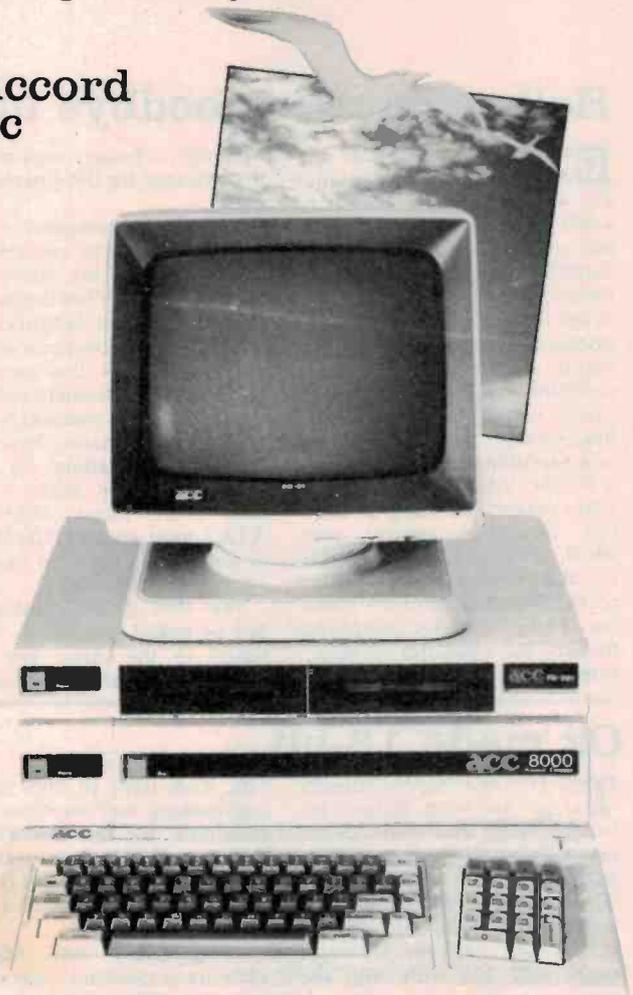
**T**he Accord ACC-8000 computer is a newcomer to the Australian market. It is a Z80-based computer that runs under the improved CP/M operating system (CP/M 3.0). This optimises the use of the machine's 128K memory, and its 'hashed' directory structures speed up the loading of programs and data. The optional hard disk (10, 20 and 40 M) is also a networking node which allows an ACC-8000 to become a file server and print spooler for up to 255 other computers.
