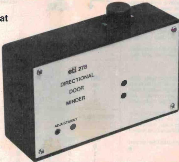
Most electronic door minders function by having a beam of light shining across a doorway interrupted, but are incapable of detecting whether the light beam is broken by a person entering or leaving the room. This project overcomes that problem with the aid of digital logic.
