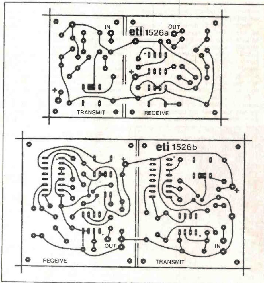
LED which, in turn, depends on the length of optic cable between transmitter and receiver. The values shown in the circuit diagram allow between five and 25 metres of cable to be used with a six volt supply.
