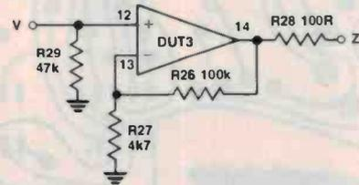
Circuit diagrams of the test sockets. Note that only one op-amp package can be tested at a time.
