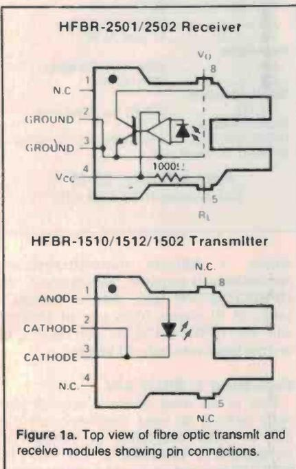
Figure 1a. Top view of fibre optic transmit and receive modules showing pin connections.
