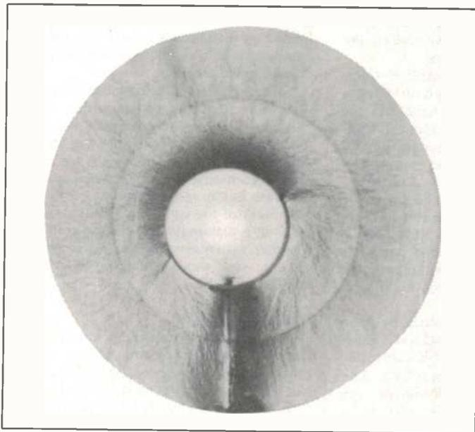
A cross section of multimode, graded index optical fibre with silicon resin coating. Coating outside diameter 380  $\mu\text{m}$ , fibre 125  $\mu\text{m}$ , core 50  $\mu\text{m}$ . (Courtesy of AWA, Optical Fibre Division.)
