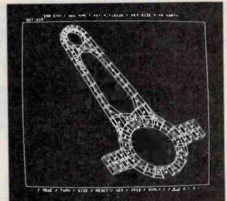
A typical CAD 'wire' drawing. Courtesy AUSTCAD.
