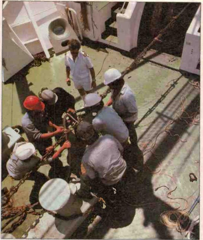
Above. Securing an end of cable even more firmly once on board. The cable can then be pulled inside the ship for testing or repairs. Below. The cable is hauled across the deck then over large drums to be fed into a series of hydraulic wheels and out to the working area.
