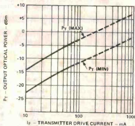
Figure 4c. Typical optical power v transmitter  $I_F$  (0-70°C).
