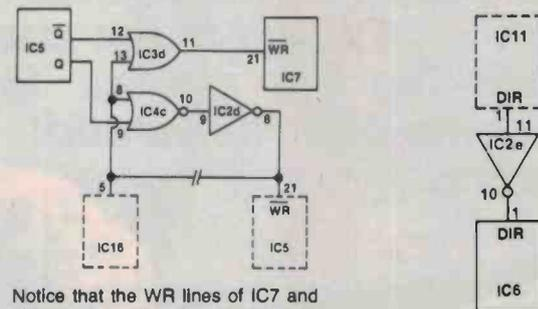
Notice that the WR lines of IC7 and IC5 should not be joined, but should be connected as shown.
