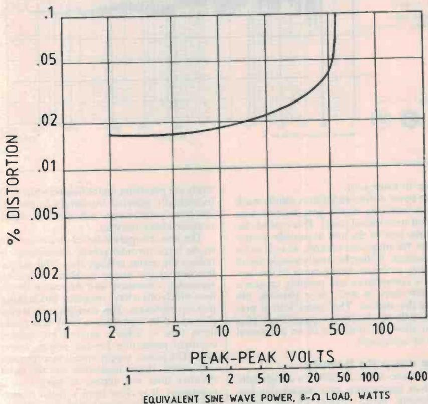
IEC high frequency total different frequency distortion QED model A230 stereo amplifier.
