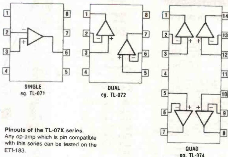
Pinouts of the TL-07X series. Any op-amp which is pin compatible with this series can be tested on the ETI-183.
