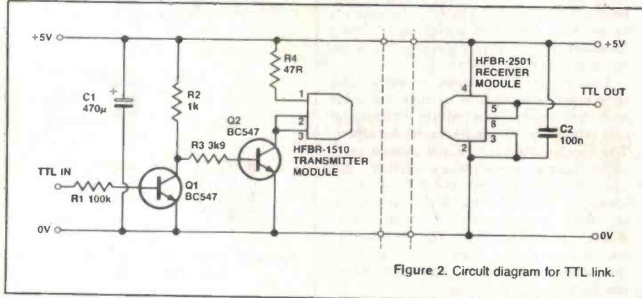
Figure 2. Circuit diagram for TTL link.
