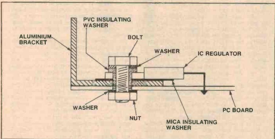
Figure 1. When mounting the IC regulators to the heatsink bracket, make sure the tabs on the regulators are electrically insulated from one another. This is done by placing a PVC insulating washer around the bolt and a mica insulating washer between the IC and the bracket.
