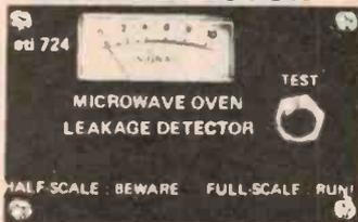
Completely passive project receives microwaves via an antenna which develops a voltage across a detector diode driving the meter. Monitor your microwave oven with this easy to build kit. All components mount on single PCB. Including the meter
