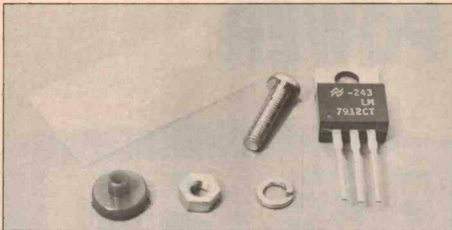
Above: IC mounting hardware. This pic shows the various bits and pieces you will need to mount each regulator. The mica washer is at the top left, and the insulating washer is at the bottom left. Below: The regulators mounted on the heatsink bracket. The 'messy white stuff' all over the bracket is the thermal grease used to provide good heat transfer.
