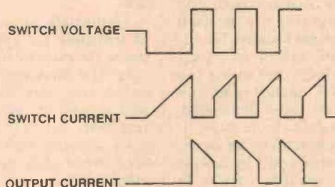
Figure 2. Circuit waveforms.
