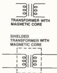
Figure 5. Transformer circuit symbols.
