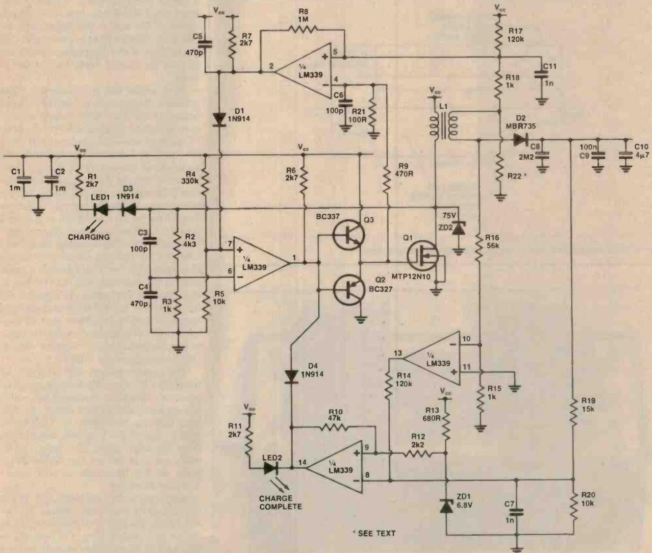
layout exactly as it is. For example, the reference 'ground' for both inputs for pins 4 and 5 of the comparator are next to each other (ie the ground ends of R21 and R22). This is because there is only a small voltage drop to be sensed across R22 and the high currents through the inverter can easily generate voltage drops along earth tracks that will swamp it. Probably the safest way is to buy a ready-made board or get the ETI artwork already checked.
