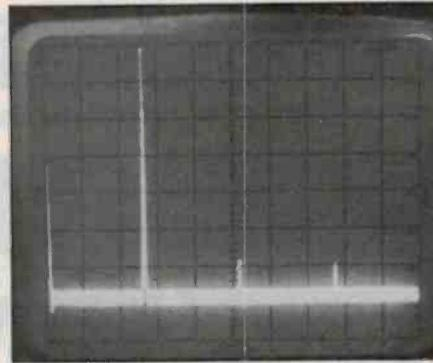
Spectral display at 52 Hz showing harmonics at 104 MHz and 156 MHz at approximately 73 dB<sub>c</sub>. Fundamental reduced 15 dB. 20 MHz per division frequency span.
