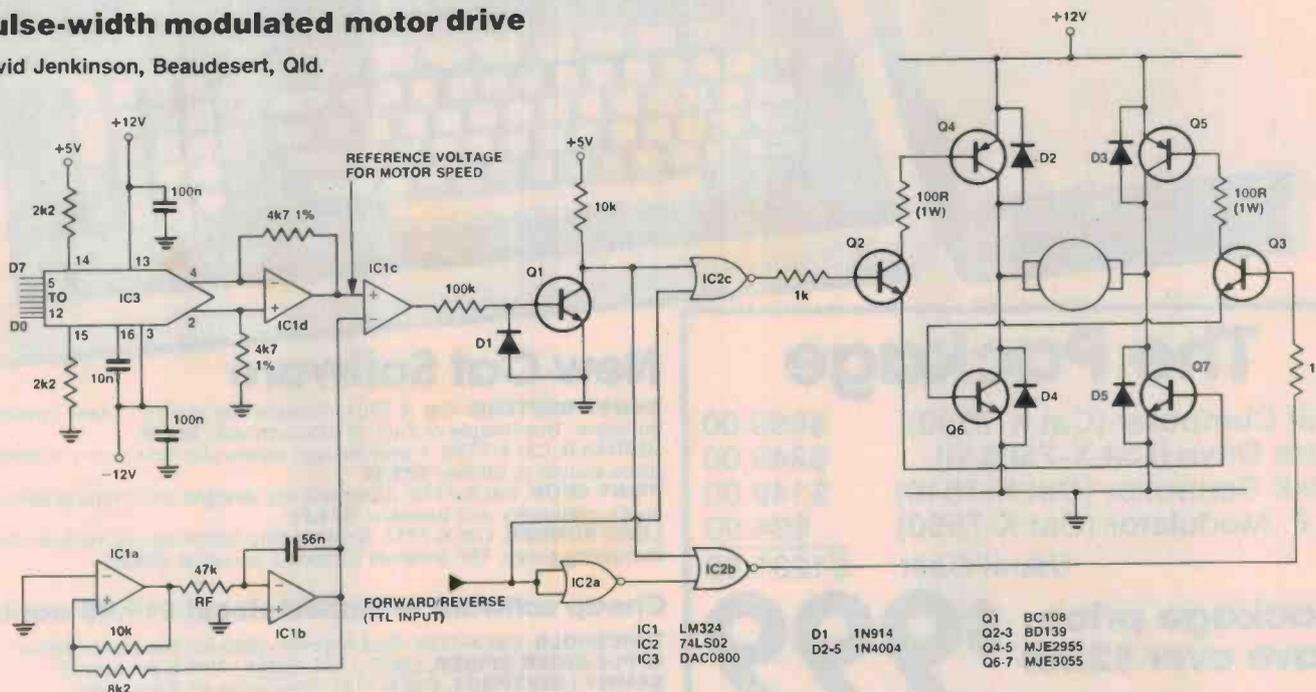
The following circuit was designed as the basis of a velocity control system for a small robot platform. However it may be used to control any small (up to 4 amp) permanent magnet dc motor, eg a slot-car or model train.
