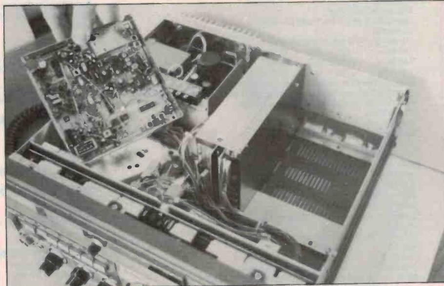
Inside the FT 726R showing the position of the satellite module and vacant space for 6 metre and 70 cm modules.
