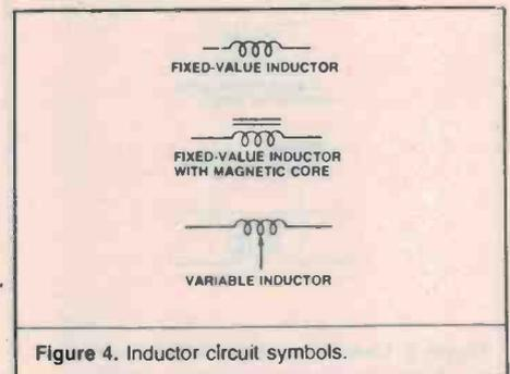
Figure 4. Inductor circuit symbols.
