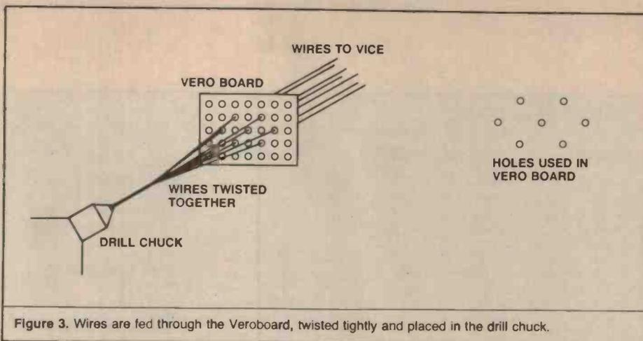
Figure 3. Wires are fed through the Veroboard, twisted tightly and placed in the drill chuck.
