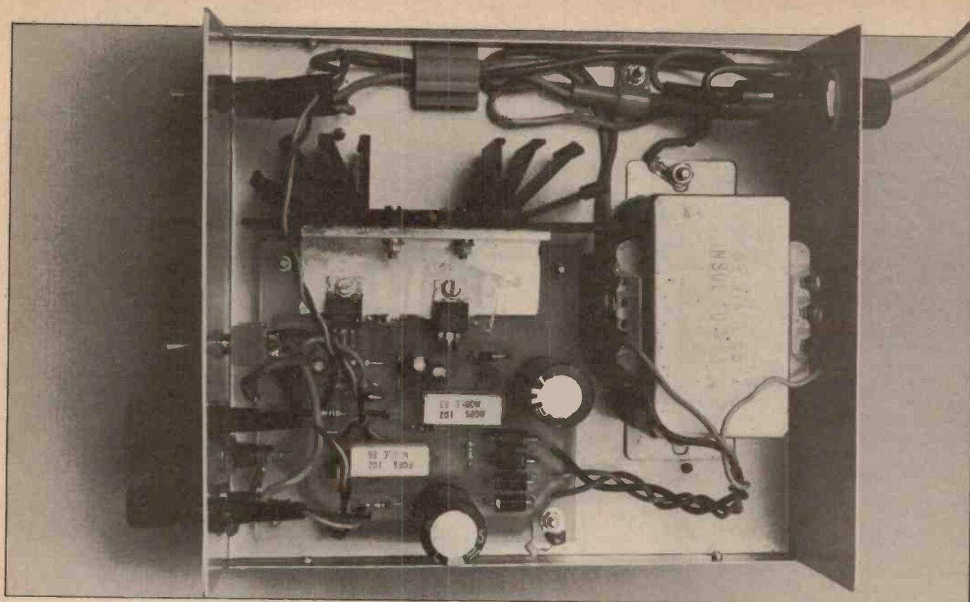
Above: The general layout inside the case. Make sure that the transformer and heatsink are clear of one another.
