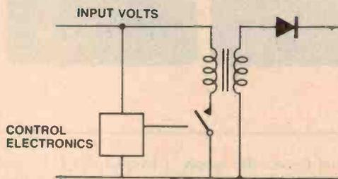
Figure 1. Simplified circuit.
