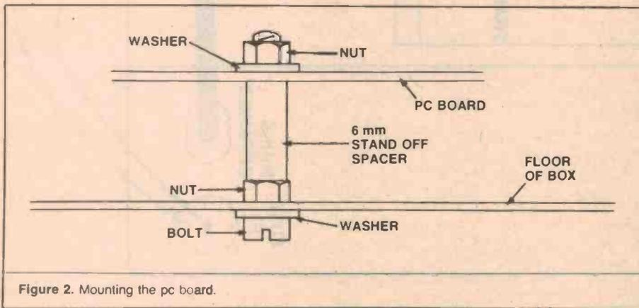
Figure 2. Mounting the pc board.
