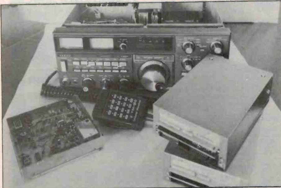
The FT 726R with satellite module (left), and 6 m and 70 cm modules ready for installation.
