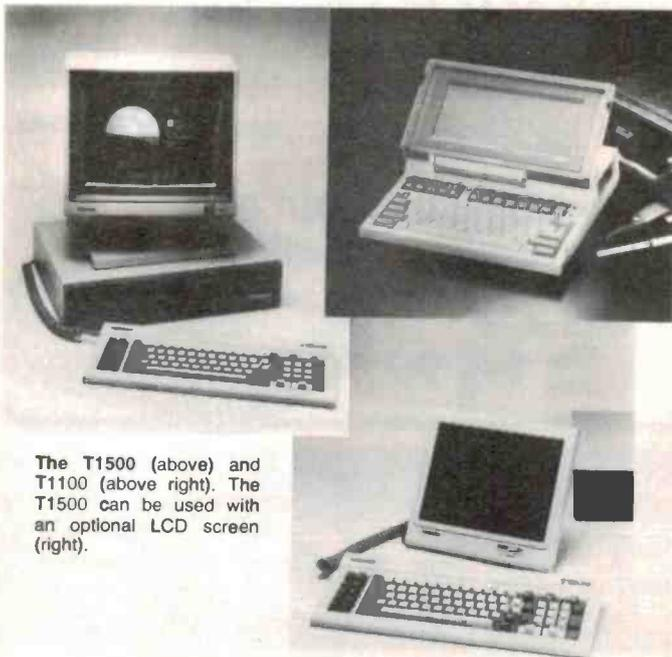
The T1500 (above) and T1100 (above right). The T1500 can be used with an optional LCD screen (right).
