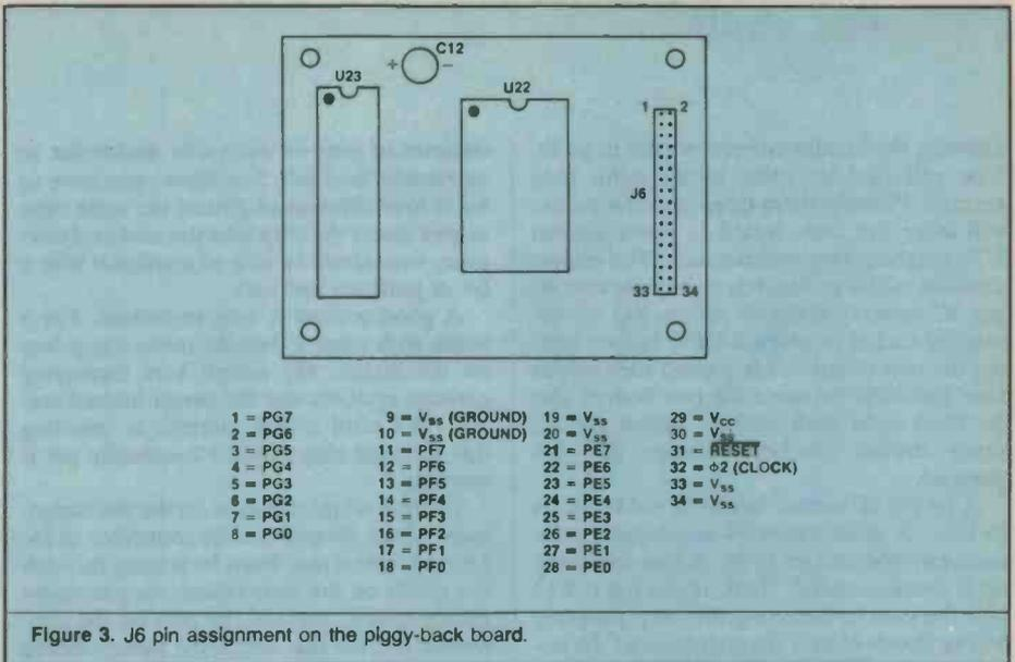
Figure 3. J6 pin assignment on the piggy-back board.
