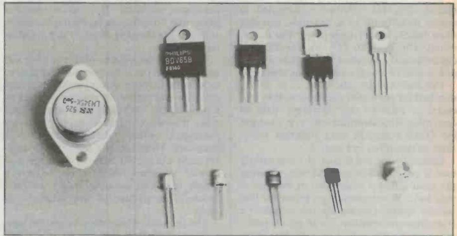
Transistors come in various packages. Shown here are (top, from left to right) a TO-3, SOT-93, TO-220, TO-202, TO-126; (bottom, from left to right) TO-72, TO-188, TO-92, TO-92 and TO-39.
