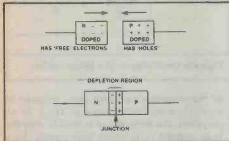
**Figure 1.** The pn junction: the doping process does not impart an electrical charge to the material; that is, if you measured it with a voltmeter no voltage would register. Rather, doping imparts carriers. The concentration of these carriers (holes and electrons) in the depletion region creates a barrier voltage of around 0.6 V for silicon and 0.2 V for germanium which must be overcome before the device can conduct.
