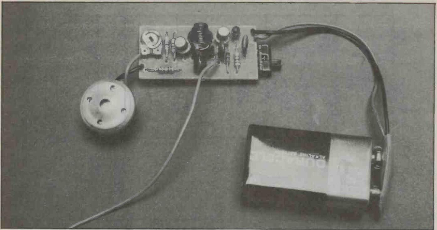
Now begin to solder the components on to the board. Begin with the resistors, then solder the two microphone leads into place. Then place the variable resistor. Do it in this order because one of the mic leads goes under the resistor, and it's rather tricky trying to get the wire into place if the resistors are already there. When you've done this, solder the two capacitors that fit on the component side into place, then the two transistors and the LED. Check the orientation of these components.
