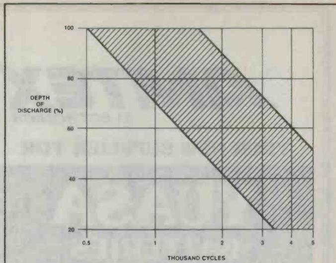
Figure 3. How to cycle NiCads — estimated life as a function of depth of discharge. Courtesy Technica.
