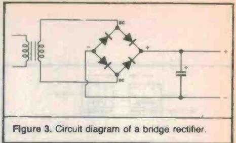
Figure 3. Circuit diagram of a bridge rectifier.
