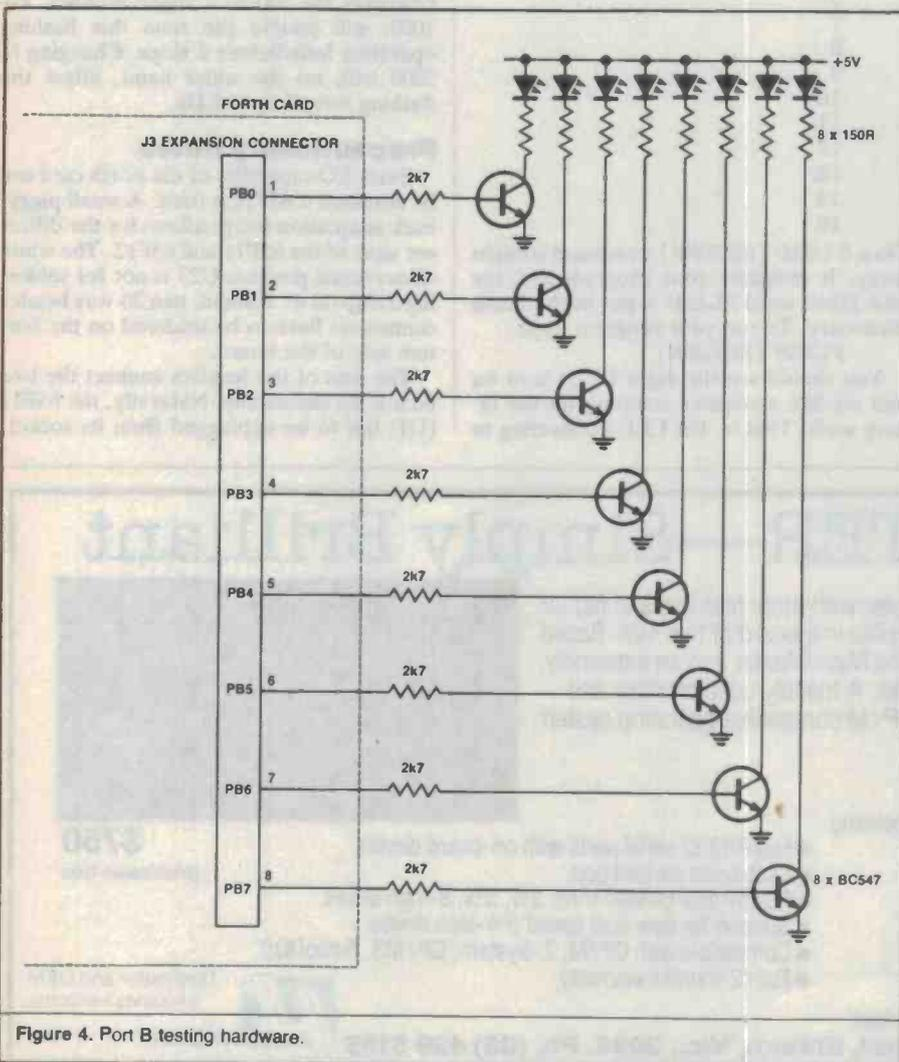
Figure 4. Port B testing hardware.
