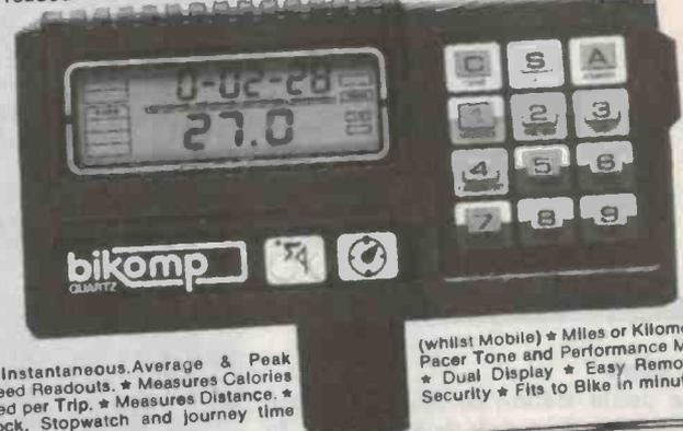
★ Instantaneous Average & Peak Speed Readouts. ★ Measures Calories Used per Trip. ★ Measures Distance. ★ Clock, Stopwatch and journey time
