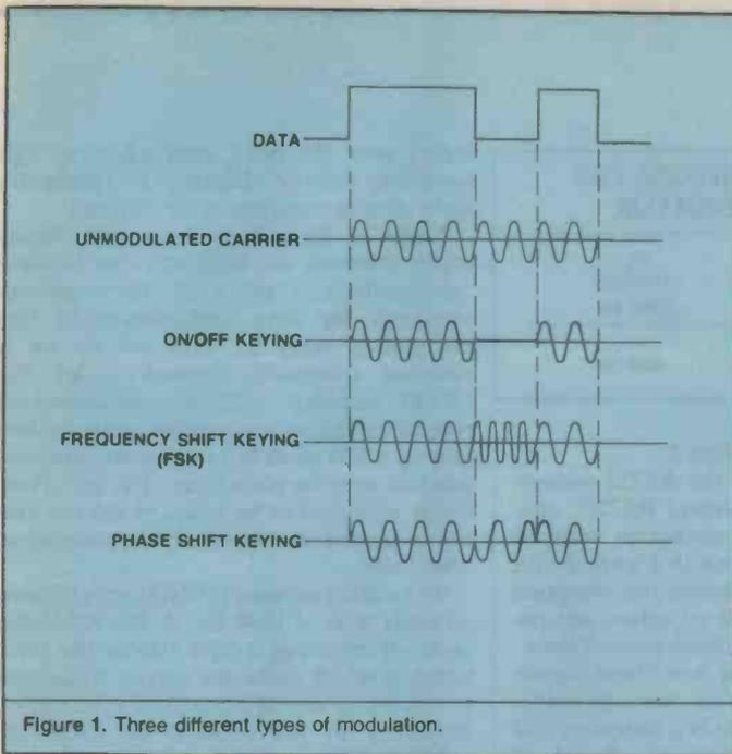
Figure 1. Three different types of modulation.
