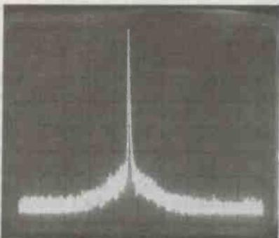
**Local oscillator injection at 100 MHz.** Vertical reference -50 dBm, 10 dB/div; horizontal 5 kHz/div; 100 Hz resolution 10 Hz VF. Note freedom from spurs and low noise close to oscillator frequency. This helps to produce a good reciprocal mixing figure and clean signals when using the synchronous detector.
