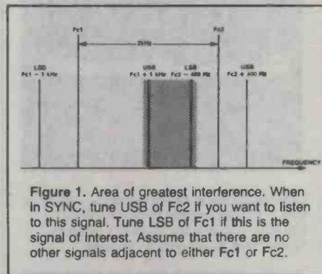
Figure 1. Area of greatest interference. When in SYNC, tune USB of Fc2 if you want to listen to this signal. Tune LSB of Fc1 if this is the signal of interest. Assume that there are no other signals adjacent to either Fc1 or Fc2.
