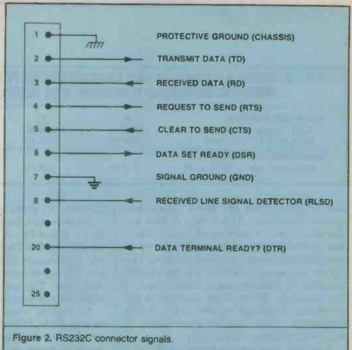
Figure 2. RS232C connector signals.
