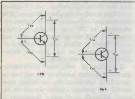
**Figure 6.** The names and polarities of normal operating voltages across transistors.  $V_{BE}$  is normally 0.6 V for a silicon transistor.  $V_{CEO}$  is the maximum value of  $V_{CE}$  that can be safely applied across the transistor. Reversing the polarity of  $V_{CE}$  or  $V_{BE}$  will often cause conduction in the reverse direction at voltages of about 5 V to 10 V.
