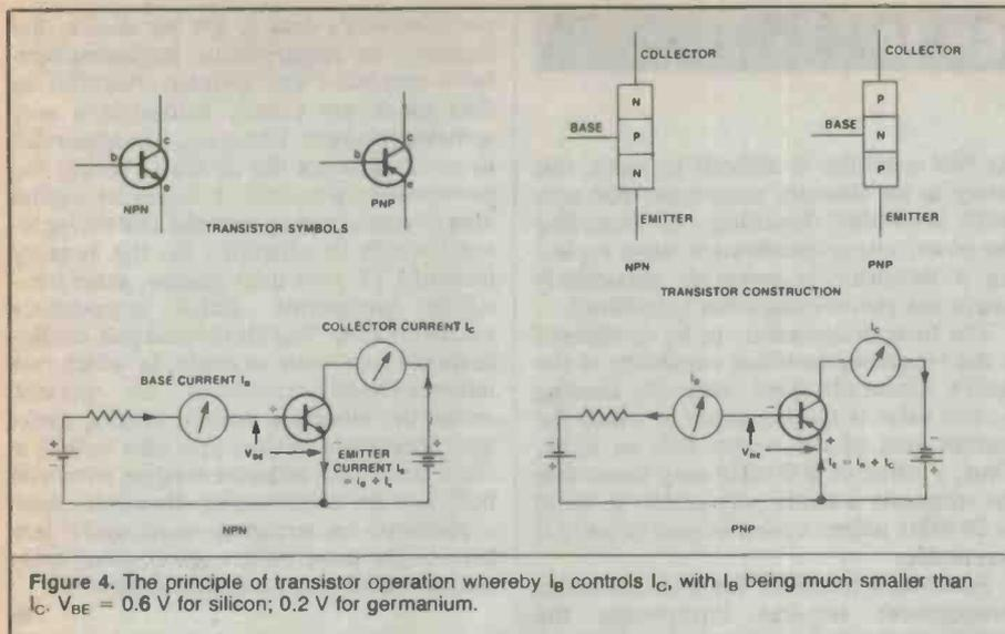
Figure 4. The principle of transistor operation whereby  $I_B$  controls  $I_C$ , with  $I_B$  being much smaller than  $I_C$ .  $V_{BE} = 0.6$  V for silicon; 0.2 V for germanium.
