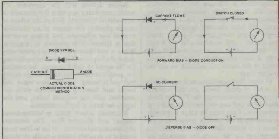
**Figure 2.** Diodes showing 'conventional current' flow, from positive to negative. A diode only conducts when the anode is positive with respect to the cathode.
