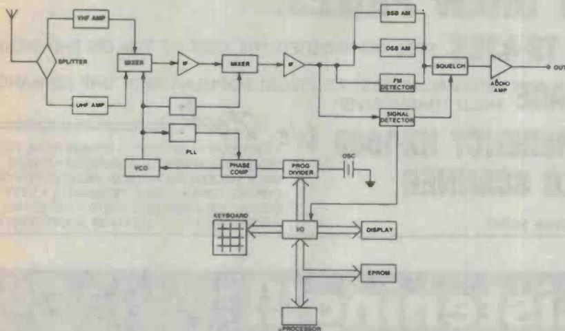
Figure 1. Typical block diagram of a scanner.
