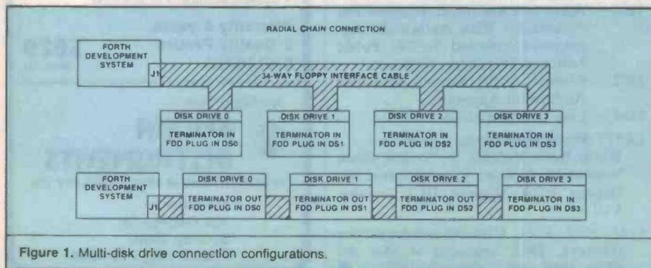
Figure 1. Multi-disk drive connection configurations.
