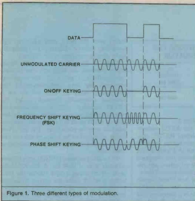
Figure 1. Three different types of modulation.
