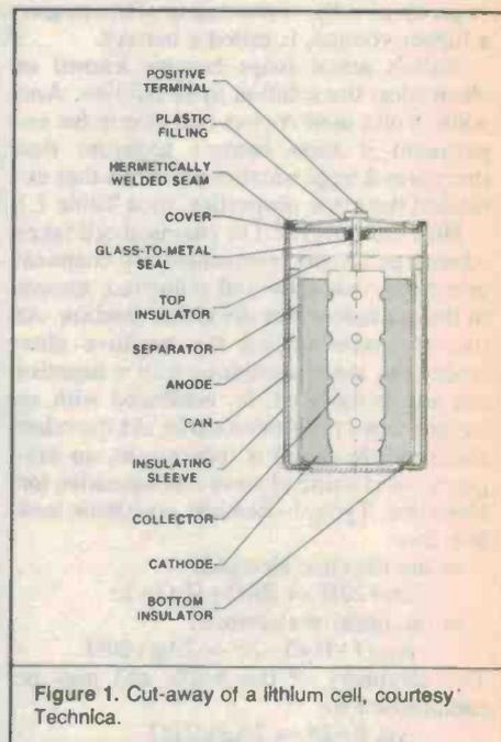
Figure 1. Cut-away of a lithium cell, courtesy Technica.
