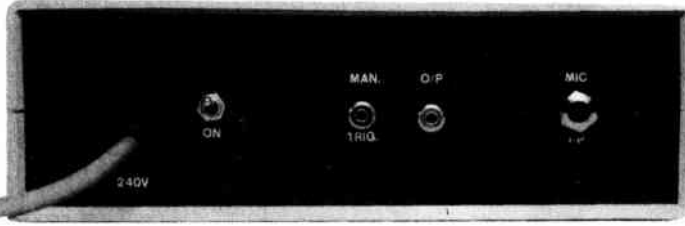
Back panel of the synthesiser. Sockets are provided for the manual trigger (an external footswitch) or a microphone, triggered by the snare drum for example.
