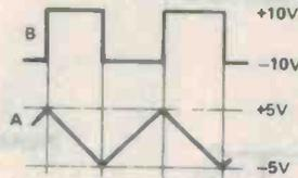
Output frequency  $F = (\text{pot fraction})/2RC$
