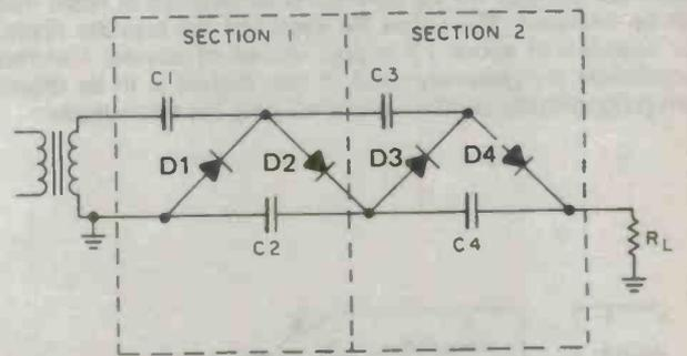
$V_0 = 2 \times V_{IN}$  PEAK-TO-PEAK
