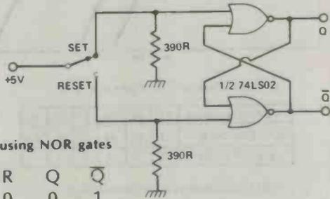
Flip-flop using NOR gates
