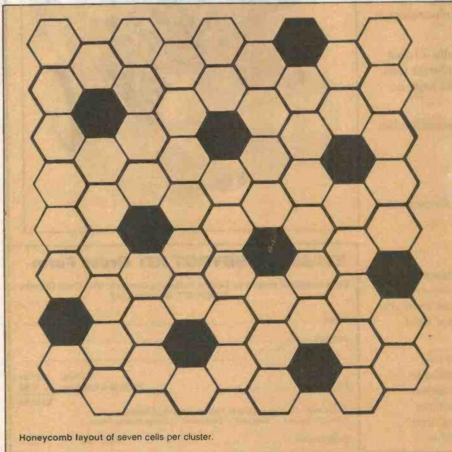
Honeycomb layout of seven cells per cluster.
