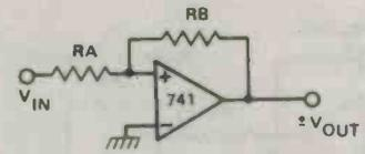
Non-inverting; input hysteresis levels =  $\pm(RA/RB) \times V_{OUT}$
