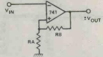
Inverting; input hysteresis levels =  $\pm(RA/(RA + RB)) \times V_{OUT}$
