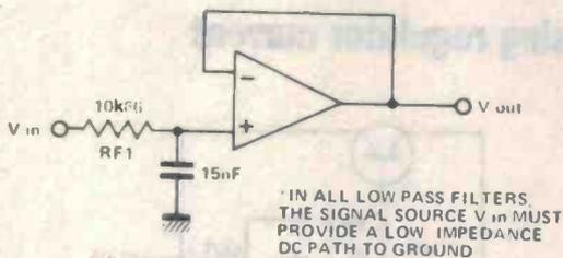
\*IN ALL LOW PASS FILTERS, THE SIGNAL SOURCE  $V_{in}$  MUST PROVIDE A LOW IMPEDANCE DC PATH TO GROUND
