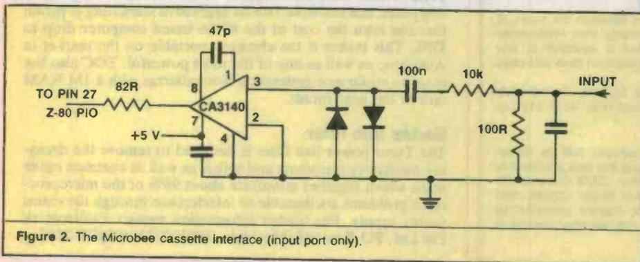
Figure 2. The Microbee cassette interface (input port only).
