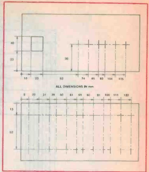
the display location on the back of the front panel so that it can be cut out in the correct place. When fitting is completed remove the board again to allow the remaining wiring to be done.
