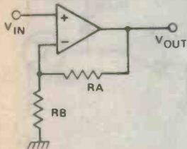
Non-inverting amplifier input must have a dc path to ground
