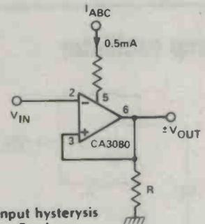
Transconductance type; input hysteresis levels =  $\pm V_{OUT}$ ;  $V_{OUT} = R \times I_{ABC}$
