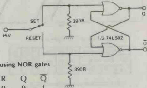
Flip-flop using NOR gates
