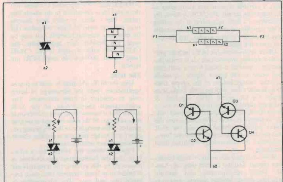
Figure 6. The diac: schematic symbol, basic construction, equivalent two-pnpn-Shockley diode representation, equivalent circuit and bias conditions.
