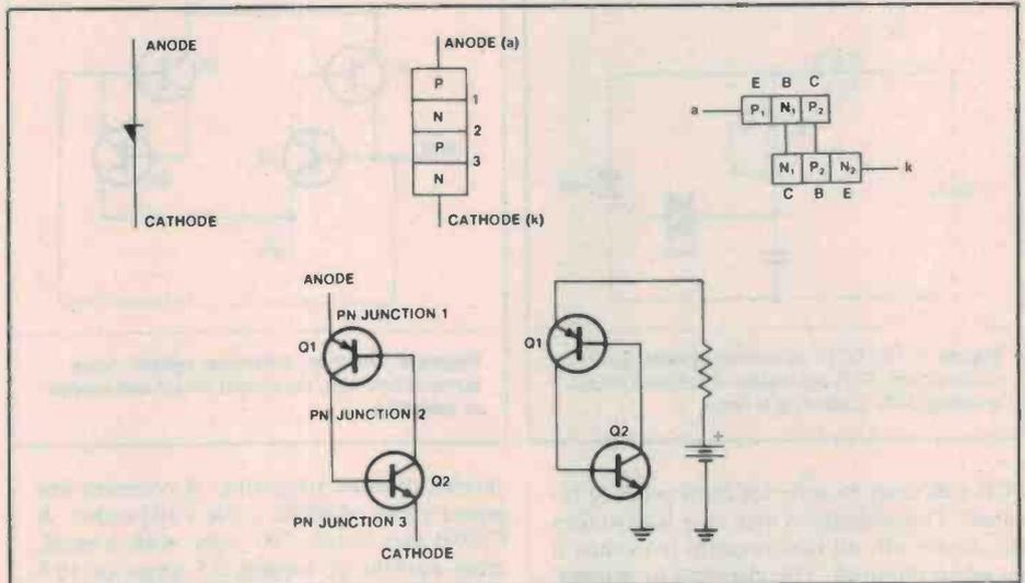
Figure 5. The Shockley diode: schematic symbol, basic construction and equivalent circuit.
