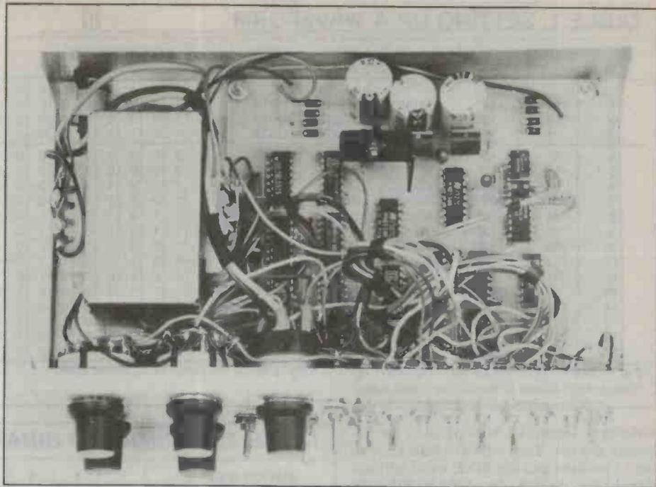
A view inside the case showing the location of the transformer and the pc board.
