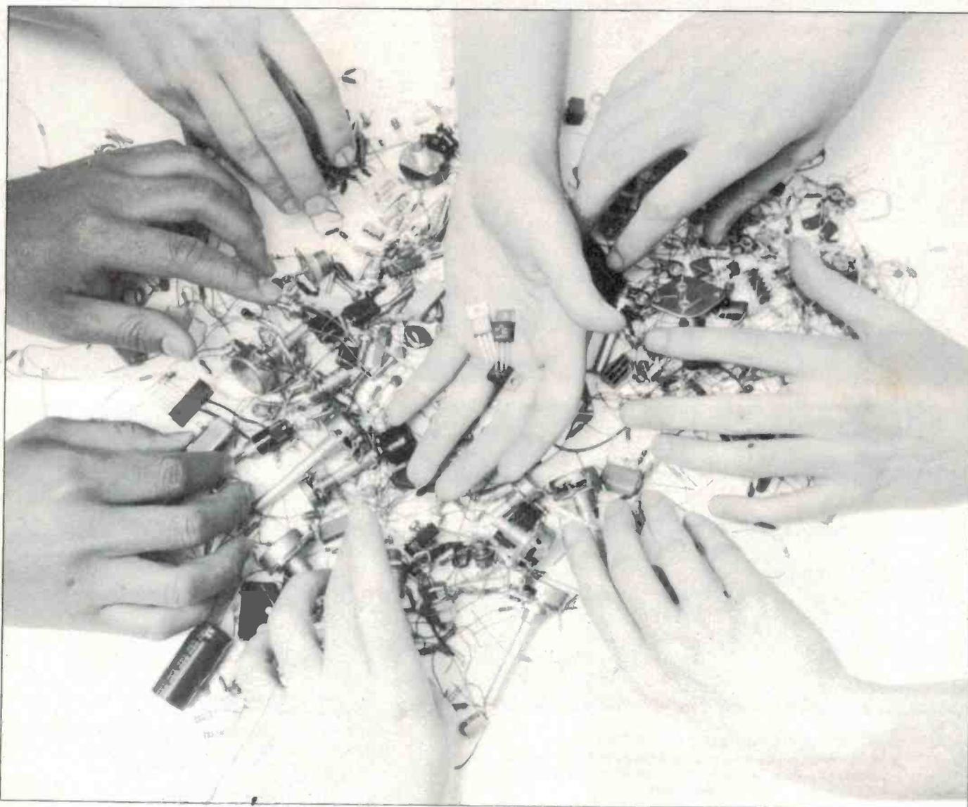
lieving them to be transistors. But, "it ain't necessarily so!" Such devices are discrete active components, 'discrete' because they are single devices rather than a part of an integrated circuit and 'active' because they need a power supply.
