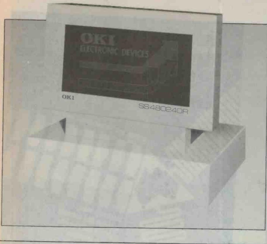
However, PDPs are far from being a perfect display vehicle. They are still monochrome in spite of the best effort of physicists, and the trade off for the bright screen is a distressingly high supply voltage. A typical anode voltage is 250 V for an orange screen; 280 V for green. Current flowing through the discharge cells can peak at 500 mA.
