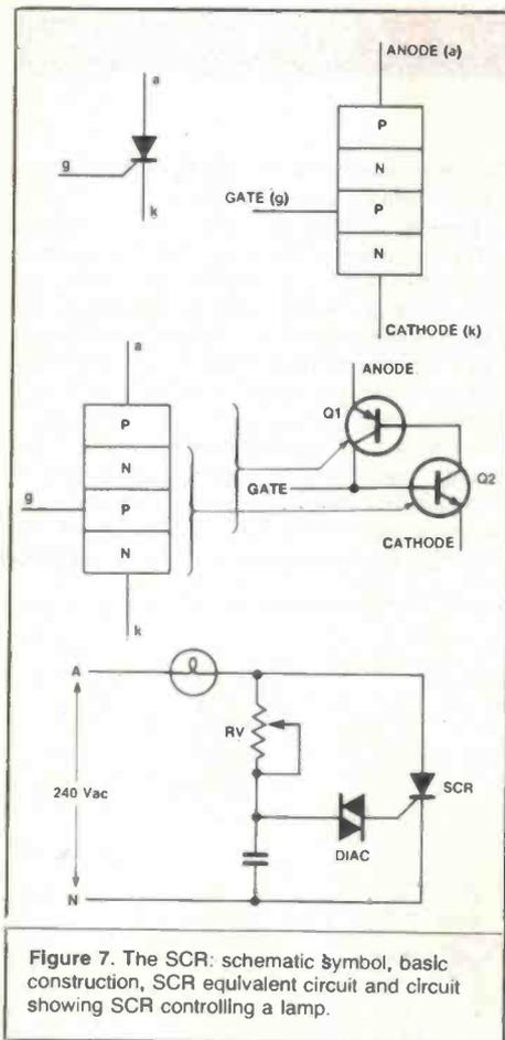
Figure 7. The SCR: schematic symbol, basic construction, SCR equivalent circuit and circuit showing SCR controlling a lamp.
