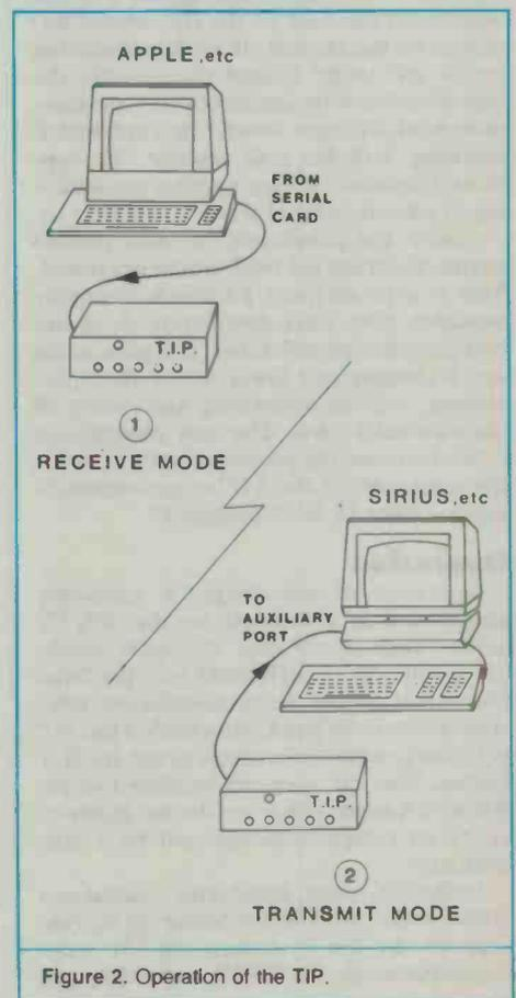
Figure 2. Operation of the TIP.
