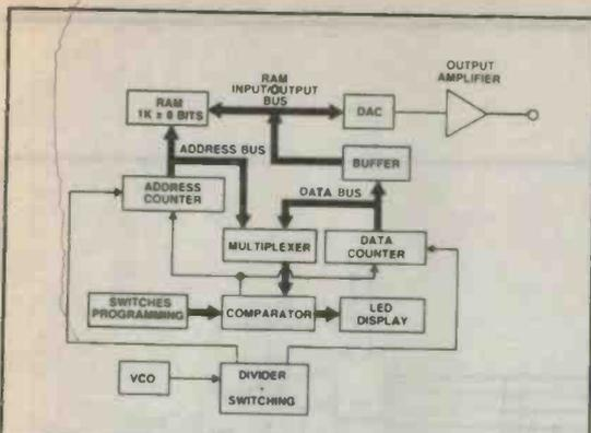
Figure 1. A block diagram of the arbitrary waveform generator.
