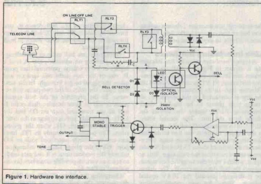
Figure 1. Hardware line interface.
