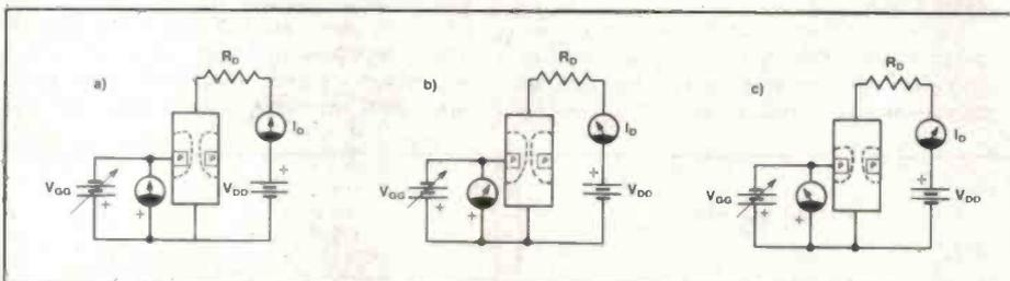
Figure 3. Operation of an n-channel JFET; a) JFET biased for conduction; b) greater  $V_{GS}$  narrows the channel, thus decreasing  $I_D$ ; c) less  $V_{GS}$  widens channel and increases  $I_D$ .
