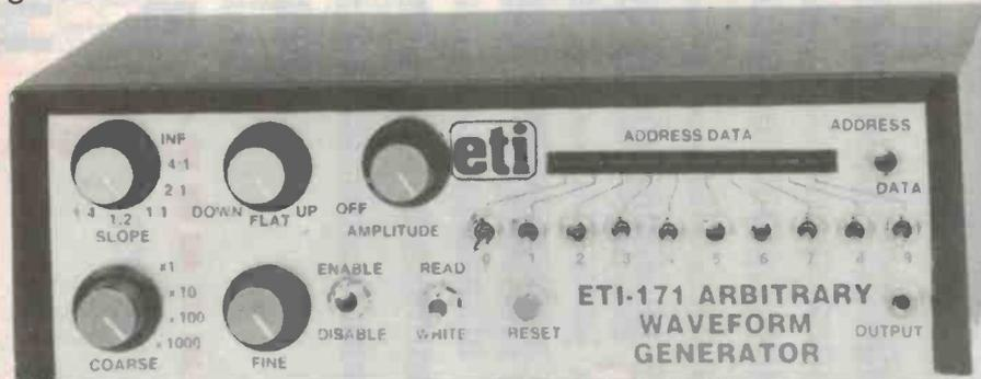
IN THE NOT too distant past when I was working with electronic test and measurement instrumentation, I was confronted with an instrument which could be programmed to create waveforms of any shape. This quite intrigued me. The applications of the device included simulation of waveforms, control signal generation and digital bit pattern generation. Instantly I saw it as the best thing since sliced bread due to its inherent flexibility and its potential for generating sound.
