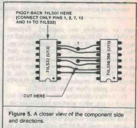
Figure 5. A closer view of the component side and directions.
