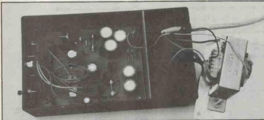
The hole size on the isolating (separating) plate has to be as small as possible, just big enough to allow three wires to go through from transformer to the pc board.
