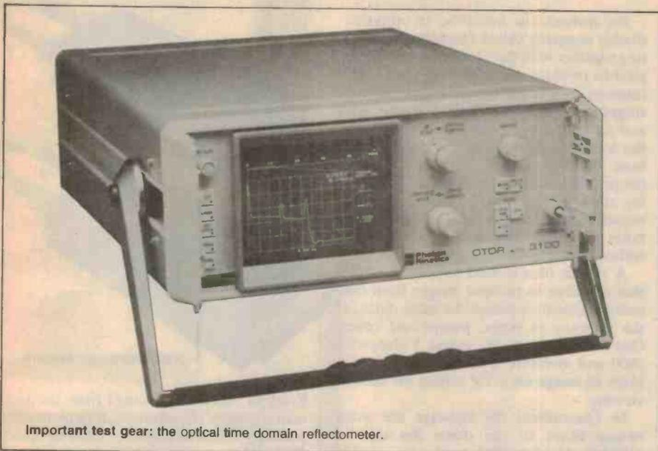
Important test gear: the optical time domain reflectometer.
