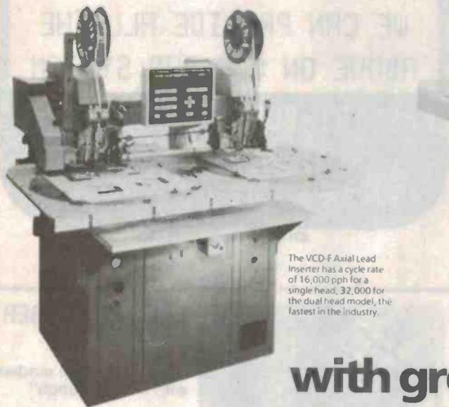
The VCD-F Axial Lead inserter has a cycle rate of 16,000 pph for a single head, 32,000 for the dual head model, the fastest in the industry.
