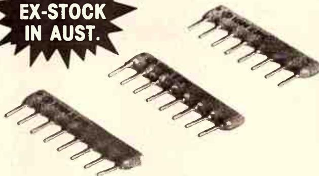
SPRAGUE ECONOLINE™ thick-film resistor networks include multiple isolated resistors, pull-up/pull-down and interface networks in low-profile-6-pin, 8-pin or 10-pin conforma-coated single in-line packages (SIPs). Pins are set on 0.100-in. centers. Packages are 0.200-in. high.
