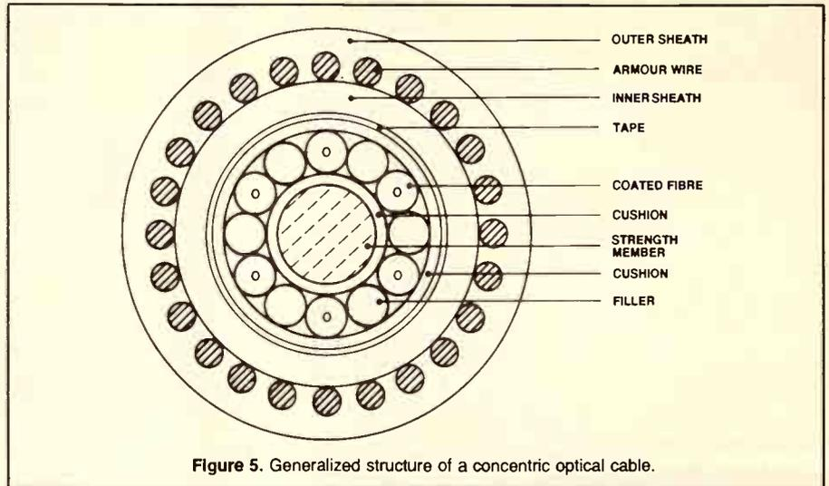
Figure 5. Generalized structure of a concentric optical cable.
