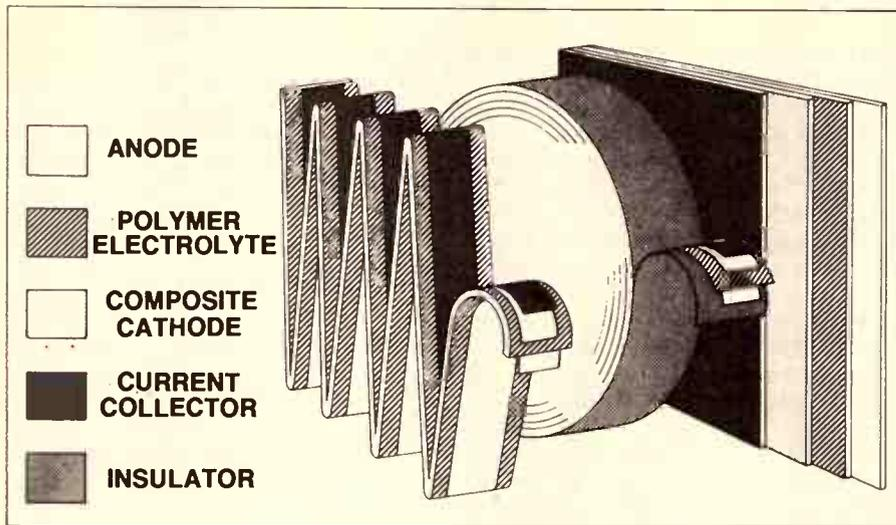
Figure 1. Three ways of constructing all-solid-state cells with large surface contact areas.
