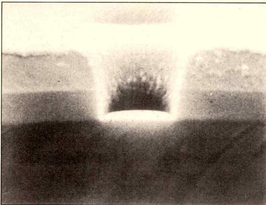
Contact hole in  $\text{SiO}_2$  showing sloped walls using controlled photoresist erosion (Plasma Technology).
