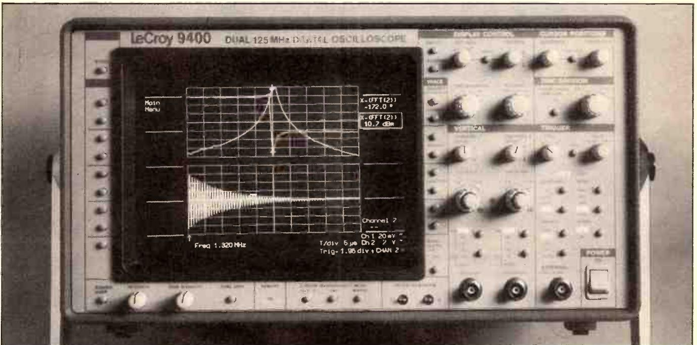
ETP Oxford has just released an FFT spectrum analysis package for the LeCroy 9400 digital oscilloscope. The screen shows a logarithmic amplitude against phase transform of the bottom trace, a 50  $\mu$ s damped sine wave.
