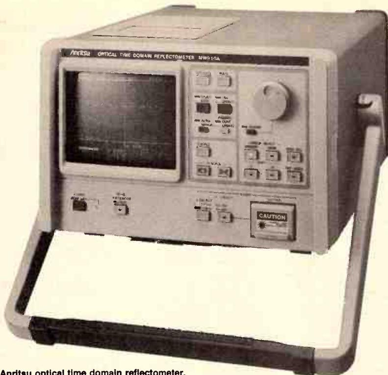
An Anritsu optical time domain reflectometer.
