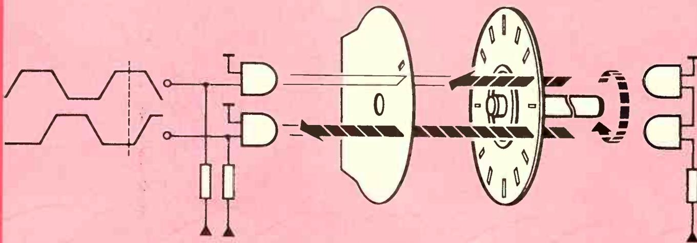
Figure 1. Schematic of rotary switch circuitry.
