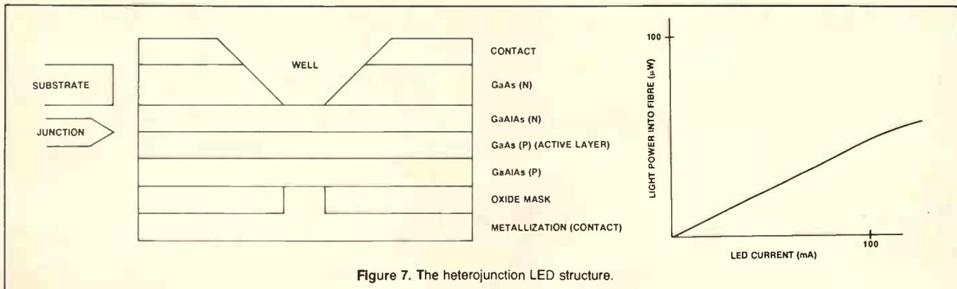
Figure 7. The heterojunction LED structure.
