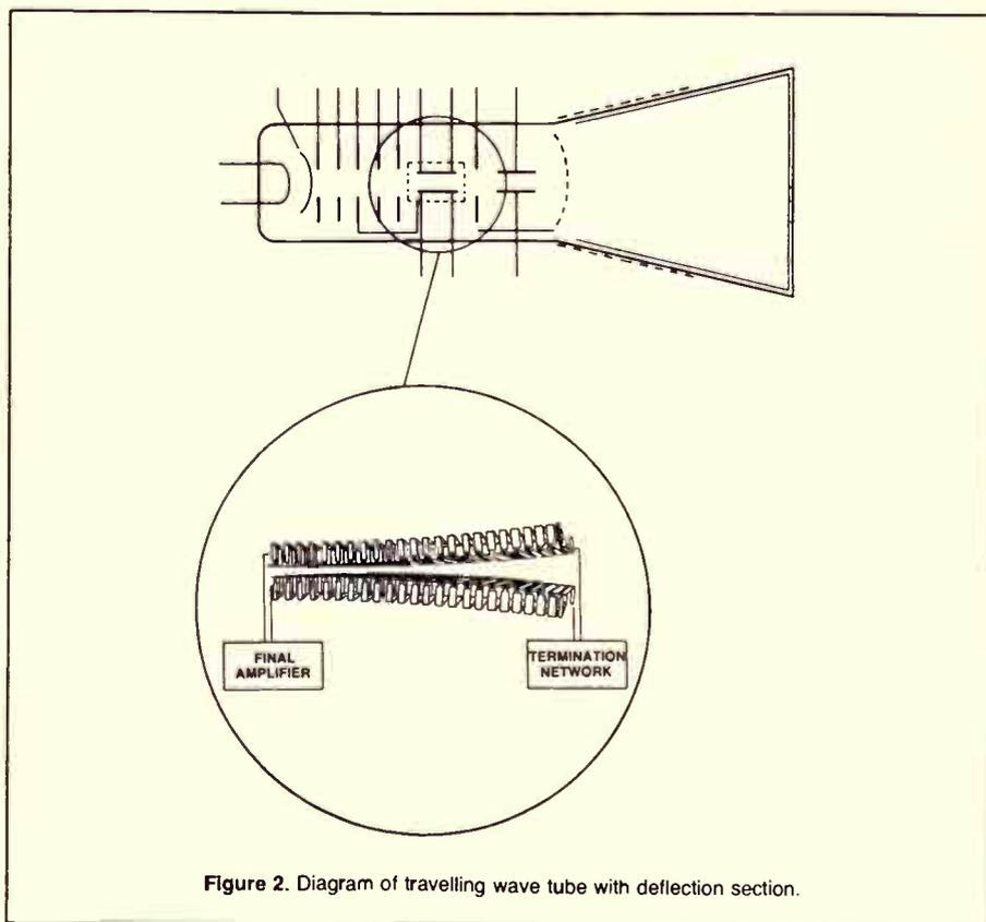
Figure 2. Diagram of travelling wave tube with deflection section.
