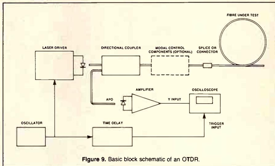
Figure 9. Basic block schematic of an OTDR.
