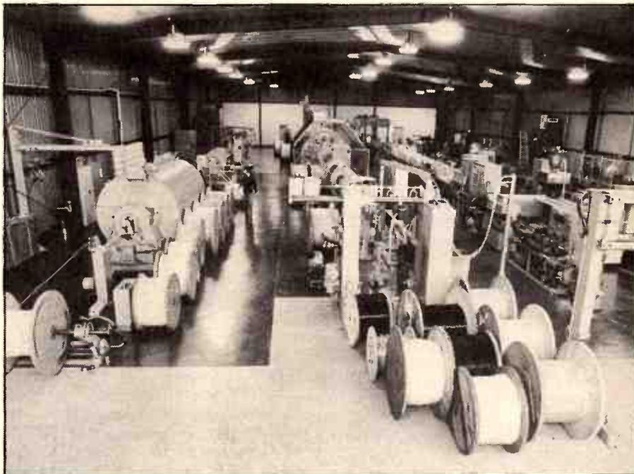
The manufacture of fibre optic cable at Olex, Melbourne.
