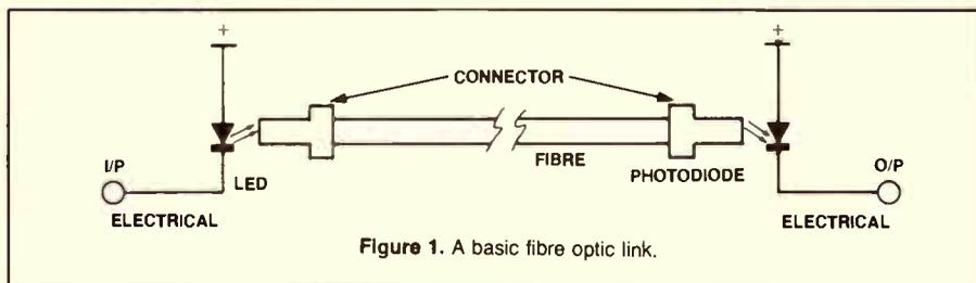
Figure 1. A basic fibre optic link.
