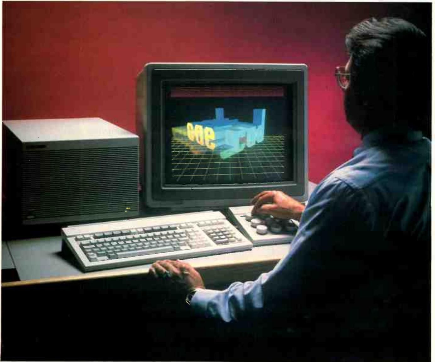
High-performance solid-rendering graphics at interactive speed are now possible with Hewlett-Packard Company's new HP 9000 Model 320SRX technical workstation. With Model 320SRX HP believes that solid images now can be rendered 10 to 20 times faster than on other workstations in a similar price range, due to innovative graphics architecture, custom VLSI and capabilities in hardware and microcode.
