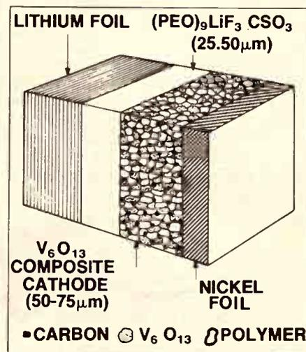
Figure 2. Basic arrangement of the elements of an all-solid-state cell. The notation PEO stands for poly(ethylene oxide).
