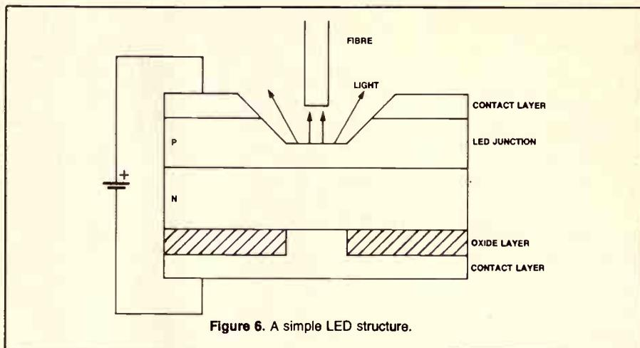
Figure 6. A simple LED structure.
