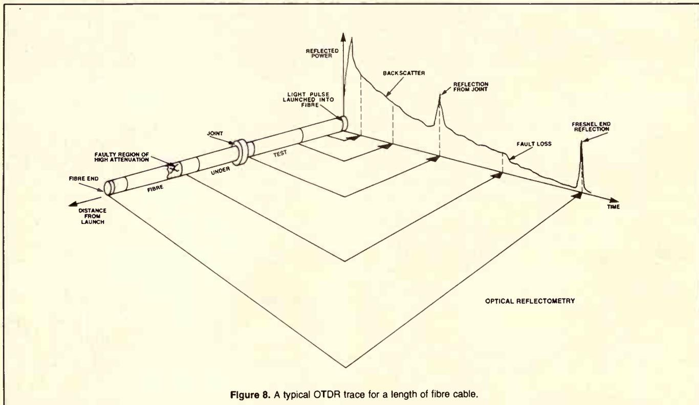
Figure 8. A typical OTDR trace for a length of fibre cable.
