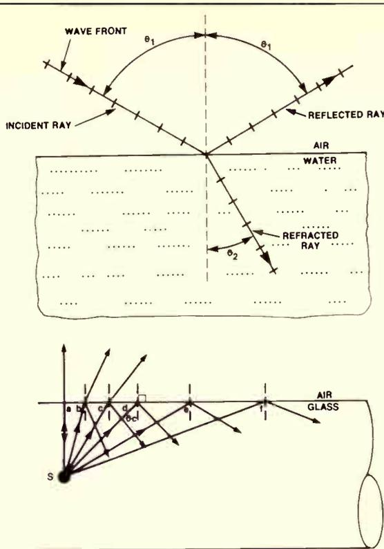
Figure 3. Total internal reflection.
