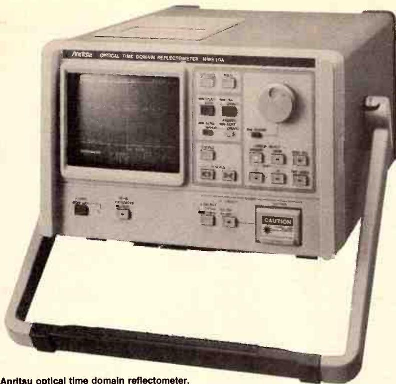
An Anritsu optical time domain reflectometer.
