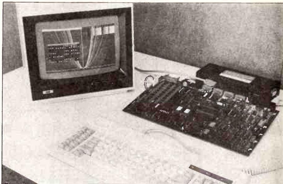
the MC68000, it has some extra instructions some of which have been made more efficient, but the main rationale for the introduction of the MC68010 is probably as a 'fix' for a limitation of the MC68000 which prevented it from resuming a program after a memory fault — a capability which is necessary for large operating systems. This MC68010 feature is not needed in a system of the 1616's size.
