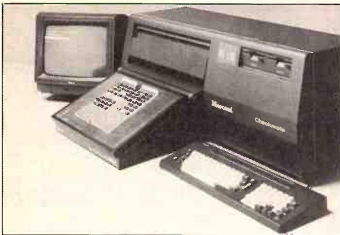
**Marconi Instruments is showing its recently-launched Checkmate bench-top ATE tester. The device offers high-speed digital testing, analogue functional and in-circuit capability with a GPIB interface and fully Interactive programming.**
