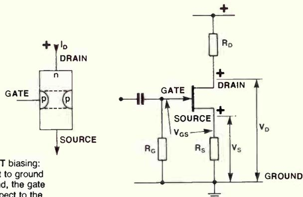
Figure 2. The n-channel JFET. FET biasing: because  $V_S$  is positive with respect to ground and the gate is connected to ground, the gate (and) ground are negative with respect to the source.
