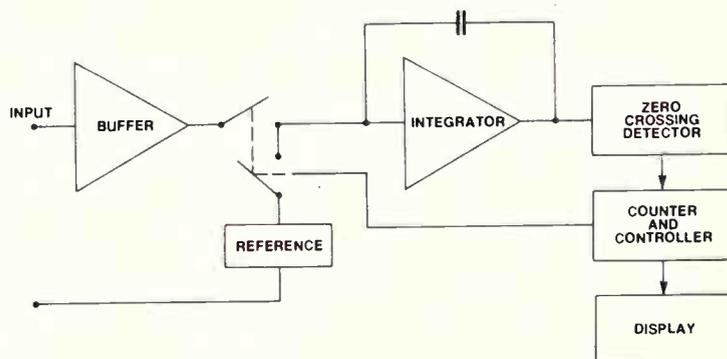
Figure 2. Block diagram of multislope approximation architecture.
