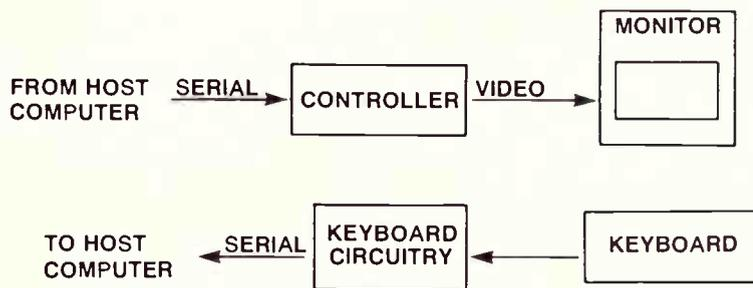
Figure 1. Monitor, keyboard and controller as a VDU.
