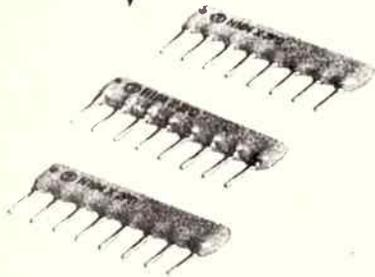
**SPRAGUE ECONOLINE**<sup>TM</sup> thick-film resistor networks include multiple isolated resistors, pull-up/pull-down and interface networks in low-profile 6-pin, 8-pin or 10-pin conforma-coated single in-line packages (SIPs). Pins are set on 0.100-in. centers. Packages are 0.200-in. high.
