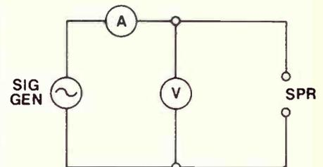
Figure 1. Speaker test circuit.
