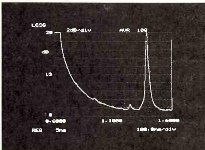
Figure 3. Loss wavelength characteristics of GI fibre (2 km).
