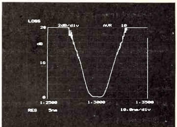
Figure 4. Loss wavelength characteristics of optical fibre.
