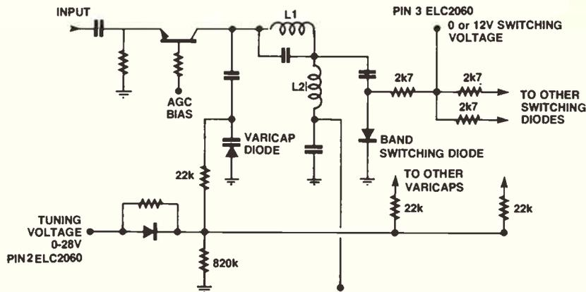
Figure 2. Tuning and band switching methods.
