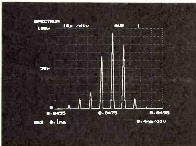
Figure 1. 0.85  $\mu\text{m}$  LD spectrum.
