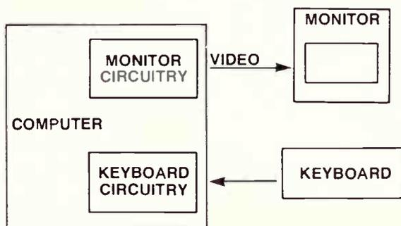
Figure 2. Monitor and keyboard attached to a microcomputer.
