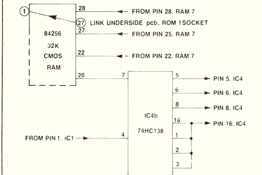
Figure 2. Circuit changes to use 32K CMOS RAM in NEC 8201A "ROM1" socket.
