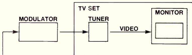
Figure 4. Modulator turns into a monitor.
