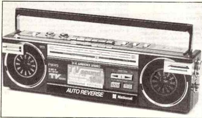
The unique new portable radio/cassette recorder from National, the RX1 M45V, features two bands for receiving TV audio signals as well as four other frequency bands including FM, AM and shortwave.
