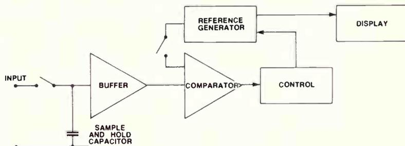
Figure 1. Block diagram of successive approximation architecture.
