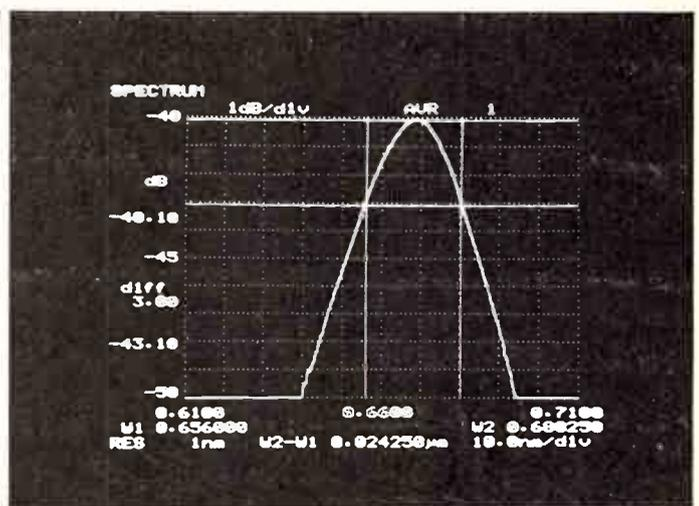
Figure 2. 0.66  $\mu\text{m}$  LED spectrum.
