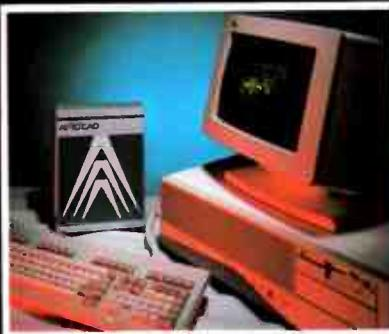
The NCR PC8 Advanced Technology (AT) PC is an ideal CAD workstation with its 8 MHz 80286 processor and native 640 by 400 colour graphics capability.
