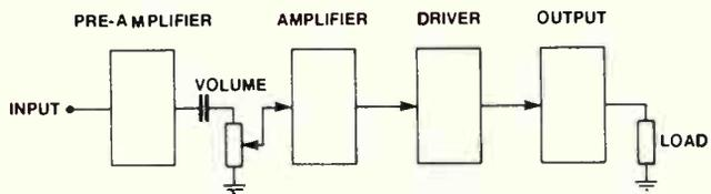
Figure 1. Block diagram of a typical audio amplifier.
