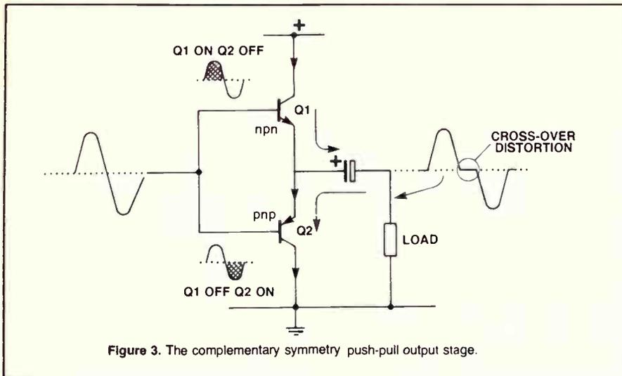
Figure 3. The complementary symmetry push-pull output stage.
