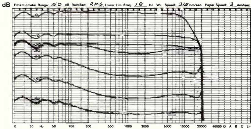
Figure 3: Swept frequency signals on NF S90 tape using the CAR circuit in 10dB steps.
