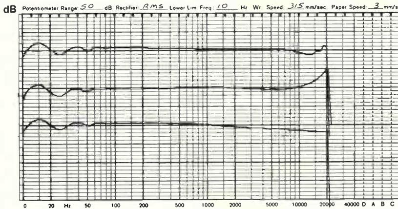
Figure 2: Record to replay reponse at -20 VU. All the traces are displaced for clarity. Top is a Sony HF-S90 (Type I) with Dolby B. Middle is a Denon DX8/60 with normal bias and no Dolby. At the bottom is a Technics RT 60MK, also with no Dolby and normal bias.
