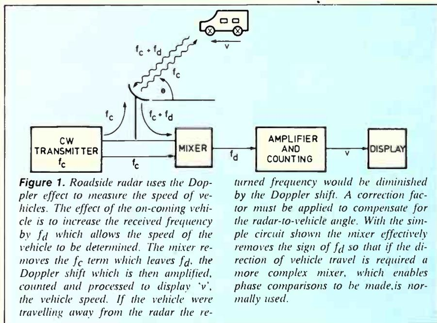
**Figure 1.** Roadside radar uses the Doppler effect to measure the speed of vehicles. The effect of the on-coming vehicle is to increase the received frequency by  $f_d$  which allows the speed of the vehicle to be determined. The mixer removes the  $f_c$  term which leaves  $f_d$ , the Doppler shift which is then amplified, counted and processed to display 'v', the vehicle speed. If the vehicle were travelling away from the radar the re-
