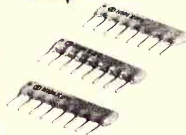
**SPRAGUE ECONOLINE™** thick-film resistor networks include multiple isolated resistors, pull-up/pull-down and interface networks in low-profile-6-pin, 8-pin or 10-pin conforma-coated single in-line packages (SIPs). Pins are set on 0.100-in. centers. Packages are 0.200-in. high.
