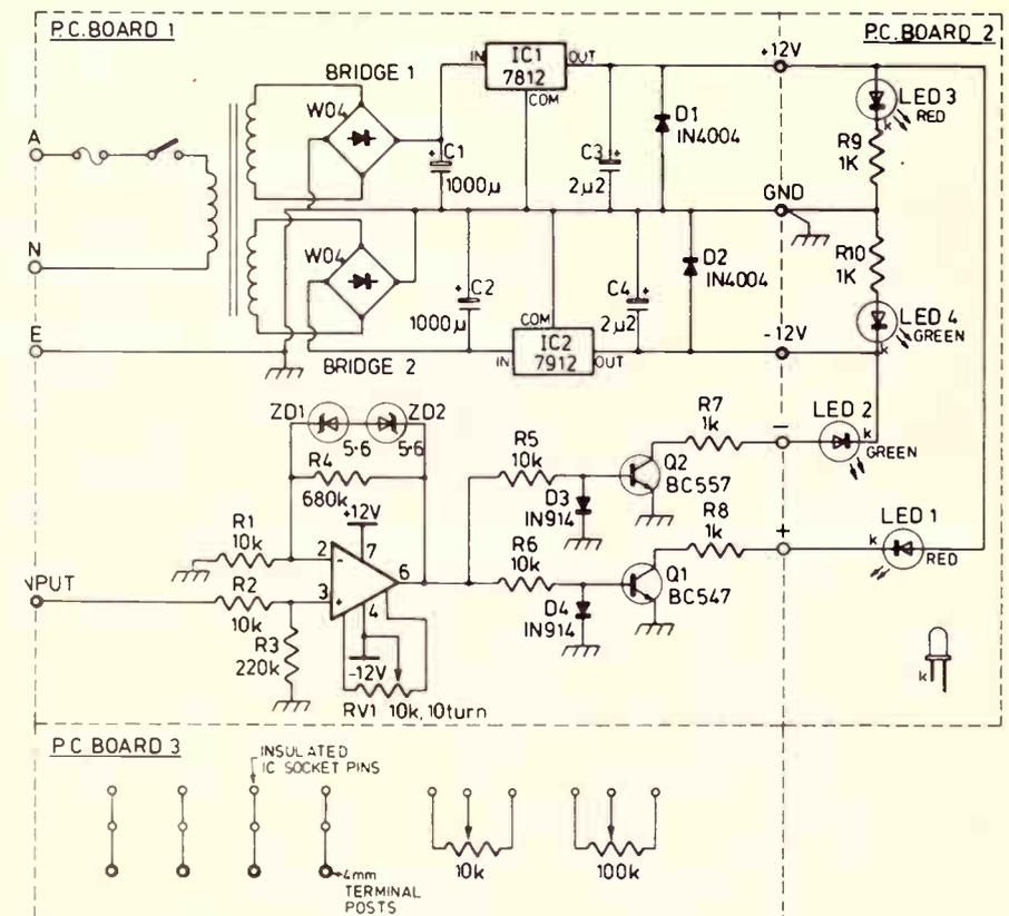
ate, supplied when the input to the op amp exceeds +10 mV. Similarly, applying -10 mV or more to the input will cause Q2 to switch on. Diodes D3 and D4 protect the transistors against reverse conduction. The input resistance of the circuit is around 200k ohms, allowing the circuit to be used
