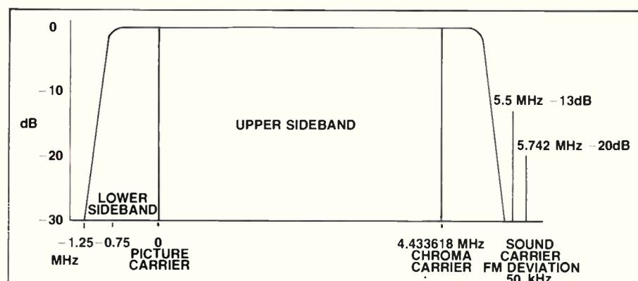
Figure 1. Standard TV channel transmission 7 MHz wide.
