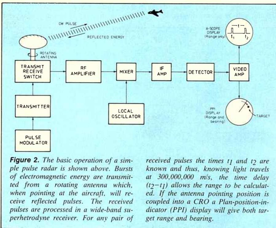
**Figure 2.** The basic operation of a simple pulse radar is shown above. Bursts of electromagnetic energy are transmitted from a rotating antenna which, when pointing at the aircraft, will receive reflected pulses. The received pulses are processed in a wide-band superhetrodyne receiver. For any pair of
