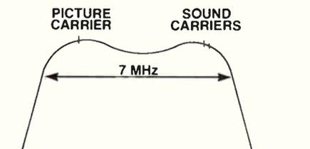
Figure 2. Typical tuner rf characteristic curve.
