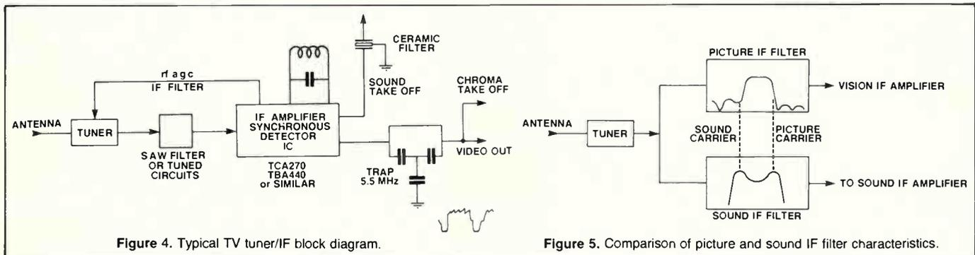
Figure 4. Typical TV tuner/IF block diagram.
