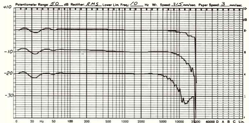
Figure 1: Frequency response. Top is Type I reference tape (Maxwell UDXL), centre is Type II (TDK SA) and bottom is Type IV (TDK WA). The traces are offset by 10 dB for the sake of clarity.
