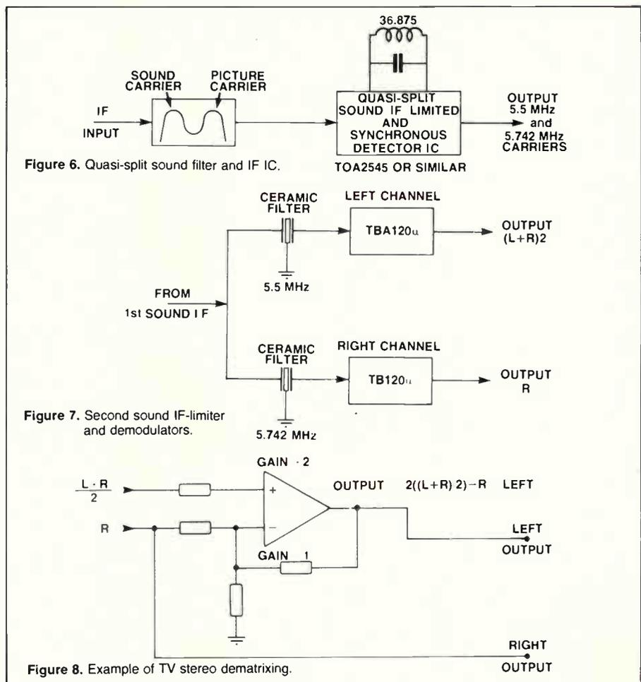
Figure 6. Quasi-split sound filter and IF IC.
