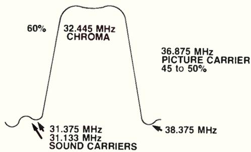
Figure 3. Typical IF characteristic curve.
