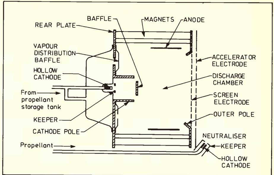
Figure 2: Schematic layout of an electron bombardment ion engine.
