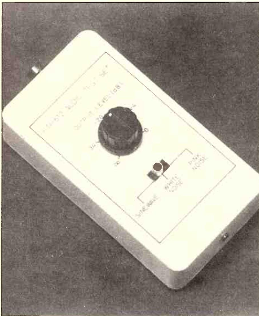
THE IDEA BEHIND this project was to design a small, hand held, and battery operated test instrument that could be used to perform many of the tests usually done with bulky mains operated equipment. This test set consists of three signal sources. A low distortion, 1 KHz calibrated amplitude sinewave, white noise source, and a pink noise source.
