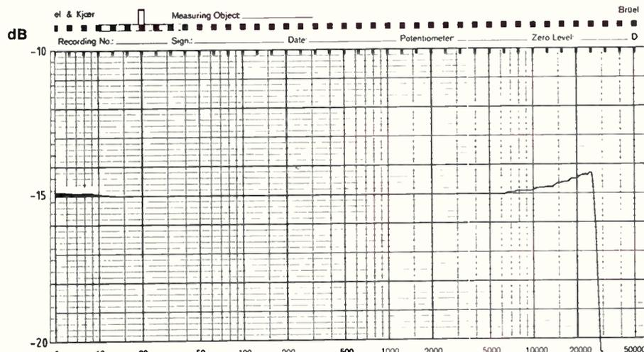
Above: Frequency response for left channel. Below: Right channel. (10 dB log plot)
