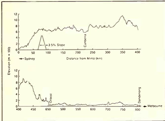
Figure 2. Natural surface profile from Sydney to Melbourne, along the route of the VFT
