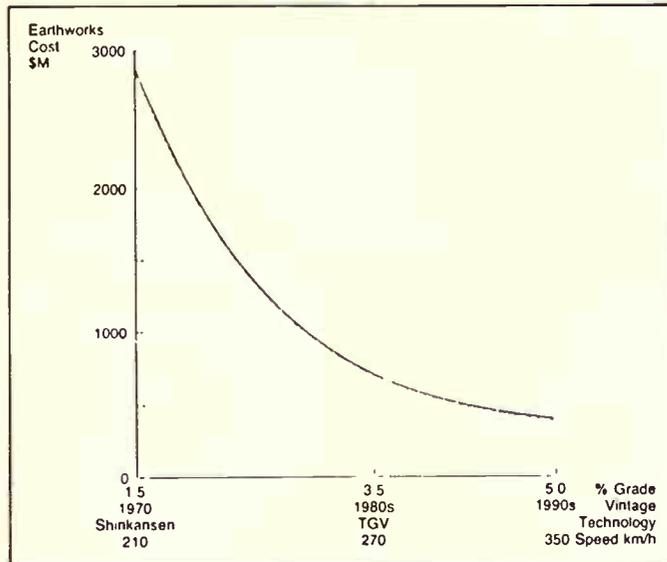
Figure 3. Earthworks cost us grade limit, technology, speed
