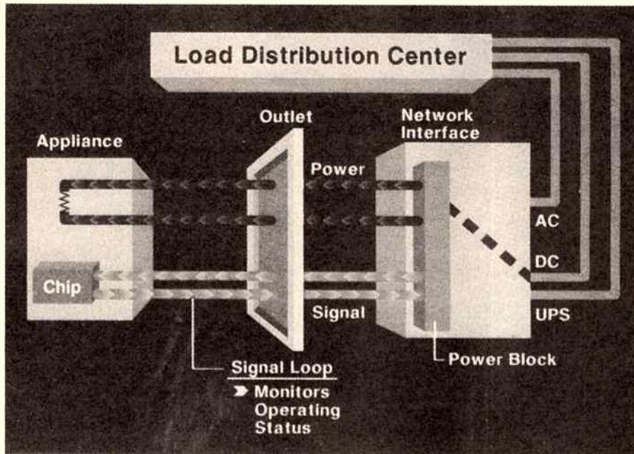
Once an appliance identifies itself and signals for energy, it is supplied and its use is continually monitored. AC or DC may be called up by the appliance. A low-voltage uninterruptible power supply (UPS) maintains signalling operations should main power fail. In the case of gas interface monitors pressure and flow.
