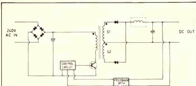
Figure 6: A typical switcher design for the 50-100 V range.
