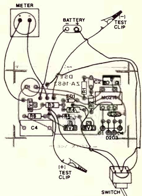
the 50V range and connect the 30V zener across the test clips. Adjust RV3 for a correct reading. This completes the setup procedure.
