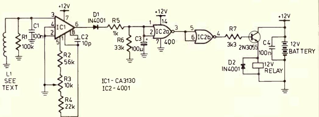
on for a suitable time. IC2 acts as a buffer to prevent C3 discharging through the transistor. R3 is a sensitivity control, adjusting the offset voltage of IC1 so that the small input voltage will trigger the circuit.
