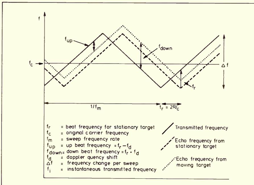
**Figure 3** FM-CW may be used to determine the range of a moving target. The CW of frequency  $f$  is modulated in frequency over a period  $1/f_m$ . On the up-sweep the echo signal range frequency  $f_r$  will be reduced by the Doppler shift  $f_d$  whilst on the down-swing the echo frequency will be increased by  $f_d$ . The range may then be deduced.
