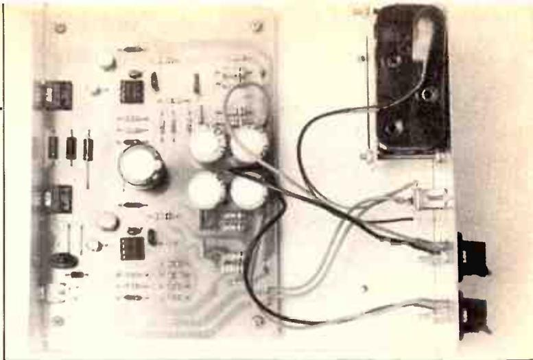
Top view of the pc board and the battery holder inside the box.
