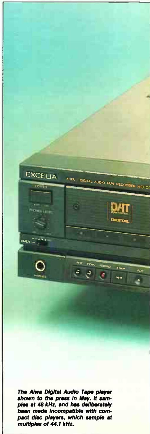
The Aiwa Digital Audio Tape player shown to the press in May. It samples at 48 kHz, and has deliberately been made incompatible with compact disc players, which sample at multiples of 44.1 kHz.
