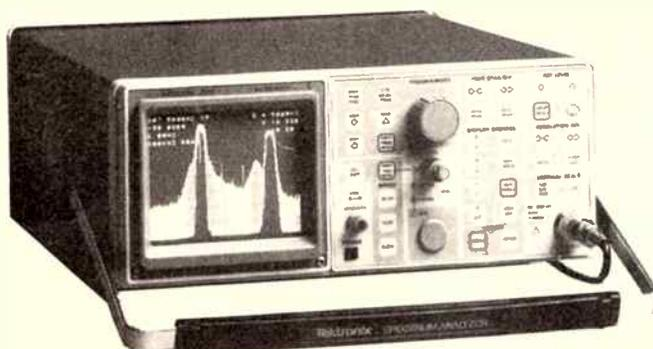
Computer control allows sophisticated ergonomics. Primary functions are accessed via dedicated keys on the front panel, and less important ones via menu driven displays. If the
