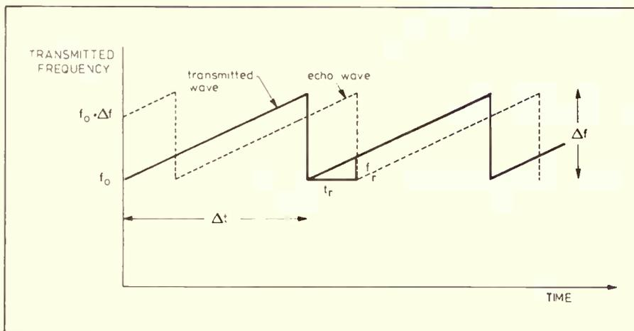
**Figure 1** The sawtooth frequency modulation of a CW of fundamental frequency  $f_0$  by  $\Delta f$  in time  $\Delta t$  provides range information from a fixed target. The echo signal received will lag the transmitter signal by  $t_r$  and so if the frequency difference  $f_r$  is measured at this point the range may be determined and displayed.
