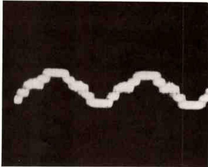
Output from a sine wave input at -80 dB
