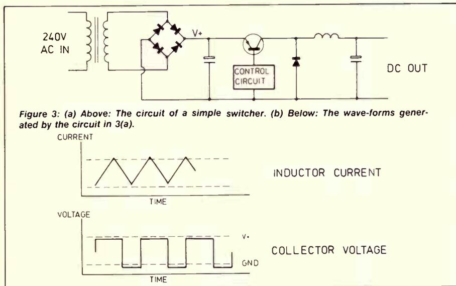
Figure 3: (a) Above: The circuit of a simple switcher. (b) Below: The wave-forms generated by the circuit in 3(a).
