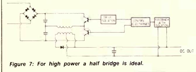
Figure 7: For high power a half bridge is ideal.
