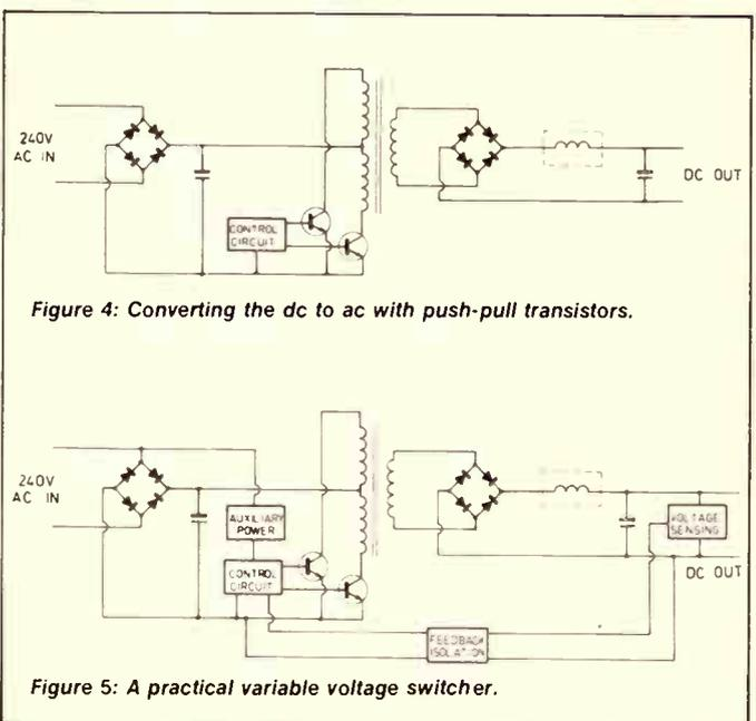
Figure 4: Converting the dc to ac with push-pull transistors.
