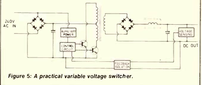
Figure 5: A practical variable voltage switcher.
