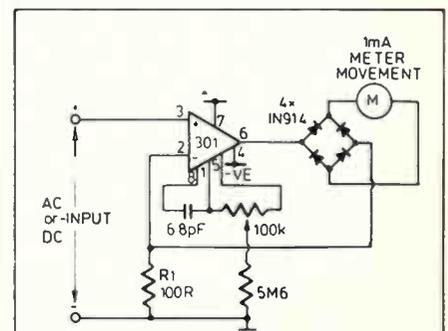
Figure 3: An ac/dc mV meter
