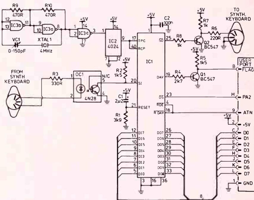
pins will be in a high impedance mode and won't interfere with input. IC1 is clocked by IC2 and IC3. The clock oscillates at the crystal fre-
