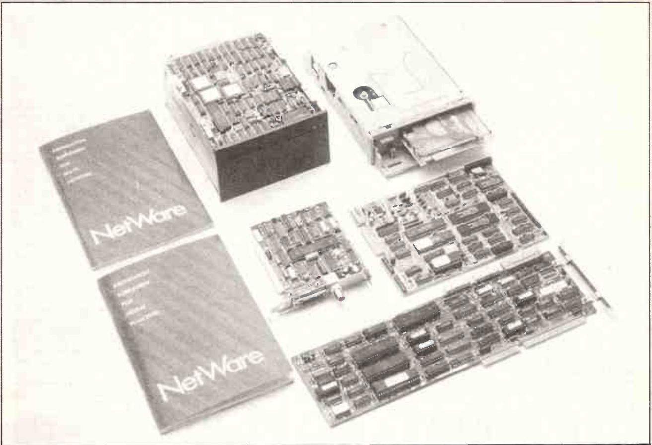
*Computer Networks distribute cards that allow up to 50 users to join together in a local area network.*
