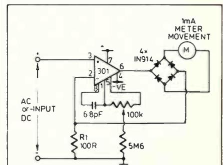
Figure 3: An ac/dc mV meter
