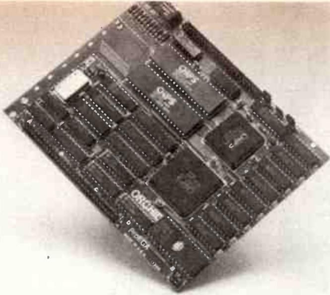
A recent development in increasing the flexibility of pcs has been the advent of multi-function cards. Often using the latest in surface mounting and large scale integration they allow a number of different and unrelated functions to take place on one card. The consequence of this is that the slots on the pc motherboard don't fill up quite as fast as they would otherwise.
