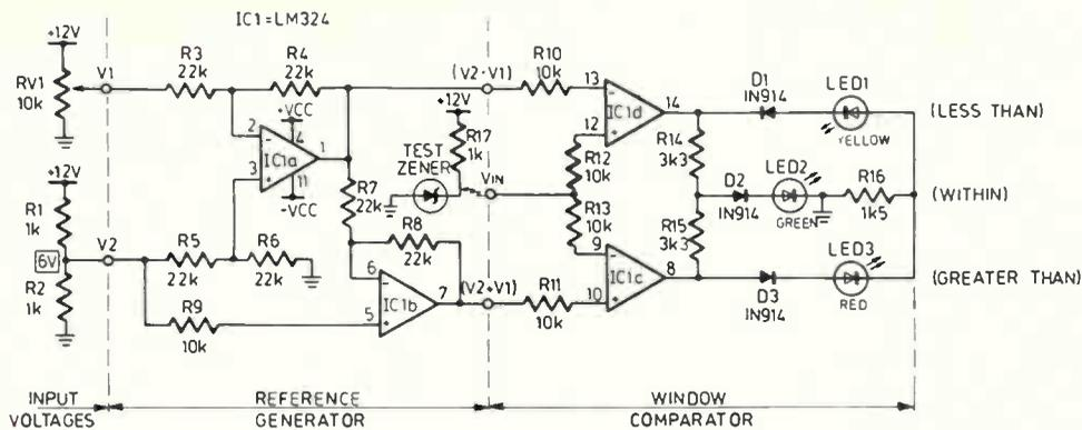
Figure 6: A window comparator with a reference generator
