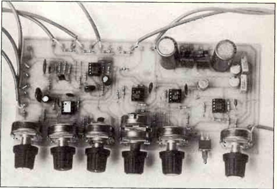
the component overlay. Do not as yet insert the IC's themselves. Insert and solder in the pc mount pots and switch, making sure that they sit firmly and parallel to the pc board. The +/- 12 V regulators (IC6 and 7) are the final components to solder in, note the orientation on the overlay.
