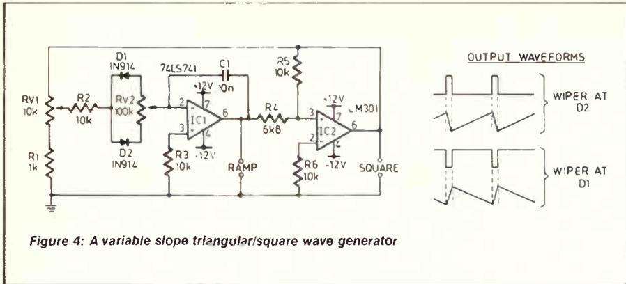
Figure 4: A variable slope triangular/square wave generator
