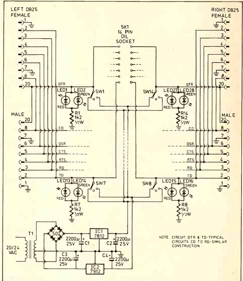
For DTE devices set all lines in centre position, set CD line on both sides to +12 V. bridge TD to RD opposite side on both sides. bridge RTS to CTS opposite side on both sides. bridge DSR to DTR opposite side on both sides.
