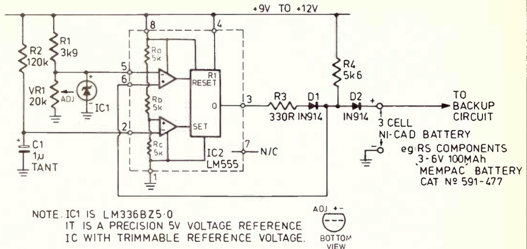
go low, turning off the main charge current. Trickle charging is then maintained via R4 and D2.
