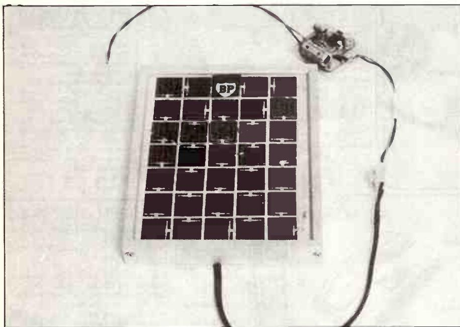
THE ETI-569 Solar Charger is designed to charge any standard 12 V lead acid car battery in any area where mains power is unavailable. It is ideal for remote data acquisition stations, caravans and boats.
