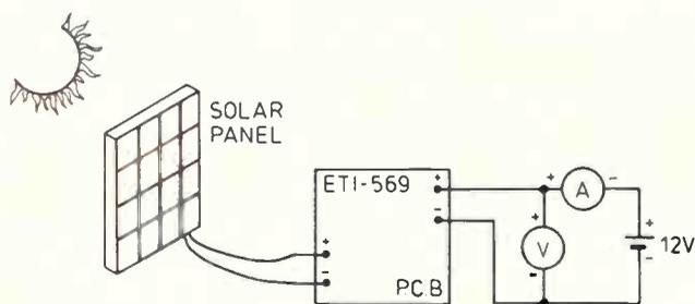
Figure 2: Test set up for the ETI-469.
