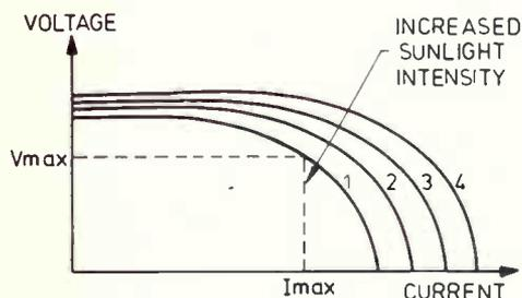
Figure 1: Voltage and current output at various light intensities.
