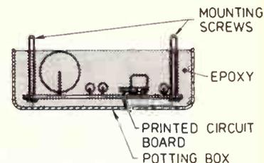
Figure 3: Schematic diagram of the potted box.
