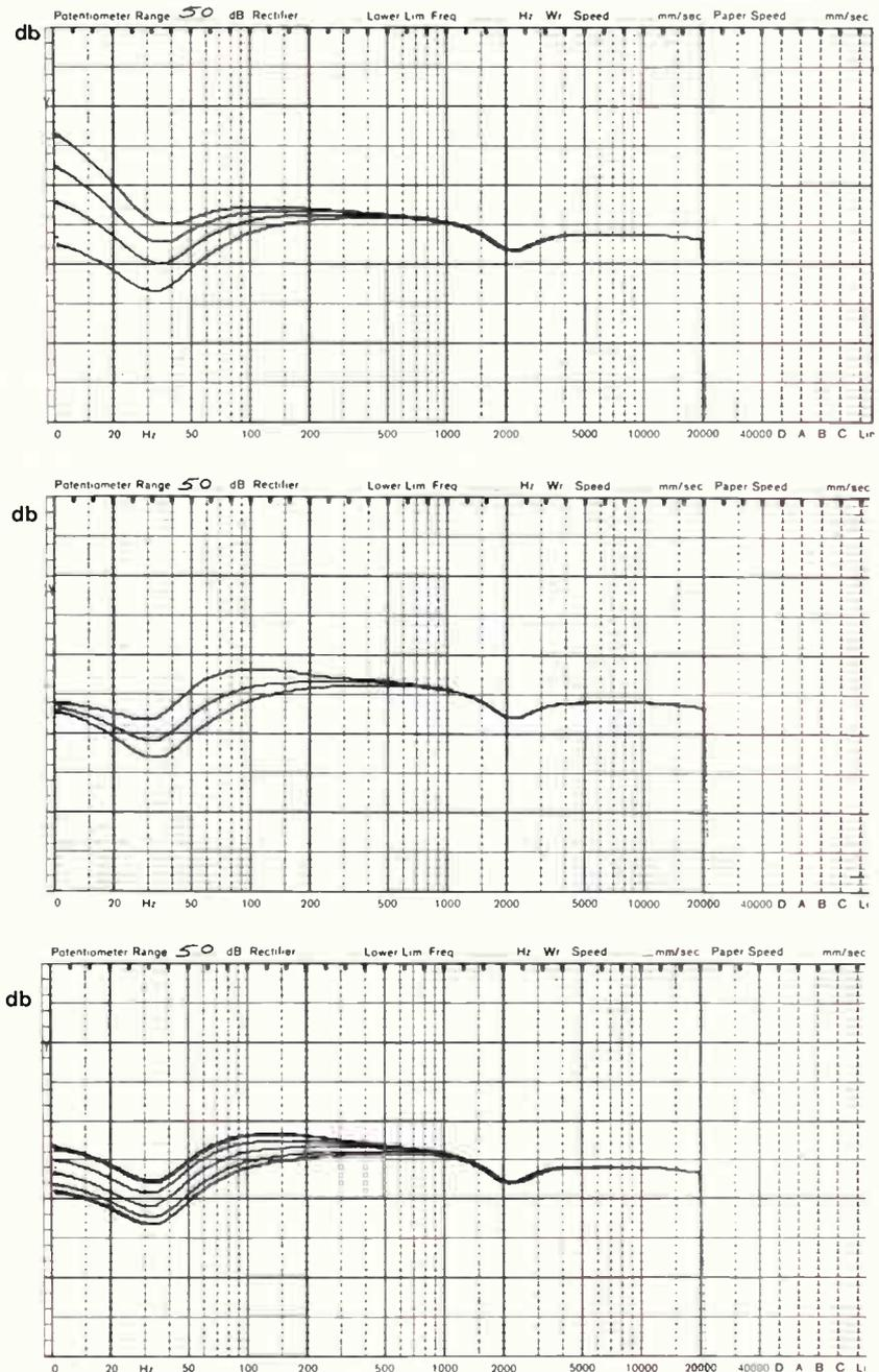
Performance of the Kube Low Frequency Equaliser. The top graph shows low end boost with Q = 0.3. The middle graph shows the effect of changing the Q and at bottom is a Q of 0.5 with differing contour settings.
