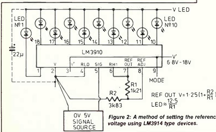
Figure 2: A method of setting the reference voltage using LM3914 type devices.
