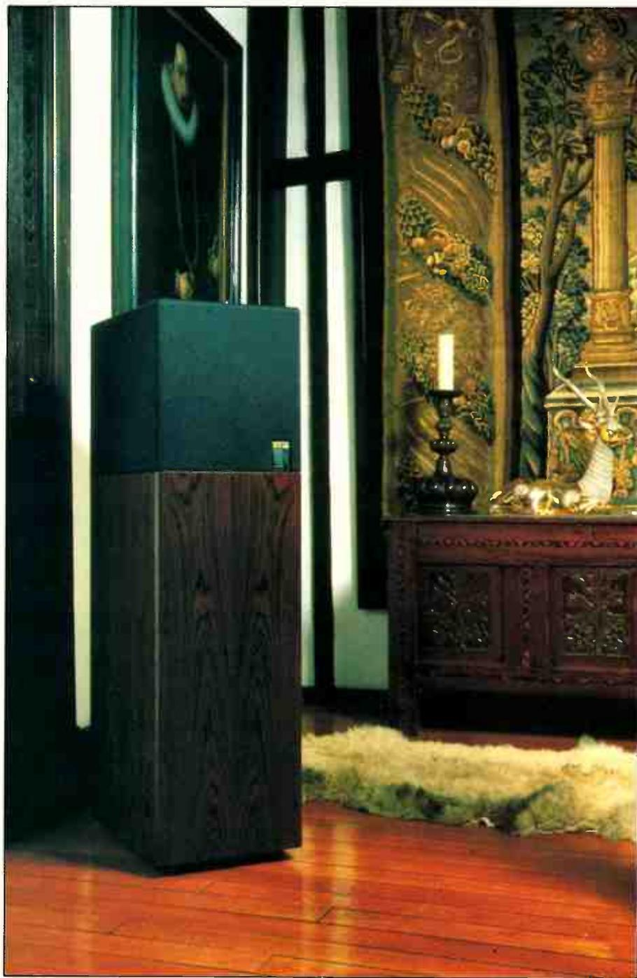
THE INNOCUOUS FRONTAL appearance of these speakers really belies their potential. It uses an unusually tall main cabinet which is beautifully finished with thick walnut veneer. The main cabinet has a volume of 72 litres and utilises the same twin coupled cavity base loading system that KEF previously developed for their 104/2 series speakers (see ETI Dec '84).
