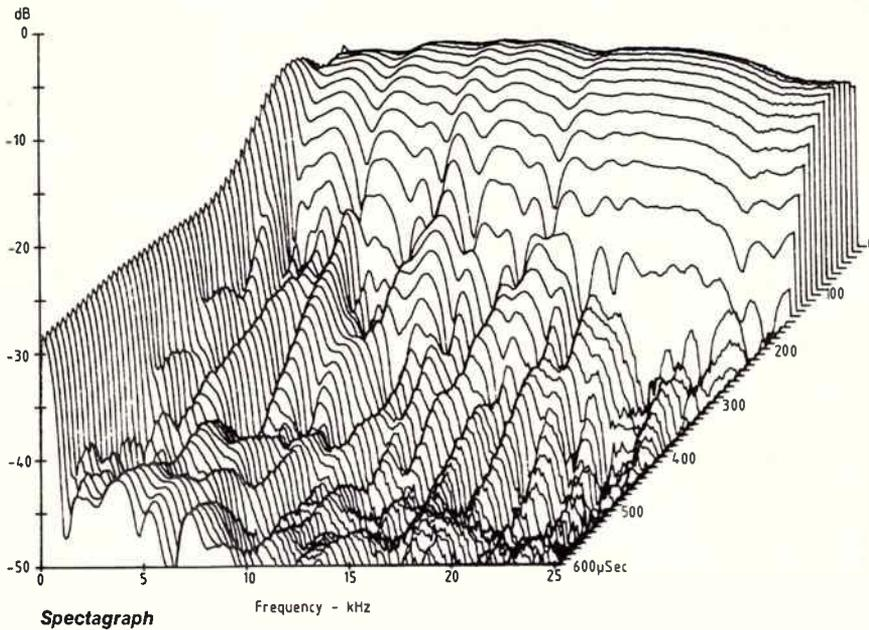
distortion at 1 kHz was somewhat higher at 3.3% and again symptomatic of the colouration at that frequency. The high frequency distortion is quite low and the tweeter's performance is extremely good.
