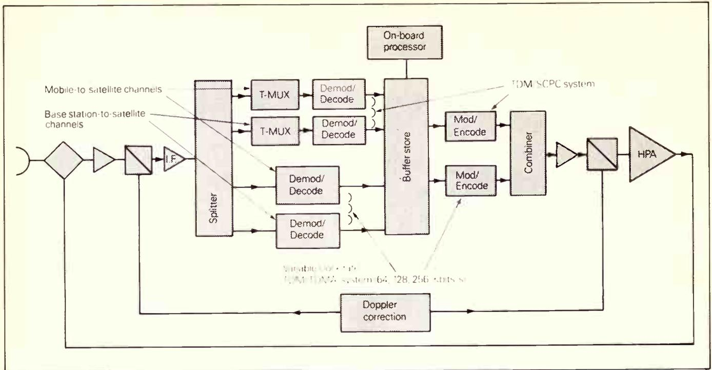
Proposed scheme for the satellite-borne payload to be used for communication with mobile and base stations.
