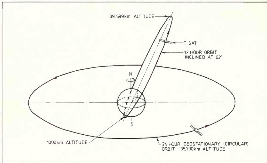
*The Molniya satellite orbit compared with the geostationary (circular) orbit.*
