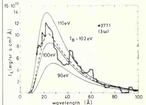
Figure 6: Measured spectrum of the radiation in the gold cavity is observed through a diagnostic hole. For comparison ideal Planckian spectra of different temperatures are shown. The dashed Planckian with a temperature of 102 eV fits the measured spectrum best.
