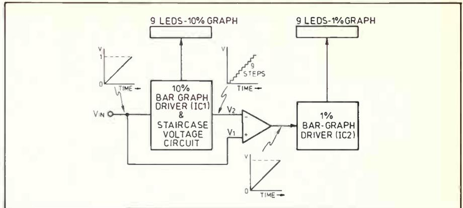
Figure 1: ETI 180 block diagram.
