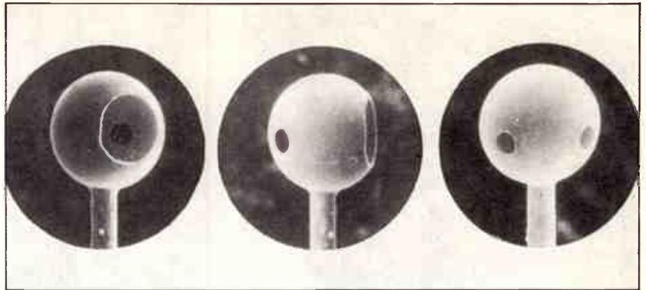
Figure 5: Three different views of a spherical gold cavity (diameter 280  $\mu\text{m}$ , wall thickness 2  $\mu\text{m}$ ). The laser radiation is injected through the large hole. The radiation inside the cavity is observed through the two smaller diagnostic holes.
