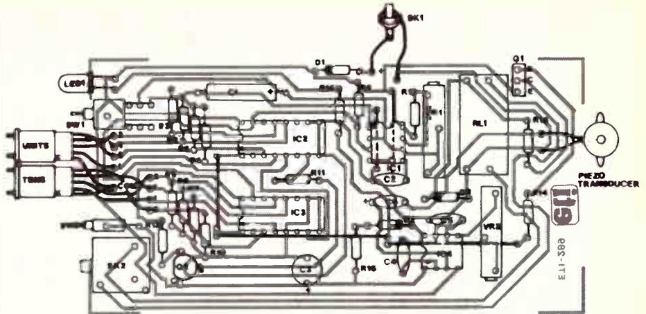
Adjust VR1 to approximately 6k2. Mount IC4, C4, C6, C5, VR2, C3, LED1, R15 and R16. Check the polarity of C6 and LED1. Attach the piezo transducer. Use long leads to do this. Power up the board and place a digital watch over the transducer. Activate the alarm. Adjust VR2 until
