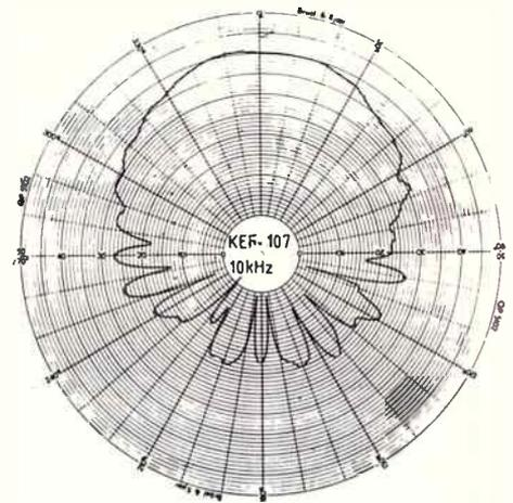
Polar diagrams at 1 kHz (left) and 10 kHz (right).
