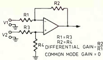
Figure 4: Differential amplifier implemented with an op-amp.
