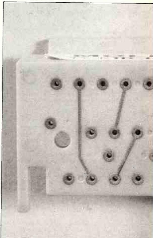
Right angle moulding of a double sided board for a simple switching device.
