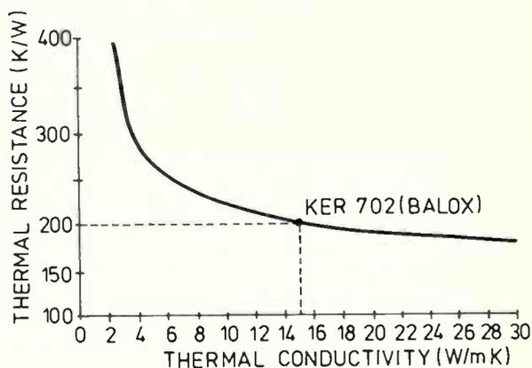
Figure 4. Thermal resistance versus Thermal conductivity.
