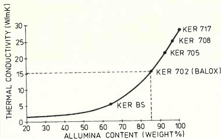
Figure 3. Thermal conductivity versus Alumina content.
