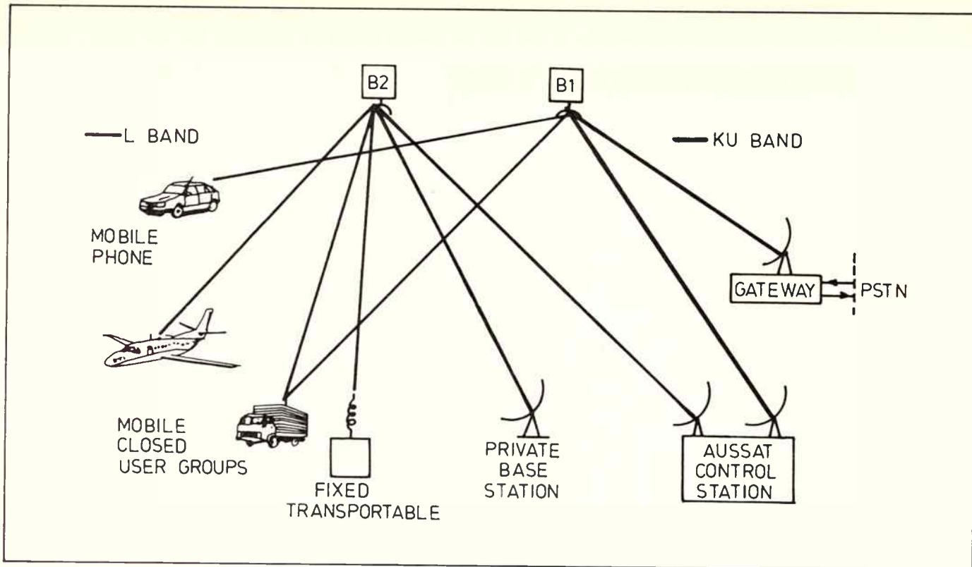
Figure 1: System Configuration
