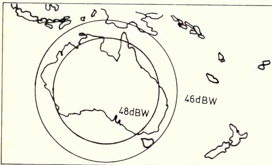
Figure 2: Proposed L band Coverage of Australia
