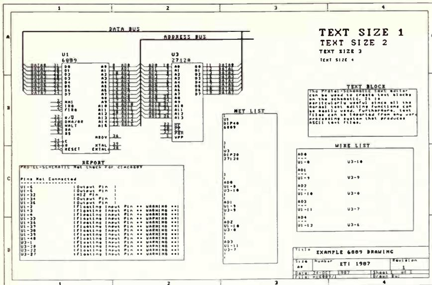
Figure 3: A Protel schematic with report, netlist and wiring file. These files were inserted into predetermined text.
