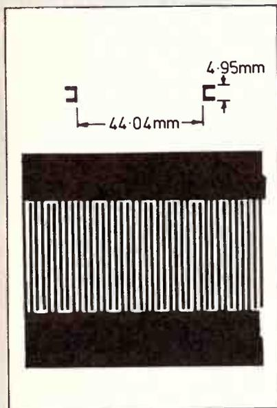
Fig 2. Surface Acoustic Wave Device showing transducer detail.
