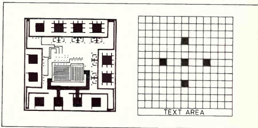
Fig. 1 Producing the mask. Dark chips are Process Control Modules.
