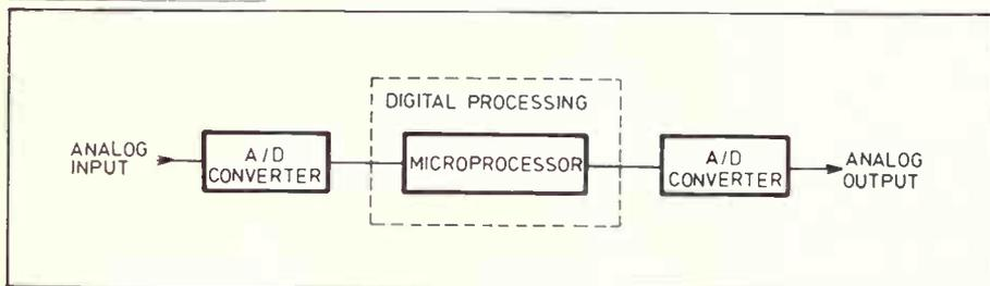
Figure 1: Basic block diagram of a digital processing system
