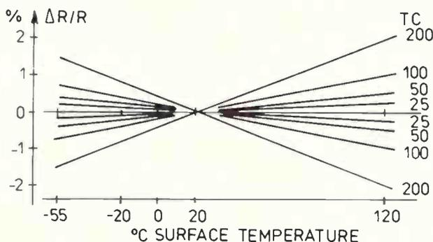
Figure 6. Possible shape of characteristic for a given thermal conductivity.
