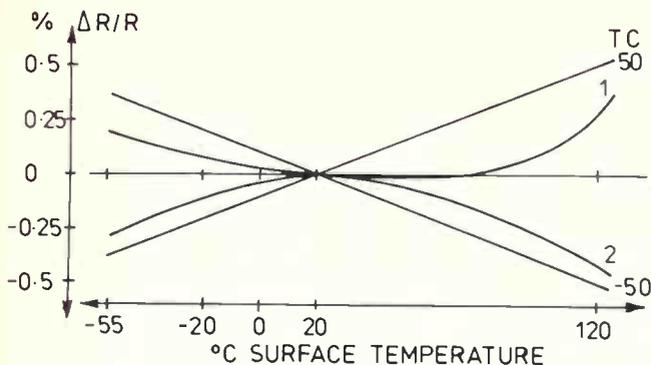
Figure 5: Change of resistance with surface temperature. The temperature co-efficient is given by the straight lines.
