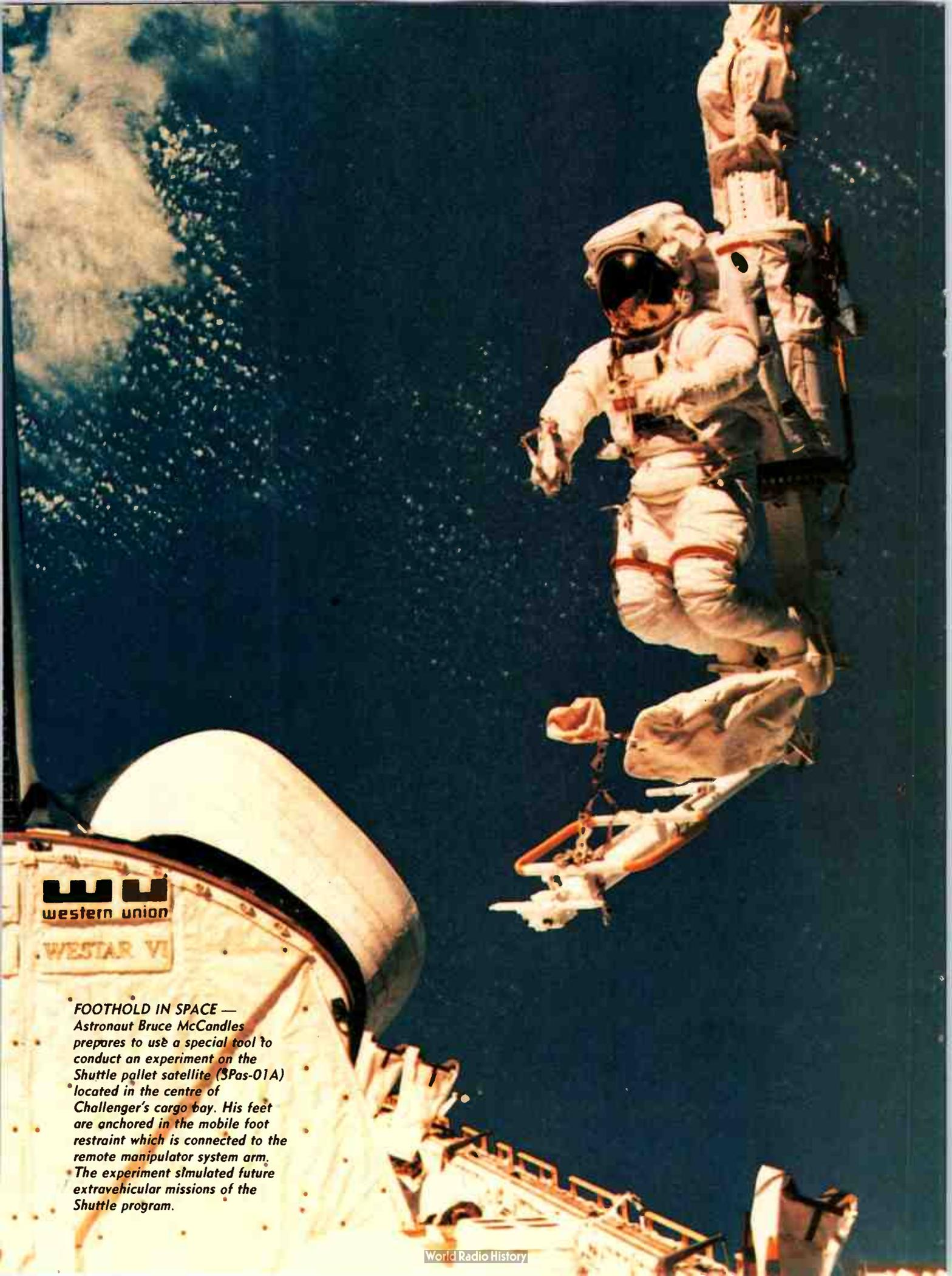
**FOOTHOLD IN SPACE** — Astronaut Bruce McCandless prepares to use a special tool to conduct an experiment on the Shuttle pallet satellite (SPas-01A) located in the centre of Challenger's cargo bay. His feet are anchored in the mobile foot restraint which is connected to the remote manipulator system arm. The experiment simulated future extravehicular missions of the Shuttle program.
