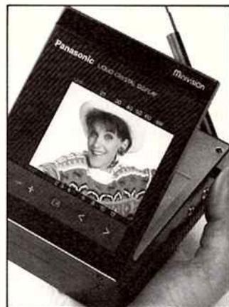
type has 308,160 pixels, with contrast ratio of 100:1. Horizontal viewing angle is 60 degrees, up is 20 down is 30.
