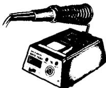
Sold in all states, may constitute a safety risk as the power switch in some units has been found to be incorrectly wired. The units which may be affected are fitted with a meter having a white, translucent background and bear the legend "AUST DES REG NO 86081" on the front nameplate below the temperature control.
