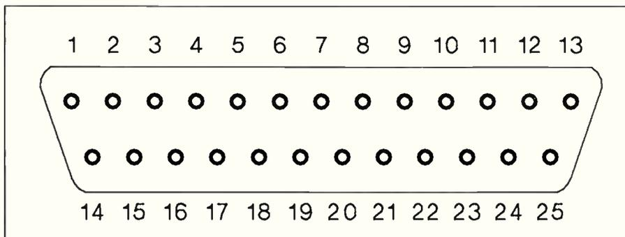
**The 25-pin D connector arrangement, looking at the pins of a plug or the connections (rear) of a socket.**
