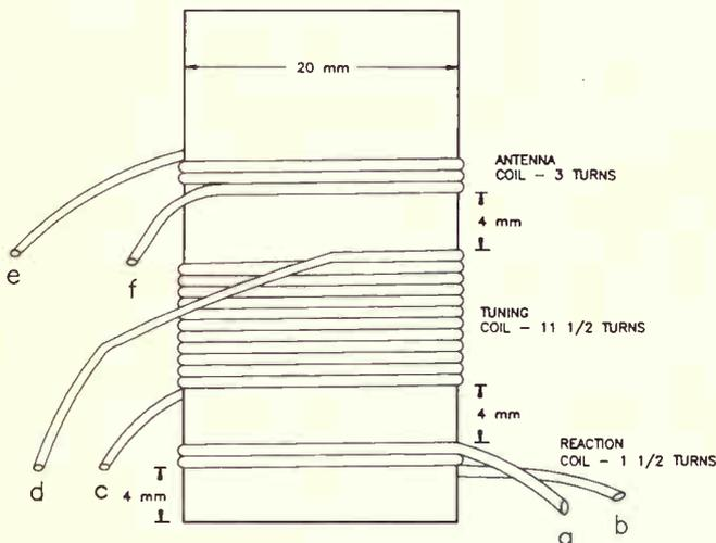
**Figure 2:** coil winding details. Use 20 gauge enamelled copper wire. All turns are wound next to one another (closewound).
