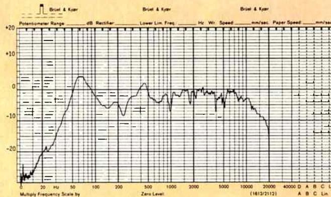
**Frequency response measured 30° off tweeter axis with control at mid position.**
