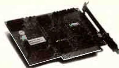
Pinpointing component problems in IBM compatible motherboards can take hours. Usually the whole system has to be working to isolate the troubled area. But not so with the new Postcard Diagnostic Module. So no other cards are necessary to test a bare motherboard.
