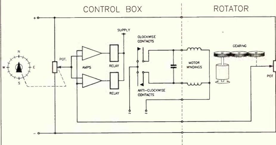
Figure 6: the more sophisticated style of control/indicator unit has a schematic rather like this, known as a balance-type circuit. Heavy duty and some medium duty rotators sport control/indicator units of this type.
