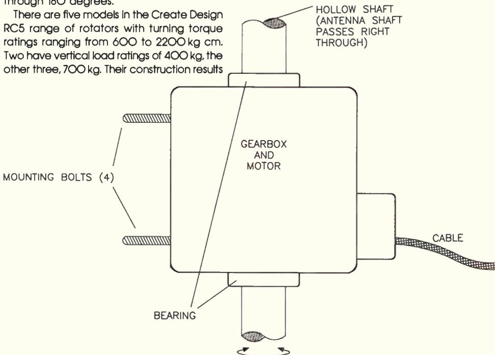
**Figure 3: this through-shaft type of rotator is less common than the other two, more often seen as an elevation rotator, for satellite antenna systems. The antenna shaft passes right through the gearbox and motor housing, with shaft clamping arrangements adjacent to the bearings at each end.**
