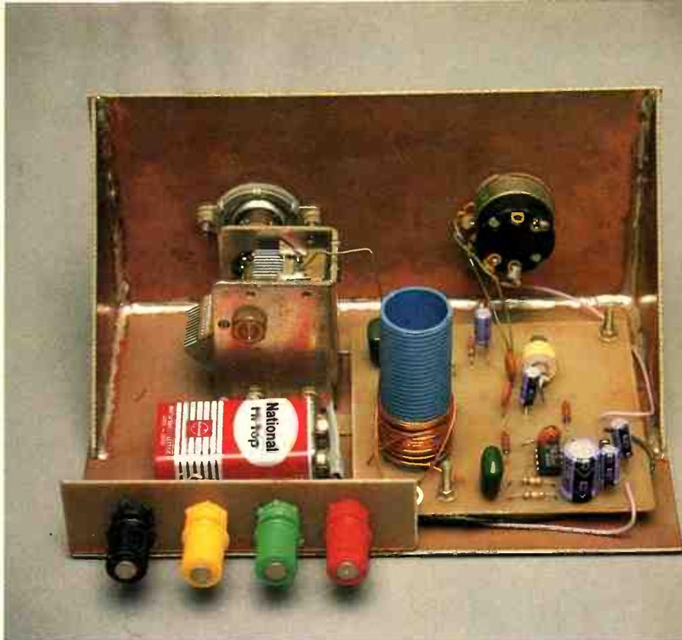
**Inside view of the shortwave receiver, showing the general assembly details.**
