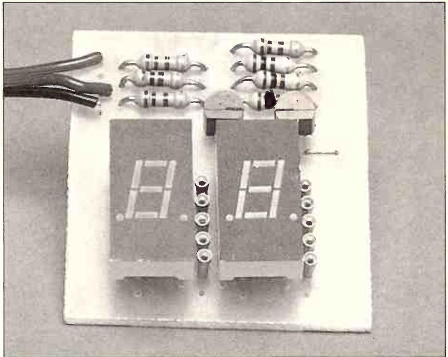
*View of the completed display board. From this you can see how the LT313 7-segment displays are oriented. Note that this prototype requires an inverted input (explained in the text).*
