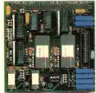
Analog output modules: 2 or 8 channel. 12 or 16 bits,  $V_0$  or  $I_0$ .
