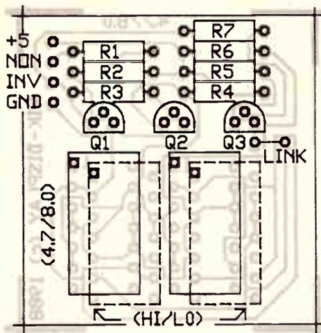
Overlay, showing the component positions. Note that Q1, R1 and R2 are optional. Note also the two possible positions for the LT313 7-segment displays. The solid lines indicate the placement for a "4.7/8.0" display, the broken lines indicate the placement for a "HI/LO" display.
