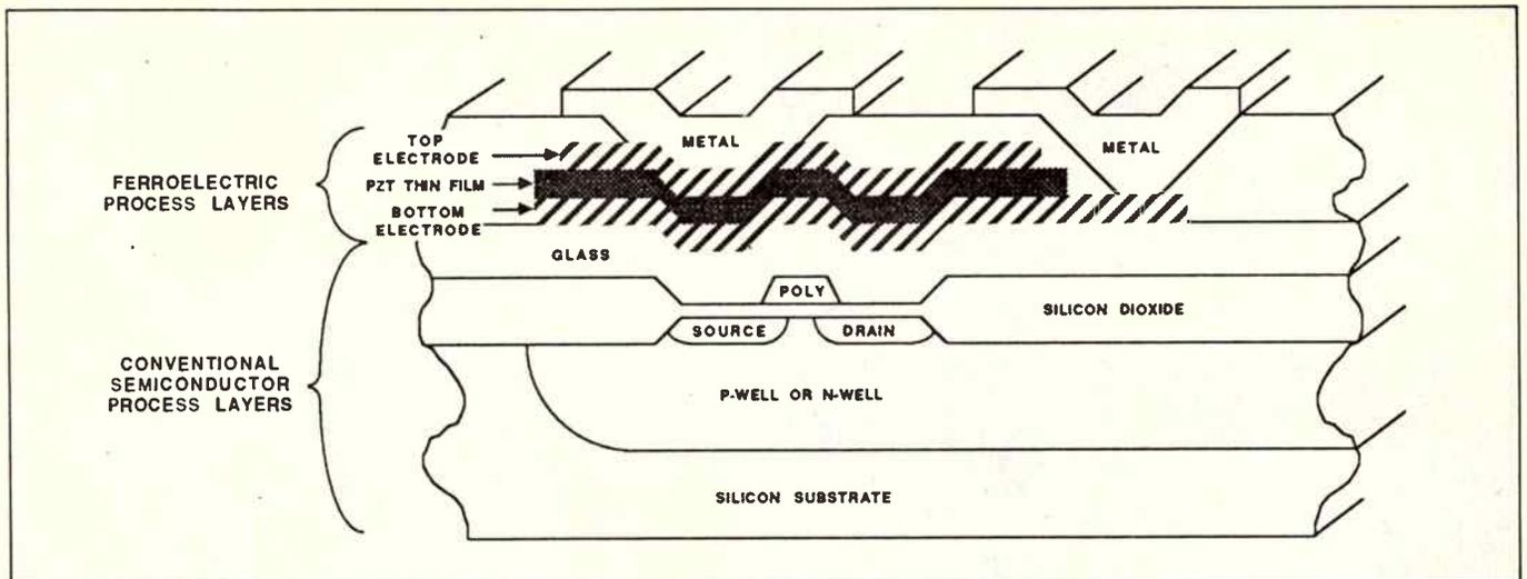
Figure 2: PZT thin film on CMOS.
