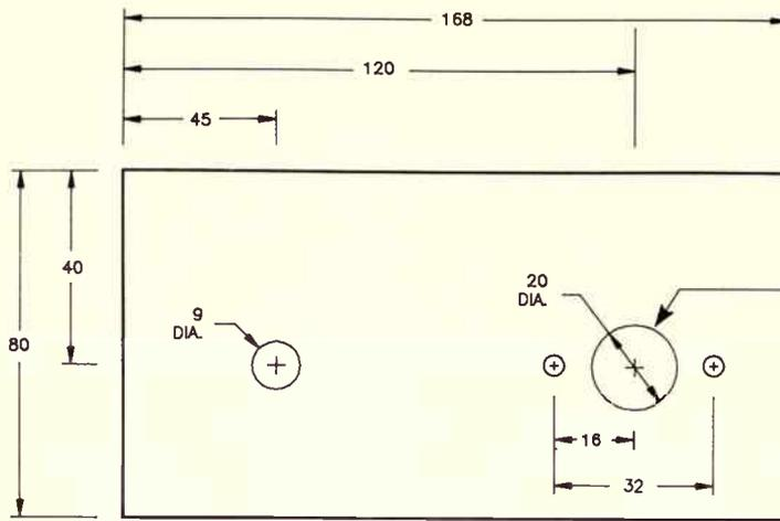
FRONT PANEL DRILLING DETAILS
