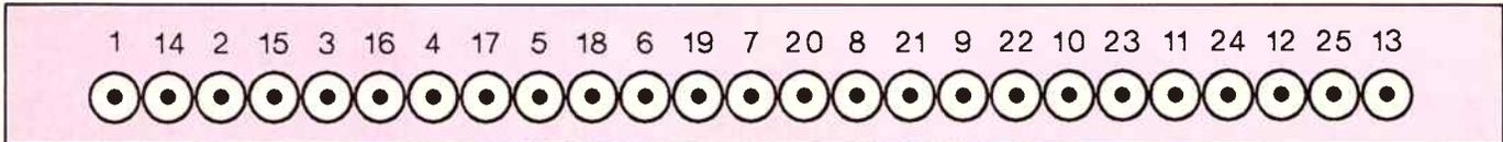
*Now that "ribbon cable" abounds and 25-pin D insulation-displacement connectors, or IDC plugs and sockets, have become relatively cheap and widely available, you often see them used in serial interface applications, particularly between computers and their peripherals, like modems, printers and plotters. Where such connectors are used, the pins connect to alternate lines in the cable, as shown here. A trap for the unwary or uninitiated!*
