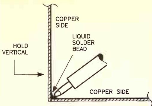
**Figure 1:** once the cabinet pieces are tacked together, a fillet of solder is run along each of the mating edges as shown here, making sure the iron tip heats both edges such that the tinning you put on initially liquifies. Touch the solder to the iron tip where it meets the two faces so that a liquid solder bead forms, then slowly run the iron along the joint.
