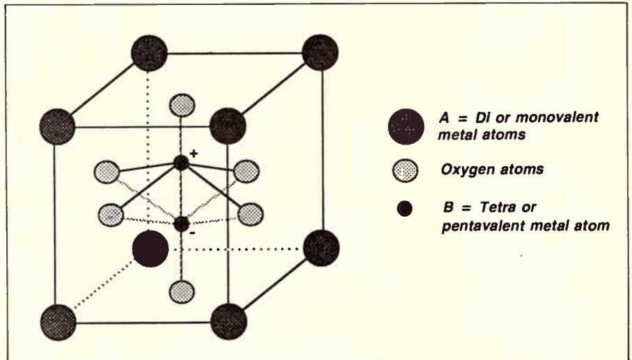
Figure 1: simplified ferroelectric molecule type  $ABO_3$ .
