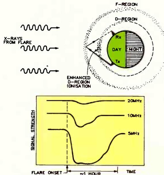
Figure 5. How X-rays from a flare affect HF signals, causing a shortwave fadeout on the dayside ionosphere. Note how the lower frequencies are affected most. The X-rays cause a sudden, large increase in ionisation in the ionosphere's D-layer, which increases absorption of the signals.
