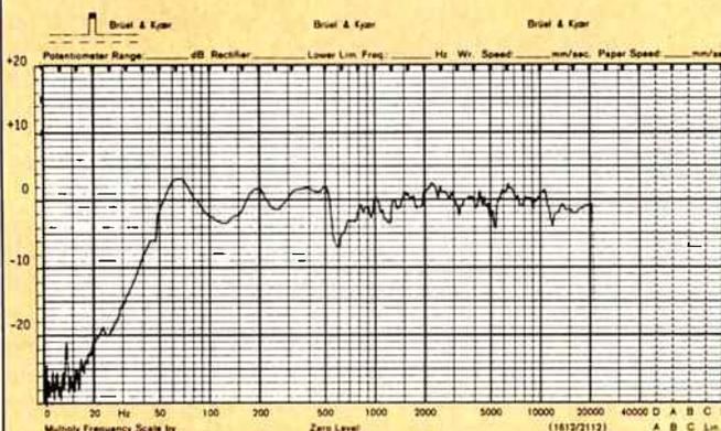
**Frequency response measured on tweeter axis with controls at mid position.**
