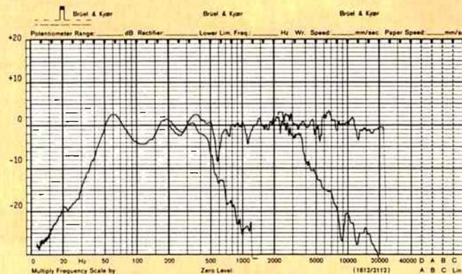
**Frequency response measured on tweeter axis showing effect of mid and treble controls at max 4.**
