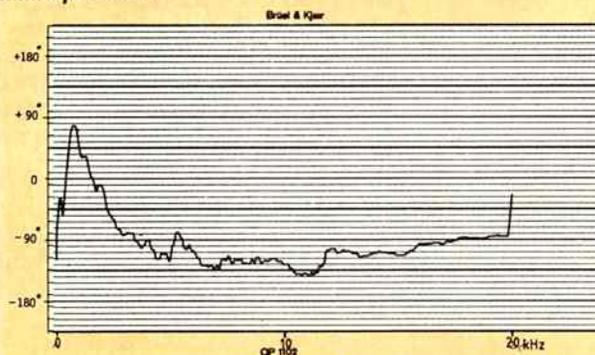
**Phase response measured at 2M on tweeter axis with controls set at normal.**
