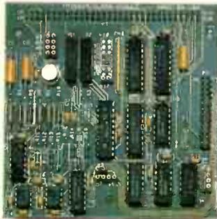
Special function modules: trigger/ alarm, simultaneous sample/hold.
