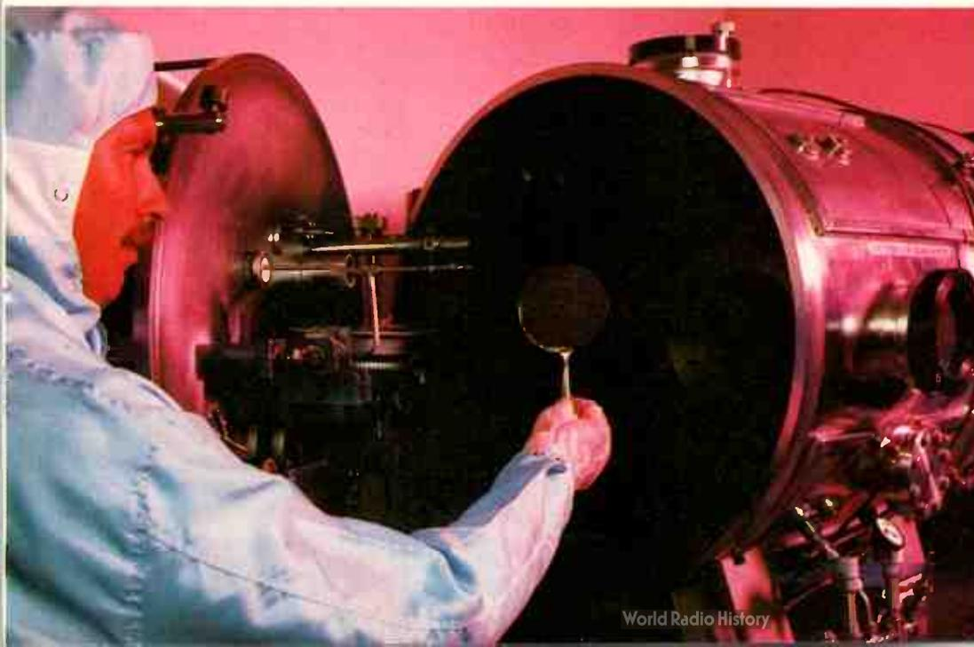
**ABOVE:** Ramtron's proprietary process involves adding a layer of ferroelectric lead-zirconate-titanate (PZT) to the existing semiconductor underlayers. **LEFT:** In Ramtron's class 100 clean room facility, standard semiconductor development and fabrication techniques are used to incorporate ferroelectric materials onto silicon wafers.
