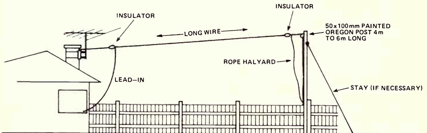
Figure 3: a useful long wire antenna for your shortwave receiver. You can use hookup wire, for economy. The insulators can be egg insulators obtainable at electronics stores.
