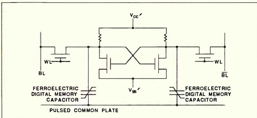
Figure 3: Ferroelectric memory based cell.
