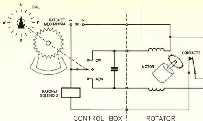
**Figure 4: simplified schematic of the simplest, lowest-cost style of control/indicator unit, employing a ratchet-and-solenoid escapement mechanism. Light duty "TV-type" antenna rotators have control/indicator units of this type.**
